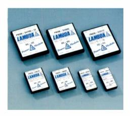
Lambda's low cost PM Series DC-DC converters conform to industry-standard pin-outs and a lower profile of 8.5mm, allowing direct replacement in existing systems. With UL, CSA, VDE, BABT, Bellcore and ETSI approvals, they're ideal for telecommunications applications. There are 96 single, dual, and triple output models with 12V, 24V, and 48V inputs, all incorporating EMI filtering. The PM Series is available from stock with four week production delivery.
