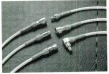
cable has a power-handling capacity of 490 W CW at 5 GHz, RF shielding of at least -100 dB at 1 GHz, and an operating temperature range of -65° to 165° C.
