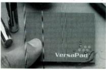
rather than the electrical capacitance of current touchpads. The semiconductive touchpad requires about 85% less power, operates in wet or dry environments, supports stylus pointing, and allows signature capture. The touchpad works with a fingertip, gloves, or a stylus. An OEM development kit is available now for \$150.
