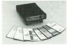
grammable, and UV-EPROM cards from most major manufacturers. The device, which complies with PCMCIA and JEIDA standards, can be used for memory-card duplication. The IC Card Drive connects to the host system through a serial or parallel interface. A 6-ft. serial cable is bundled with the 15-oz. drive. Automatic baud-rate selection is available from 1200 to 115,200 baud. Available now, it sells for \$795.
