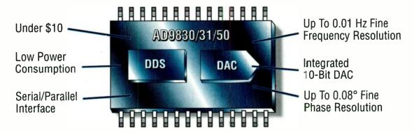
Now you don't have to sacrifice price and power for the fine frequency resolution and phase control associated with DDS solutions. Analog Devices' AD9830, AD9831 and AD9850 are leading a revolution for digital frequency synthesizers that will replace your analog alternatives.
