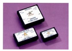
For low power (1.5W to 6W) applications, Lambda's low profile, low cost PP Series is an ideal solution. They have industry-standard pin-outs, a height of only 8mm and are available in single and dual outputs with 5, 12/15, 24 and 48 volt inputs.
