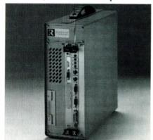
a universal-input, 80-W power supply, and is cooled by a dc fan above the boards. EMC compliance is ensured through the use of in-line mains filtering, a VDE Level-A power supply, and conductive panels with overlapping joint fingers. The larger ES-10 and ES-20 models are 500 mm deep and come with a 10- or 20-slot backplane powered by a 450- or 750-W supply. Pricing for an ES-3 enclosure starts at \$2,300 and delivery is four to six weeks ARO.
