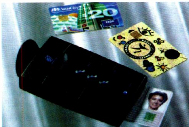
Fig. 2 This pocket-sized viewer from French smart-card maker Gemplus uses the Motorola Vituo Vue as an eyepiece display. The viewer is slightly bigger than the smart cards it's meant to be used with.
