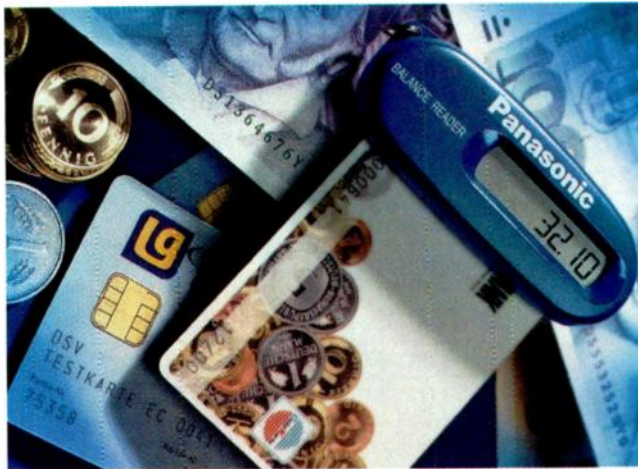
2. A balance has been written onto a processor chip within this card to be spent at special terminals. Over 50 million money cards have been in circulation since the summer of 1996.
