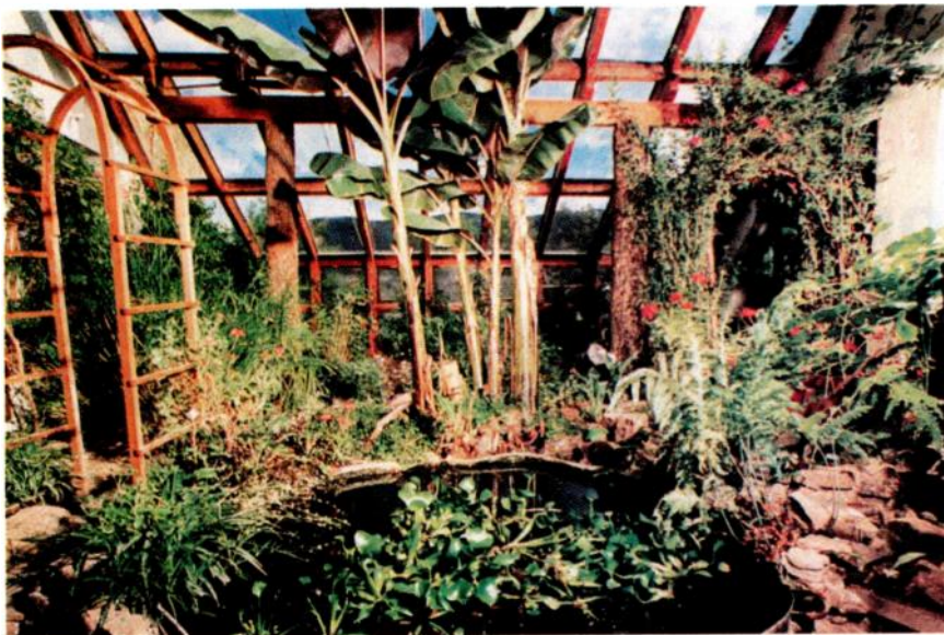
2. The heart of the RMI heating system is this solar greenhouse which also serves as a warm, green haven during the harsh Colorado winters, where temperatures drop to as low as 46° below zero. A small wood stove serves as a backup heater for the entire building.
