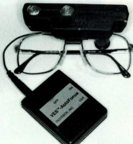
Weighing less than three ounces, the VES-EF auto-focus telescope attaches to an ordinary pair of glasses (with modified lenses) to provide enhanced eyesight for many visually-impaired people. The compact system contains a set of high-performance optics, an infrared ranging system, and a stepper motor-driven, auto-focus mechanism.
