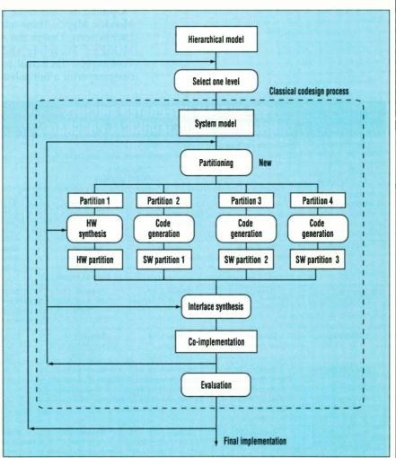
1. By enhancing the typical codesign methodology through the addition of multiple partitioning stages to more efficiently explore the design space, the scheme developed by the Ecole Polytechnique of Montreal and Mentor Graphics provides a means to better analyze the design alternatives and find the most optimal solution.
