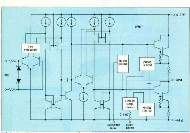
2. The Burr-Brown OPA547 op amp sports user-programmable current limits which can be set digitally by connecting a voltage or current DAC to the current-limit-set pin. The status of the thermal shutdown circuit is another feature available to users.
