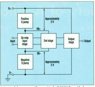
op amp, drop it in, and forget 2. A pair of charge pumps (Q pumps) in the MAX4162 provide the op about any circuit design. And amp with rail-to-rail input specifications by boosting the plus and minus most applications require supply rails (V+ and V-) by approximately 2 V.
