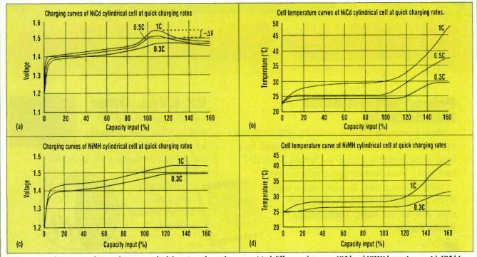
3. From an application standpoint, charging methodology is perhaps the most critical difference between NiCd and NiMH batteries — with NiCd (a and b) being considerably more tolerant of overcharge than NiMH (c and d). Constant-current charging is recommended for both types, and the highest capacity is attained by charging to about 150% of charge input. Excessive heat or internal pressure build up (overcharge beyond the oxygen recombination ability) must be avoided in both cases.
