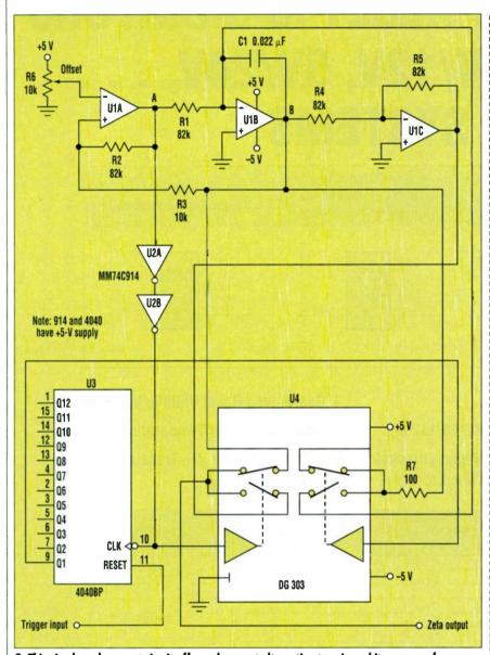
2. This simple and compact circuit offers a low-cost alternative to using arbitrary waveform generators for producing Zeta waveforms.
