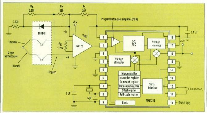
1. A thermocouple can be interfaced with an instrumentation amplifier and a  $\Delta$ - $\Sigma$  ADC to achieve 21-bit accuracy for a full-scale input range of 50 mV. the cold-junction compensation circuit shown uses a diode an a resistive network on an isothermal block.
