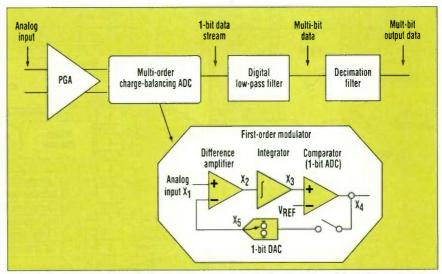
2. Block diagram of a generic high-performance  $\Delta$ - $\Sigma$  ADC. This type of modulator has an input programmable-gain amplifier that's followed by a multi-order charge-balancing section that performs the first step in low-frequency noise-reduction, and digitizes the signal ones and zeros. This stage is followed by a digital low-pass filter.
