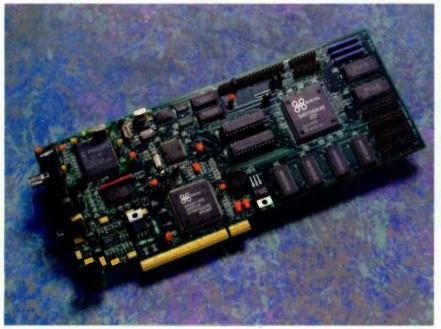
2. The VCP Video Communication Processor from 8x8 Inc., shown here in a videoconferencing board, is a hybrid dual-processor chip that contains a 32-bit MIPS-X RISC engine that operates as a vision controller. It handles syntax decoding, system multiplexing and frame-rate conversion. Its 64-bit programmable DSP is designed to perform video processing.
