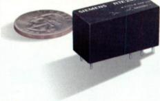
RT series relays rise only 0.62" (15.7mm) above the PC board, but they switch up to 16A at 240VAC. And they provide 8mm spacing between contacts and coil for more than 5kV isolation. That's a level of performance you might not expect from a relay this small.
