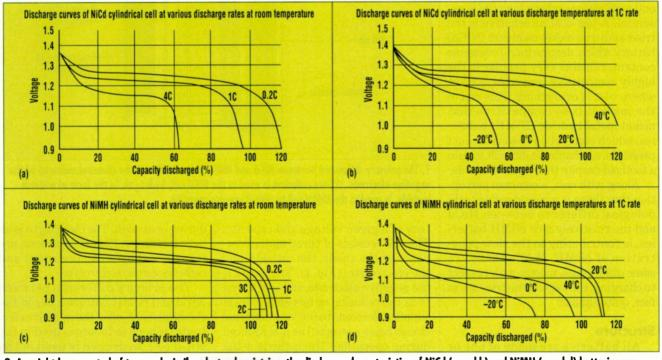
2. As might be expected of two such similar electrochemistries, the discharge characteristics of NiCd (a and b) and NiMH (c and d) batteries are essentially the same. Both types are characterized by a flat discharge profile, with a discharge voltage that is dependent on current and/or temperature. Generally, the higher the current or the lower the temperature, the lower the operating voltage.
