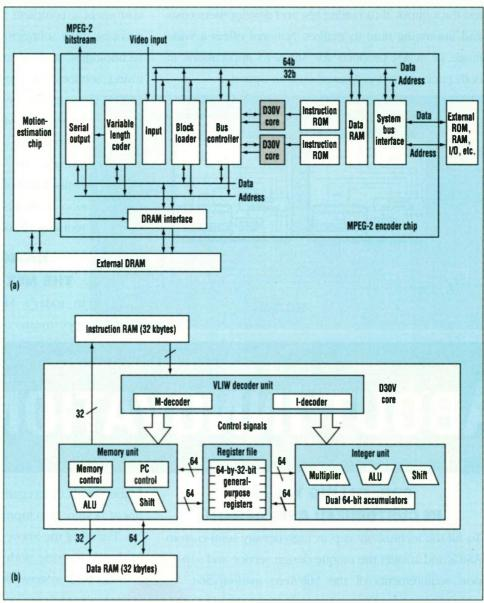
puts. That makes the logic as 4. The heart of a real-time MPEG-2 encoder/decoder chip (a) developed by Mitsubishi Electric consists of a easy to synthesize as static circuits and allows synthesis tools developed for static circuitry encoder chip to deliver a peak throughput of 1 gigaoperation per second.
