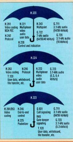
ITU developed a videoconferencing standard, H.324, designed for regular telephone lines. Approved only last year, the standard will insure that all videoconferencing systems, whether standalone or computerbased, and whether hardware- or software-driven, will be able to talk to each other. The standard specifies a common method for video, voice and data to be shared simultane-
