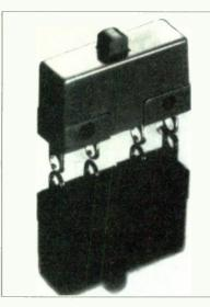
DOUBLE-BREAK SUBMINIATURE BASICS May be subminiature in size but these basics switch up to 10 amperes with 100,000 minimum cycle life; over 1 million cycle mechanical life! Constructed in accordance with MIL-S-8805/7. Precision operating points. UL recognized. Replaces ITW Switches Type 16. Ask for OTTO B5 series.
