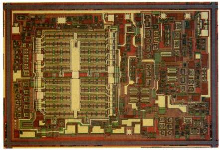
1. The two power transistors in the Burr-Brown OPA547 op amp (large blocks) each consist of 120 individual BJTs, each with an emitter ballast resistor.
