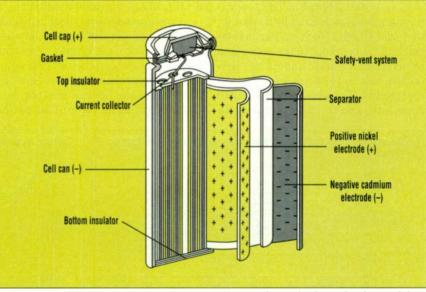
1. The primary difference between NiCd and NiMH batteries lies in the chemical make-up of the negative electrode. Where cadmium is used in the NiCd cell, hydrogen, in the form of a metal hydride, is used in the NiMH cell to give it greater capacity.
