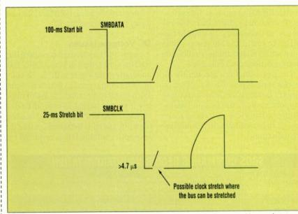
Adequate Start-bit response enables the SMBus to run at the highest possible speed. A Stretch bit allows for some devices, such as a smart-battery's microcontroller, to take more time than is available in a 100-kHz-rate data frame. PIPS
