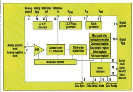
clock. The charge that's stored on  $\{5. \text{ The full representation of a } \Delta-\Sigma \text{ ADC} \text{ is shown above. Not only does this circuit digitize the these capacitors is then transferred to the second pair of capacitors C3 and the microcontroller of some overhead tasks such as offset and full-scale calibration.}$
