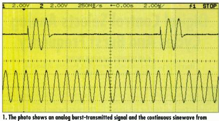
which it's derived. Only a minor amount of crossover distortion can be observed in the burstoutput waveform, which will typically have a negligible effect on the system function.
