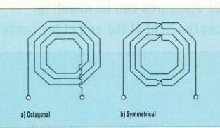
1. These on-chip inductors were developed for use in high-performance Rather than using exotic VCOs that operate in the 900- and 1800-MHz region. An octagonal techniques such as forming profile (a) yields a better inductance ratio than square profile inductors. inductors with bonding wire, The symmetrical configuration allows the use of a single inductor in a the authors applied finite-ele- perfectly balanced differential oscillator (b).
