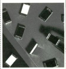
resistance range of 100 to 300  $\Omega$  and a voltage rating of 50 V. The capacitance range is 22 to 100 pF. The resistance and capacitance tolerance is 20% while maintaining a dissipation factor of 5% maximum. The chip comes on 8-mm tape with 5000 pieces/reel. Pricing is \$35 each in 1000-unit lots and delivery is 8 weeks.
