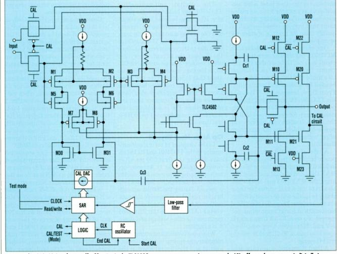
1. An on-chip SAR-ADC performs self calibration in the TLC4502 op amp at power up. It measures the IC's offset voltage, stores it digitally in a register and when calibration is complete, applies it to the CAL DAC the output of which nulls the input offset voltage via current mirror M30/M31.
