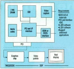
of 352 by 288 pixels, which 3. The TMS320C82 processor from Texas Instruments can be used with are specially designed to a graphics chip and video palette to implement a videoconferencing
