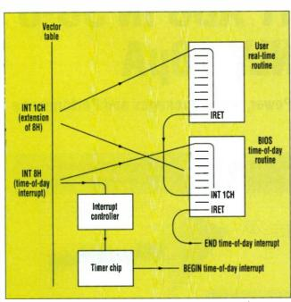
By changing the vector to point to a procedure in your particular program, a PC's "dummy" interrupt (INT 1CH) can be called 18.2 times per second for use as a real-time timing reference.
