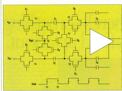
one-like a gain of two-the second rising clock edge does not transmit the signal from the second capacitor pair to the modulator section. The second pair of capacitors (C3 and C4) retain the original charge from the first sample and adds it to the charge from the second sampled input. In this manner the charge on the second pair of capacitors is approximately doubled. As the gain of the PGA stage is increased to 2, 4, 8, or 16, more time is required to fully sample the input.
