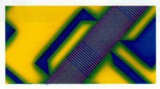
Section of a wafer for a low-loss filter.
