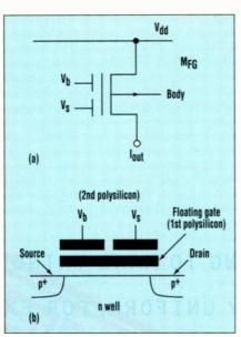
3. The University of New South Wales' floating-gate MOSFET current source in circuit form (a), and its cross-section (b). The twoinput gate structure allows for device operation in a DAC to be at less than 1 V.
