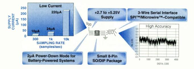
The new MAX1241 ADC is designed for 3V, 3.3V, and 5V applications. It requires only 0.9mA at 73ksps, and only 10 $\mu$ A at 300 samples/sec, which helps keep you well within your power budget in portable and battery-powered applications. The MAX1241 complements existing 4-crannel (MAX1247) and 8-channel (MAX147) devices (see table). For 10-bit applications, use the pin- and software-compatible MAX1243/MAX1249 and MAX148, which have 1, 4, and 8 channels, respectively.
