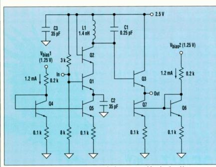
1. Fabricated with a production SiGe process, this low-noise amplifier developed by IBM operates at 6.25 GHz and exhibits a minimum noise factor of 2.2 dB and a gain of 20.4 dB.
