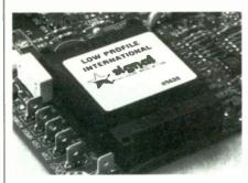
The devices are designed to meet VDE 0805, and can be interchanged with the company's Flathead Low Profile printed-circuit-mount transformers. Available in 2- and 6-VA versions, the devices have heights of 0.72 in. and 0.895 in., respectively. Output voltages range from 5 to 230 V.
