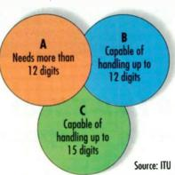
the world. Countries that failed to comply with Time T and did not expand the number-handling capacity of their equipment would only be able to make operator-assisted calls to countries that had expanded their numbering plan to 15 digits (see the figure).
