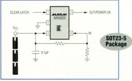
The MAX835 has a push/pull output while the MAX834 has an open-drain N-channel output driver.
