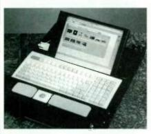
signed to replace color CRTs in standard 19-in. instrument racks, the VueMiser reduces front-panel height from 10U to 1U and power consumption from 17 to 24 W. Displays are available with resolutions from 640-by-480 to 1024-by-768 pixels. Options include keyboards, trackballs, and resistive touch screens. On-screen menus offer easy set up and adjustment. Available now, prices for the VueMiser display system start at \$3040.
