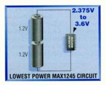
Total system current of 85mA (MAX1245 current < 1mA)</li> SPI and QSPI are trademarks of Motorola. Microwire is a trademark of National Semiconductor
