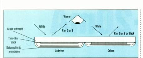
3. The IMod MEMs-based display technology is based on an optical cavity that can be deformed to change the color of the reflected light with the application of a voltage. Traditionally IMods have exhibited low power requirements, and require only passive matrix addressing.
