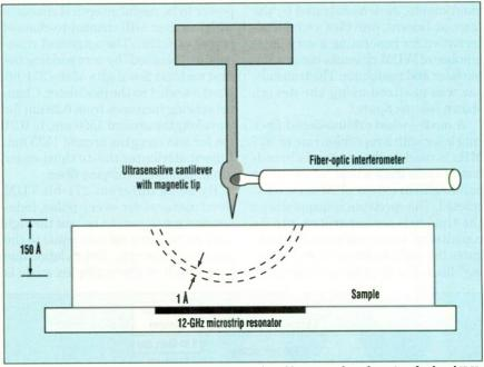
The magnetic resonance force microscope being developed by researchers from Stanford and IBM uses a microscopic silicon cantilever that allows measurement of forces in the attonewton range.
