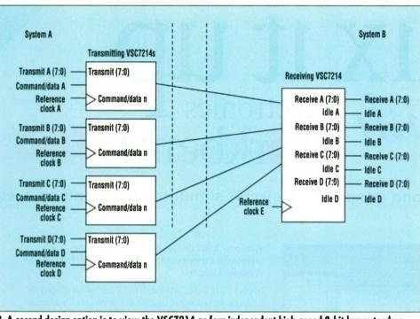
2. A second design option is to view the VSC7214 as four independent high-speed 8-bit bus extenders. Like the 32-bit bus extender, communications with another system take place over a copper cable or fiberoptic link.
