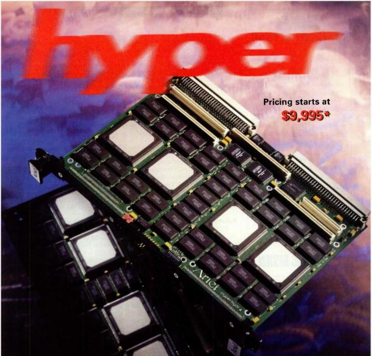
HyperHydra. It's the ultimate octal 'C44 DSP engine you knew you could expect from Ariel's Hydra family. With a symmetrical architecture designed for optimized data flow, HyperHydra couples the explosive floating-point performance of 8 TMS320C44s with Ariel's Open Hardware Architecture, featuring OpenIO support for off-the-shelf or
