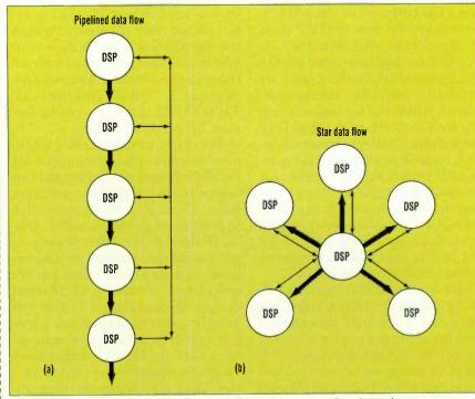
1. Two types of data-flow architecture are used in multiprocessor digital signal processing systems, pipelined (a) and star (b). Pipelining moves data in a linear flow through DSPs, while star depends on a central processor to move data among DSPs.
