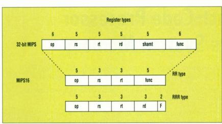
2. The 32-bit MIPS register has a 6-bit OP, three register fields (5 bits each), 5 bits for the shiftamount (SHAMT) field, and a 6-bit function that modifies the basic operation.
