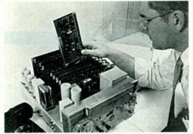
+55 C. This stable gain is achieved through dc feedback to stabilize the operating point, and ac feedback to achieve broad band-width, high input impedance and good wave form. Two models are available: Model 196 shown above is equipped with germanium transistors, suitable for environmental temperature from -55 C to +55 C, and Model 198 using silicon
