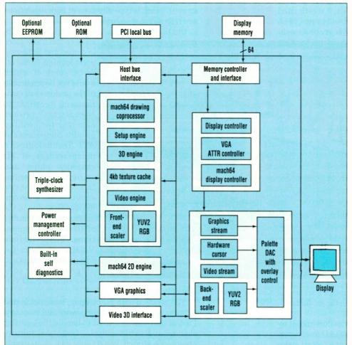
An advanced graphics controller, the 3D Rage Pro from ATI Technologies, takes full advantage of Intel's Accelerated Graphics Port (AGP) with 133-MHz operation. The chip's high performance comes from a setup engine that can process up to 1.2 million triangles/s, a rate much greater than the industry average.
