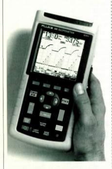
test point to another and always get a stable waveform without adjustments. A proprietary circuit continuously analyzes input signals and a microprocessor uses the information to control instrument settings. The two-channel unit displays scope waveforms and meter readings simultaneously. Users can access 26 measurement functions from a simple menu list.
