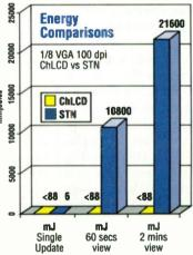
Unlike STN displays which use power to continuously refresh images, CbLCDs do not require refreshing to keep energy usage to a minimum.
