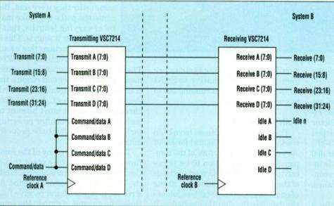
1. The VSC7214 Fibre Channel Transceiver, from Vitesse Semiconductor Corp., can operate as a 32-bit bus extender, communicating with another system over a copper cable or fiber-optic link.
