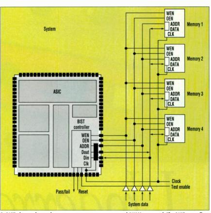
2. BIST also can be used to test system memory arrays and SIMMs at speed. The BIST controller can be placed inside one of the system's ASICs or on a reconfigured FPGA.
