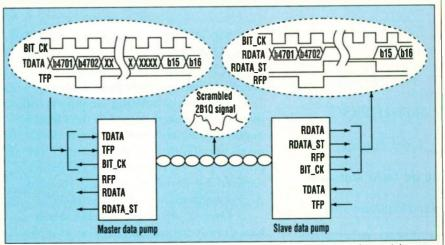
1. Level One's two-chip multi-rate DSL data pump (MDP) employs 2B1Q line coding and data scrambling to produce a signal that's robust enough to carry high-rate data across twisted-pair phone lines for up to 22,000 feet. The incoming data stream is broken down into 4688-bit-long frames, with a 14-bit frame synchronization header appended to it.
