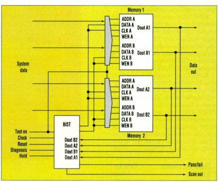
1. Designing the memory BIST controller's state machine and multiplexers into separate blocks minimizes the routing impact on the address and data lines.
