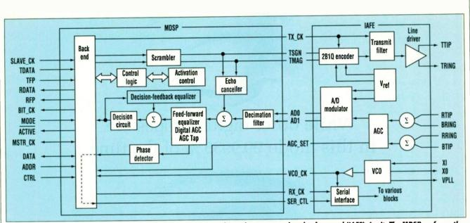
2. The MDSL transceiver consists of a specialized MDSL DSP (MDSP) chip and an integrated analog front-end (IAFE) circuit. The MDSP performs the data scrambling, adaptive equalization, and echo cancellation on the digitized signal, and extracts a bit stream. The IAFE performs all the line-interface, encoding, and clock-generation functions.
