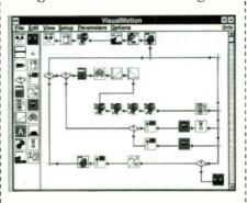
applications such as InTouch from Wonderware Software Development Corp. or Microsoft's Visual Basic programs. The interface runs on any IBM PC/AT-computer with Windows 3.1 or higher and 4 Mbytes of RAM. The user builds a motion-control sequence on-screen by clicking on applicable motion icons in a logical sequence. Each icon represents a step in the motion-control application.
