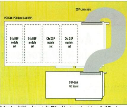
2. An external I/O board connected to DSP modules gives system designers flexibility when adapting the system to specific design tasks. Standard modules, such as Spectrum's DSP Link, provide a separate I/O bus, thus offloading the system bus.
