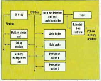
tionality of various flavors 4. The FlexLink interface connects the TinyRISC CPU to the specialized onto the network interface cores, using a building block approach. Such blocks include a bussuch that only a limited interface unit and cache controller, multiply-divide unit, extended busamount of passive analog interface unit controller, timer, write buffer, debug module, a two-way components are needed to set-associative instruction or direct-mapped cache, and a data cache.
