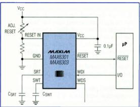
Get complete flexibility: set your timeout delays and trip thresholds as needed.
