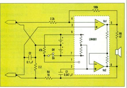
This short-circuit detector improves on an earlier Idea For Design by employing the LM4861, which ultimately makes it a much more compact, battery-powered tester.
