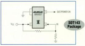
The MAX836 and MAX837 voltage monitors come in a 4-pin SOT package. They have 5mV of hysteresis and no latch.
