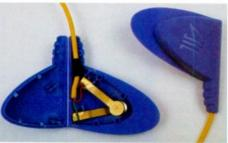
one contact is banging away at the other. Considering that this banging causes wear. Pencak decided that a base metal with a nickel plate on it would be best for the application. Previously, the Virtual Music had been using brass.
