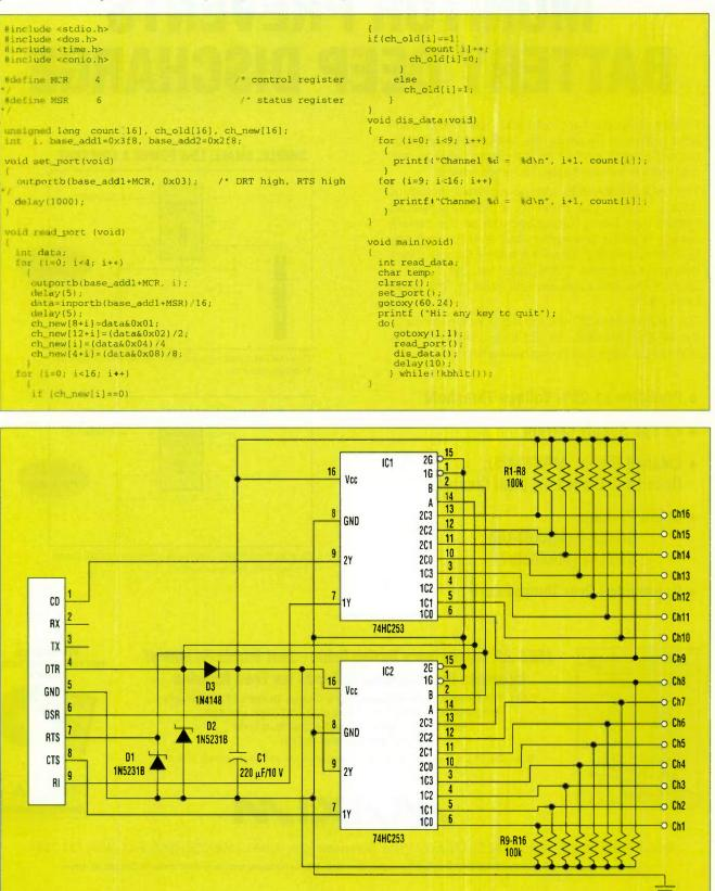
This simple data acquisition circuit allows a PC to read 16 digital inputs while deriving its power supply directly from the PC serial port.
