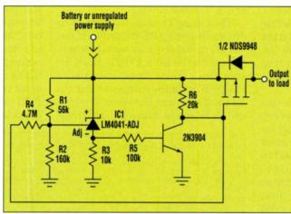
mum threshold, it's often This low-cost, space-saving circuit will shut down a portable system good practice to disconnect when the supply voltage drops below a minimum threshold.
