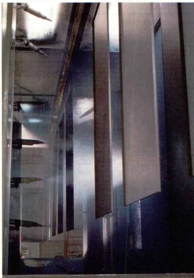
In Bud Industries' clean room, powder-coat spray guns (left) apply powder to parts (right) as they move along a conveyor belt. The company has two such spray booths which feature a series of 14 programmable guns that dispense the powder onto the parts.
