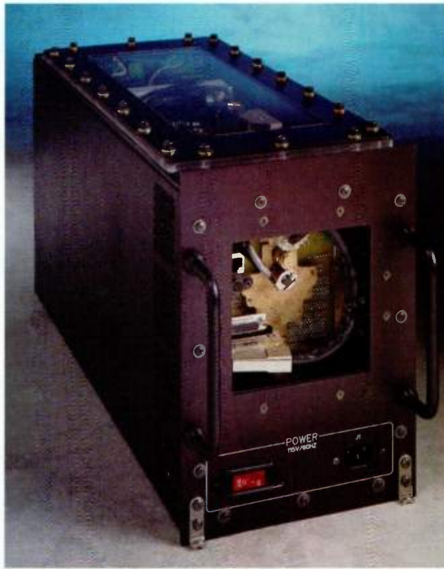
The vapor-phase cooling system mists the interior of the enclosure with a dielectric fluid that vaporizes on contact with the heated electronics. The vapor carries the heat away to the walls of the enclosure where it condenses and is recycled back into the spray. This system allows Themis to embed COTS VMEbus boards in harsh environments usually reserved for expensive, specially ruggedized boards.
