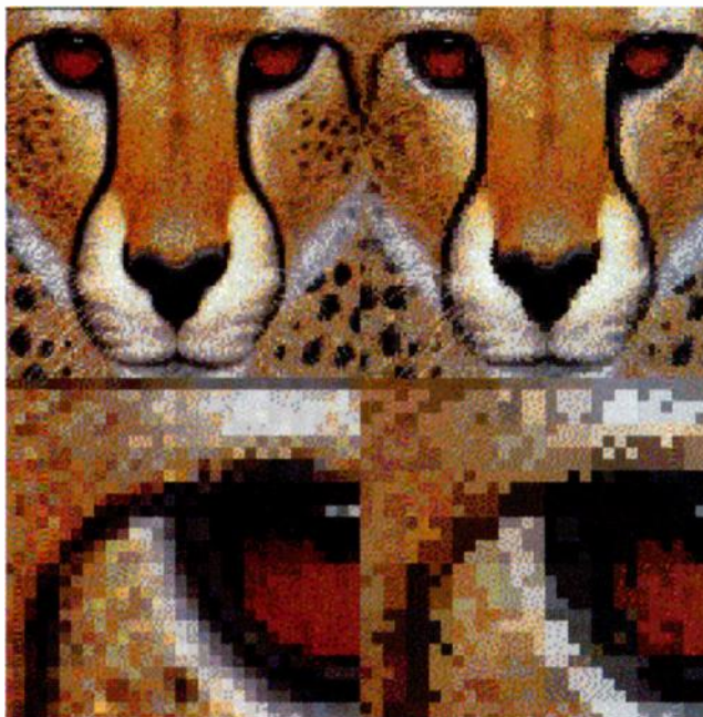
2. 3D graphics often result in extremely large images. Fortunately, full texture mip-maps can be compressed. As shown, factors of 10:1 or better are achievable with minimal texture degradation (compressed image on right).
