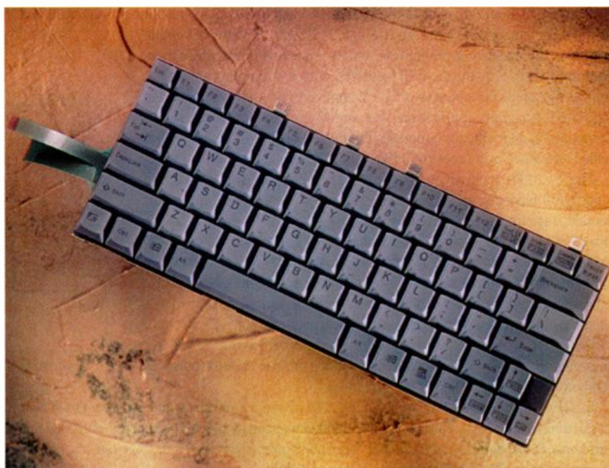
1. The FKB7600 series of 85-key keyboards has a vertical height of just 6.5 mm. However, it retains a 3-mm, full-travel keystroke by employing a gear-link mechanism in the keyswitch.
