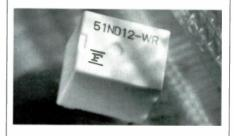
tions at 16 V dc with an in-rush current of 28 A. The relay measures 15.5 by 12.1 by 13.7 mm, weighs 6 g, and has a rated coil power of 600 mW. Pricing is \$1.19 each per 1000; delivery is from stock.
