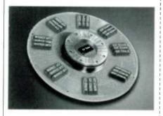
relays have a switching speed of up to 500 Hz, a contact resistance of 150 mW, and a contact rating of 10 W (typical). The dielectric strength from switch to coil and shield is 1000 V dc/peak ac. Pricing is \$2 each per 10,000.
