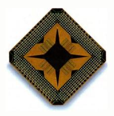
Density up to 20 million gates 300 MHz benchmarked system speed Power dissipation down to  $0.04 \,\mu\text{W/MHz/gate}$  at 2.5V Integration of DRAMs and analog circuits Volume production by Q4 '97
