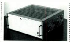
dles, and fan covers. The boxes use 14-18 Ga cold rolled steel construction and come with 1/16 to 1/8-in. aluminum front/back plates. Pricing ranges from \$50 to \$300 and delivery is from stock.
