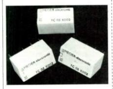
switching resistance of  $100~\text{m}\Omega$  and consume 200~mW. Constructed with gold-palladium contacts, the fully sealed 2 Form C devices are rated at 30~W at 1.25~A and have a 4-ms operate time and a 1.5-ms release time. The devices are UL/CSA and BT approved. Pricing is from \$1.25 each per 10,000.
