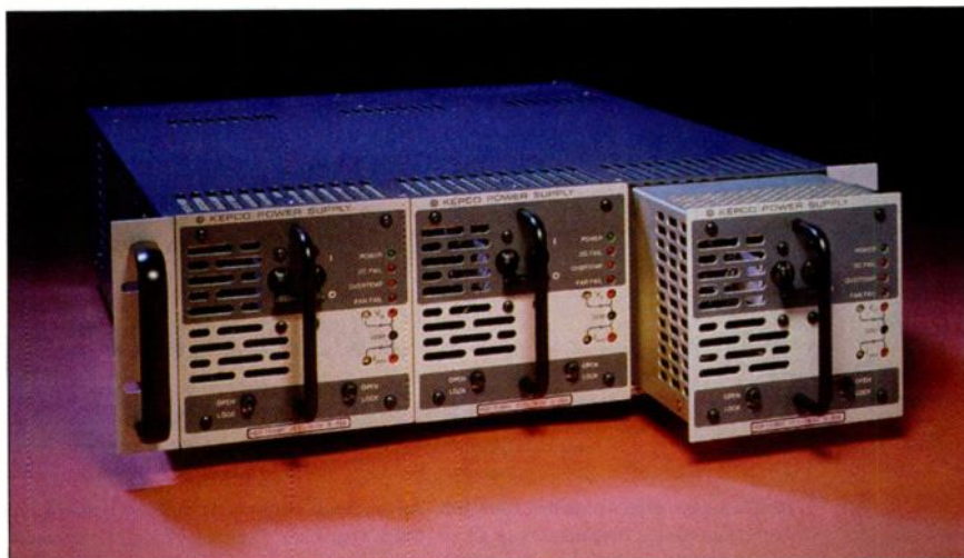
1. The HSP series of 1000-W power supplies comply with many requirements of the fault-tolerant systems now becoming pervasive in data-processing, telecom, financial, and transportation systems. These requirements include N+1 redundancy with current sharing, hot-swappability, and universal input-voltage ranges.
