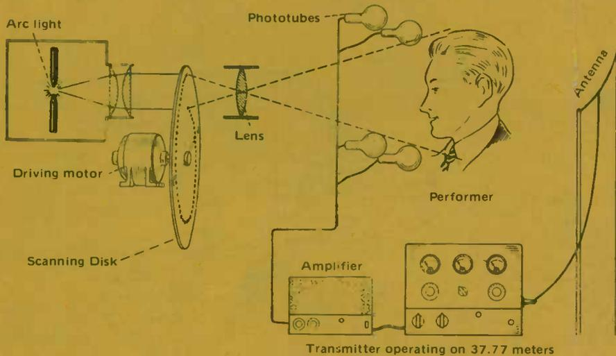
Fig. 6 Plan of a 1930 scanning-disk television transmitter.
