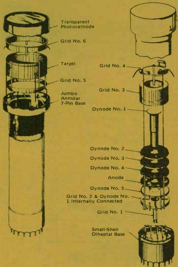
Fig. 18 Construction of an image orthicon tube.
