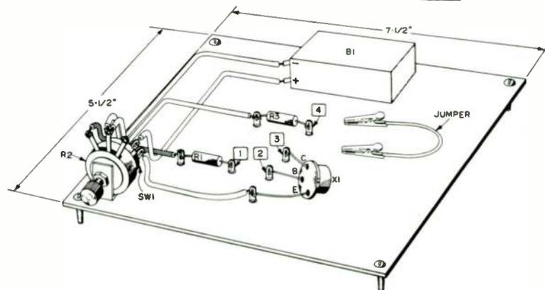
Fig. 2. Pictorial drawing of common-emitter amplifier.
