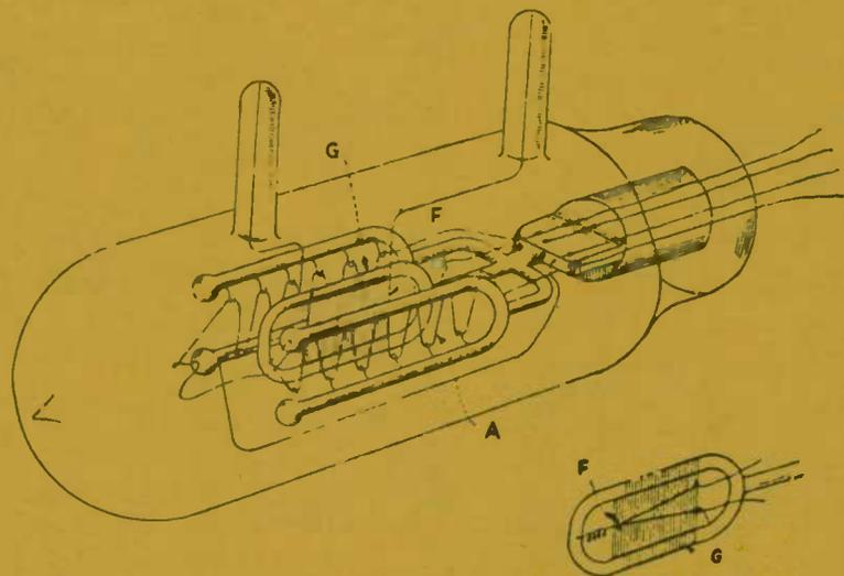
Fig. 3 A small sized Plotron for use as an oscillation detector. G is a tungsten grid; F, a tungsten filament and A, the anode of tungsten wire. Plan of the experimental detector tube.
