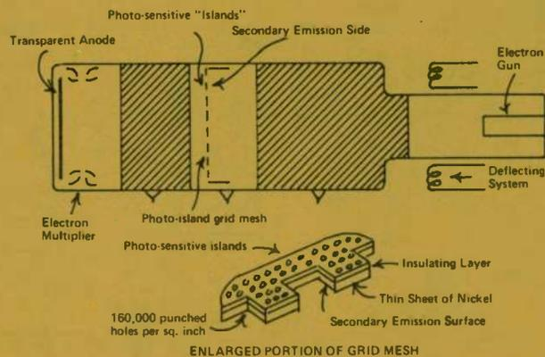
Fig. 15 A later version of the Farnsworth camera tube.
