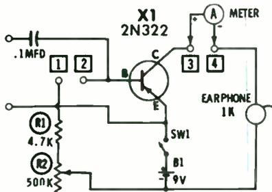
Fig. 6 - Practical AC amplifier circuit.
