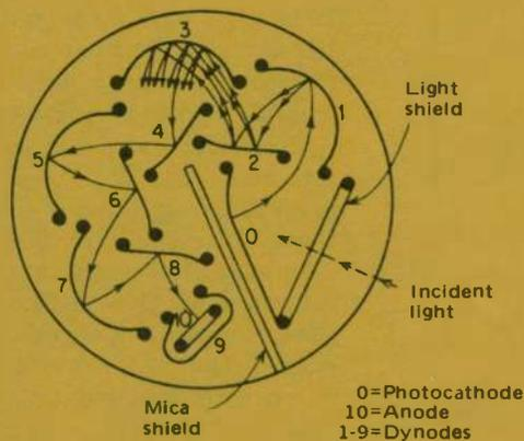
Fig. 23 Plan of a photomultiplier tube.
