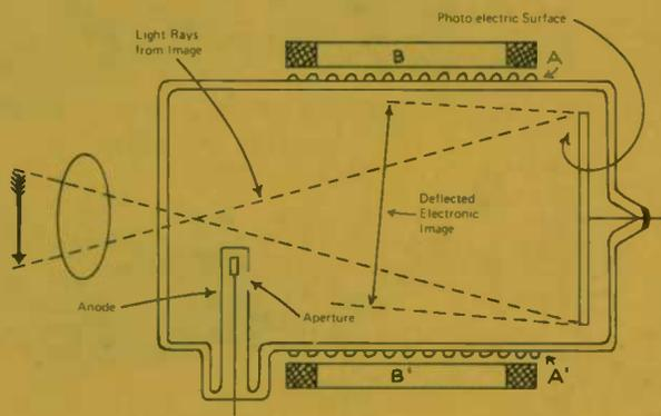
Fig. 12 Plan of the first Farnsworth image-dissector camera tube.
