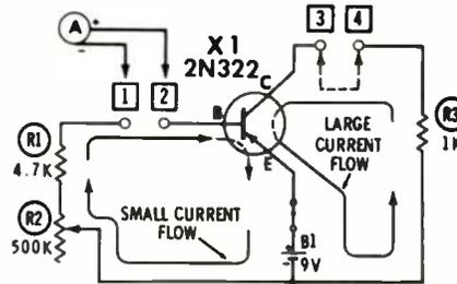
Fig. 1. Common-emitter amplifier circuit.
