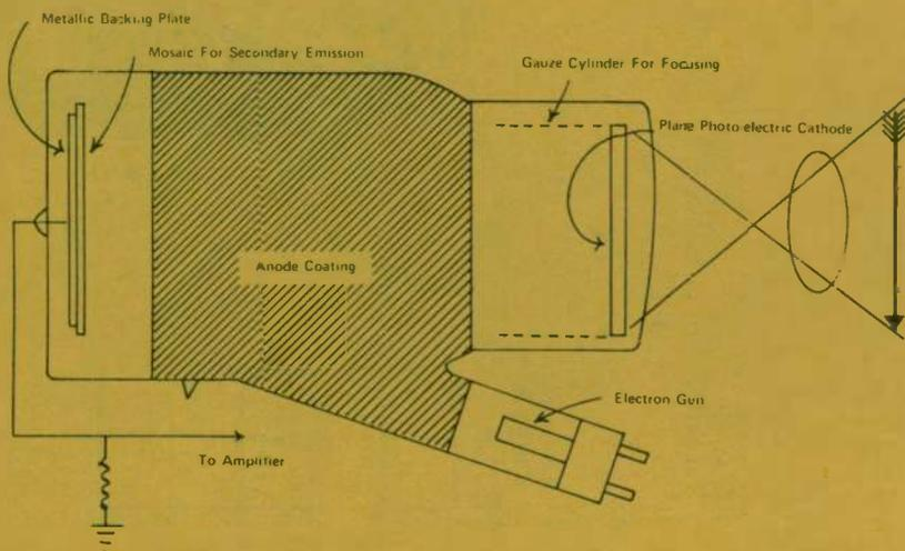
Fig. 16 Plan of the image iconoscope.
