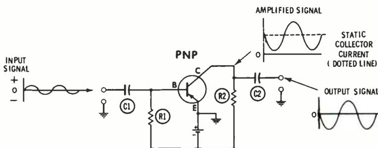
Fig. 5 — Basic AC amplifier circuit.
