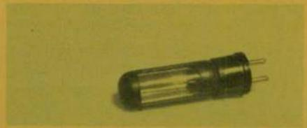
Fig. 10 A phototube with a "window" envelope.
