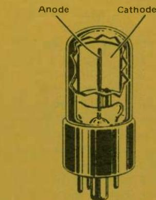
Fig. 8 Construction of a phototube.
