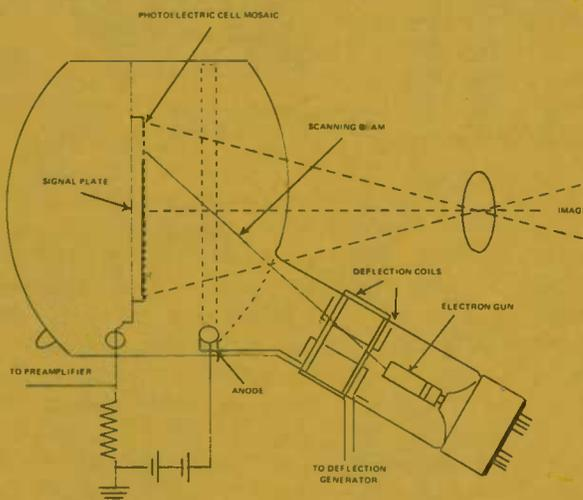
Fig. 14 Plan of an iconoscope.
