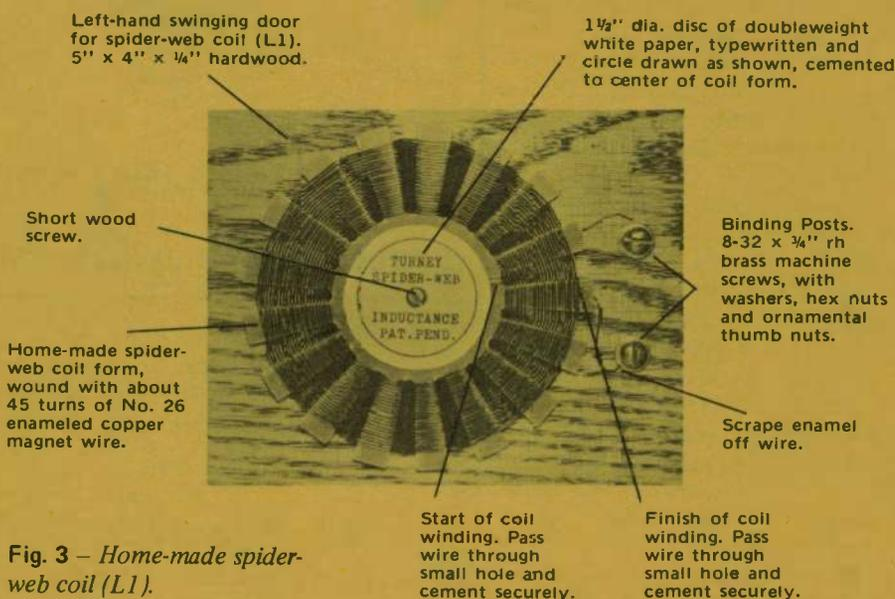
Fig. 3 - Home-made spider-web coil (L1).
