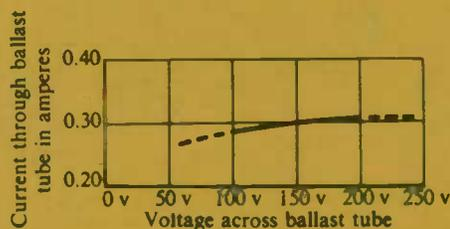
Fig. 27 Typical E-I characteristic for a barretter.
