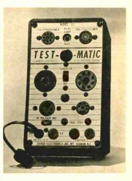
This new compact battery-operated tube tester is quite versatile. Only 3<sup>3</sup>/<sub>4</sub>" x 6", the unit will test most tube types and circuits for continuity. In addition it will check out high voltage circuits, fuses and pilot lamps. Priced at \$6.95 from Empire Merchandising Co., 170 Marbledale Road, Tuckahoe, New York. The tester is manufactured by Darod Electronics, Inc., Mt. Vernon, N. Y.
