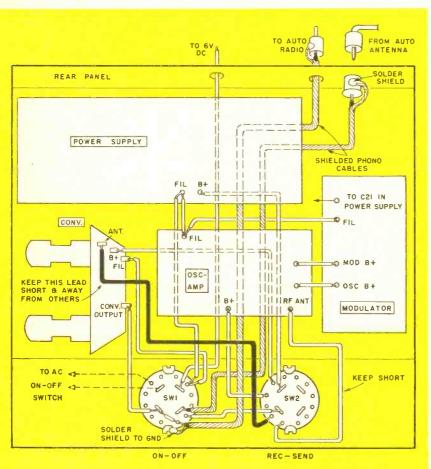
Wiring guide below shows all modules properly interconnected in chassis.
