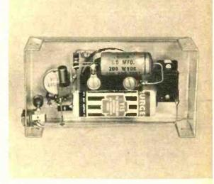
Neatness of wiring is evident from this view. Transistor socket is suspended by wiring.
