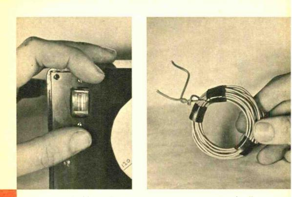
A miniature AM tuning meter provides accurate reading of wattage when properly calibrated. An inked-in scratch marks its "null" point. Simple coil serves as high-current, low-resistance input shunt resistor.
