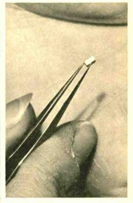
General Electric research scientists have successfully made tunnel diodes which work at frequencies above 4000 megacycles. Key to the improved performance is the use of gallium arsenide, a little known and rarely used semiconductor material, as the basic element in the device's construction. Frequencies well above 10,000 megacycles are possible with tunnel diodes made of gallium arsenide.
