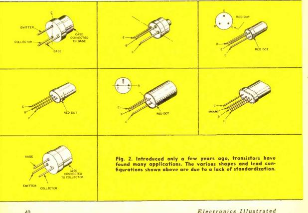
(rather than solid connectors) frequently has a yellow emitter, black base, and red collector wire. Sometimes the collector may have a red dot with the base and emitter positioned away from it.
