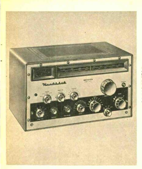
Primarily for General and Technician Class licensees, Heathkit "Seneca" transmitter tunes up on all the VHF ham frequencies, covering both six and two meter bands. It has built-in VFO, four crystal positions and delivers 120 watts input for phone work.
