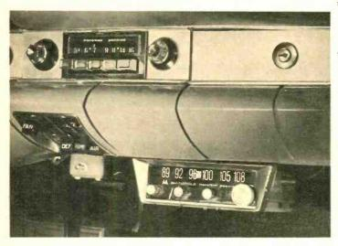
under-the-dash-installation unit can operate independently of the car's AM set. Three transistors power the hybrid circuit, which contains seven additional tubes. FM-900 shares the AM set's antenna and can be used with any 12-volt, negatively grounded ignition system. No need to sell the FM set when you sell vour car. It may be moved from auto to auto, or auto to boat. Other features are AGC, AFC and \$125 price.
