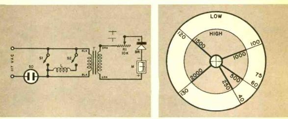
Rectification of voltage developed in the transformer secondary enables the potentiometer R1 to calibrate the meter according to the varying loads. Circular scale above is rough guide for use in the calibration procedure.
