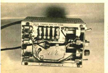
Underside view of chassis. Wires have been laced for permanence and neatness. Each circuit has an individual fuse held in its place by a clip-holder. Cutout for clock mechanism on chassis is seen in photo.
