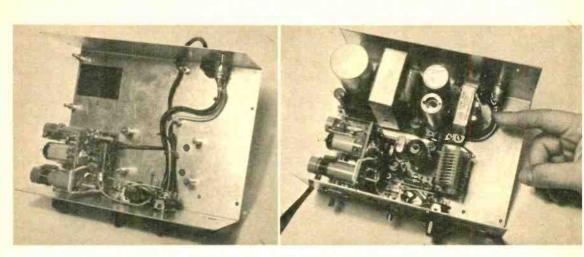
On upper left corner of chassis, strips of tape prevent vibrator socket from shorting to case.
