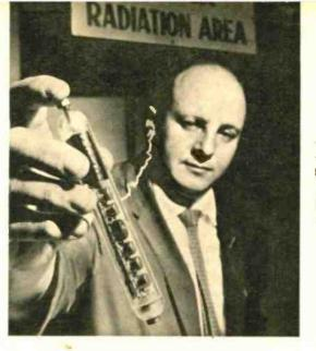
The radiation detector, battery and amplifier all are enclosed in this single small package that has been tabbed an "Alpha cigar" by Hughes.
