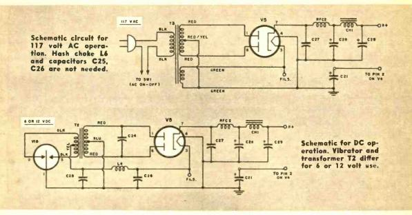
plies described here to minimize this but results are somewhat unpredictable. To reduce hash, keep the power lead (6 or 12 volts DC, as the case may be) as short as possible. A good ground is important, too. The best way to find a suitable grounding point is to connect a wire to the case of the rig and touch various metallic points under or near the dashboard. Find the one producing the quietest response in the speaker and connect the wire to it. More on installation later.
