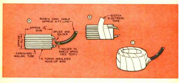
Figure 2. A step-by-step procedure for constructing the RF pick-up coil is shown in the drawing above. Black electrical tape holds wire to coil form.
