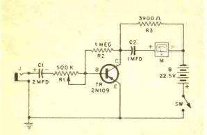
R3 provides the recommended source impedance for proper damping of the VU meter.
