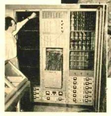
Above, census worker sits at console of FOSDIC III and examines 16-mm microfilmed copies of original census documents. At left is portion of the unit's electronic equipment. Central element is scanning system that reads any portion of film.
