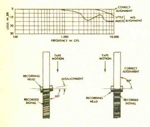
This sounds like a matter of azimuth adjustment. If the angle of the head (or heads) in each machine is not the same, high-frequency loss will be the result when tapes are swapped. I'd say your machine was alright in this respect since the pre-recorded tapes sound good. Play one of these on the other machine. If it sounds dull, the azimuth (head angle) must be adjusted on your neighbor's machine. Don't make this adjustment yourself; special equipment is needed.
