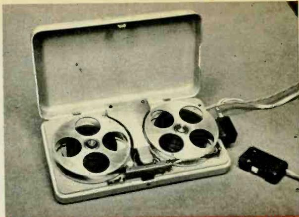
Fig. 1—Basic model of EDI recorder, now used for security work has sophisticated design, simple controls. Consumer models will be somewhat restyled, can be bought with cordless plug-in mike.
