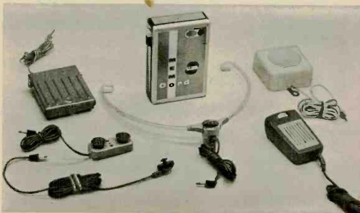
Fig. 4—Recorders for business use accept many accessories. Clockwise from Memocord recorder are extension speaker unit, conference microphone, stethoscope-type earphone, single earphone, telephone pickup, transcription pedal switch. Some recorders also have lapel mikes, carrying cases, holders for spare tape reels.
