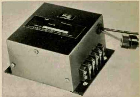
24 V and positive-ground systems to negative ground. A major use is expected to be found in adapting 12-V, negative-ground CB gear (and similar equipment) for use in foreign cars. Handles 30 watts. \$29.95. Pearce-Simpson, Inc., Box 800, Biscayne Annex, Miami, Fla. 33152.
