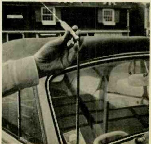
Adaptor antenna with loading coil simply clips to car's whip, feeds AM and CB through a splitter.
