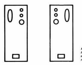
Finished enclosures should be located in the listening room such that tweeters are innermost.
