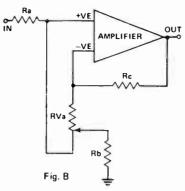
The output of the amplifier in this case is approximately the input signal times  $(10\ 000\ +\ 1000)/100\$ giving a gain of 20 dB. If the slider is at the other end of the potentiometer, (Fig. B), the signal appearing at the positive input, and thus also the negative input is about 0.1 (1000/ (10\ 000\ +\ 1000)) of the input. There will still be no current of the potentiometer and in RC, thus the output will be 0.1 of the input. That is, there will be a loss of 20 dB.
