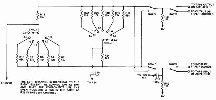
Fig. 2. Changes in the circuit for the left channel. The changes are only to simplify the PCB layout.
