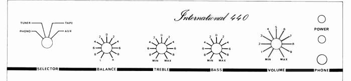
Fig. 7. Front panel artwork. Full size 335 x 83 mm.
