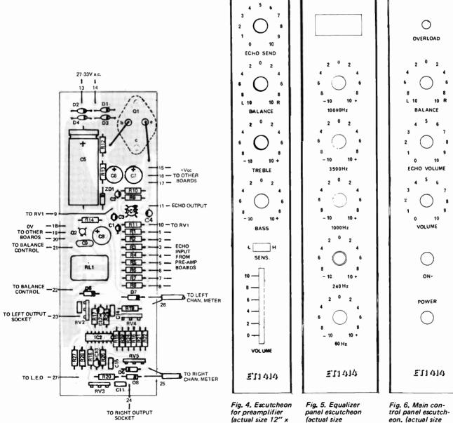
Fig. 3. Component overlay of power supply board.
