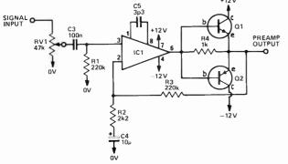
Fig. 3. The circuit of the preamplifier-buffer.
