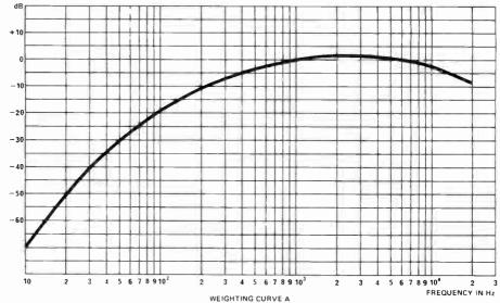
Fig. 4. Curve of 'A' weight response.
