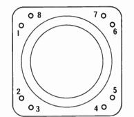
Fig. 5. The pin numbering sequence for T1.
