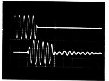
Fig.5 (a) Top trace – the input tone burst of five cycles. (original design). (b) Bottom trace – the response of a low-cost speaker at 1 kHz. Note the reduced amplitude of the first half cycle and that ringing has added another cycle at the end of the burst. The room reflection can be seen on the trace after the burst.
