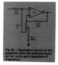
reduced, but a range of  $\pm 10$ dB is still available. With the wiper of the potentiometers set midway - Fig 2c, the gain will be unity regardless of frequency, due to the symmetry of the entire network.
