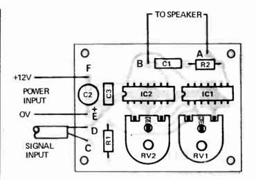
Fig. 3. Component overlay.
