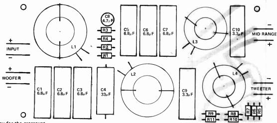
Fig. 4. Component overlay for the crossover.
