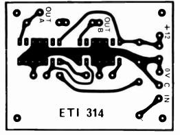
Fig. 2. Printed circuit board. Full size 50 x 65 mm.
