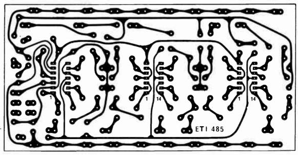
Fig. 2. Printed circuit layout. Full size 150 x 75 mm.
