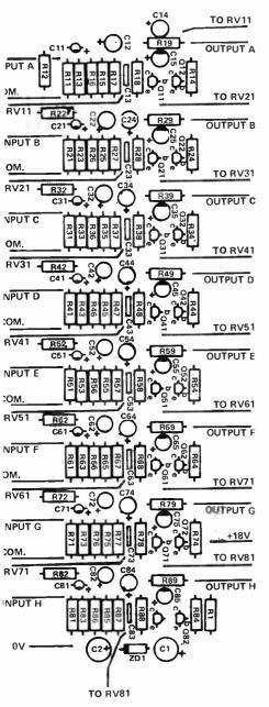
Fig.2. Component overlay for the preamplifier board.
