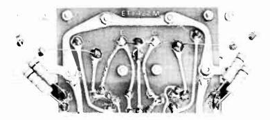
Rear view of the 100 W module showing the links and resistor which are external to the pc board.
