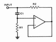
of the network. At either side of resonance the impedance will rise (with a slope dependant on the Q of the network which is 3) due to the uncancelled reactance. This will be inductive above resonance and capacitive below resonance. We can therefore represent the equalizer stage by the equivalent circuit below.
