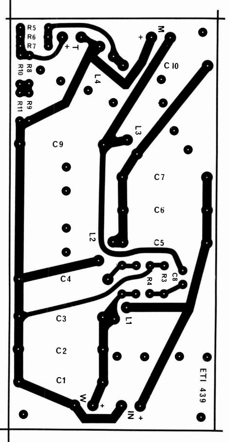
Fig. 8. Printed circuit layout for the crossover board. Full size 224 x 113 mm.
