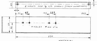
Fig. 10. Details of the heatsink bracket.
