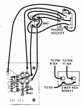
without upsetting the crossover point. Change over may be effected by using either a toggle switch or a push button. The tone-burst generator controls should be set for eight cycles on and off as this position will effectively remove any contact bounce.
