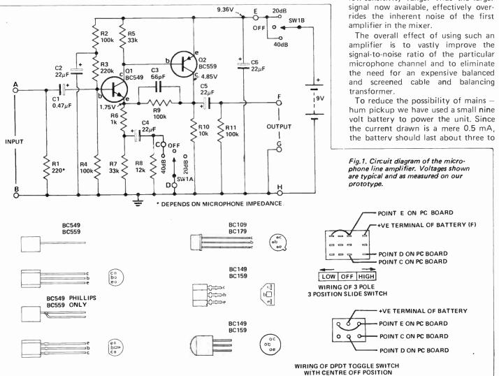
MODERN high quality microphones are low impedance units having a very low output voltage. To minimize noise, picked up on long leads, it is usually necessary to use special balanced and screened leads together with balancing transformers. An alternative approach is to use a low noise amplifier to boost the signal *before* passing it down the cable. The ETI 430 line amplifier, described here, is intended for this purpose.
