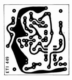
Fig. 4. Printed Circuit board layout. Full size 60 x 55 mm
