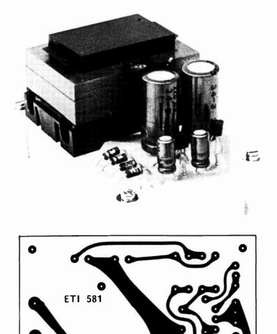
Fig. 1. Printed circuit layout. Full size 90 x 60 mm.
