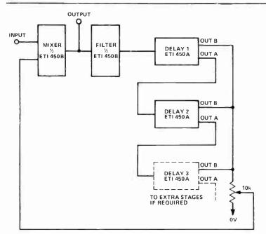
Fig. 8. The interconnection for reverberation.
