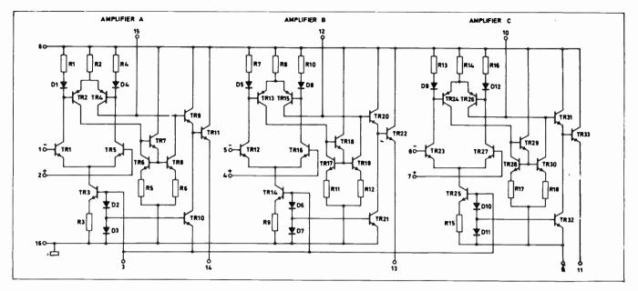
Fig. 1. Circuit diagram of the TCA220 triple-operational amplifier.
