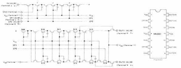
Fig. 2. The internal circuit of the MN3001 showing the first three and last four stages.
