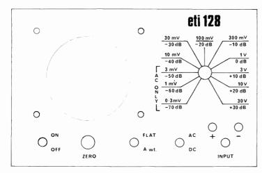
Fig. 6. Front panel artwork. Full size 189 x 121 mm.
