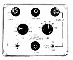
ACCURATE attenuators are required in a multitude of design, service, testing and measuring situations. These units are designed with varying degrees of accuracy and as many steps of attenuation as the designer feels necessary. They may be balanced or unbalanced and have whatever input and output impedances the designer requires.
