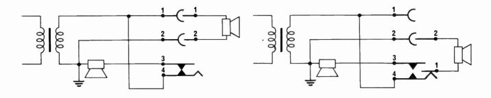
Fig.1a. Example of using the type 05 connector inserted in position A. Both speakers are operational.
