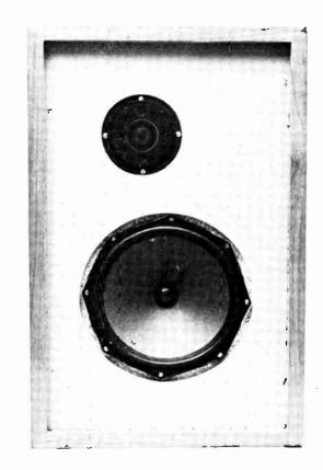
The completed speaker before front panel is painted or grille cloth fitted.
