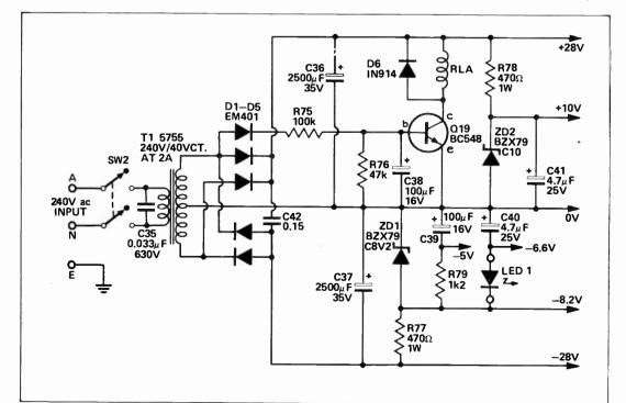
Fig. 2. Power supply for the 25 watt amplifier,
