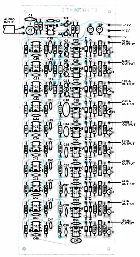
Fig. 5. The component overlay of the filter-rectifier board.
