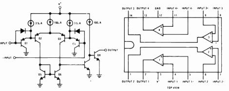
Fig.3. Internal circuitry and pin corrections of the LM339 IC.
