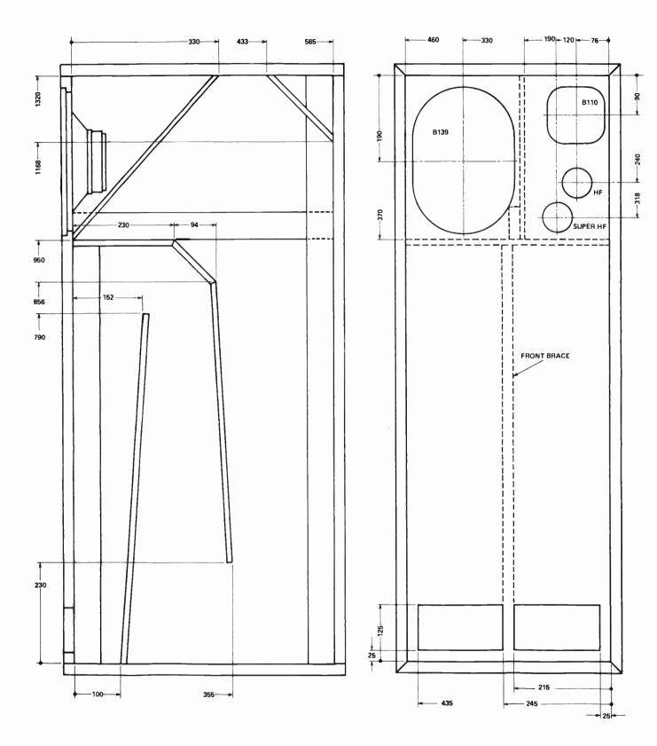
Study these drawings in conjunction with the one on the following page. Note that ideally the speakers should be built as a 'mirror-image' pair — that is, so that when placed in the listening room the tweeters should be innermost.
