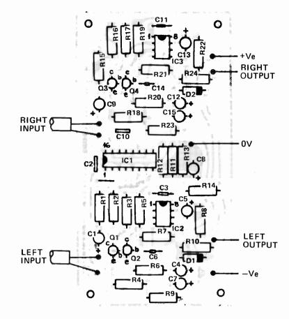
Fig. 2. Component overlay.
