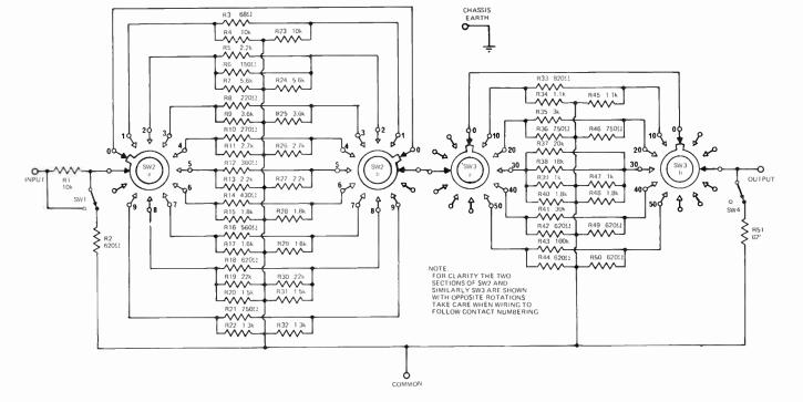
Fig. 1. Circuit diagram of the attenuator.
