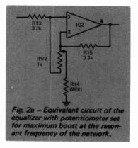
RV2. The voltage on pin 3 (IC2) is therefore equal to the output of the mixer since there is virtually no current through and no voltage drop across R13.
