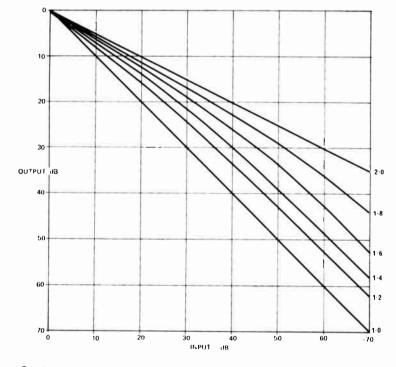
Graph showing relationship between input and output for the various compression ratios.
