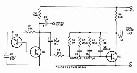
Fig. 1. Circuit diagram of the noise generator.
