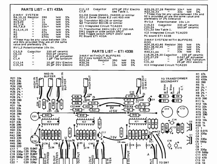
Fig.4. Component overlay for complete three-way system capacitance values are in microfarads except where otherwise noted.
