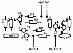
Component layout of printed circuit board version.
