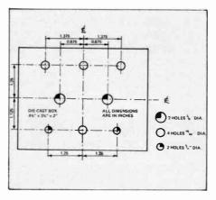
Fig. 2. Drilling details for the die cast box.
