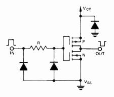
Fig. 6 Internal circuit diagram of one of the six inverter stages in the CMOS 4049 IC
