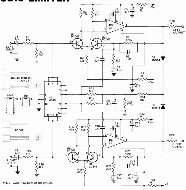
The circuit basically consists of a voltage-controlled attenuator followed by a low-noise amplifier with a gain of 46 dB. The output of this implifier is rectified to generate a dc voltage which is used to control the attenuator.
