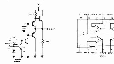
Fig.4. Internal circuitry and pin connections of the LM3900 IC.
