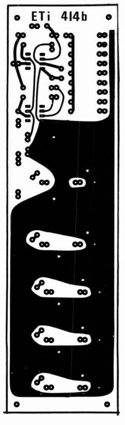
The main mixer and equalizer printed circuit board pattern - shown full size.
