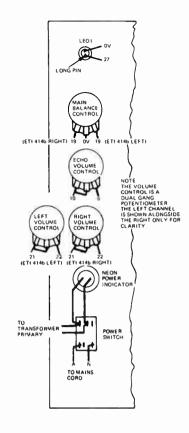
Fig. 7. Wiring to rear of main control panel.
