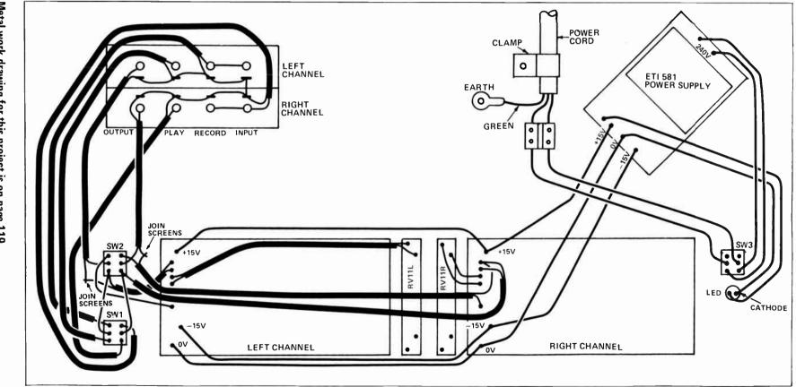
Fig. 6. Interconnection diagram for the unit.
