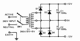
Fig. 2. The power supply circuit.
