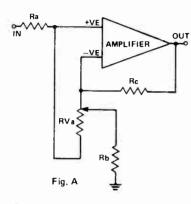
It must be emphasized that this equivalent circuit represents the condition with one tilter only, at its resonant frequency. Additionally letters have been used to designate resistors to avoid confusion with components in the actual
