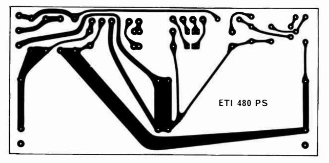
Fig. 7. Printed circuit layout of the power supply. Full size 160mm x 76mm.
