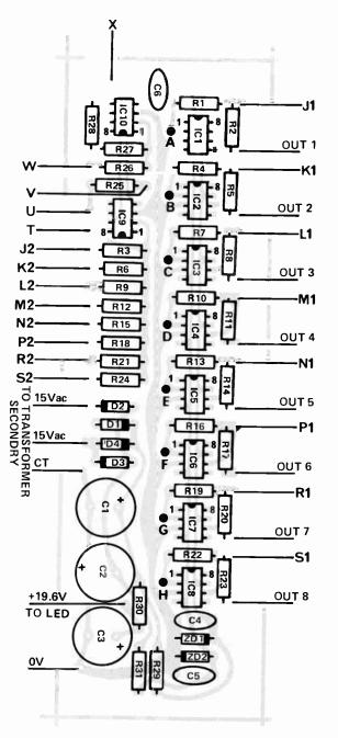
Note that pins 1 to 9 of the multi-cable socket will have 2 sets of leads, one set from the mixer outputs and one set from the VU meter selector switch.
