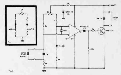
two diodes. The potentiometer provides a variable offset current giving a temperature offset range of about ± 5.5°C.
