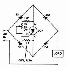
This circuit enables a single SCR to provide fullwave control of resistive loads.
