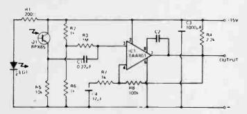
This circuit generates a fast rise time pulse each time the illumination of the BPX65 photo transistor by the LED is broken by a small object or rotating disc segment etc.
