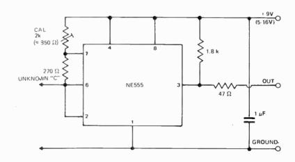
The prototype unit accurately measured a 50 000  $\mu$ F capacitor and a 2  $\mu$ F could still be measured
