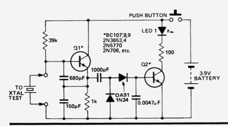
For checking fundamental HF crystals on a 'Go-No-Go' basis, the above circuit works quite well, An untuned Colpitts oscillator drives a voltage multiplier rectifier and a current amplifier. If the crystal oscillates, Q2 conducts and the LED lights. A3 or 6V, 40mA bulb could be substituted for the LED.
