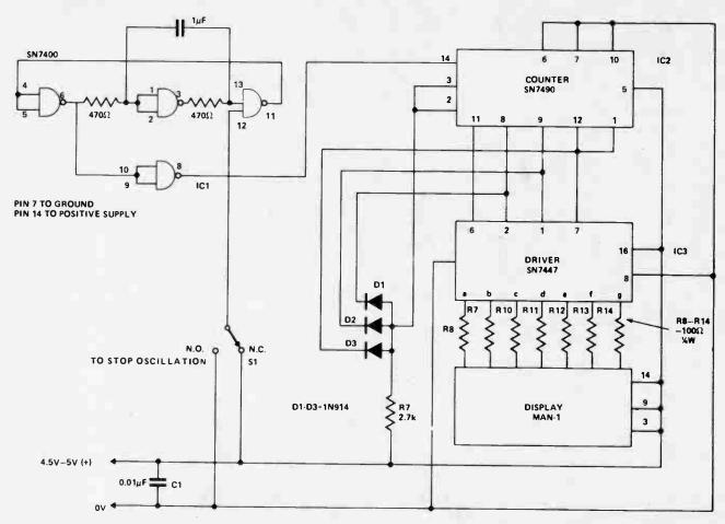
This device is based on a multivibrator (ICI) which has a frequency of about 1kHz. Oscillation continues as long as the input to pin 12 is high; as soon as the input is taken low or connected to earth it stops the cycle. This is used as
