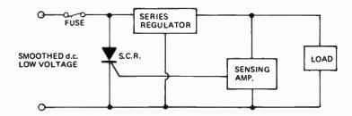
Conventional SCR crowbar power supply overvoltage protection circuits have some drawbacks.
