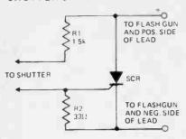
This three component device will keep sparks out of your camera shutter, when using a flash gun, by letting an SCR carry the firing current.
