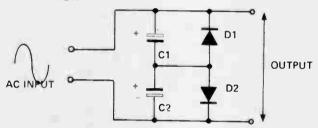
Quite often, especially when constructing operational amplifier circuits, capacitors of several  $\mu$ Farad values are required and they must be of the non polarised type (non elect-
