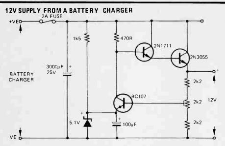
This 12V regulator unit was designed to enable bench testing of mobile equipment (radios, tapes, C-D units, etc.) using a battery charger, thus avoiding the expense of a complete bench supply and the inconvenience of a car battery.
