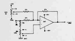
This circuit takes an input voltage x, and outputs a voltage y in accordance with the general linear equation y=mc+c. The offset is variable between +10V and -10V, by setting VR1; and gain m can be set anywhere between +1 and -1 (including zero) using VR2. There is no interaction between these two controls.
