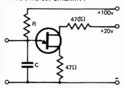
The linearity of a UJT relaxation oscillator may be improved by returning the 'timing' resistor R to a high voltage supply.
