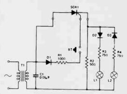
With a good SCR, lamp. L1 (6.3 volt 0.25A) will come on, and stay on, only whilst push button BT is depressed. If Lamp L1 comes on before the push button is pressed the thyristor defective — most probably due to an internal short.
