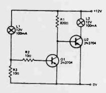
A signal lamp used to indicate failure of a vital piece of equipment is subject to failure itself.
