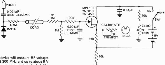
This device will measure RF voltages beyond 200 MHz and up to about 5 V with the components as indicated. The diode etc should be mounted in a remote probe, close to the probe tip. Sensitivity is excellent and voltages less than 1 V peak can be easily measured. The unit can be calibrated by connecting input to a known level
