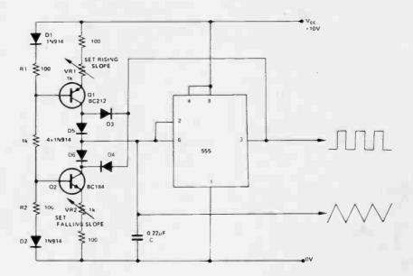
capacitor, and Q1 is allowd to linearly charge it up; when the capacitor voltage reaches  $2/3V_{CC}$  the 555 output goes low again, and the cycle
