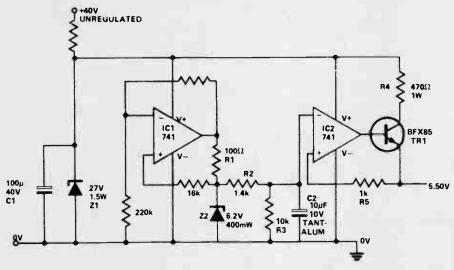
This circuit was evolved to provide a highly stable and ripple-free voltage to act as the reference for the stabilised power-supplies of an electronic music synthesiser; the stability of its voltage-controlled oscillators depended directly on the constancy of supplyrail voltages.
