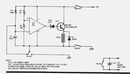
At the instant the door switch is operated the +Ve 741 input is at 2/3 the rail voltage. The -Ve 741 input is fully negative. The -Ve input is thus -Ve with respect to the positive input and an output near the rail voltage results turning on VT1 and operating RLA.
