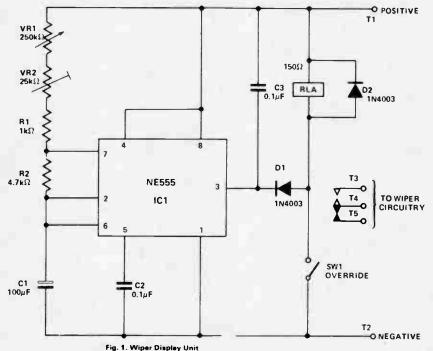
Having recently experienced some difficulty in trying to fit a thyristor type wiper delay unit to the car, the trouble was eventually found to be a result of the design of the car's wiper circuit and also by noise spikes which spuriously trigger the thyristor. The following circuit should overcome these problems in both negative and positive earth vehicles.
