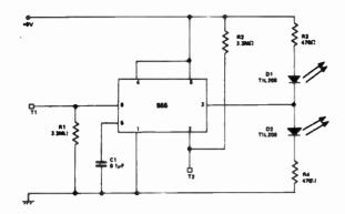
This circuit was devised as part of a touch controlled lighting system. It uses a 555 timer operated in the bistable mode.
