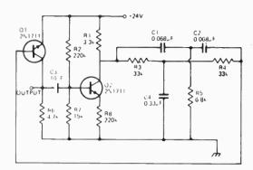
The frequency of oscillation of this circuit is determined by a twin T network and is stable to within 0.05% for  $\pm$  10% supply variation.
