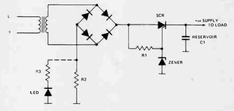
charge via the load, whatever power is being supplied, until the gate is once more positive, when the SCR will fire again. One or more half cycles are sufficient to raise the reservoir voltage sufficiently to prevent further firing.
