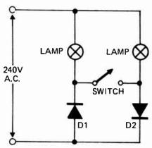
When setting up photographic floodlamps it is sometimes desirable to operate the lamps at lower power levels until actually ready to take the photograph. The circuit shown allows the lamps to operate on half cycle power when the switch is open, and full power, when the switch is closed. The diodes D1 and D2 should have a 400 volt PIV rating at 5 amps.
