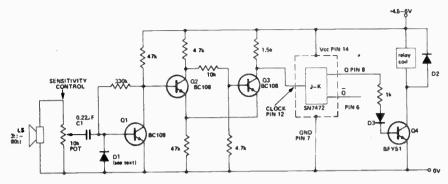
Schmitt trigger's output which is fed to the clock of the JK flip-flop causing it's output to change state. This is used to turn a relay on and off. Because the circuit is only sensitive to sharp noises it is generally unaffected by talking or sounds caused by movement. (The sensitivity control can be adjusted to prevent such noises triggering the circuit if this does arise). A moving coil loudspeaker is used as a microphone as it can respond to sounds from any direction. It was
