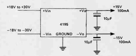
erature of the chip exceeds +175°C, so there is no danger of thermal damage. The short circuit is typically 220mA.
