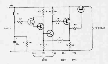
causing a sharp regenerative switching action to take place. TR5 is driven from TR4 collector and handles the supply current to the circuit being switched. R1 ensures C1 fully discharges since as long as any charge remains TR1 and TR2 continue to pass a small current (1mA).
