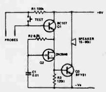
Almost any NPN silicon transistors can be used for Q1 and Q3 and almost any unijunction for Q2.
