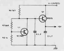
When it is necessary to power a few TTL packages, a simple zener diode—emitter follower stabliser is often used. If a zener of the appropriate value is not available, then the circuit shown may be used instead. Q1 is a standard VBE-multiplier; the current through Q1 increases until its VBE-drop is established across R3. Hence about 8 times VBE is established across Q1, and this voltage is used as a reference for emitter follower Q2.
