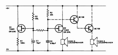
The circuit consists of two unijunction relaxation oscillators. Q1 for low
