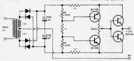
A variable power supply using complementary output transistors is capable of swinging the voltage at the output from +12 V through zero to -12 V.
