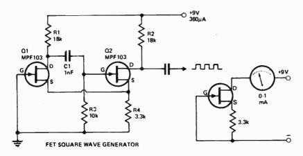
Field effect transistors lend themselves readily for use in astable multivibrator circuits.
