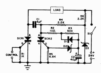
Originally developed by the Unitrode Corporation, this circuit will supply up to four Amps for a period of one second when triggered by an external positive going pulse.
