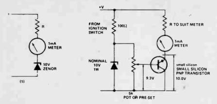
To make a meter cover the range 10 to 15V or 10 to 20V over its whole scale, then circuit (1) is often used. The zener must be exactly 10.0V and may not be available. In this case use the arrangement shown in (2).
