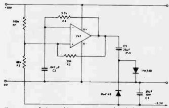
the operating range of the oscillator is pulled down until it is outside the operational range of the 741, and the charging ceases. This provides a form of switching regulation of the output voltage, roughly halving the output impedance. The output voltage can be
