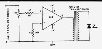
As the current drain for the whole circuit is small it can be supplied either from the main dual-voltage supply lines of the existing equipment or alternatively two PP3s. (Should last for several months).
