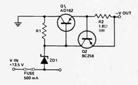
These short-circuit protected stabilisers give 6, 7.5 and 9 V from an automobile battery supply of 13.5 V nominal, however, they will function just as well if connected to a smoothed dc output from a transformer/rectifier circuit.
