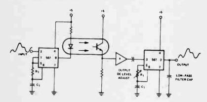
SOMETIMES it is necessary to transfer an analogue signal from one system to another without making any electrical connections.
