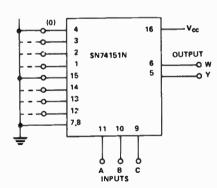
example implement a function to produce an output only if the binary number ABCD is exactly divisible by three.) If it is preferred, each input may be tied to a high level via its own resistor which may then be left in circuit even if required to short the input down to earth.
