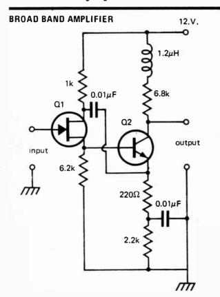
This circuit has a typical gain of 10dB and bandwidth of 90 MHz.
