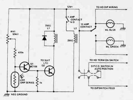
headlamp wire is removed from the headlamp switch and taken to the unit and another is run back to the vacated terminal. The LDR should be mounted in a bicycle rear light housing (torpedo shape) and mounted at bumper height on the offside of the
