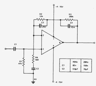
magnetic cartridge may be only about 5mV 'normally a musical peak may well force the cartridge output to 100mV. Clearly unless a large signal swing is possible the sound emmanating from the speaker is not going to be Hi-Fi.
