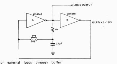
TWO CONTROL SIGNALS DOWN ONE WIRE
