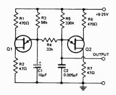
This circuit will produce a continuous sequence of increasing frequencies (in steps) until the highest is reached. The system then resets itself and starts again.
