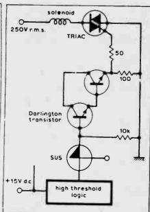
High-threshold logic, operating from a 15-V supply, produces a logic '0' output of 0 to 1.5 V and logic '1' output of 12.5 to 15 V. Noise amplitudes which increase the '0' level to 6.5 V and reduce the '1' level to 8.5 V can be tolerated.
