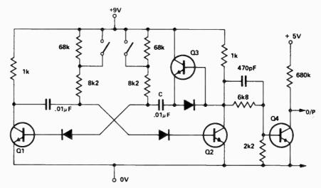
output is used for driving TTL the collector load must be returned to a voltage no greater than +5V.
