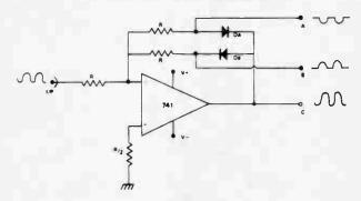
This circuit separates the positive and negative halves of an input waveform, and presents them (both phase-inverted) at separate output terminals. When the input swings positive, terminal A swings negative by an equal amount, terminal B remaining at zero voltage due to the reverse-blasing of DB and the virtual-earth action of the op-amp. For negative inputs, terminal B swings positive by an equal amount, terminal A remaining at zero due to the reverse-biasing of DA.
