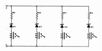
This circuit provides sequential closing of a relay series by appropriately increasing an applied voltage.
