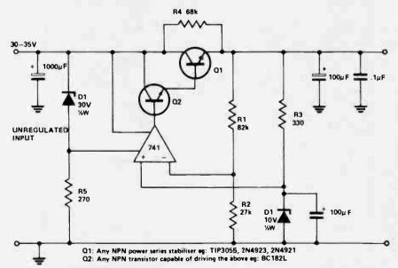
by replacing R1-R2 with a potentiometer, but in its present form, the circuit cannot be made to regulate below the zener voltage of D2. If continuous variation is required, the reference source R3-D2 must be supplied from the unregulated input, with consequent slight loss of stability,
