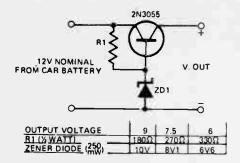
Many transistorised items such as radio, cassettes and other electrical items operate on batteries. Usually these are in the 6–12V range and sockets are provided for external power supply.
