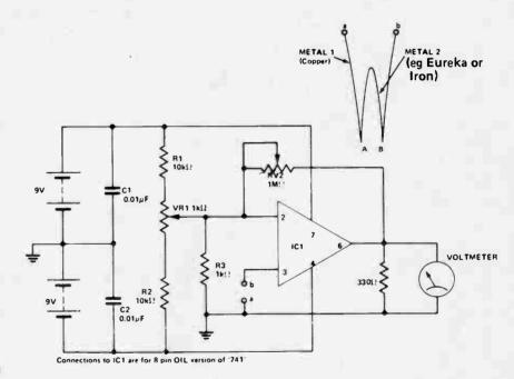
gain of the circuit is set high (at 1,000), electrical noise pick-up and drift become serious problems and it is advisable to assemble the circuit in a metal, earthed box and to ensure the unit is kept at constant temperature.
