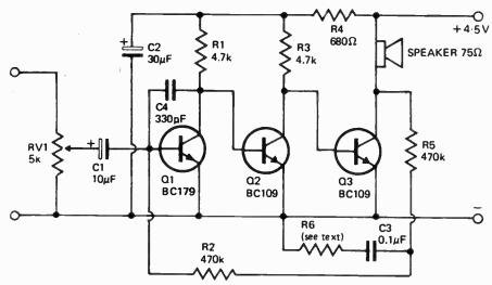
When power output, harmonic distortion, frequency response are not the absolute parameters for an
