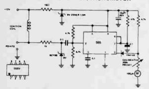
The Signetics NE555V Timer/Monostable Multivibrator is probably the most important standard IC to appear since the 741 op amp. Its versatility is obvious, but it can also perform a variety of tasks, with a 4½ to 18V supply and its ability to sink 200mA.
