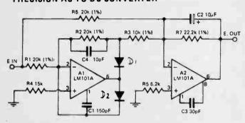
The circuit shown provides better than 1% conversion accuracy of ac signals up to 100 kHz. The output is calibrated to read the rms value of the sine-wave input with less than 1% ripple at 20 Hz.
