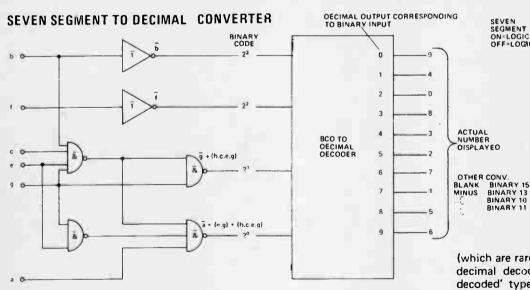
Note that the output from the gates is not straight' BCD so the outputs from the BCD to decimal decoder are
