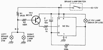
NOTE: The circuit needs only 3 connections A, B and C to existing wiring.
