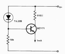
This current source is very temperature-stable; the output current varies by less then 1% over the temperature range -55°C to +100°C. This is possible because the transistor is biased by an LED, whose forward voltage drop has a temperature coefficient of -2mV/°C, the same as the base-emitter voltage of a silicon transistor. Hence near-perfect temperature compensation is possible, a great improvement over conventional methods of biasing with zener diodes.
