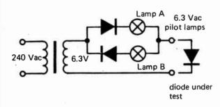
If lamp A or lamp B is illuminated the diode is serviceable. If both light the diode is short circuit. If neither light, diode is open circuit.
