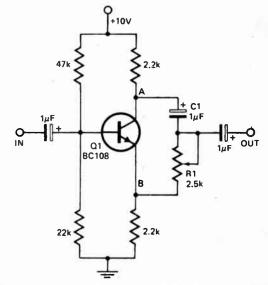
The circuit shown provides a simple means of obtaining phase shifts between zero and 170°. The transistor operates merely as a phase splitter, the output at point A being 180° out of phase with the input. Point B is in phase with the input phase. Adjusting R1 provides the sum of various proportions of these and hence a continuously variable phase shift is provided.
