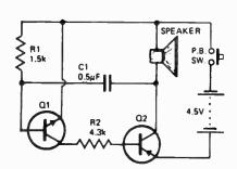
This circuit consists of an assymetric multivibrator activated by a pushbutton. The loudspeaker is a transistor radio type with a voice coil impedance of about 25 to 40 ohms. Earpieces up to 500 ohms can be used for lower power output. R1 varies frequency over the audio range.
