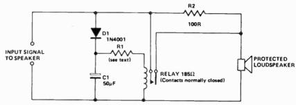
R1 is adjusted to give adequate protection at whatever power is being used. Resistor R1 value should be selected according to the power at which the speaker will need to be
