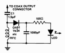
An RF output indicator using a LED is very useful for monitoring the output of a transmitter. This circuit will give indication from a 5 W transmitter. The capacitor C1 and the RFC are chosen for the appropriate frequency. The RFC could be replaced by a resistor for wideband use. The sensitivity depends on the value of C1 and the resistor used if the RFC is replaced. For high power transmitters, C1 could be a small 'gimmick' capacitor.
