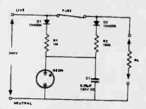
up to the striking voltage of the neon, diode D2 must have a PIV rating greater than peak mains plus this voltage. D1 can be rated at peak mains or greater. The types specified are suitable easily-obtained devices. Also, built-in resistors in certain types of neon indicator supplied for use at common supply voltages must either be removed or 'shorted'. The resistors should be ½W.
