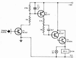
In the circuit shown, hum is induced into the touch plate when touched with a finger. This hum signal is rectified in envelope detector/amplifier T1 and the resultant dc current amplified by T2, T3 and T4.
