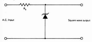
A zener diode clips one half-cycle of the input sine-wave in this simple square-wave generator. The zener voltage must be a small fraction of the input voltage for acceptable results.
