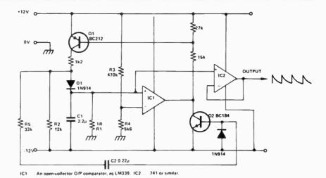
seconds by the positive feedback loop through R5, C2 and Q2, to ensure C1 charges fully. After this time C2 is also fully charged, and Q2 turns off, turning off Q1, and allowing the slow discharge of C1 to begin again.
