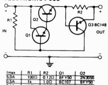
Here is a circuit for protecting modern transistorised gear which requires a faster action than can be provided by an orthodox fuse.
