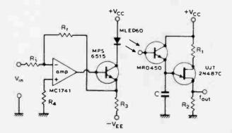
The output takes the form of a signal, the frequency of which is proportional to the applied voltage.
