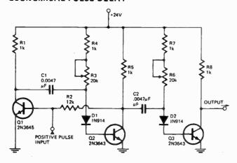
The circuit shown is of an economical pulse delay which utilizes only three transistors instead of the four normally required for a pair of one shots.
