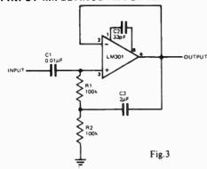
The LM301 may also be used to construct a simple high input-impedance ac amplifier as shown in Fig. 3. In this circuit even though the bias resistor is only 200 k, as required for good dc stability, the bootstrapping by C3 provides an input impedance of 12 M at 100 Hz increasing to 100 megohm at 1 kHz.
