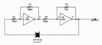
at fundamental frequency, whereas many crystals (particularly higher frequency ones) are stamped with the overtone frequencies. These will operate at the fundamental and not the marked value.
