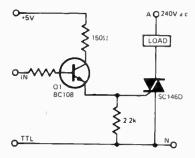
Here is a useful circuit for driven mains operated devices direct from TTL logic circuits. Although it works well, it has the inconvenience that the neutral line is connected to circuit ground.
