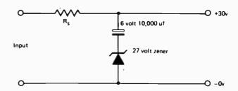
Electrolytics combining large capacity and high working voltage are bulky, expensive, and frequently difficult to obtain.
