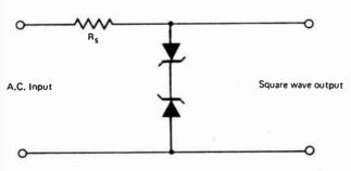
If a larger output is required, opposed zener diodes may be used to clip both halves of the input sine-wave.
