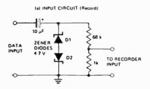
The two circuits shown allow digital data to be recorded and replayed on an ordinary domestic recorder.
