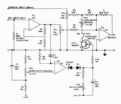
This is an autofade circuit for use in discotheques and the like. This autofade unit has advantages over VCG ICs which introduce distortion and noise (the 741s may be substituted by low noise op-amps) by using a FET to switch the signal gain characteristic. The principle may be easily adapted into existing mixers.
