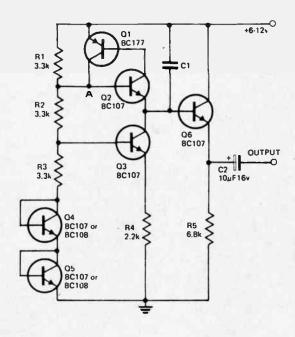
In this circuit two transistors Q1 and Q2 are connected so that they operate as a unijunction transistor.
