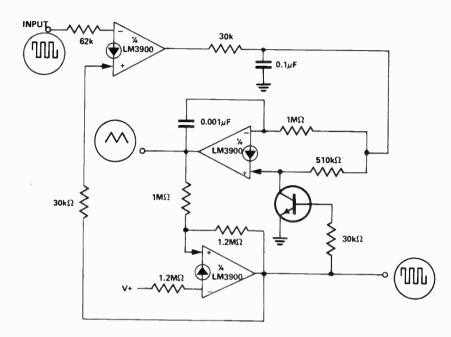
Integrated circuits which have been specially designed as complete phase locked loops are available, but many of them tend to be rather expensive devices. The circuit shows how the economical LM3900N integrated circuit can be used to build a phase locked loop which has a centre frequency of about 3kHz.
