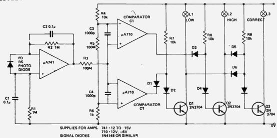
When conducting optical experiments, or calibrating photocells, it may be necessary to set a known light level each time before the experiment is performed. The circuit provides a simple means of setting a light level to a particular value.
