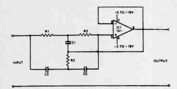
This narrowband filter using the 741 operational amplifier can provide up to 60 dB of rejection. Setting resistors equal to 100 k and capacitors equal to 320 pF the circuit will reject 50Hz.
