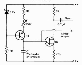
This circuit provides a linear time-base with a sweep time adjustable from a few milliseconds to over one minute.
