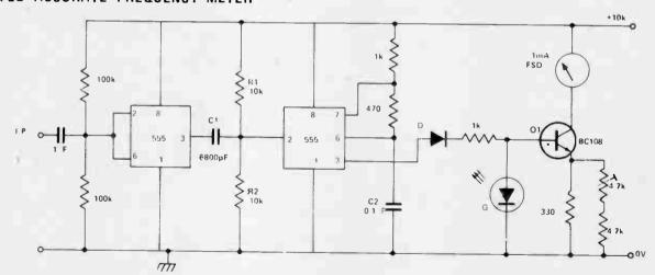
This circuit provides a meter deflection that is strictly proportional to the frequency of the input signal over the range 10Hz-300Hz. The first 555 timer IC is used as a Schmitt trigger, to convert the I/P signal to a fast-edge square wave. This is differentiated by the network C1, R1 and R2, and the resulting spikes used to trigger the
