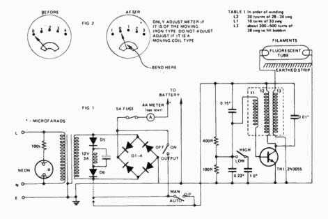
voltage divider for the biasing of C2, 3. With C3 in circuit the inverter in fact becomes more efficient, but has a lower output. Using a 2N3055 enables the inverter to be modified to give higher output and also guards against thermal runaway when used for long periods. A heatsink is advisable.
