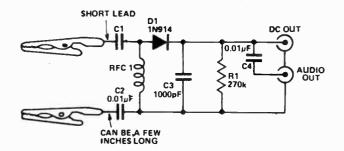
choke down to 470  $\mu$ H (i.e. Aegis C13, UPC560 or VPC470). In the VHF range C1 can be a 2 to 10 pF capacitor or 0.8 to 7 pF trimmer. RFC1 can be between 47  $\mu$ H and 150  $\mu$ H (i.e. Aegis VPC 150, UPC120, VPC100, VPC82, VPC68, VPC56 or VPC47).
