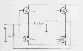
The value of capacitance existing between points 1 and 2 may be varied over a 1000 to 1 range by RV1.
