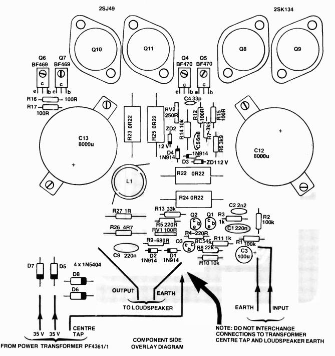
removed and remounted, possibly with a new insulating washer. Finally, solder the leads to the transistors.
