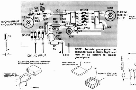
former. Overall gain is around 12 dB and the noise figure is around 6-7 dB. This sort of performance is more than adequate for normal service reception of UHF transmissions.
