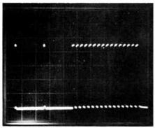
Figure 1. Transmitter waveform, monitored across R7 on pc board ETI-599a. Vertical scale 100 mV/ div.; timebase 5 ms/div. for first four divisions, showing 25 kHz burst repetition, then 100  $\mu$ s/div. for rest of sweep showing 25 kHz pulses.
