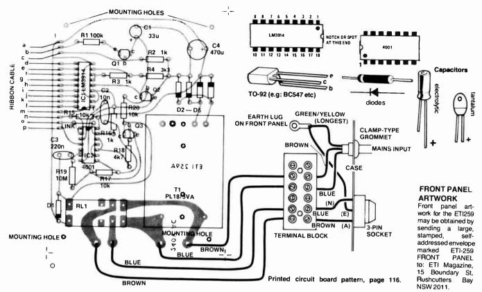
point. Now mount the piezoelectric buzzer and solder its leads in place, as shown on the overlay. Attach knobs to the shafts of SW2 and RV1 last of all.
