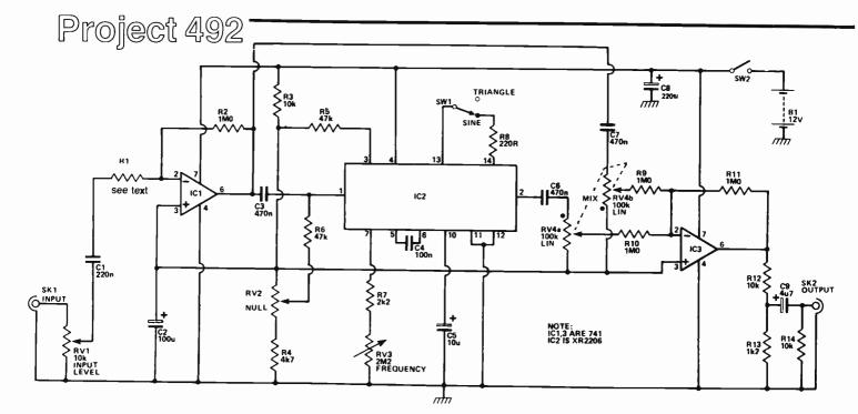
By mixing or 'multiplying' an audio signal with an oscillator or 'carrier' signal that may be varied from the sub-audible to the mid-range of the audio spectrum, the original signal may be altered in a variety of ways. Mixing an audio signal with a sub-audible carrier produces a tremolo effect — a form of amplitude modulation; mixing speech with a carrier around 1 kHz to 2 kHz produces 'robot' voices. That's just to name a few of the more familiar effects possible.
