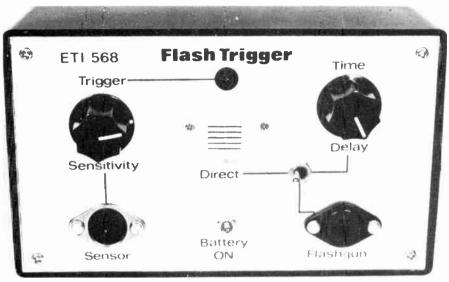
The prototype was housed in a 'jiffy' box measuring 160 mm long by 95 mm wide by 50 mm deep. The front panel was dressed up with a Scotchcal transfer. These should be available through suppliers — see Shoparound on page 128.
