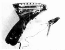
Modified hand controller with connection to both ends of resistance wire.
