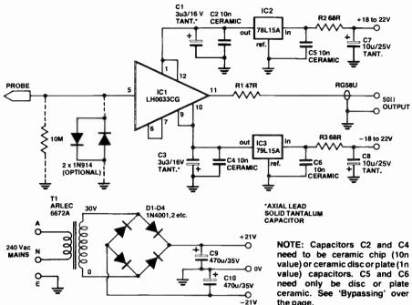
used to keep the unit compact. An external unregulated supply of between 18 and 22 volts at around 50 mA is required to power the probe.
