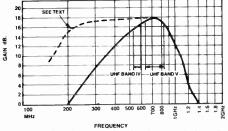
Measured bandpass and gain characteristics of the amplifier. You can alter the response to that shown by the dotted line by adding one turn to L1 and L2.
