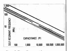
Figure 5. The self-resonant frequency versus capacitance of a typical 5 mm disc or plate ceramic capacitor with differing lead lengths (from lower curve, up - 25 mm lead length, 22 mm, 13 mm, 6 mm and none).
