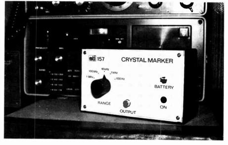
used to calibrate the timebase oscillators of frequency counters and period timers simply by plugging the marker output into the counter's input and setting the timebase frequency to obtain the correct display!
