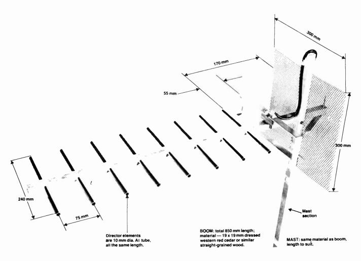
General construction. Note that a metal mast may be used instead of the wooden one.
