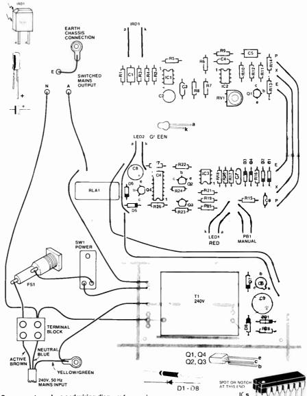
Component overlays and wiring diagram for receiver.
