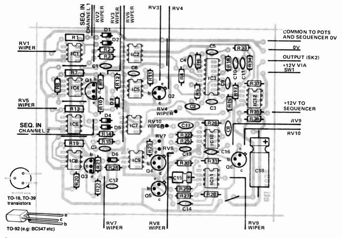
Component overlay. Note that the board has been laid out for the Q1 and Q3 transistors with an e-c-b pinout. Watch the pinout of the transistors you use; you may have to cross the base and collector leads.
