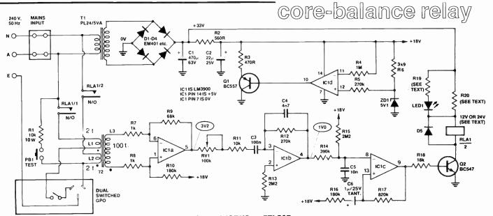
The circuit can be divided into three parts: the unbalance current sensor (T2), the trip circuit, and the power supply. We'll examine each in turn.
