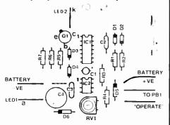
Component overlay for transmitter.
