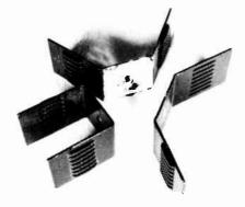
The heatsink we used for Q2 was made up from two 'flatpack' heatsinks, Dick Smith No. H3402, bent as illustrated and mounted back-to-back on the transistor. This ensures they fit in the case. Use plenty of silicone heatsink compound to get good thermal conduction. The unmodified heatsink is shown at lower left.
