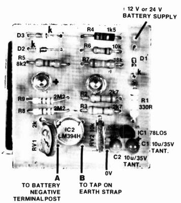
Component overlay for the pc board (pc board pattern is on page 32). Trimpot RV1 is for BALANCE while RV2 is for ZERO SET. The latter, along with R7, is left out if you use a centre-zero meter.
