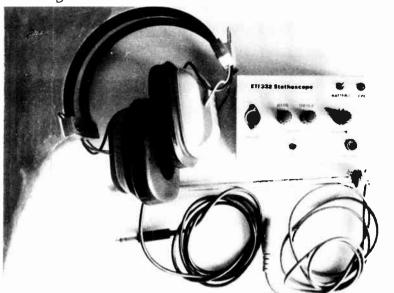
Completed stethoscope, ready for action! The probe here was made from a crystal earpiece, a length of 10 mm tubing being pushed over the ear plug.
