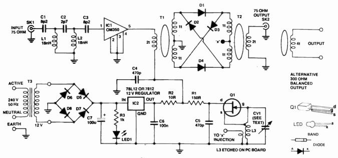
The converter's format is quite conventional — an RF amplifier drives a mixer, local oscillator injection being provided by a variable frequency oscillator, the frequency of which is set by a small variable capacitor. A full-wave bridge rectifier followed by a threeterminal regulator provides regulated 12 Vdc to power the circuitry.
