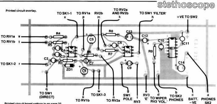
Printed circuit board pattern is on page 32. technique. The buffer electronics is protected by encapsulating it in quicksetting epoxy. The mechanical coupling arrangement will depend very much on the particular mic insert employed and the application you have in mind. We made up several probes to suit different applications. If the mic has a metal case connect it to the probe cable's shield.
