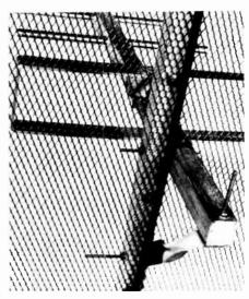
Rear view showing support strap for the rear of the boom. The picture was taken when the reflector mesh was only thumb-tacked to the mast. It has since been more securely fixed with screws. Project 156
