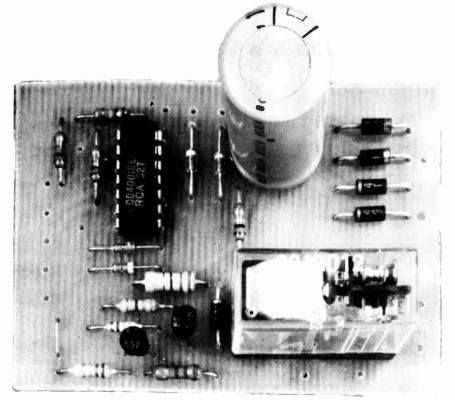
The relay driver board is simple, yet versatile. The external input/output pins are located around the edges of the board.
