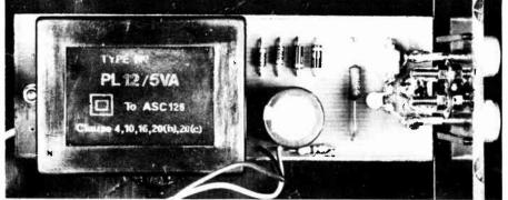
Internal view of the power supply. Note the pc board is double-sided.
