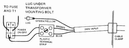
Mains wiring diagram
