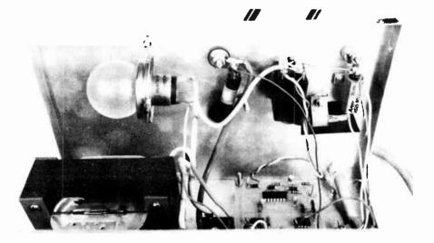
View of the rear panel showing how we mounted the various major components. Note the 45 W lamp 'ballast'. The relay was glued in place between the two output terminals. The Arcoi metal-clad resistor is mounted as close as possible to the positive output terminal.
