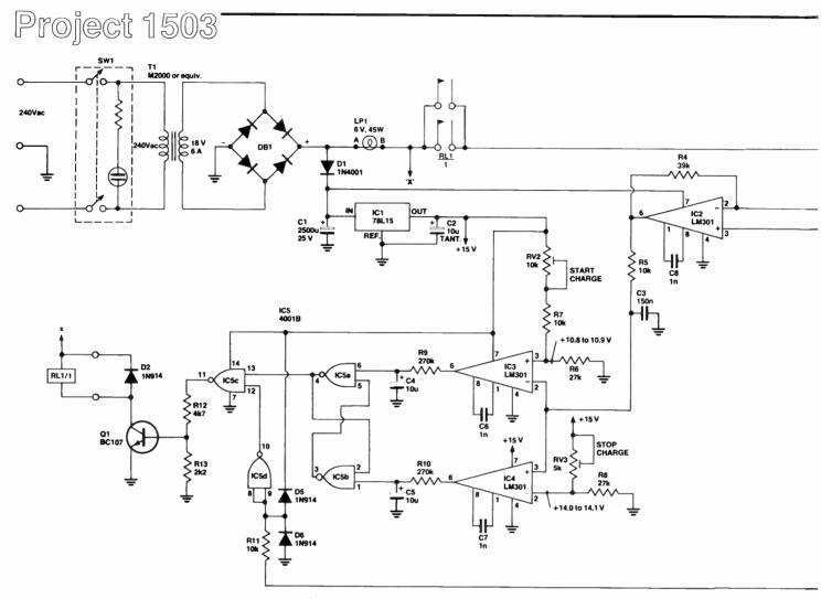
The overall function of the device is as follows: when the open-circuit potential of the battery fails to below about 10.8 volts the charger turns on, charging the battery until the potential rises to about 14 volts, whereupon it turns off the charging current and waits dormant until the cycle repeats.
