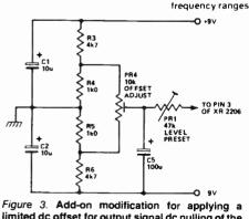
limited dc offset for output signal dc nulling of the circuit in Figure 2.
