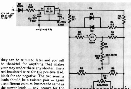
red-insulated wire for the positive lead, black for the negative. The two sensing leads should be a twisted pair — again use different colours, but not the same as the power leads — say, orange for the battery -ve terminal post lead (A) and white for the earth strap tapping lead (B). This is so that the meter will indicate in the correct direction for charge (+) and discharge (-) currents.
