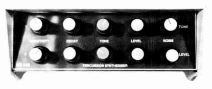
We housed our project in a light but sturdy ABS plastic case and attached a Scotchcal label to the front panel — artwork for this panel and for the pc board is reproduced on page 130. The two 'transducer' inputs, the output and supply input are located on the rear panel. Small speakers serve as input transducers and are mounted in separate small boxes.
