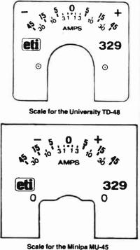
1400 ohms, while for others (particularly the University models) it is 2000 ohms. Resistors having a 1% or 2% tolerance can be used (E48 or E96 series), and values of 1k4 and 2k are available. Alternatively, a parallel combination of standard value, 5% tolerance resistors can be used and will result in sufficient accuracy in this application. For a 1k4 shunt, parallel a 1k5 and a 22k.
