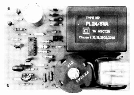
The completed pc board. Assembly is fairly straightforward (pcb pattern is on page 51).
