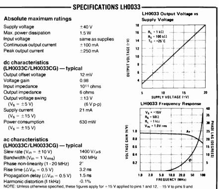
10, and pin 6 shorted to pin 7. Specifications apply over temperature range between -25°C and +85°C; typical values shown are for a temperature of 25 °C
