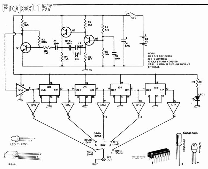
4017s). The first Schmitt inverter provides 1 MHz output, which is buffered by another Schmitt inverter to provide the 1 MHz output to the output selector switch. The output of each decade divider stage is also buffered by a Schmitt inverter to provide, respectively, the 100 kHz, 10 kHz, 1 kHz and 100 Hz outputs to SW2.
