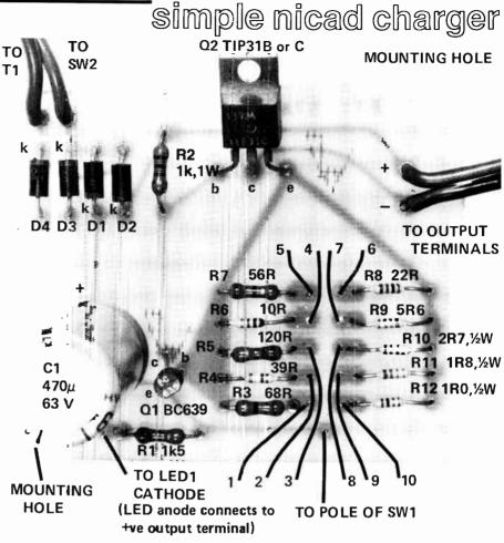
Component overlay for the pc board. Take care with orientation of the semiconductors.
