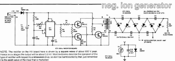
primary of transformer T1. As both Q1 and Q2 are NPN transistors, one has to receive an inverted drive signal so that it is off when the other transistor is on and vice versa. Thus Q3 is employed to invert the drive to Q2.
