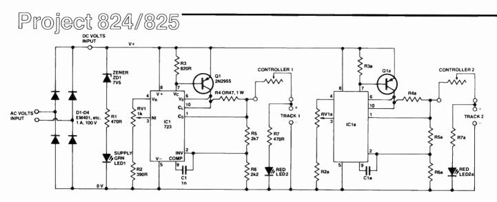
This is basically a crude series voltage regulator, based on the 723 variable regulator IC, that supplies power to the rheostat in the hand controller. The rheostat is in series with the motor in the car, via the track connections. The voltage supplied to the controller and car can be preset anywhere between about 3 V and about 12 V.
