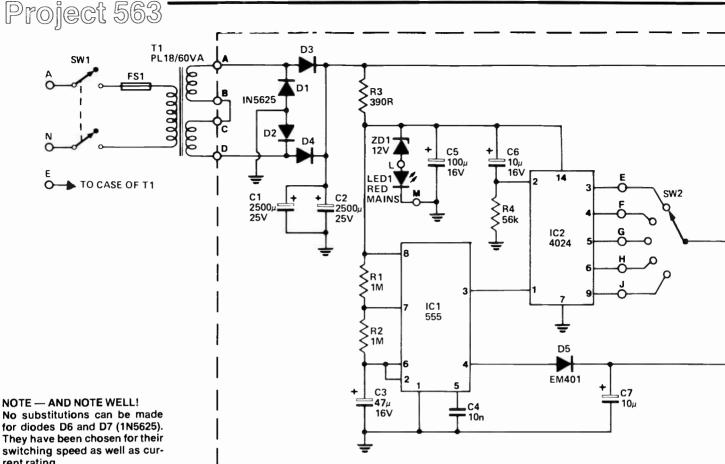
No substitutions can be made for diodes D6 and D7 (1N5625). They have been chosen for their switching speed as well as current rating.
