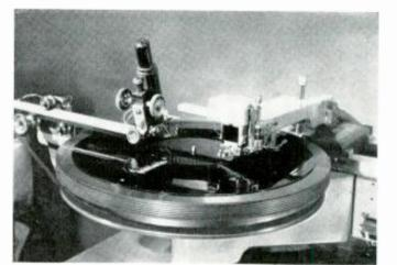
Close-up view of the master recording lathe that was used.
