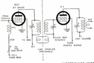
Fig. 3. Preferred circuit for r.f. driver and final amplifier.
