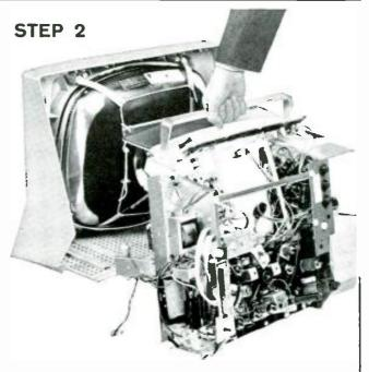
Just two more screws remove the entire chassis! If it ever becomes necessary to pull the chassis, simply remove two more screws and lift it out. The dualette carrying handle becomes a carrying handle for the chassis!
