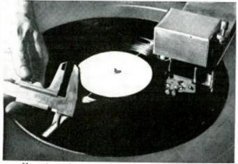
Measuring width of reflected light pattern on test lacquer.
