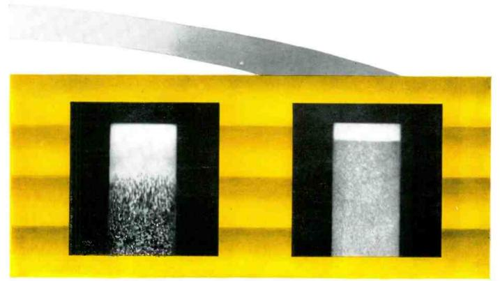
Inherent physical superiority of Sylvania's exclusive Sarong cathode, right, over a conventional cathode, left, is evident in this photomicrograph comparison. The texture,
