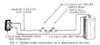
the test. Reversing one of the speaker leads will of course reverse the phasing between the two speakers by 180 degrees,
