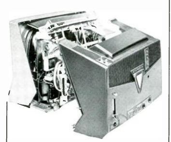
Take out only 8 screws to remove the back cover! All check points and tubes are accessible. A burned-out tube can be located in seconds! 90% of all service jobs and adjustments can be made without even removing the chassis!
