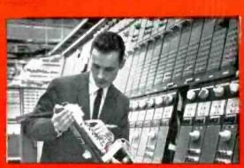
**Checking ponel wiring of Simplex console**
