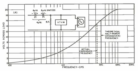
Fig. 9. Transmission curves of back-to-back or non-polarized (A) and polarized (B) electrolytic capacitors for maximum undistorted power transfer. Refer to the text.
