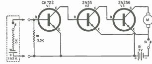
Fig. 2. Diagram of a less sensitive motor control circuit. An input control signal of  $\frac{1}{2}$  milliampere will operate the motor. The several components within the dashed lines may be used for testing the circuit. These will provide an input control current of  $\frac{1}{2}$  ma. A penlite cell may be employed.
