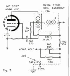
$R_{\rm M}$ . With a picture properly tuned in, the horizontal-hold potentiometer control is set to the center of its range. Then  $L_{\rm HeA}$  is adjusted for correct frequency and waveshape, the latter being the typical waveform of pulsewidth horizontal a.f.c. circuits. The top slug of  $L_{\rm HeA}$  is used to adjust for correct frequency. The bottom slug is used to achieve correct waveshape. After this is done the picture should hold sync over the entire range of the hold control.
