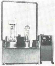
In bending, for example, only the area of the bend itself need be heated and since induction heating does this so quickly, the rest of the work piece will remain rigid and retain its shape. Fig. 4 shows a moving coil fixture in which an aluminum door handle is heated to  $900^{\circ}$  F and bent at right angles in 3 seconds, the entire operation being completely automatic, accurately controlled, and without forming scales, discoloring, or distorting.
