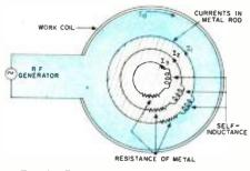
Fig. 6. Cross-section of currents in rod.
