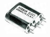
ture range is from -65 degrees C to +125 degrees C. Sensitivity is 200-250 milliwatts. The new model is offered in three different header combinations. The relay will withstand shock tests of 50 G's; vibration frequency of 20 to 2000 cps at 20 G's. Coil resistance is up to 10,000 ohms maximum and contact resistance is .020 ohm maximum.
