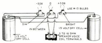
Fig. 2. A somewhat more accurate lamp output meter is shown.
