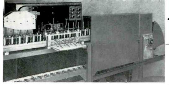
Fig. 1. A conveyor carries beaters for home mixing machines through this induction heating unit which brazes the beater blades to the main stems automatically.
