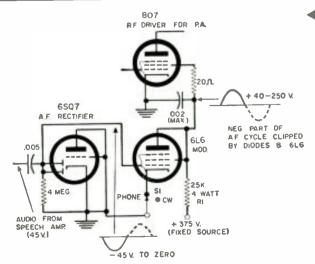
Fig. 2. Triode-connected 6L6 modulator is clamped to r.f. driver screen. Modulator draws current of only 13 ma. on zero audio.
