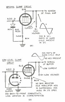
Fig. 1. Changes made in early clamp-tube circuit to allow low-level modulation. less power consumption. and lower voltages.
