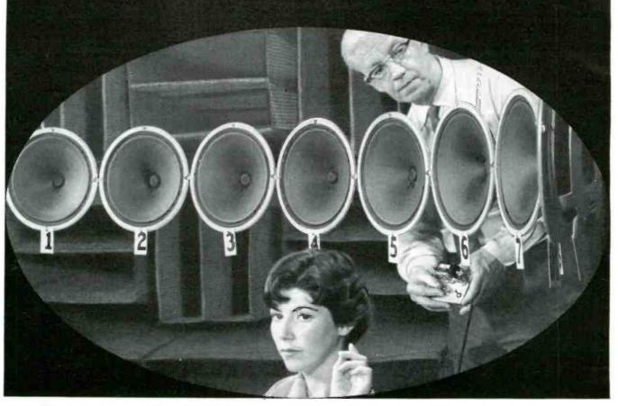
Which speaker is making the sound? In echoless chamber at Bell Labs, Robert Hanson measures test subject's ability to localize sounds — observes how two ears operate in partnership. This and other tests may point the way to better telephone instruments.
