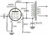
Fig. 5. The reactance tube is in shunt with the oscillator tank, through  $C_{\rm abs}$ .
