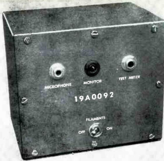
Fig. 1. Compact 27-mc. radiotelephone transmitter will take up little space in the home or office and is small enough to be clamped to car's steering post or under dash.
