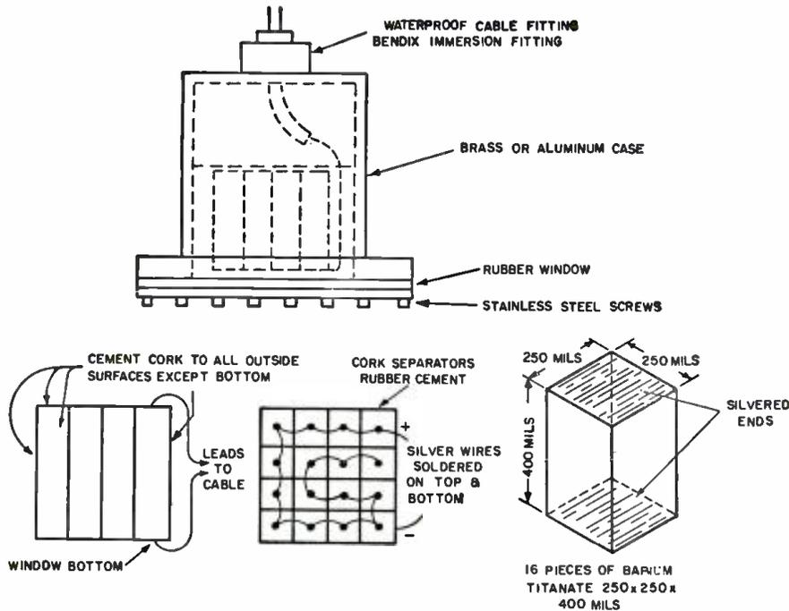
Fig. 2. Mechanical details showing the construction and assembly of transducer.
