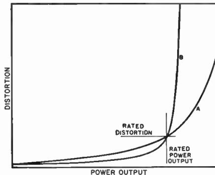
Fig. 3. Which power vs distortion curve indicates the better sounding amplifier? Both have the same rated power output and distortion rating, but (A) will probably give the better impression of distortion-free power when judged by listening test.
