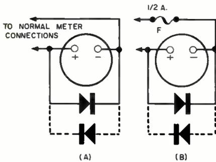
Fig. 1. Hook-ups for the protective diode(s) with and without added fuse.
