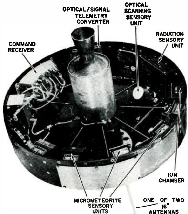
Fig. 5. Photograph of the electronics payload that is employed in "Pioneer I."
