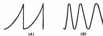
Fig. 5. Nonlinear saw-tooth output (A) from scope's horizontal amplifier will distort total trace (B) seen on screen.
