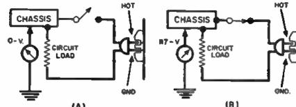
Fig. 3. This circuit presents a shock potential only when the equipment is on.
