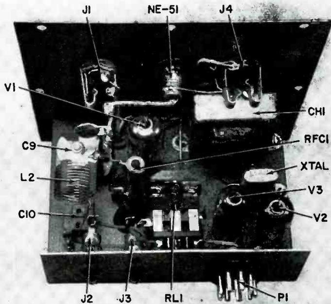
Fig. 2. Top-chassis view showing location of parts. Note that author wired up the transmitter directly from his schematic. No pictorial drawings are available.
