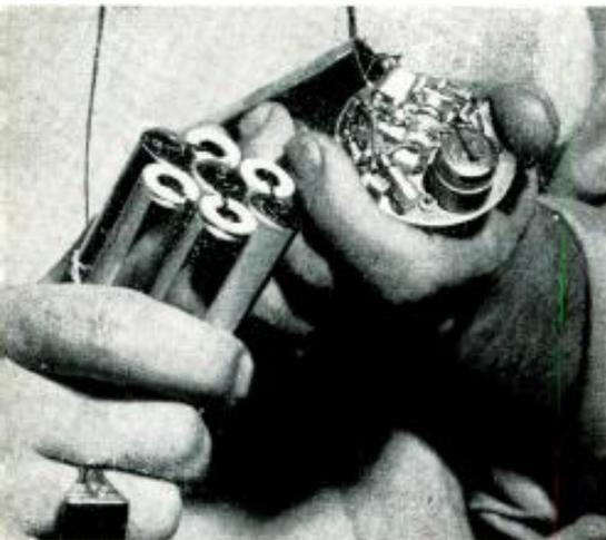
Fig. 6. Beacon or tracking transmitter with mercury battery power supply (left).
