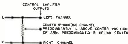
Fig. 17. Phantom channel with mixing.
