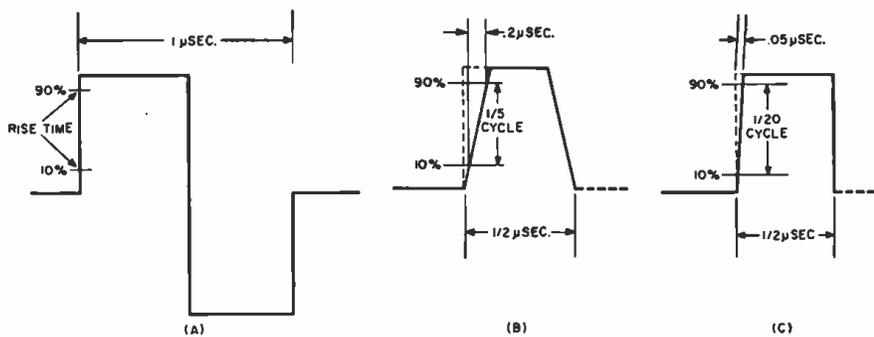
Fig. 1. A square wave (A) or any high-frequency waveform will be distorted considerably (B) by slow rise time, but only slightly (C) by short rise time.
