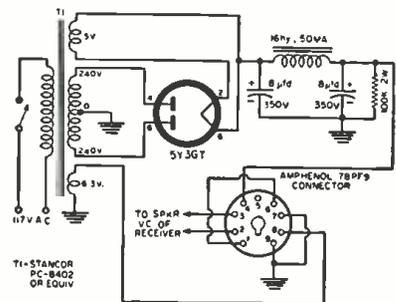
Fig. 5. Small power supply suitable for use with transmitter at fixed location.
