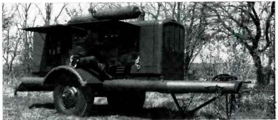
One of the two 30-kw. trailer-mounted Diesel power generators. The tubular frame actually serves as a fuel tank—holding enough fuel for 24 hours of operation.
