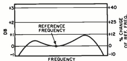
Fig. 2. A response curve, "flat" to the ear, within  $\pm 1$  db. The same variation as seen on a scope will seem less flat.
