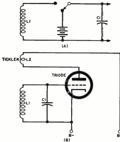
Fig. 2. (A) Basic oscillatory circuit. (B) A regenerative tube oscillator.
