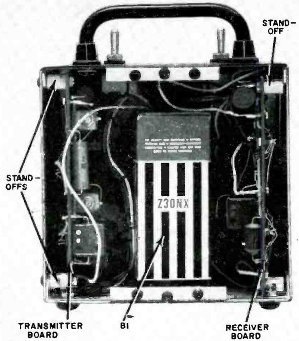
Rear view of the unit with its back panel removed. Both circuit boards, placed on edge, are mounted with stand-off posts.
