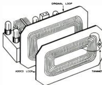
Fig. 2. Added loop antenna with tuning trimmer to act as absorption trap.
