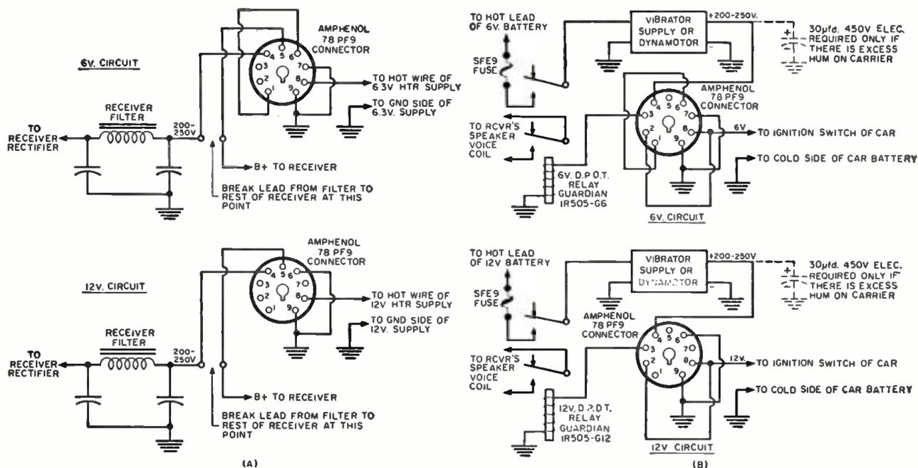
Fig. 6. (A) Methods for obtaining transmitter power from fixed or mobile receivers or (B) from a 6- or 12-volt auto battery.
