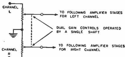
Fig. 1. Here is the circuit arrangement employed in a basic balance control hookup.
