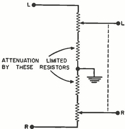
Fig. 8. The system diagram at the right shows hookup that may be employed for channel balancing. See text for operation details.
