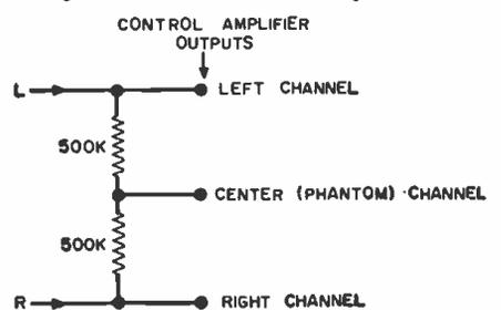
Fig. 16. Phantom channel output circuit.
