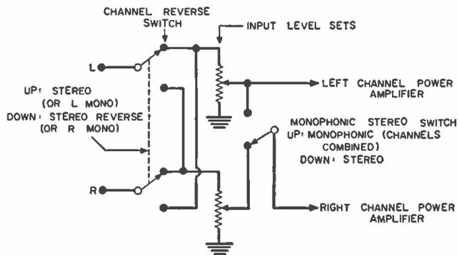
Fig. 19. Switch for feeding both outputs of stereo amplifier to a monophonic speaker.
