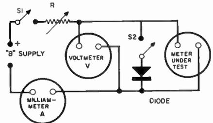
Fig. 4. The test circuit used by the author to confirm the effectiveness of the recommended protective technique.
