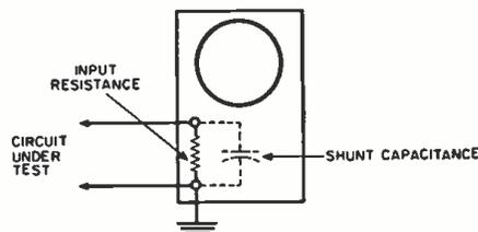
Fig. 4. Scope loads h.f. circuits with input capacitance as well as resistance.
