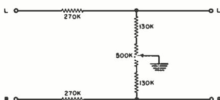
Fig. 4. Single control for channel balancing with limited (about 10 db) attenuation.
