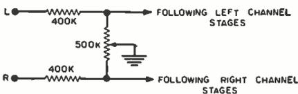
Fig. 2. Single control for balancing.
