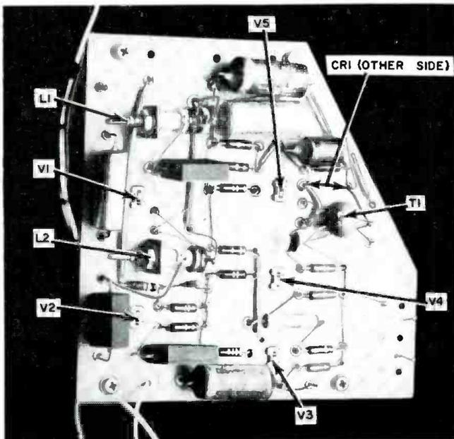
View showing components that are mounted on the receiver board.
