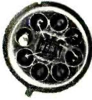
**T**HE electronics industry is on the verge of a new era with the introduction of integrated microelectronic circuits. This new concept, now in active development by a score of laboratories, can pack over a million parts into a cubic foot of space and, at the same time, greatly increase reliability. Already circuits are available in quantity, in packages only 0.3 inch in diameter and 0.2 inch high, to build complete logic and arithmetic sections of computers.
