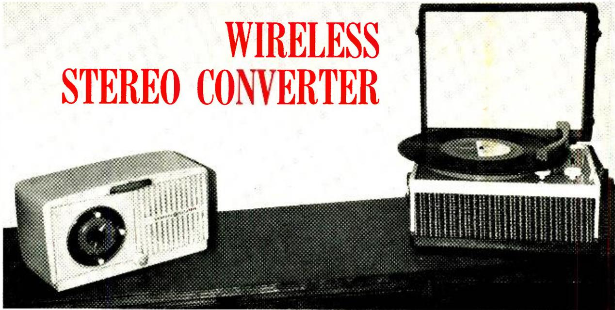
The stereo system is shown here in use. The small table radio at the left picks up the left channel from the wireless oscillator built into the phonograph. The phono plays back the right channel through its own built-in amplifier and speaker. Total cost for the conversion shown was about \$10. To convert to stereo by making a duplicate of the existing amplifier and providing an inexpensive baffle for the extension loudspeaker would have cost something on the order of \$16.00.
