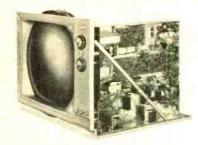
• 27 tube, 8 diode circuit with optional UHF • High definition RCA 70° 21" color tube with anti-glare, bonded face safety glass • Built-in dot generator for initial set-up adjustments • All critical circuits factory-built and tested • Au-
