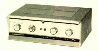
16-WATT HEATHKIT STEREO AMPLIFIER . . . OPERATES WITH MAGNETIC PHONG-GRAPH CARTRIDGES; DELIVERS FULL POWER WITHIN ± 1 DB FROM 30 TO 30,000 CPS; HAS FULL-RANGE CONTROLS, 4 STEREO INPUTS, 2 FOUR-STAGE PREAMPLIFIERS, 2 PUSH-PULL POWER OUTPUT STAGES; PLUS NEW MOCHA BROWN, BLACK & SILVER STYLING; AND IT COSTS JUST \$39.95! COMPARE AND ORDER NOW!
