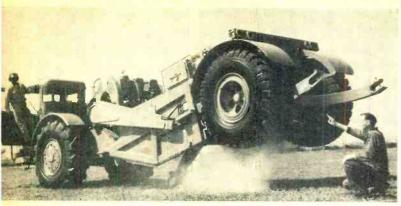
Fig. 1. A gas-explosion chamber built into this 18-ton vehicle is used to produce an acoustic shock wave for oil exploration.
