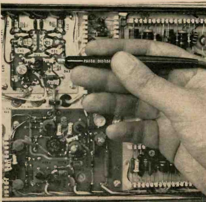
cable and the scope input circuit increase the attenuation at the higher frequencies. A simple isolation probe can only be used on signals below 10 kHz and does not permit really accurate measurements.
