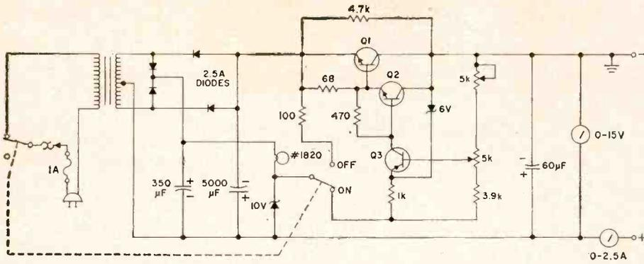
supply. Because the auxiliary supply is of opposite polarity to the main supply, a change in its zener voltage due to temperature effects tends to offset temperature effects in the main supply.
