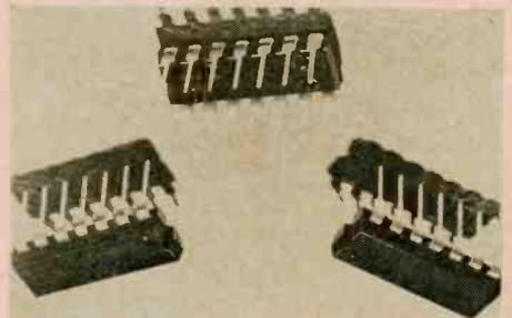
4-input gates as well as dual buffers and dual J-K flip-flops. The initial series has an operating temperature range of  $+15^\circ\text{C}$  to  $+55^\circ\text{C}$ . Motorola
