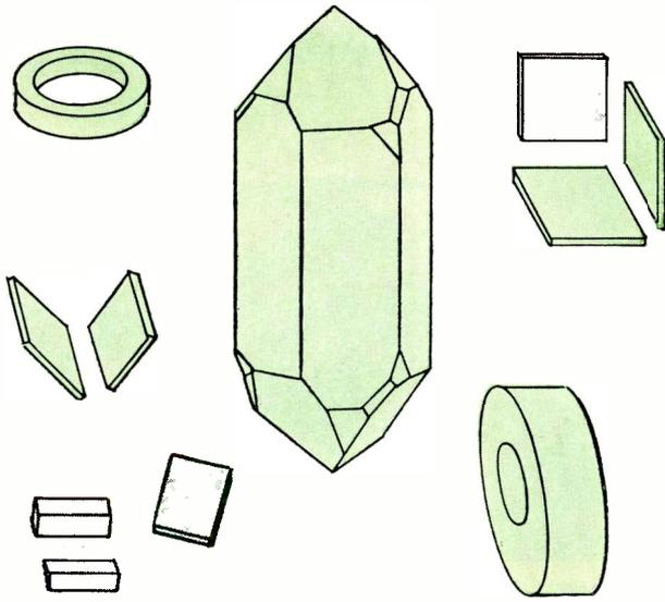
Quartz crystals are widely used in accurate electronic clocks. Cuts of various sizes, shapes, and at different angles are obtained from the larger mother quartz crystal, which is either found naturally or grown artificially at high temperatures and pressures.
