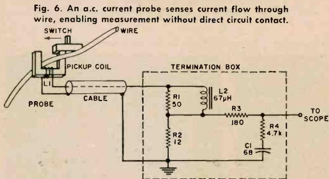
Fig. 6. An a.c. current probe senses current flow through wire, enabling measurement without direct circuit contact.
