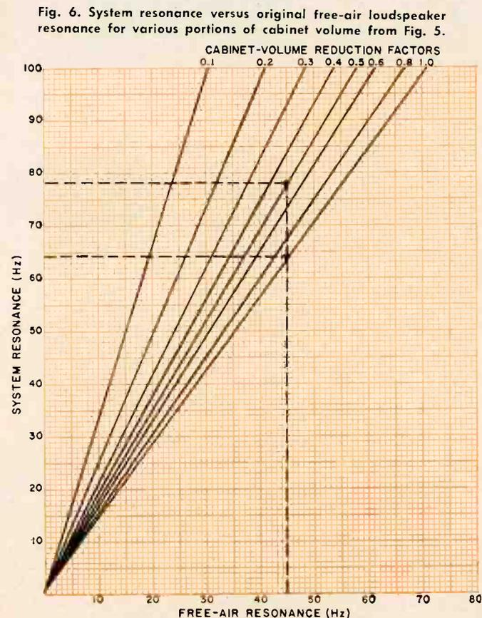
Fig. 6. System resonance versus original free-air loudspeaker resonance for various portions of cabinet volume from Fig. 5.
