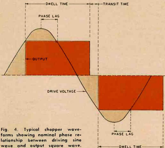
Fig. 4. Typical chopper waveforms showing nominal phase relationship between driving sine wave and output square wave.
