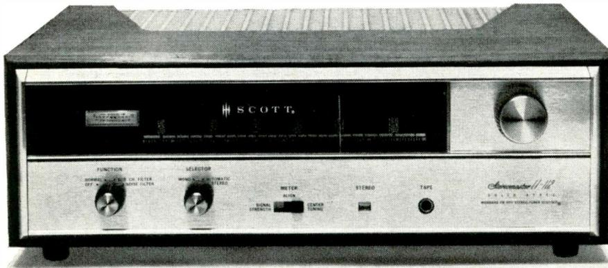
"The Scott LT-112 met or exceeded all its specifications that we were able to check. Its sensitivity was 2.1 microvolts (rated 2.2). Harmonic distortion at 100 per-cent modulation was about 0.5 percent (rated 0.8 per-cent). Capture ratio was 2.4 db (rated 4 db). Hum was -66 db, which is the lowest we have ever measured on a tuner . . . it is a logical choice for anyone who wants the finest in FM reception at a most reasonable price."
