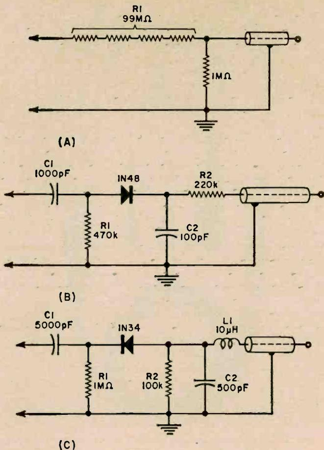
Fig. 5. (A) High-voltage (100×) probe. (B) Typical demodulator probe. (C) One variation of the demodulator probe.
