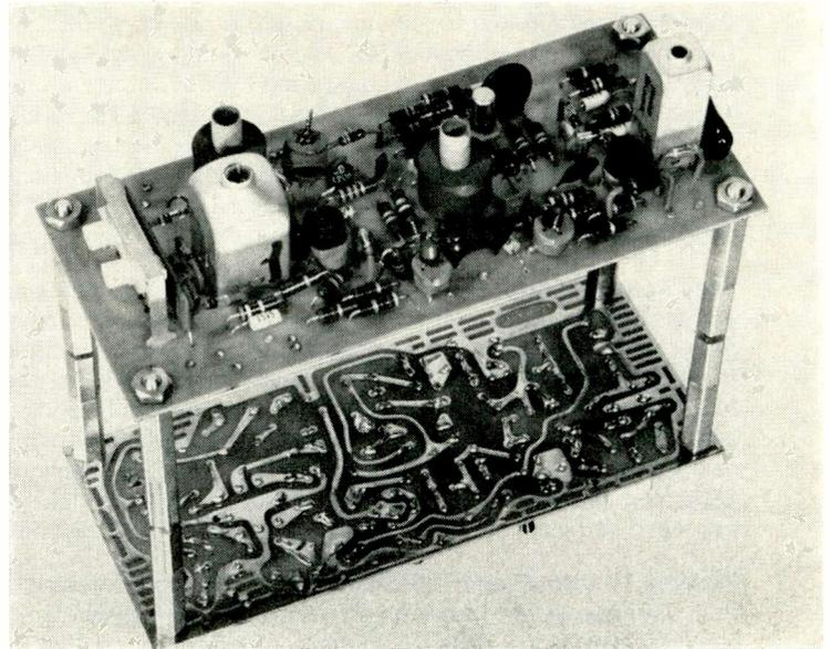
Automatic demodulator subassembly is pictured placed over a mirror in order to show its printed circuitry.
