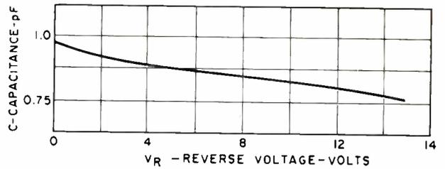
Fig. 3. Typical 1N3600 capacitance versus reverse voltage.
