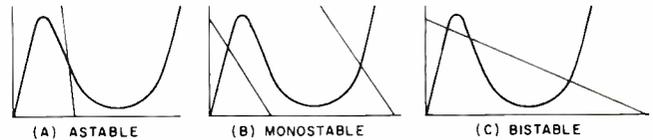
Fig. 3. Biasing modes that are employed for tunnel diodes.
