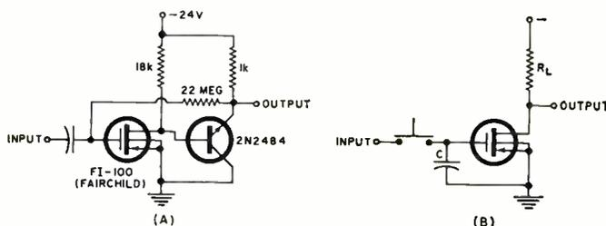
Fig. 3. (A) Adding an emitter-follower results in low output impedance. (B) "Catch and hold" circuit. (C) Proximity alarm.
