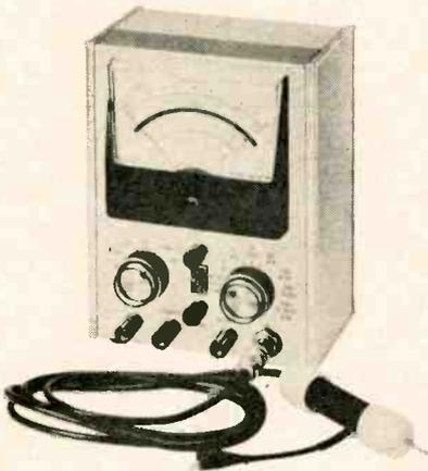
THE industry's first broadband FET voltmeter is the Model SSV-1 by Data Instruments. The new device has extremely high input impedance and can make measurements over a very wide frequency range. Input impedance on d.c. is greater than 100 megohms, and on a.c. it is about 15 megohms shunted by 2 pF.
