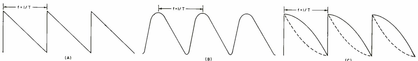
Fig. 1. (A) Ideal linear saw-tooth where the frequency is the reciprocal of time. (B) Loss of high frequencies. (C) Excessive low-frequency response can result in a bowing out of the saw-tooth, while a loss in the lows can result in a concavity.
