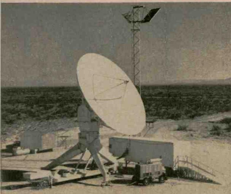
**Mobile Radar System.** (Bottom left) The mobile radar station shown here has been delivered to the U.S. Army by Sylvania recently. The station will be used as part of Project Defender, a program exploring defense against missiles and developing penetration aids for U.S. missiles. The system uses microwave and ultra-high frequency links to maintain communications between two sites. It consists of two 30-ft diameter dish antennas and vans with radar receivers and recorders.
