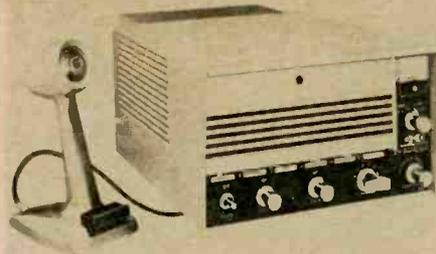
The unit will mount under the dashboard of most vehicles, eliminating the necessity of a separate control head and connecting cables. Transistorization has reduced the current requirement to less than 0.16 ampere on receive, permitting constant monitoring without excessive battery drain. Plug-in power modules, either a universal 12, 24, 32 volt d.c. or a 115/230 volt a.c. unit, permit instant conversion from mobile to base-station use.
