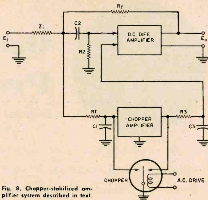
Fig. 8. Chopper-stabilized amplifier system described in text.
