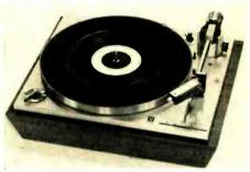
shape and friction; a cartridge shell that accepts all cartridges with an exact slide-fit mounting; a single-lever command center which controls start, stop, repeat, cueing, and lift; automatic start and shut-off in either single play or with a stack of records; and an exclusive automatic scanning device which measures the diameter of any record and adjusts the tonearm accordingly.
