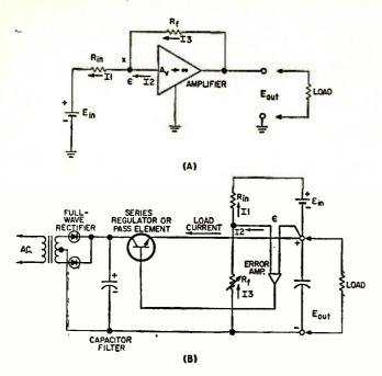
Fig. 2. (A) Operational amplifier. (B) Regulated supply.
