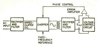
Fig. 4. Efficient phase-modulated switching power supply.
