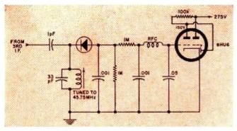
Fig. 5. Target-ray tube used as tuning indicator in a Philco.
