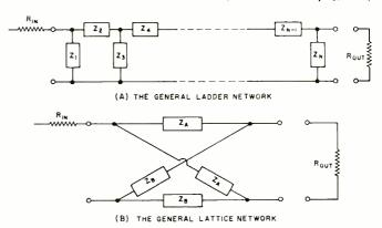
Fig. 2. (A) Unbalanced and (B) balanced arrangements.
