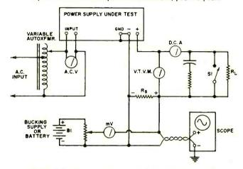
Fig. 4. Setup for measuring constant-current power supply.
