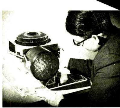
Infrared Scanner for Moon Landings. (Top left) The 24-in telescope shown is equipped with an infrared scanning system to evaluate possible Apollo landing sites. By analyzing the heating and cooling rates of lunar areas during the day-night cycle, information becomes available for planning touchdown and subsequent exploration. The IR scanner, designed by Barnes Engineering, is attached to the back of the telescope tube while associated electronics is in cabinet shown at the bottom.
