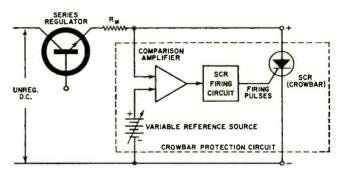
Fig. 5. Typical crowbar overvoltage protection circuit
