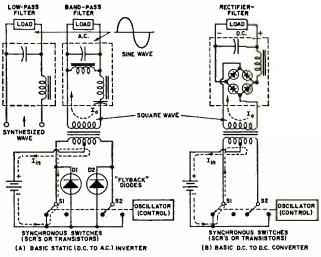
Fig. 1. Basic configurations of (A) inverter and (B) converter. Direction of electron current flow is indicated by dashed arrows.
