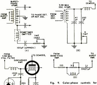
adjusting the hue or tint. (A) Most popular: control and coil or capacitor across half of burst-transformer secondary. (B) Similar, but across oscillator output transformer. (C) Capacitance diode shifts phase of burst fed to subcarrier amp. (D) Another simple control.
