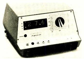
THE Model 333 "Digitest" digital multimeter has been introduced by Honeywell for the technician who likes the versatility of a v.o.m., but who still requires the accuracy and convenience of a digital voltmeter. The meter can be operated from either built-in rechargeable nickel-cadmium batteries or the a.c. power line. A built-in charging circuit is provided. Automatic overrange indicator, decimal point placement, and polarity indication are included.
