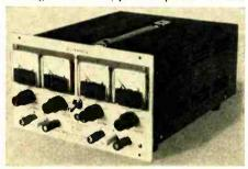
outputs, the supplies can yield two times the voltage or two times the current, up to 500 volts or up to 3.4 amps. Auto series/auto parallel (master-slave) permits tracking to a common reference. Four meters provide simultaneous monitoring of both voltage and current for each output. Crowbar overvoltage protection up to 70 volts d.c. is available as an accessory.
