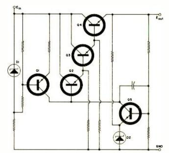
Fig. 2. Schematic of Beckman's hybrid voltage regulator.
