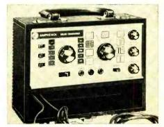
The generator is housed in a luggage-type case, with handle, that has plenty of storage space for probes, tubes, etc. Amphenol Distributor Div. Circle No. 3 on Reader Service Card
