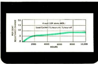
Typical stability test data: 10,000-hour load cycling test. Average resistance change is less than 1%!
