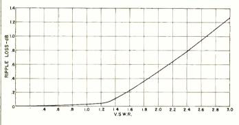
Fig. 3. The amount of loss due to ripple for various v.s.w.r.'s.
