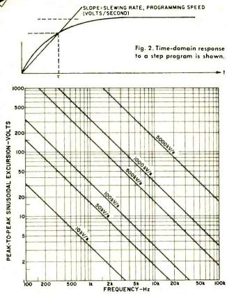
Fig. 3. Chart showing the maximum sinusoidal frequency vs the peak-to-peak voltage excursions for number of slewing rates.
