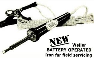
Now get controlled 700°F tip temperature from a battery! Lightweight TCP-12 iron features Weller's patented "Temperature Sensing" system, clips to any 12-volt battery or 12-14 volt AC/DC source. Also available for 24-28 volt operation (Model TCP-24). A must for mobile communications work.
