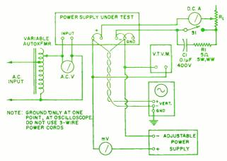
Fig. 2. Setup for measuring constant-voltage power supply.
