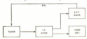
Fig. 7. Closed loop that forms automatic fine-tuning system.
