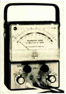
THE new WT-501A recently introduced by RCA is a portable, battery-operated transistor tester, designed for both in-circuit and out-of-circuit applications. The instrument measures d.c. beta from 1 to 1000, collector-tobase leakage ( $I_{CBO}$ ) as low as 2  $\mu$ A, and collector-to-emitter leakage ( $I_{\rm CEO}$ ) ranging from 20 µA to 1 A. Special lowimpedance circuitry assures reliable measurement of in-circuit transistor current gain.
