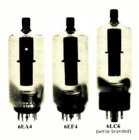
In early 1967, General Electric started a modification program to eliminate the possibility of soft downward x-radiation emission from some of its large screen color television receivers. This modification program, which involved replacement of the obsolete regulator tubes pictured above, is now complete except for a very few receivers which have not yet been located.
