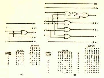
Fig. 8. Logic diagrams and state tables of biquinary decoders for both the (A) modulo 6 binary counter and (B) modulo 10 binary counter circuits shown in Figs. 4 and 5, respectively.
