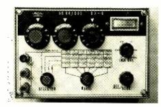
tion testing as well as for laboratory applications. The portable unit is powered by an inexpensive 9-volt battery although six 11/2-volt penlight cells may be used as well.
