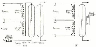
Fig. 3. (A) Electrical and (B) magnetic latch. The dots indicate similar magnetic polarity; a reversal of such polarity is obtained by either reversing the electrical polarity of the applied voltage or reversing the winding direction of the coil. In (A) the circuit is latched or held closed by application of smaller, magnetically in-phase latching signal; circuit is reset by opening reset switch. In (B) circuit is latched by aiding PM; reset is by magnetically bucking reset-coil field.
