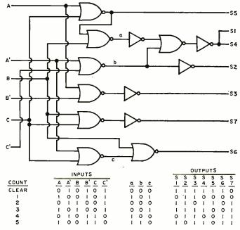
Fig. 14. Logic diagram and state table of BCD-to-seven segment decoder for modulo 6 binary counter shown in Fig. 4.
