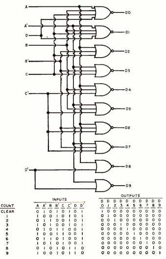
Fig. 12. Logic diagram and state table of BCD-to-decimal decoder for the modulo 10 binary counter shown in Fig. 5.
