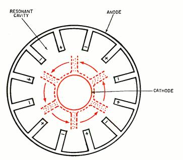
Fig. 5. Magnetron cross-section showing 12 resonant cavities and rotating "spokes" of focused clouds of electrons moving from central cathode to anode under influence of high voltage.
