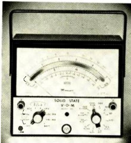
low-power ohms circuit, on the other hand, applies only 35  $\mu$ W of power to the device under test on the corresponding range, and lower power at the higher resistance ranges. This means that we can measure front and back resistance of transistors, diodes, and IC's without the ohmmeter voltage source biasing the semiconductors either into or out of conduction.
