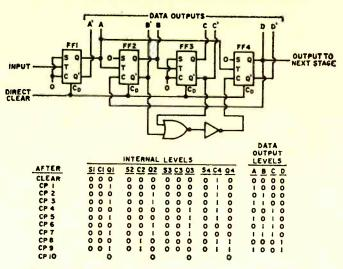
Fig. 5. Modulo 10 binary counter logic diagram and state table.
