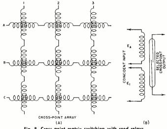
Fig. 8. Cross-point matrix switching with reed relays.
