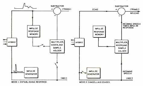
Fig. 7. Echo canceller of the impulse-response type is illustrated. For clarity, each line represents a pair of wires.
