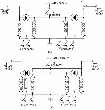
Fig. 7. Reed-relay flip-flops with (A) electrical and (B) magnetic memories. Number of contacts used is optional.
