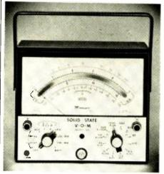
N EW solid-state v.o.m.'s are coming from the test-equipment manufacturers almost faster than we can count them. One of the latest we have seen is the new *Triplett* Model 801. The manufacturer refers to this unit as a laboratory instrument and it should find much use not only in laboratories but for advanced electronic servicing as well.
