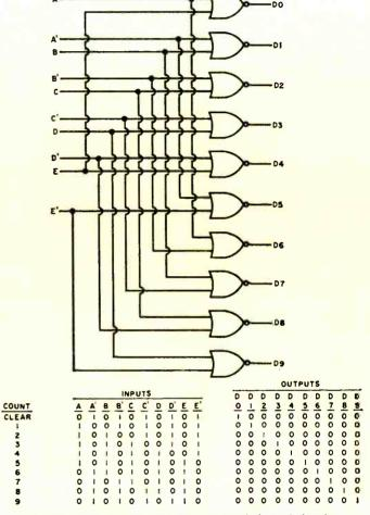
Fig. 10. Logic diagram and state table of decimal decoder for the modulo 10 ring counter circuit shown in Fig. 7.
