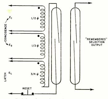
Fig. 9. Circuit diagram of matrix element with a memory.
