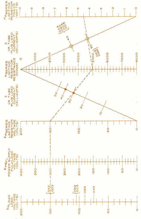
Fig. 3. Design nomogram showing resistance and power for series limiting resistor.
