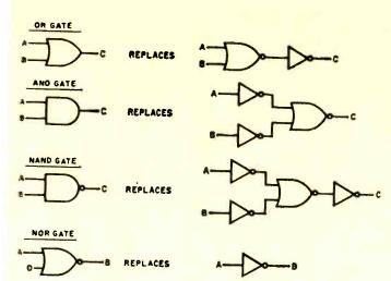
Fig. 2. The "nor" gates and inverter combination on the right may be replaced with the logic elements shown on the left.
