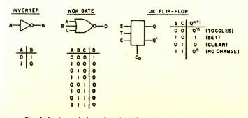
Fig. 1. Logic symbols and truth tables of basic logic elements.
