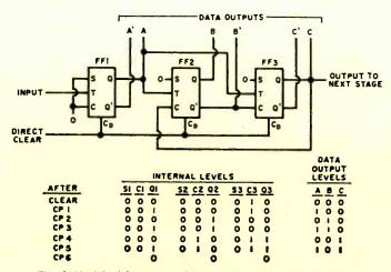
Fig. 4. Modulo 6 binary counter logic diagram and state table.
