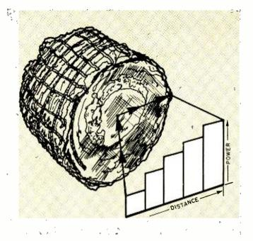
Fig. 7. More power is absorbed near the outside of food, such as a beef roast, than is absorbed near the center.
