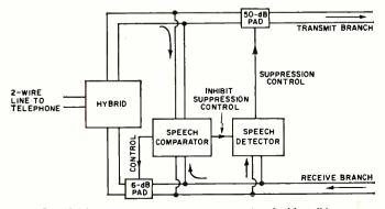
Fig. 6. A current echo suppressor permits double-talking.
