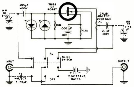
\* IN914 OR ANY HIGH-FREQ., HIGH-BACK-RESIS. SILICON DIODES FOR GATE PROTECTION \*\* OPTIONAL ADJUSTMENTS FOR BEST SQUARE-WAVE RESPONSE
