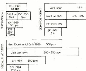
Fig. 5. Graphs comparing exhaust emission control of contaminates of car equipped with EFIs y s t e m with those using 1969 carburetor and California's 1974 requirements.
