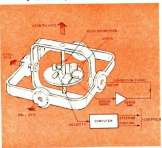
Fig. 2. This is a simplified representation of the gimbaled stable platform that is the heart of the system's navigation unit. There are three accelerometers which sense the magnitudes of the three components of the jet's acceleration, and three gyroscopes to control direction in which accelerometers' sensitive axes point.
