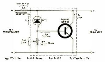
Fig. 1. Schematic of simple shunt regulator circuit. Components in box are used to simulate large (10- to 50-W) zener.
