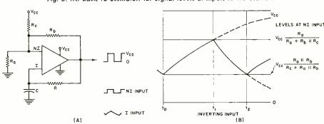
Fig. 3. (A) Basic IC oscillator. (B) Signal levels at inputs to the oscillator.
