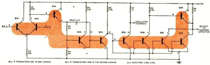
Fig. 4. Schematic diagram of the IC generator section, which employs two IC transistor arrays.
