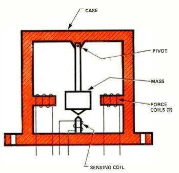
Fig. 1. Schematic representation of an accelerometer.
