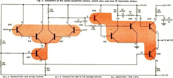
Fig. 5. Schematic of the meter-amplifier section, which also uses two IC transistor arrays.
