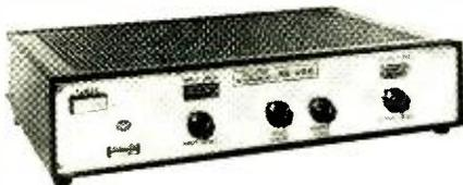
Model RE-100. The unit uses IC's and incorporates computer technology to provide a compact unit. Input and output amplification and equalization are self-contained and no additional equipment is required for connection to a system. Front-panel switches provide selection of various types of reverb and reverb time. Melcor
