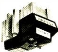
Here is why fractions-of-a-gram are important to record and stylus-tip life:  $\frac{3}{4}$  gram tracking exerts a pressure of 60,000 lbs. per sq. in. on the groove walls—and this rises to 66,000 lbs. per sq. in. at 1 gram, and 83,000 lbs. per sq. in. at 2 grams. At 2 grams you have added over  $1\frac{1}{2}$  tons per sq. in. to the groove walls over  $\frac{3}{4}$  gram tracking! Think about it.
