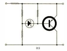
Fig. 2. Circuit schematics of various shunt regulator types. (A) Grounded-collector "p-n-p" for positive output, (B, C) "n-p-n" and "p-n-p" configurations, respectively, for higher output voltages than available selection of zeners, and (D, E) Darlington "n-p-n" and "p-n-p" cascade types, respectively, for increasing amplification factor.
