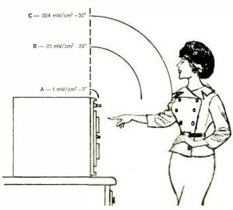
Fig. 1. Examples of microwave-radiation power densities at various distances. Leakage occurs only around the door seal.
