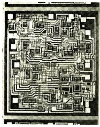
Fig. 4. Photomicrograph of Motorola's MRTL MC780P decade up-counter digital IC that operates at frequencies to 4 MHz.
