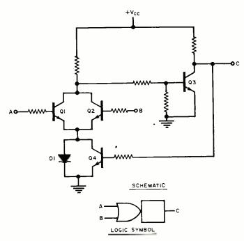
Fig. 2. This schematic diagram of an IC Schmitt trigger shows how an IC device sometimes uses a different circuit design approach than discrete component counterpart. Most obvious difference is dual signal/gating inputs and the diode and transistor in the emitter circuit of Q1 and Q2. Note the logic symbol.
