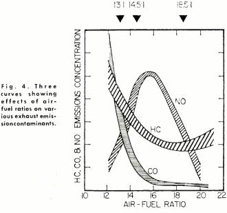
to I air-fuel ratio range (middle arrow on top axis). From the curves of Fig. 4, we can see that the three contaminates can be significantly reduced by running the engine very lean at approximately 19 to 1 air-fuel ratio. The curves also show that if a reactor is used, (Continued on page 68)
