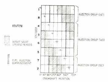
Fig. 2. Injection timing chart for a typical eight-cylinder American car having a firing order of 1-8-4-3-6-5-7-2. The fuel is injected to each group of cylinders at the same time.
