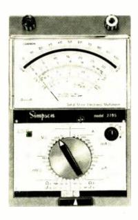
THIS new Simpson Model 2795 solid-state v.o.m. has no less than 68 switch-selectable functions plus 12 output (dB) ranges. It can measure a.c. and d.c. voltages as low as 1 mV full-scale, a.c. and d.c. currents as low as 1  $\mu$ A full-scale, and it has six low-power resistance ranges that are safe to use for measuring transistor and 1C resistance values. The meter is temperature-compensated over a range of 0° to 50°C, and has a rated accuracy of  $\pm 1$  percent for both a.c. and d.c.
