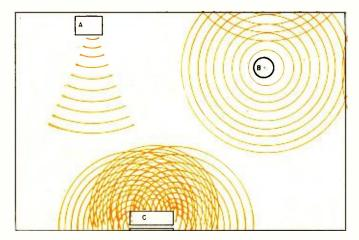
Fig. 2. Simplified representation of (A) directional sound source, (B) omnidirectional source, (C) diffuse source.
