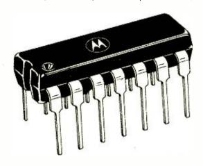
Fig. 5. This 14-pin plastic dual in-line package (DIP) is used for popular MC700/MC9700 series of resistor-transistor logic.
