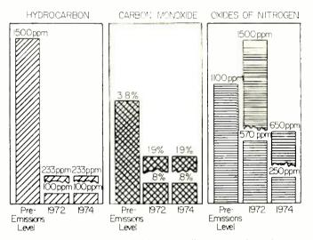
Fig. 3. Graphs showing California's pollution control requirements that must be met by automobile manufacturers in 1970's.
