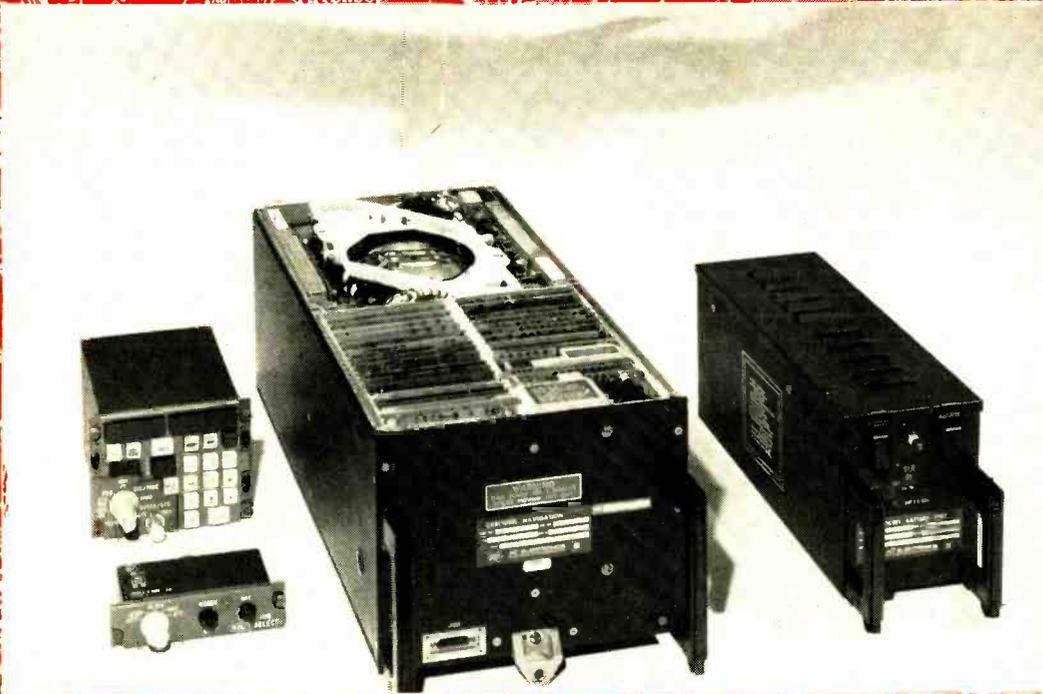
These black boxes make up the inertial navigation system. At left are the pilot's links with the all-weather system, the mode selector in foreground, and the display
