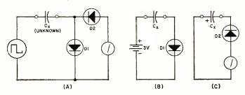
Fig. 1. (A) Basic circuit of capacitance meter. (B) Charging and (C) discharging of the unknown capacitor is shown.
