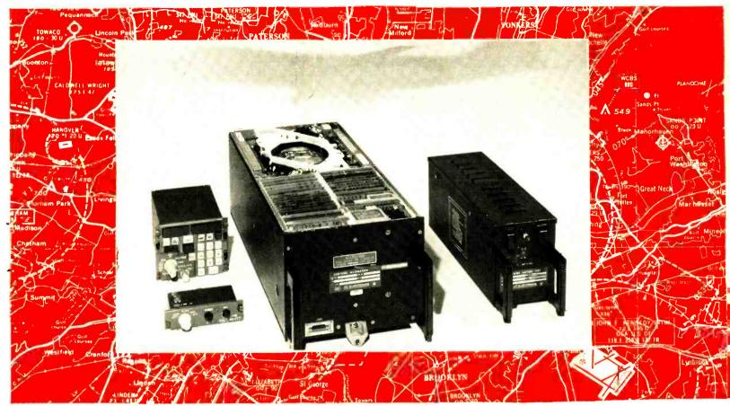
These black boxes make up the inertial navigation system. At left are the pilot's links with the all-weather system, the mode selector in foreground, and the display unit. At center is the heart of the system, the navigation unit, which contains inertial platform and a high-speed digital computer. At right is the backup battery supply.
