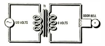
In this door bell circuit, which kind of transformer is T<sub>1</sub> — step-up or step-down?
