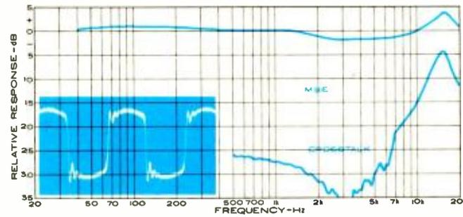
M3D required 3 grams, while the M91E and V-15 Type II (Improved) operated well at 1 gram. The V-15 was able to cope with most music records at  $\frac{3}{4}$  gram, but had considerable IM distortion at high velocities with that force and we would favor operating it at 1 gram.
