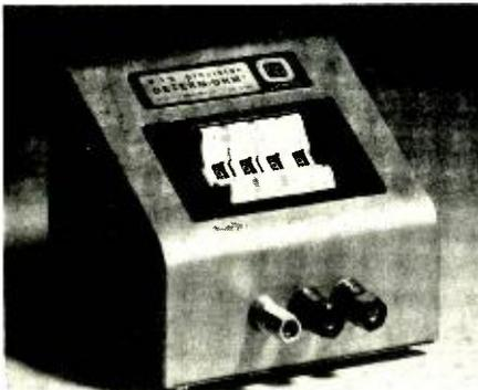
RESEARCH and development labs frequently make use of precision resistance decade boxes in some of their measuring and testing setups. Such boxes are also useful for some production-line tests where exact resistance values are needed. Service technicians also use decade boxes to make component substitutions although this application requires higher power and much lower accuracy resistors than the ones used in the new *Ohmite* "Determine-Ohm" decade boxes.
