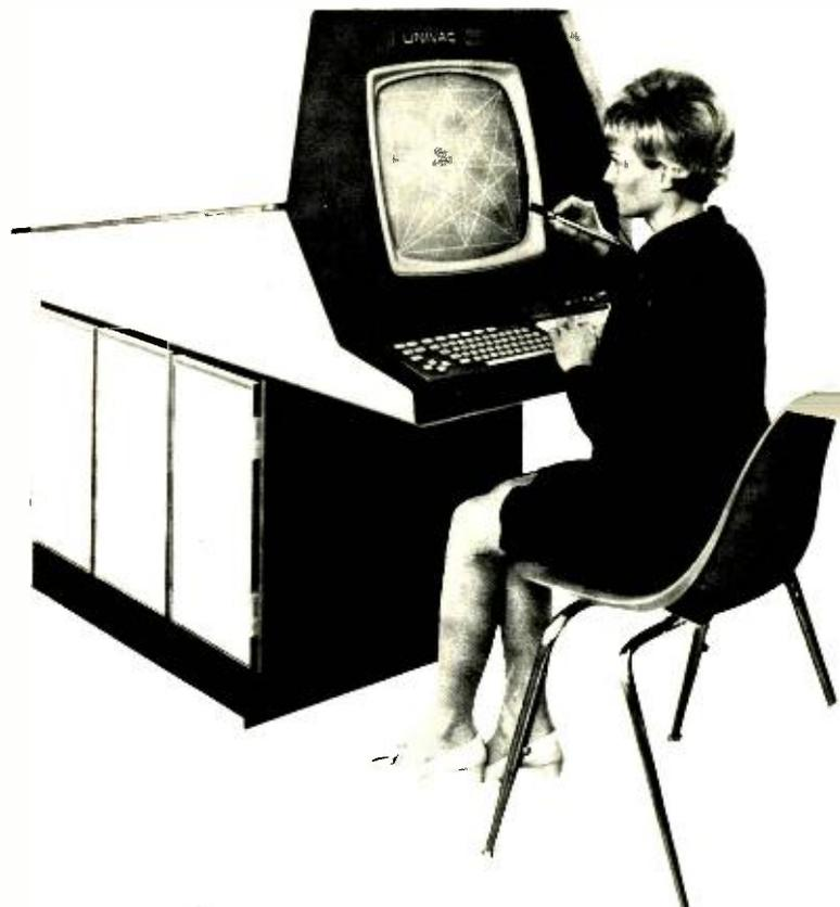
The operator is shown using light-pen device to draw geometric figure on graphic display terminal screen. Light pen can also be used by operator to wipe out any line it touches by using in "erase" mode.
