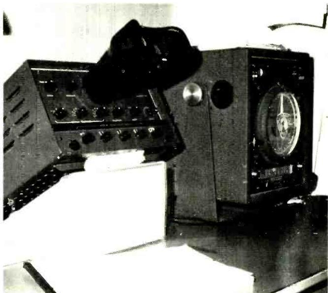
Fig. 4. Shown here are (left) modern Loran set and (right) radio direction finder that marine service technicians must be thoroughly familiar with in order to make needed repairs.
