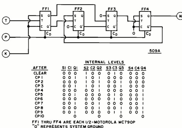
Fig. 12. Logic diagram and the state table for the minimum-hardware modulo-10 counter circuit (509A) shown in Fig. 3.
