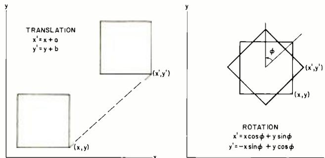
Fig. 3. Examples of kinds of (left) translations and (right) rotations made possible with graphic terminal/CPU system.
