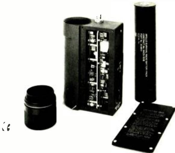
Fig. 4. Transceiver with covers removed. Battery pack shown on right is contained in the cylindrical compartment and retained by the screw-on cap shown. The electronics package, containing the receiver and transmitter circuit boards, becomes accessible when the flat cover is removed. The flexible quarter-wave whip antenna can be seen in the foreground.
