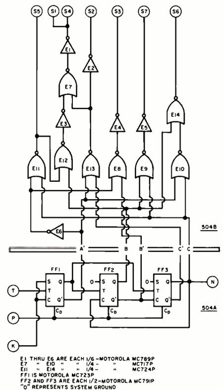
Fig. 6. Logic diagram of modulo-6 binary counter and BCD-to-seven segment decoder used with drivers and readouts of Fig. 8.
