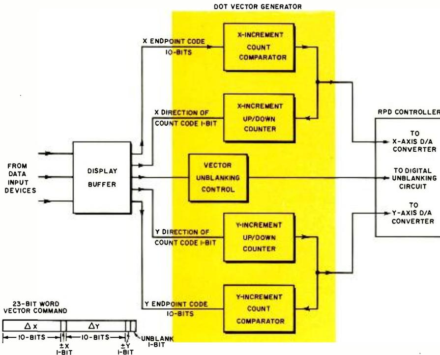
Fig. 1. Block diagram of dot-vector generator used with random-point display controller to permit vectors to be plotted in same time it takes to plot single point. As shown in illustration, typical vector-command word contains 23 bits.
