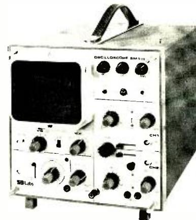
ment offers 2 mV/cm to 50 V/cm range, a time base of 200 nanoseconds/cm to 1 s/cm, and a 10 cm × 8 cm CRT with a phosphor 31 trace.
