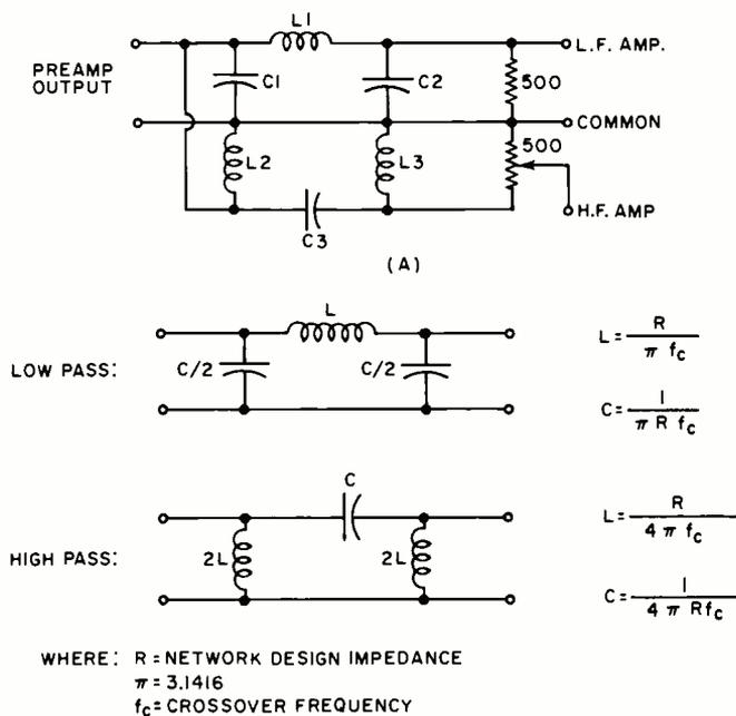
Fig. 4. Frequency-dividing networks used at input of amplifier.
