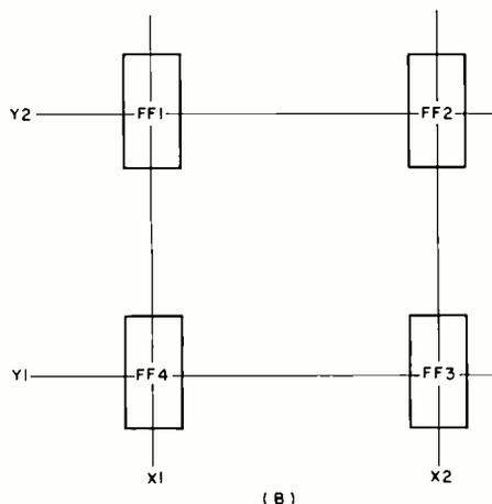
Fig. 2. Random-access memory showing the write and sense control lines.
