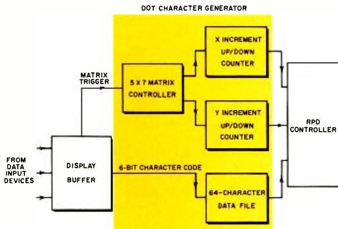
In the dot-character generator mode, the X- and Y-axis up/down counters automatically scan out a  $5 \times 7$  dot matrix. When they complete the scan of one of these matrices, the counters move the beam to the next character position where they can scan through another matrix.
