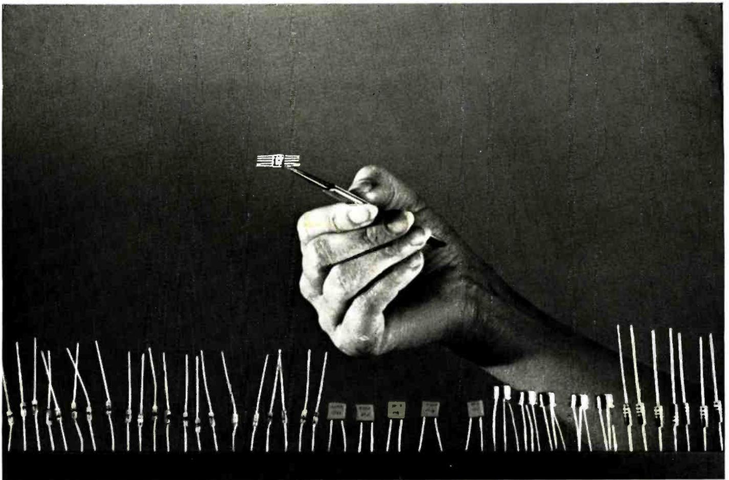
50 functions in a single chip. The functions of 50 separate transistors, diodes, resistors and capacitors can now be performed by the tiny dot in the center of the integrated circuit held by the tweezers.
