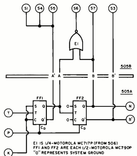
Fig. 7. Logic diagram of modulo-4 binary counter and BCD-to-seven segment decoder used with drivers and readouts of Fig. 8.
