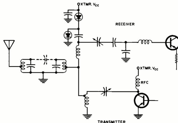
Fig. 2. Schematic diagram of the antenna coupling network.
