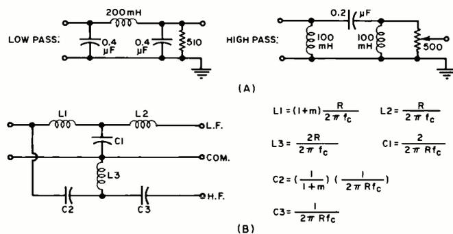
Fig. 5. (A) Values used by author. (B) M-derived filter networks.
