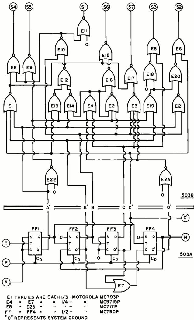
Fig. 5. Logic diagram of modulo-10 binary counter and BCD-to-seven segment decoder used with drivers and readouts of Fig. 8.
