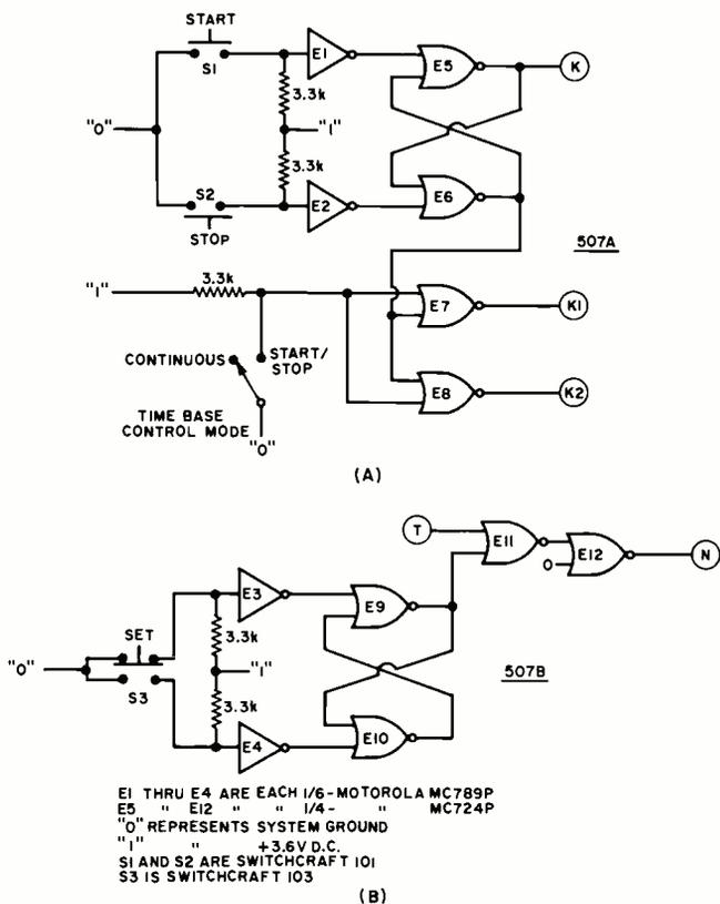
Fig. 9. Logic diagrams of the (A) Start/Stop control circuit (507A) shown in Fig. 2 and of the (B) Time-Set circuit shown in Fig. 2.
