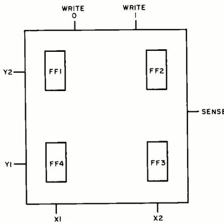
It has been shown that a single FF can store a "0" or "1". However, for large-memory operation, many FF's are needed, therefore making it convenient to arrange them in symmetrical fashion. Fig. 1B shows four FF's in a conventional 2 x 2 matrix configuration. Statements about this small matrix can be directly applied to a matrix of any size.
