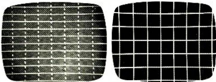
On the left, a pattern\* produced by an ordinary color bar generator. On the right, the equivalent pattern\* produced by Leader's LCG-388. Perfectly stable, the instant you turn the power on.
