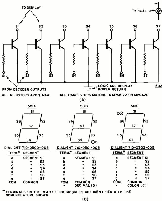
Fig. 8. (A) Schematics of display drivers and (B) layout and terminal arrangement of Dialight 7-segment digital readouts.
