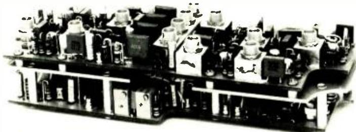
Fig. 5. Electronics package showing receiver circuit board mounted on top and the transmitter circuit board on bottom.
