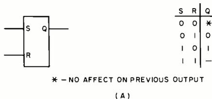
Fig. 1. (A) Logic symbol of set-reset flip-flop and its truth table and (B) a conventional 4-element flip-flop.
