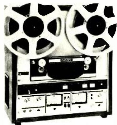
and completely modular electronic construction. Fully accessible bias and equalization adjustments make service and maintenance easy. The two-track and quarter-track head blocks can be interchanged in seconds with no need for head realignment. Each head block contains one erase, one record, and two playback heads.
