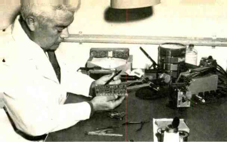
Author points out one of the encapsulated microcircuits which require precision soldering. NASA has established new high-reliability standards and Lowry AFB has developed tools.
