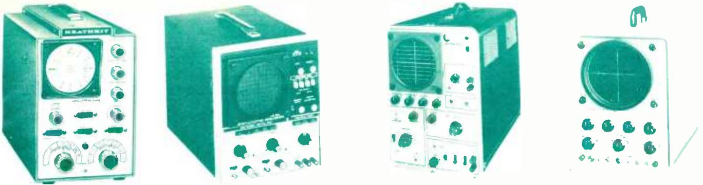
Some of the newer bench-type scopes: Above (from left to right): Heathkit IO-101 vectorscope; Sencore PS163; Lectrotech TO-50; Simpson 458. Below Eico 465. Bottom (from left to right): Leader LBO-301; Hickok 5002; Kikusui 5122; RCA WO-33A.
