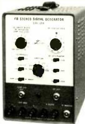
with a continuously adjustable frequency range of 75 to 110 MHz. Separation is over 30 dB from 50 to 15,000 Hz.
