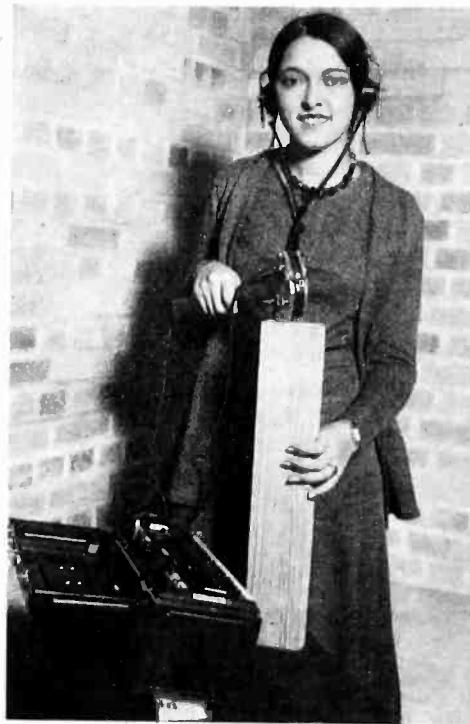
Portable instrument devised by U. S. Bureau of Standards to measure moisture in lumber. Nail-like contacts are driven into board-end
