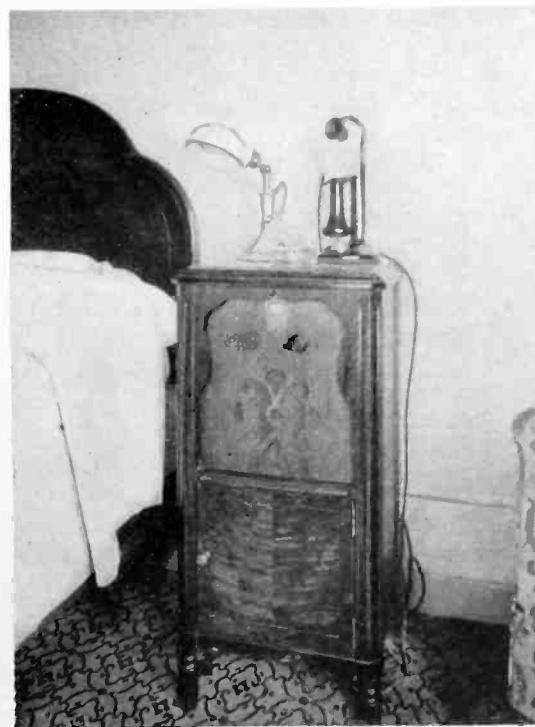
Fig. 3—Individual radio receivers using one tube are installed in a standard bed-side table
