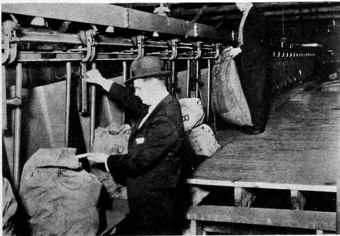
ABOVE Setting the photocells at proper levels corresponding to destinations of bags. Each level corresponds to an unloading platform. When the light is passed, the carrier opens
