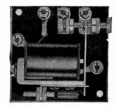
These relays will operate on approximately 14 milliwatts. Where smaller gaps between contacts are permissible, the relay can be adjusted to give positive operation on 4 milliwatts.
