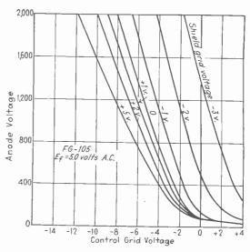
Fig. 6—Effect of varying shield grid voltage on relation between anode and control grid voltages at start of discharge
