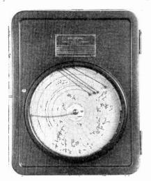
contacts for the relay as well as the galvanometer contacting mechanism, the recording chart, and the automatic standardizing relay contacts.
