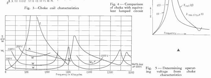
frequency rises, the valleys in the watts curve also become filled in to a greater degree.
