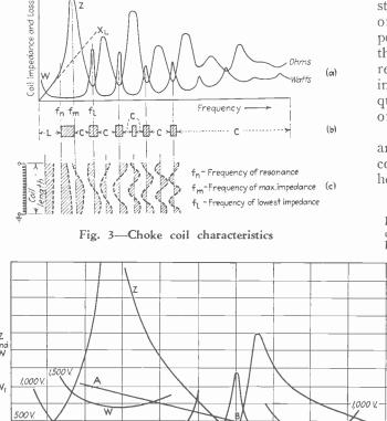
The measurement of impedance was repeated for several different coils, and in each case the results were in general the same as those just described. These results do not bear out the assumption mentioned above, that the distributed capacity can be regarded as a single lumped capacity shunting the coil, because:
