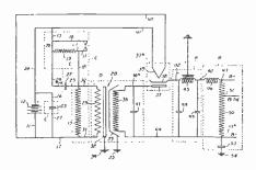
**Cold tube amplifier.** A multi-stage amplifier with several glow discharge devices having cold electrodes. August Hund, Wired Radio, Inc. No. 1,950,003.
