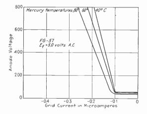
Fig. 1—Grid current at start of discharge for 3-element tube
