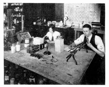
Material entering into cathodes must be accurately weighed and gaged
