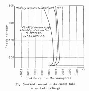
With this test the FG-57 initially passes a test which requires it to cease conduction (after five minutes warming up operation at full load) with a resistance of 10 megohms and a negative voltage of not more than 50, whereas the FG-95 under the same conditions is capable of cuting off with a resistance of 100 megohms and a negative voltage of not more than 50.
