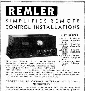
Small adaptor units available at low cost which plug into condenser microphone inputs, leaving main units perma-nently equipped for condenser microphone operation. Reliable, economical and efficient. Features include: level indicator, ladder attenuators, main gain control, and lock connectors, 60db. gain at 1000 c.p.s. Impedance inputs: 50 to 500 ohms. Output impedance: 600 ohms. Power supply 100 to 130 volts. Attractive discounts to Broadcast Stations
