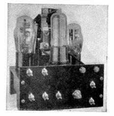
and utilizes a unique circuit. In this unit one-half of the 25Z5 furnishes plate voltage and the other half furnishes fixed bias for the grid of the amplifier. In this manner the bias on the tube is independent of changes in plate current produced when the illumination on the phototube changes.
