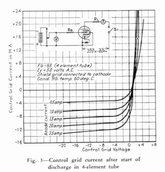
duces an impedance drop in these circuits which tends to reduce the actual grid voltage. In very high impedance circuits this drop tends to make the operation of the tube independent of the intended actuating voltage. In addition to this, the impedance drop may vary, for example, as the grid emission changes, due to the tube warming up under load, the grid current would vary and thus operation would be made unreliable.
