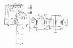
Traffic signal. Traffic varies the oscillatory character of a vacuum tube circuit. W. C. Nein and T. W. Varley, New York. No. 1,950,741.
