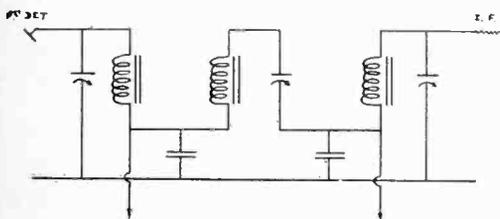
Circuit used in iron-core-coil receiver
