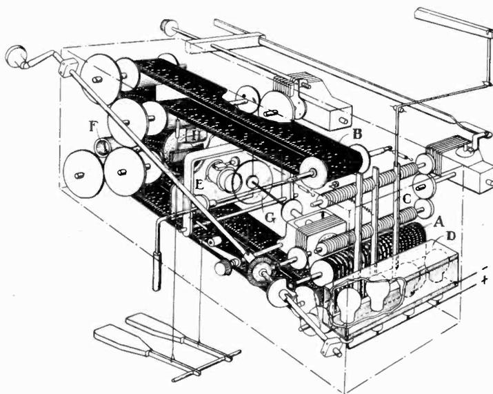
Diagram of one of the units, showing "quality" film *A* and "pitch" film *B*. Photo-cell pickup is at *F*
