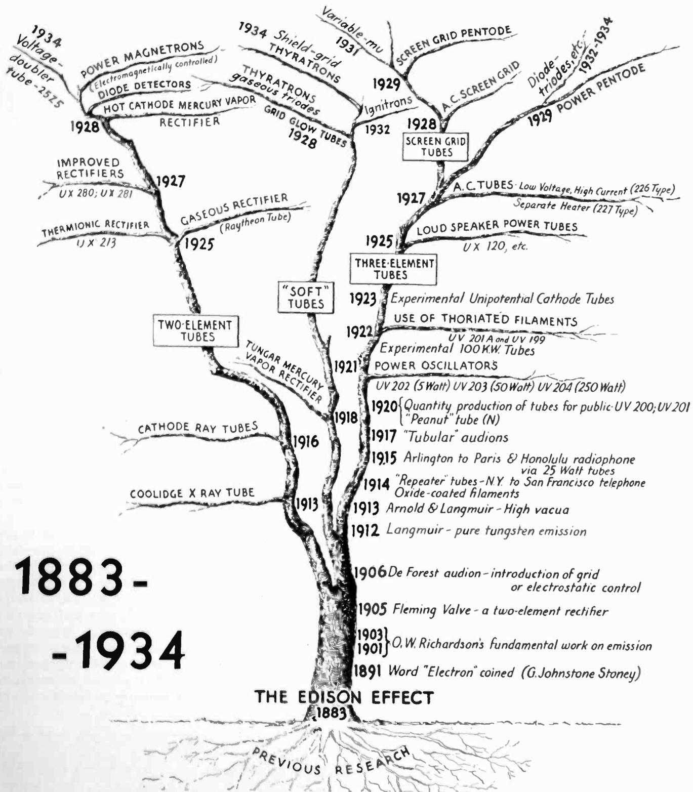
So rapid are the changes in the tube art that the chart showing the Family Tree of the Thermionic Tube, first published in Electronics, May, 1930, is out of date. Therefore, recent additions have been made showing the new branches to this fast-growing tree. Such tubes as the variable-mu, voltage-doubler, the many combinations of triodes and diodes and pentodes were unthought of in 1930—but will be found on the tree above.
