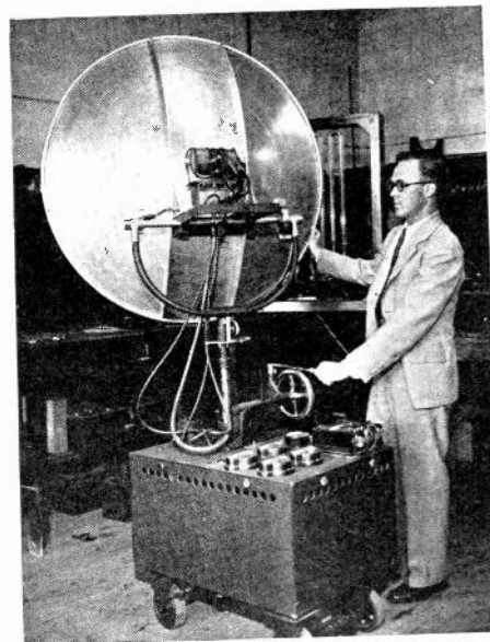
Dr. Irving Wolff demonstrates the artificial Heaviside layer (ionic tube shown at left of reflector) which modulates the four-inch waves produced by the transmitter.
