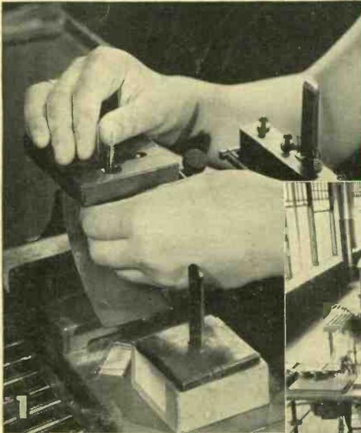
(1) Gauging grids. This operation is typical of the scores of painstaking measurements and tests conducted in the Parts Assembly Section. (2) A view of the General Assembly Section. Here the mounts are assembled before being
