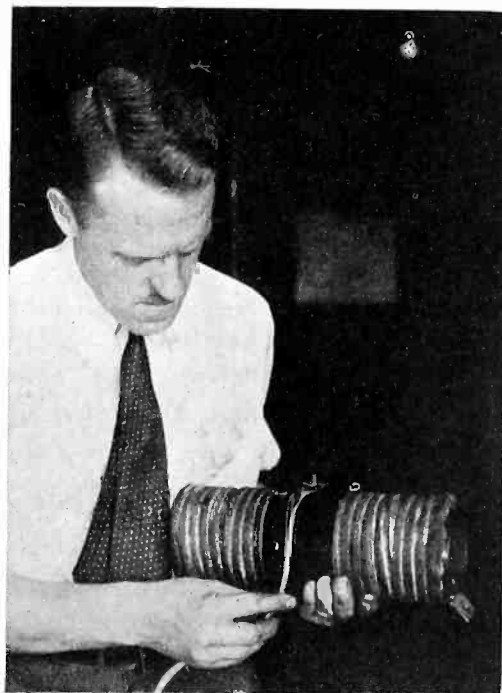
Copper strap twisted into a cylinder by the action of a radio frequency current, shown by W. G. Roman of the Westinghouse high voltage laboratories
