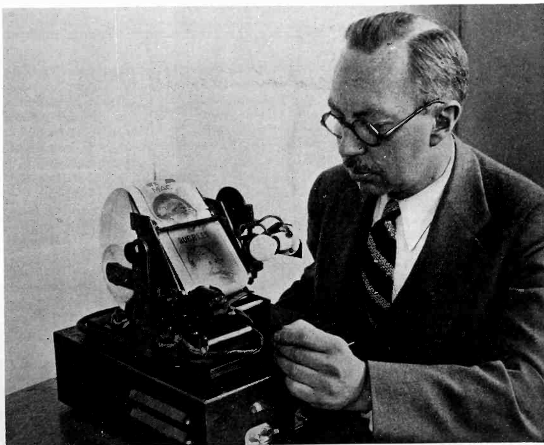
John V. L. Hogan of New York, and his "radio pen." The fountain stylus, carrying ink, draws lines rapidly across the paper
