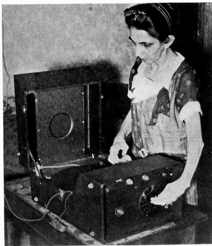
In this new combination radio-phonograph "talking book" developed by the American Foundation for the Blind, Grand Central Palace, New York City, the dial markings are in raised Braille characters. Long-playing records of standard books and popular novels are now available in libraries for the blind
