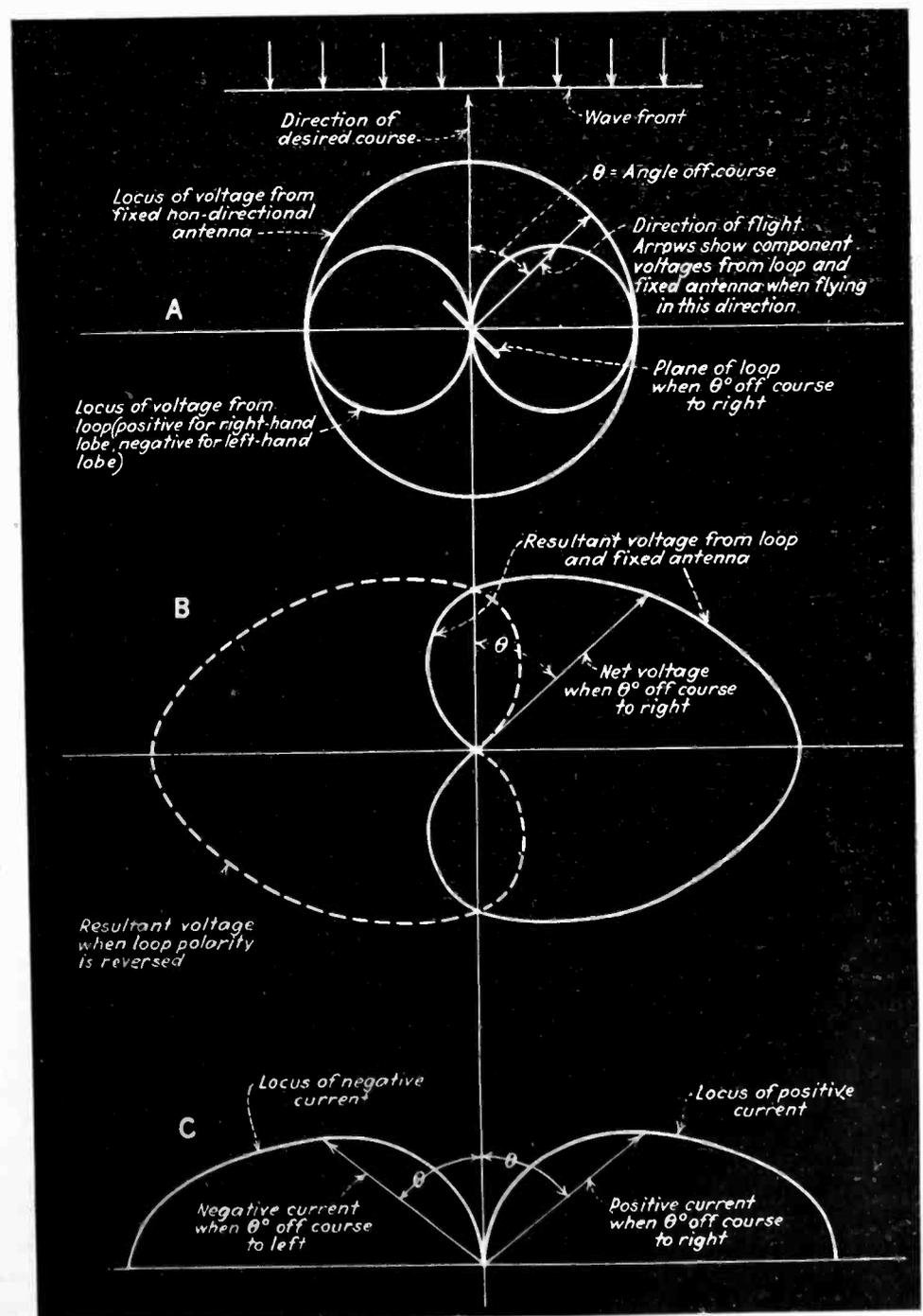
Fig. 2—Right, diagram showing transformation of loop-bearing into a right or left meter indication.
