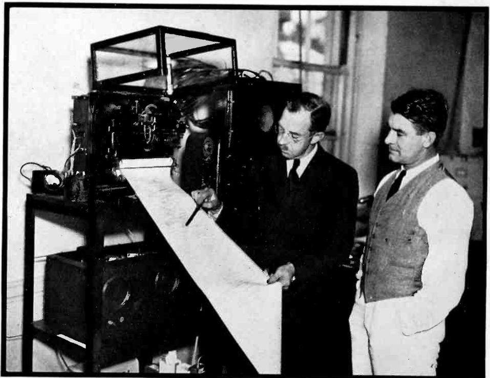
Dr. Harlan Stetson, and Thomas S. McCaleb of Harvard with an automatic signal-strength recorder. The record indicates that the moon as well as the sun causes changes in ionization of the upper atmosphere
