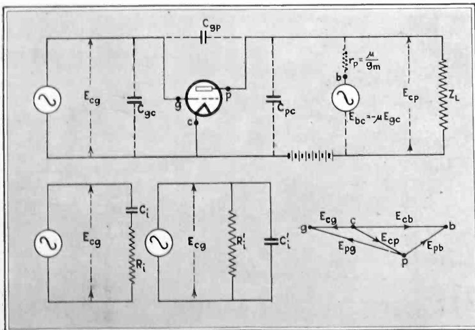
Circuit for making use of controlled input capacity
