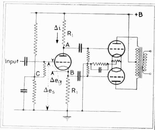
Mr. Richter's circuit for coupling a driver to a push-pull stage by a capacity-resistance network
