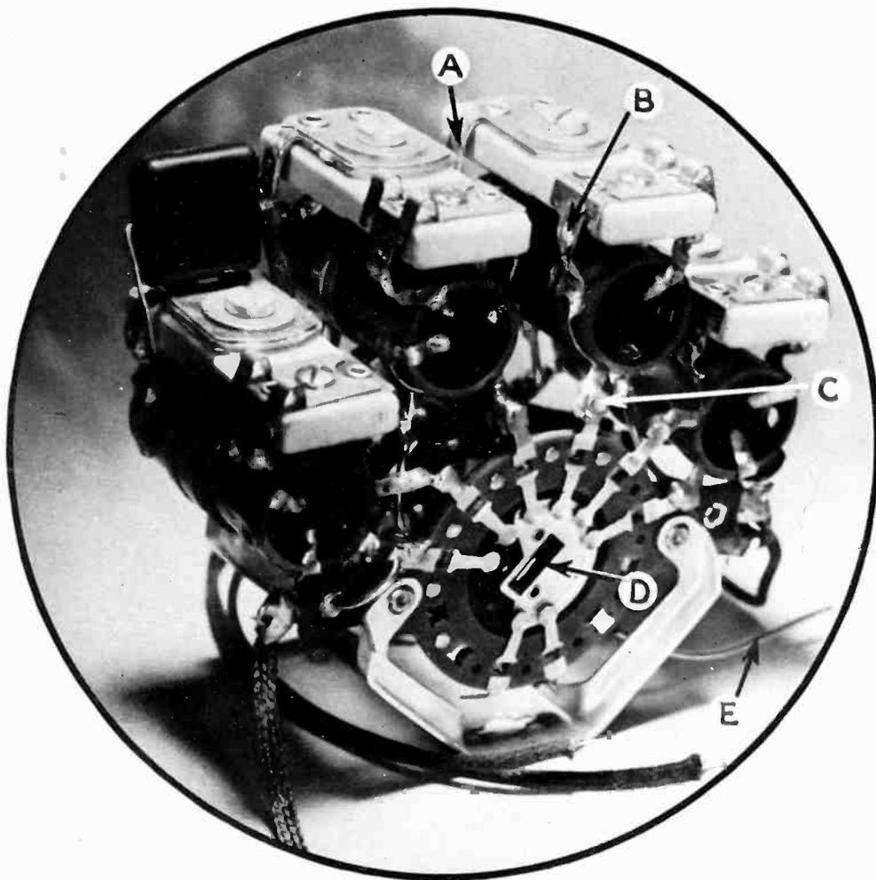
*Oscillator section. A. Isolantite base. B. Condenser supported on coil by solder lugs. C. Coils supported by solder lugs. D. Rectangular opening for actuating shaft. E. Bus to stator, braided to rotor of gang condenser; insulated wire to sockets and power supply*
