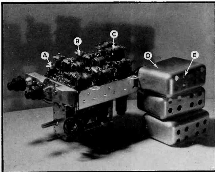
*Bottom view with interstage shields removed. A. Antenna section. B. R-F section. C. Oscillator section. D. Shields. E. Holes through which alignment is effected when shields are in place*
