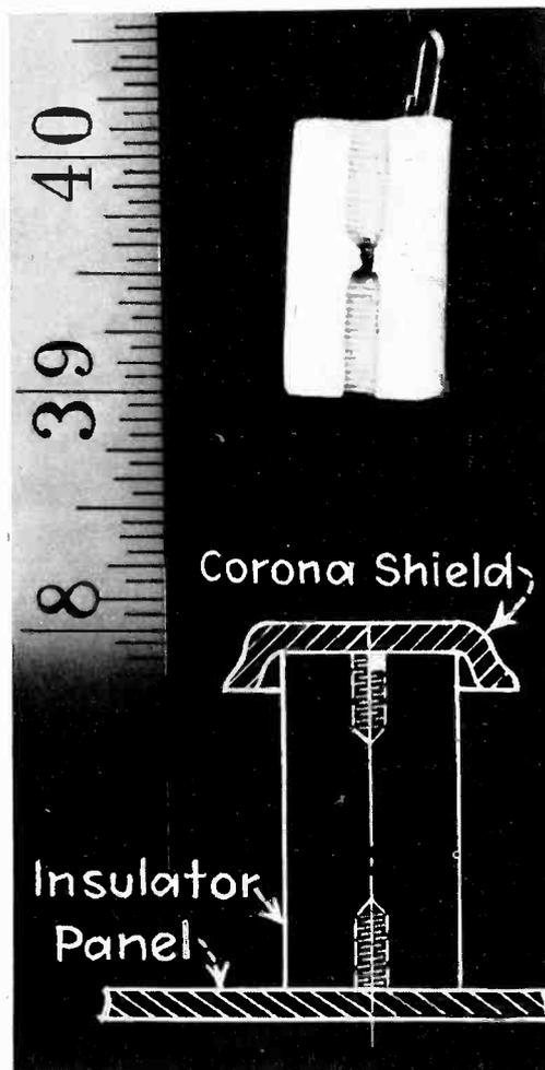
Fig. 1—Below, outline of typical insulator. Above, insulator after breakdown (actual size).
