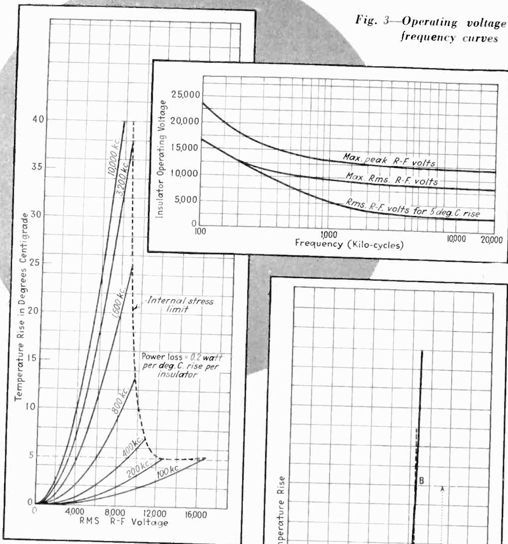
Fig. 2—Insulator voltage—temperature rise curves and limits
