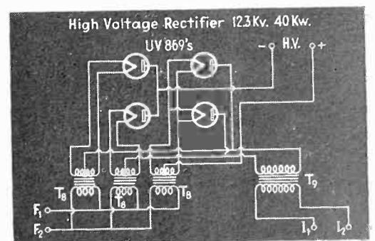
High voltage power supply for h-f generator
