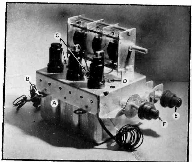
*Unit without dial. A. Interstage shields. B. Lugs with soft rubber shock-proof bushings. C. Extruded dowels for alignment. D. Bus connection from coil and switch. E. Tuning knob. F. Wavelength change switch*
