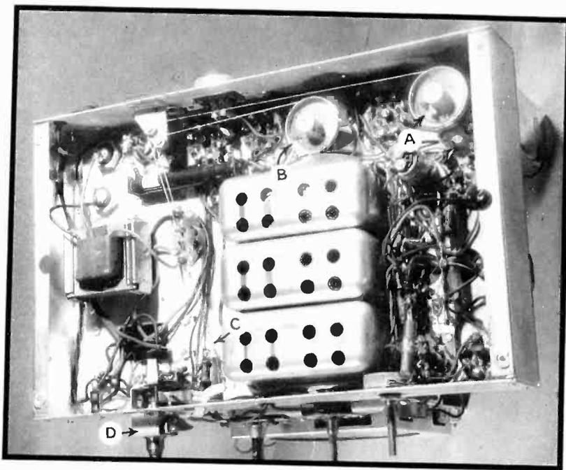
*Bottom view, Bosch Model 595. A. Spiral spring coupled between pulleys and frame of transformers exerts a force in a direction to wind up the cords. B. Pulleys are on the shaft of the rotating coils of the variable selectivity i-f transformers. C. Cords. D. Cam and lever mechanism for changing bandwidth*
