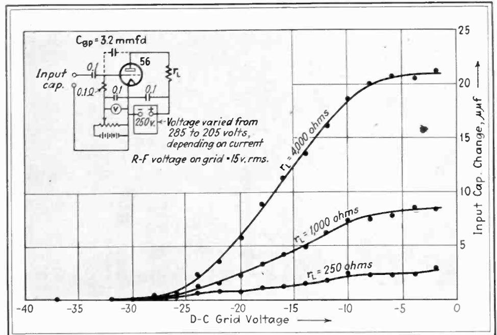
Extent of capacity change secured from use of a standard triode as control tube
