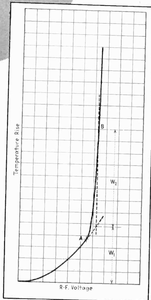
Fig. 4—Typical\* temperature rise plotted against r-f voltage
