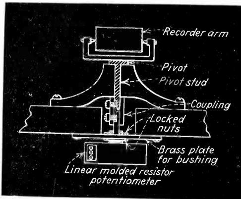
Mechanical coupling of recorder arm to resistor
