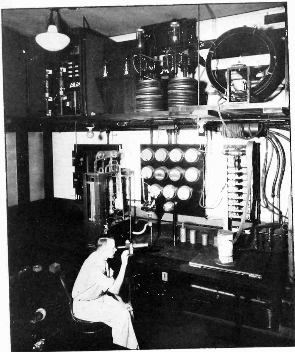
The high frequency generator used to heat a charge in a crucible, in the Westinghouse Laboratories. The output transformer is shown at the upper right, with the amplifier tubes to the left
