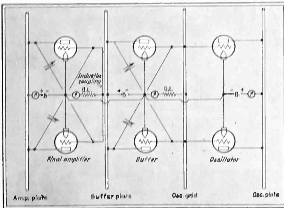
Each vertical bar in the electrical diagram above represents the resonant-line unfolded, i.e., the center of each is the shorting bar. The neutralizing condensers connect directly from plate to grid in each case.
