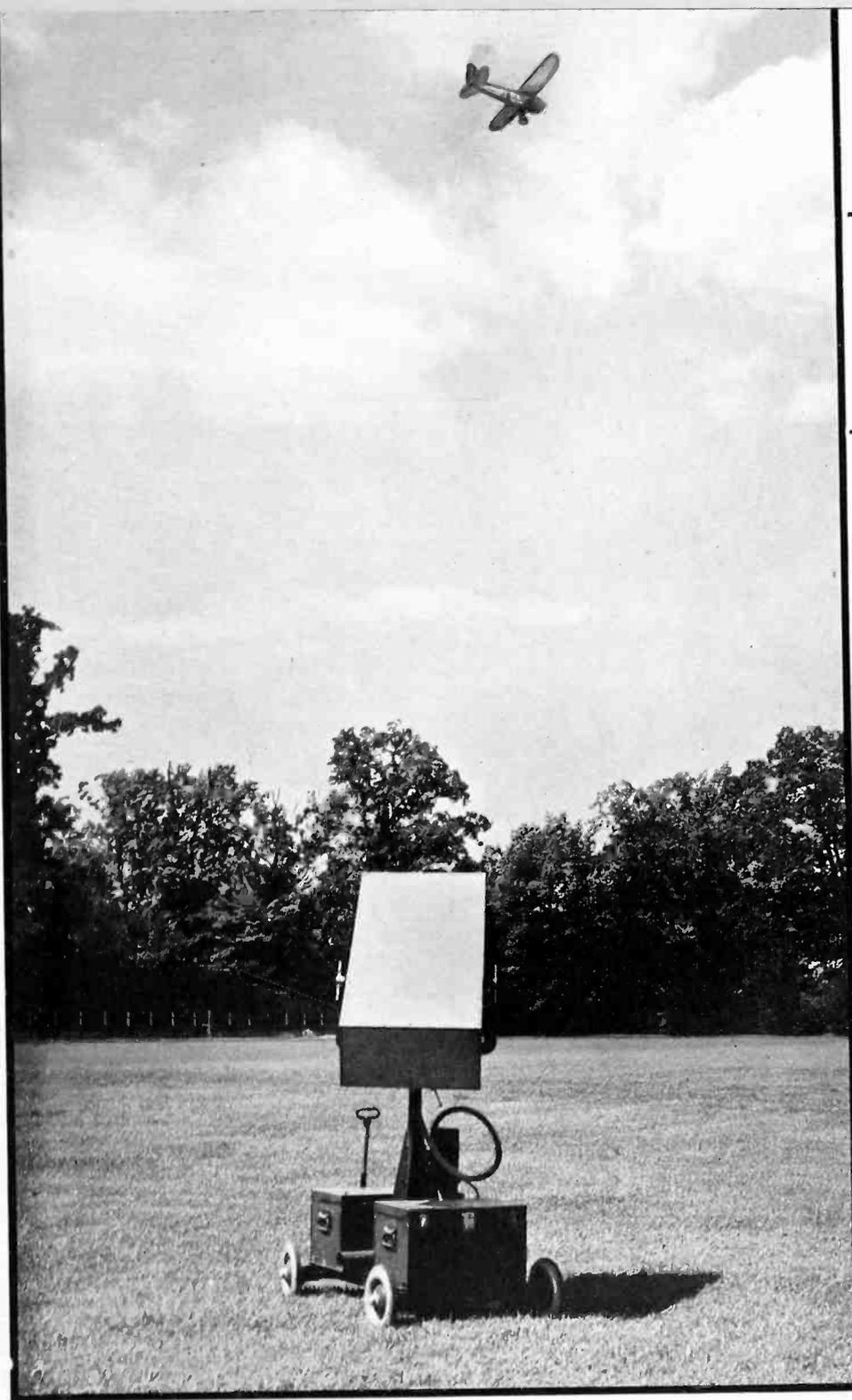
*Exposure made when a bell rung by the Petoscope indicated it had picked up the aircraft*
