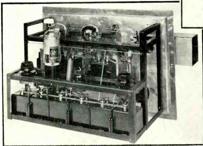
*Interior of an intermediate amplifier showing low loss construction and the use of a neon stabilizing device. The amplifier boxes are double screened and sound proof*
