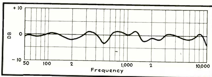
Output characteristics measured on normal axis 10 feet from horn
