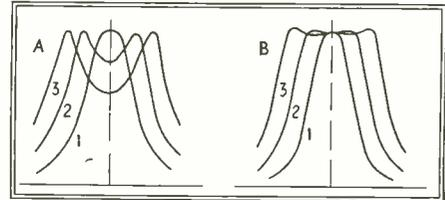
(A) Typical band-pass response curves showing humps produced by increasing coupling
