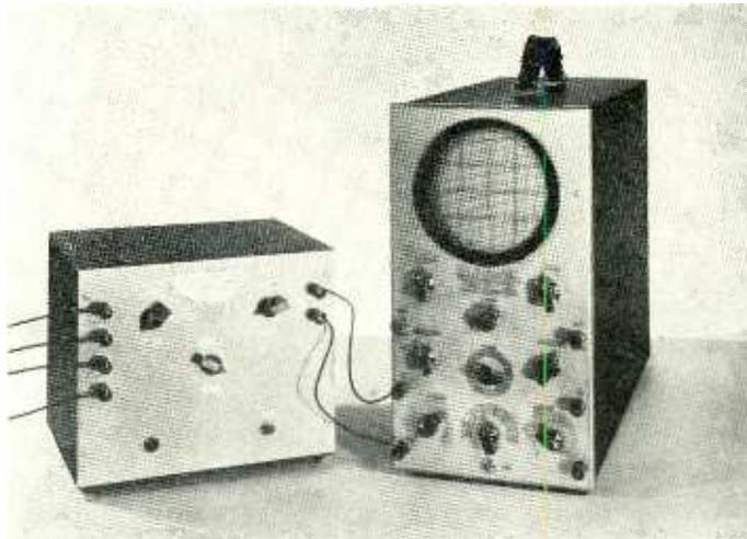
Another feature, contributing to outstanding performance is an *Improved Synchronizing Circuit* permitting locking sweep with fractions as well as multiples of wave.
