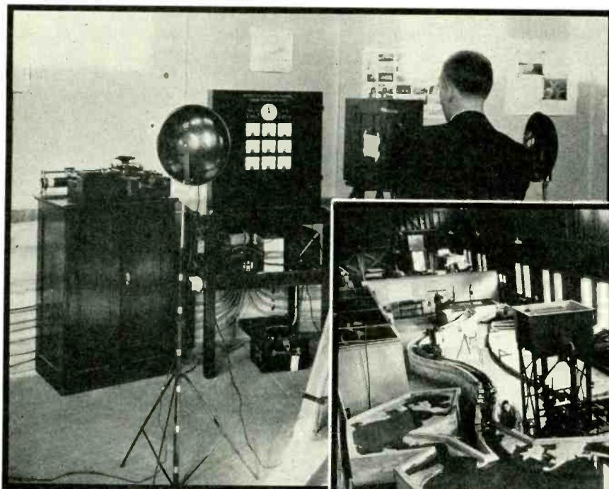
This scale model (right) is used in the Hydraulics Laboratory of M. I. T. to study the currents in a proposed widened and deepened form of the canal. Meters (above) connected to electronic depth-indicators supervise the water levels at important points, while a motion picture camera makes a permanent record of their movements
