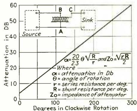
To accomplish this attenuation a variable ladder network consisting of a series element on which the contact rides, and which has a shunt element connected to it along its entire length, is used.
