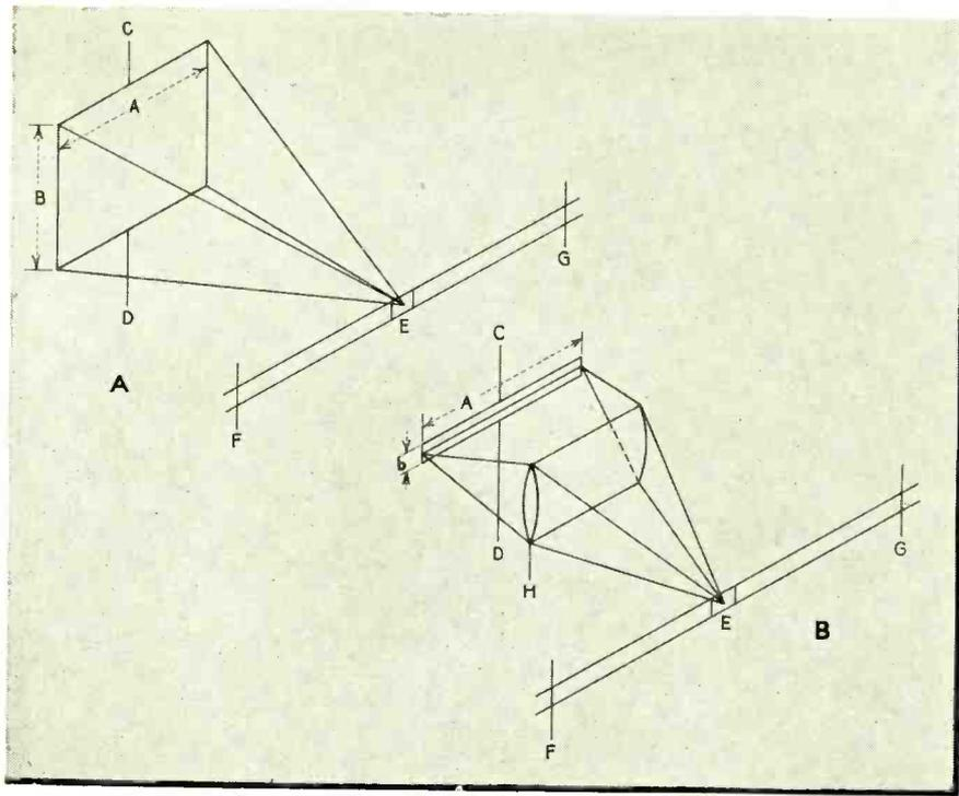
Fig. 2—Illustrating the advantage of split-focus system in reducing scanner dimensions, or increasing illumination
