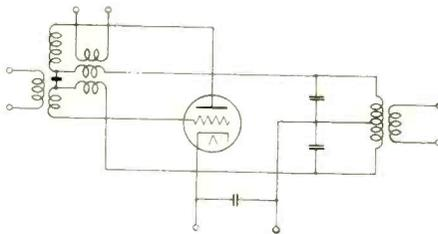
Fig. 8. Circuit with deflection tube similar to a conventional triode
