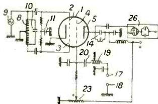
Modulating voltage is applied to an outer or screening grid. Radio Akt.-Ges. No. 435,561.
