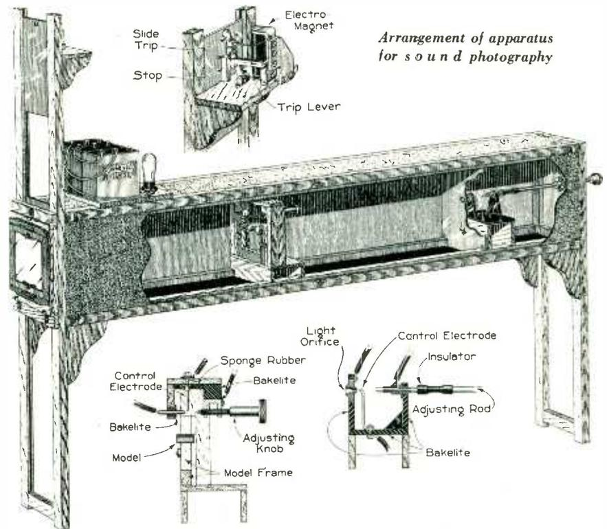
*Arrangement of apparatus for sound photography*
