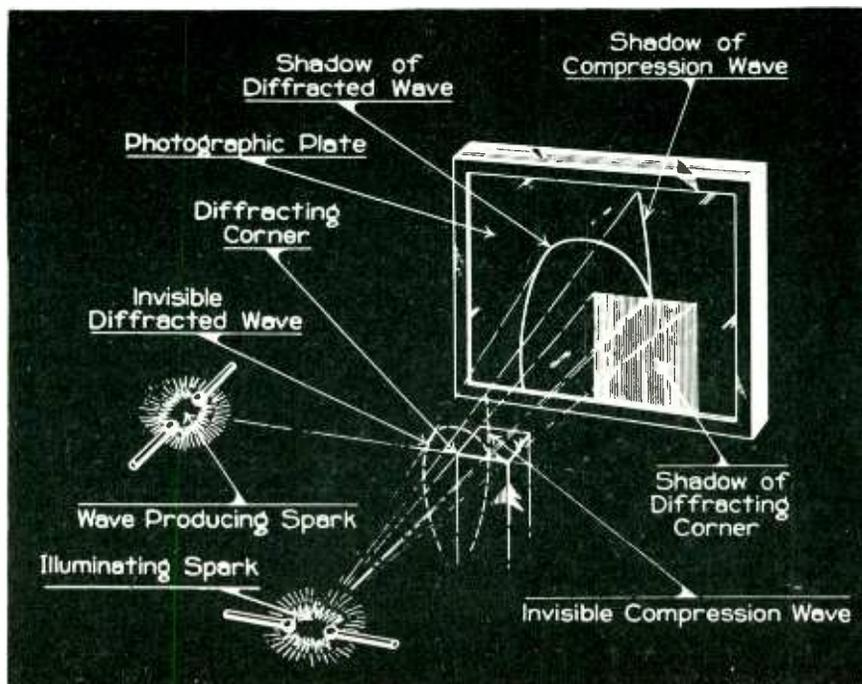
*Timing arrangement used in past for sound wave photography*
