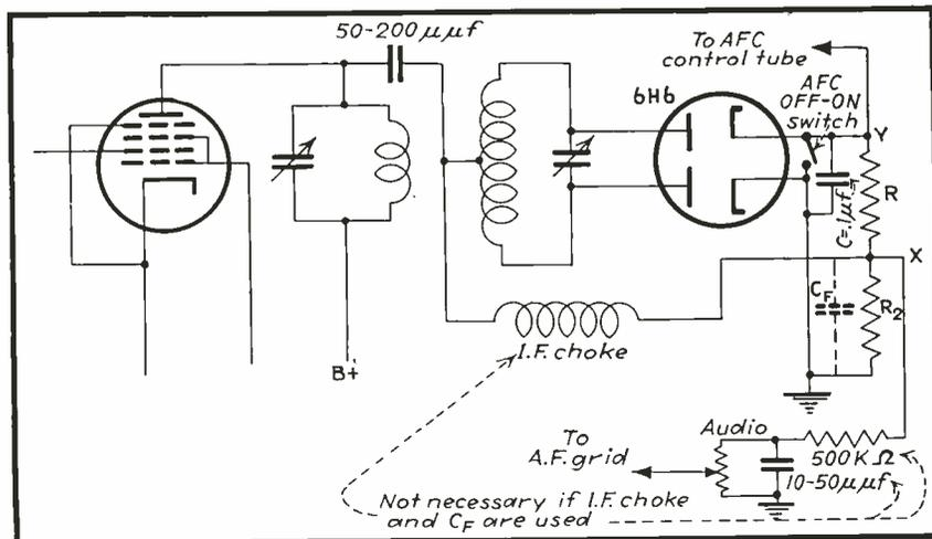
Fig. 1 AFC discriminator circuit which depends on phase difference between primary and secondary i-f transformer voltages
