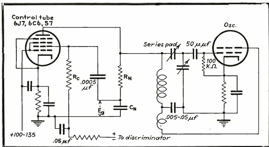
Fig. 6 Simple control circuit using pentagrid converter
