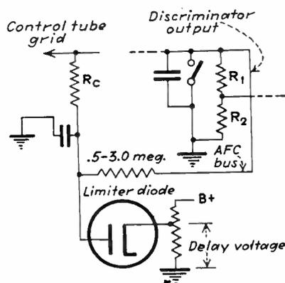
Fig. 7 Delay diode to limit positive voltage to discriminator
