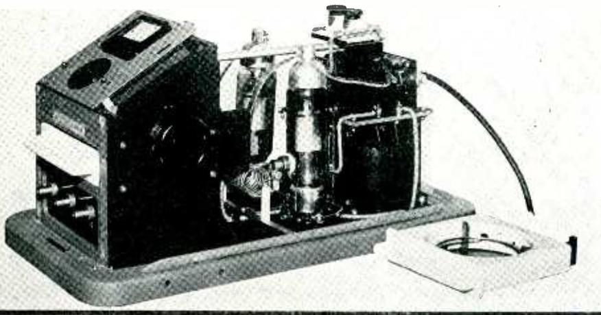
*Above: The interchangeable coils permit operation between 5 and 18 meters. The knob on the side of the unit controls output which is measured by the meter. The control just below the meter is a time switch which automatically determines length of treatment. Below: Interior view of half-kilowatt diathermy machine. The power supply is at the right. A portion of the oscillating circuit can be seen to the left of the tubes*
