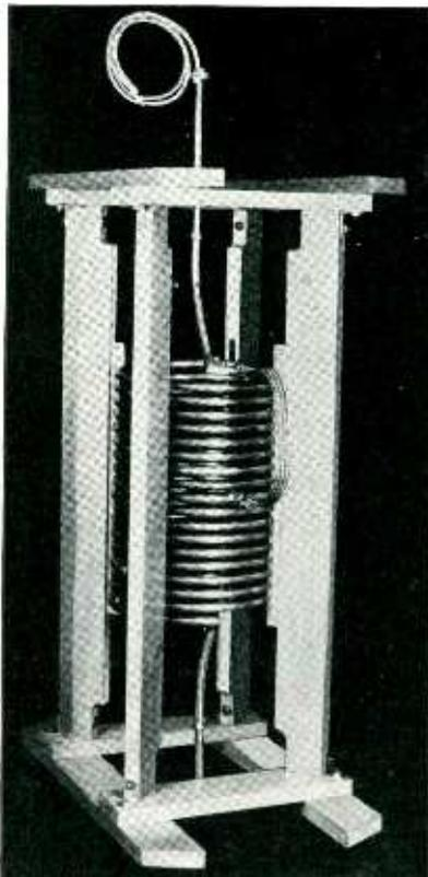
Antenna loading inductor, with tower lighting wires drawn through tubing. Mycalex insulated, mounted in a large weatherproof copper can.
