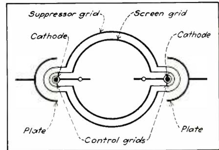
Section through the middle of the push-pull pentodes
