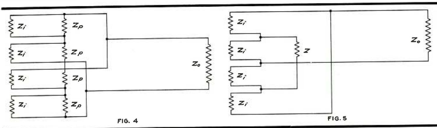
Fig. 1—Simple series type of mixer; Fig. 2—Series-parallel mixer circuit; Fig. 3—Compensated mixer arrangement; Fig. 4—A second compensated type of circuit; Fig. 5—Circuit with added series resistance
