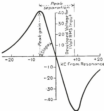
Fig. 2 Resonance curve for Fig. 1; loose coupling between primary and secondary
