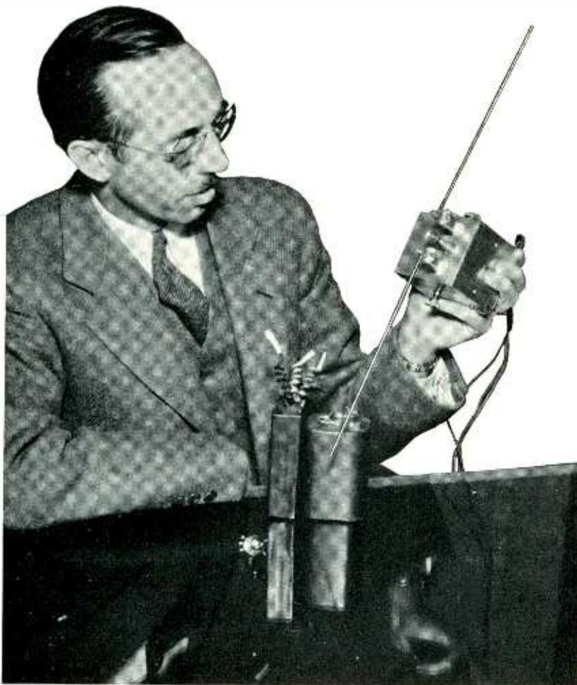
*Chief Engineer: O. B. Hanson with the miniature micro-wave transmitter (0.2 watt, 1 meter) produced by the Development Group*
