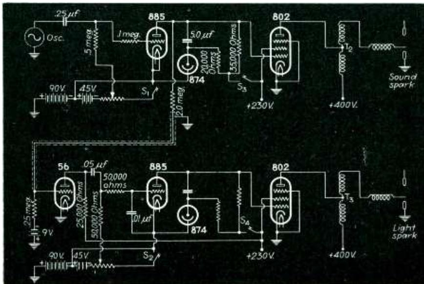
New timing circuit for sound wave photography
