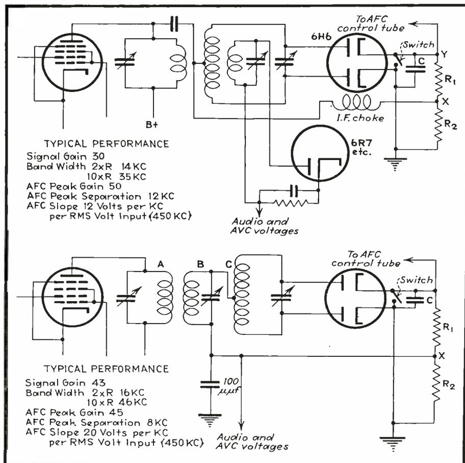
Fig. 4 & 5 Discriminator circuits with improved selectivity. The circuit of Fig. 5 (below) permits smooth operation over wide frequency band
