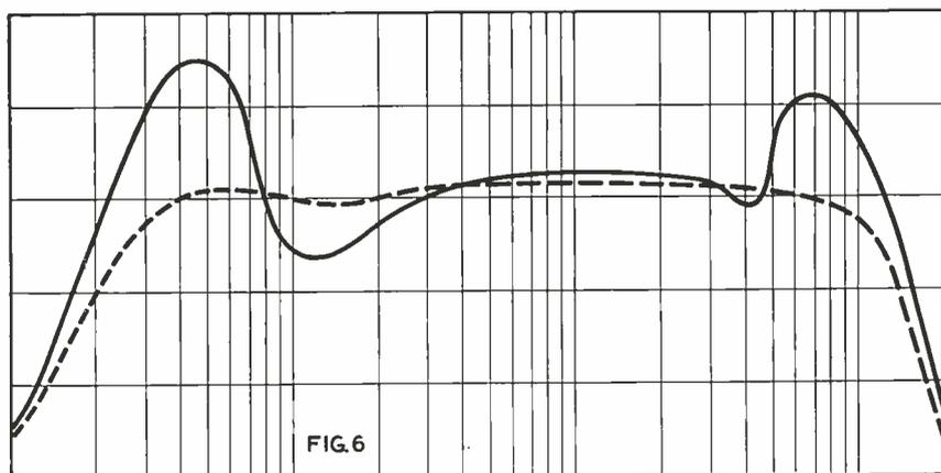
Fig. 6—Response of microphone with complex internal impedance (full line curve) and response (broken line curve) of same microphone and transformers with impedance adjusting pad between transformers and primaries in parallel
