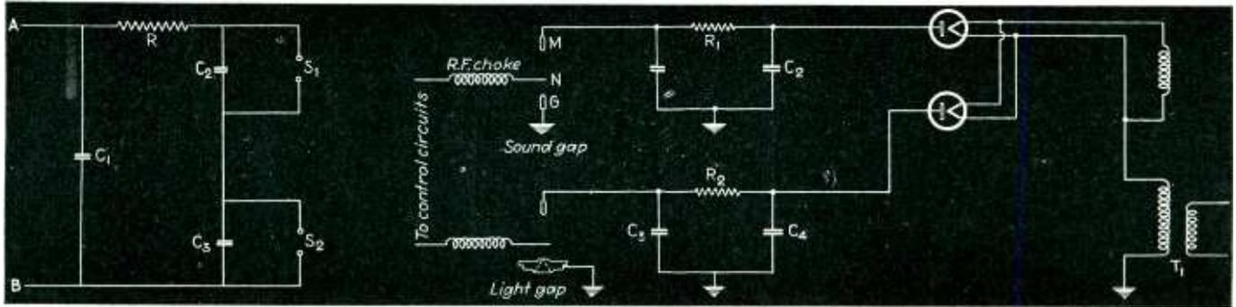
Fig. 1—Timing circuit used in the past. Fig. 2—New spark gap circuits and high voltage source
