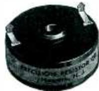
Type M: 1 Watt; Accuracy 1%. Resistance Range .05 to 500,000 ohms. Size: 1" dia., x 1/2" high.
