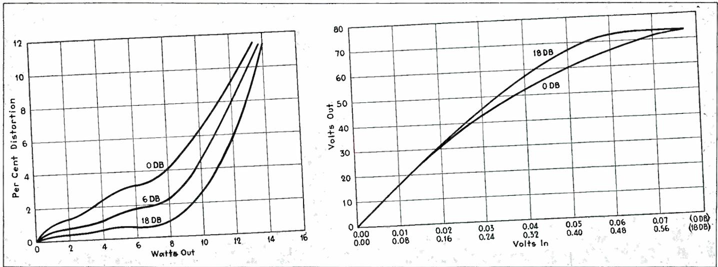
Figs. 12 and 13—Distortion and overload characteristics of the amplifier shown in Fig. 10. At 8 watts output, the distortion is halved by 6 db feedback, reduced below one per cent with 18 db feedback
