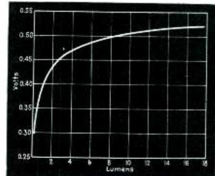
Fig. 3—Voltage output vs. illumination, high levels
