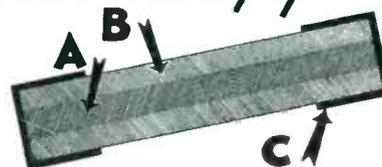
**A.** Center core of resistance material is surrounded by a dense shock-proof ceramic, providing strength and protection against humidity.
