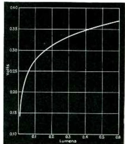
Fig. 4—Voltage output at low light levels
