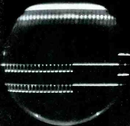
(4) Odd and even framing pedestals and sync impulses
