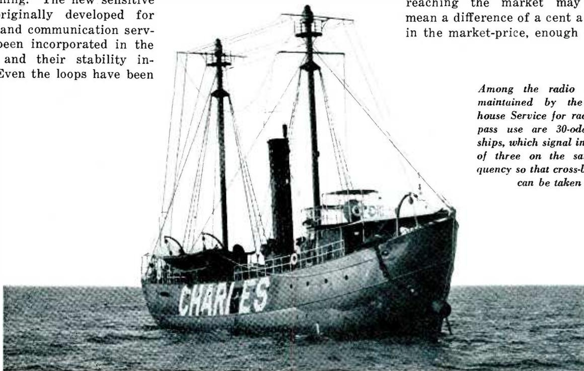
*Among the radio beacons maintained by the Lighthouse Service for radio-compass use are 30-odd lightships, which signal in groups of three on the same frequency so that cross-bearings can be taken*
