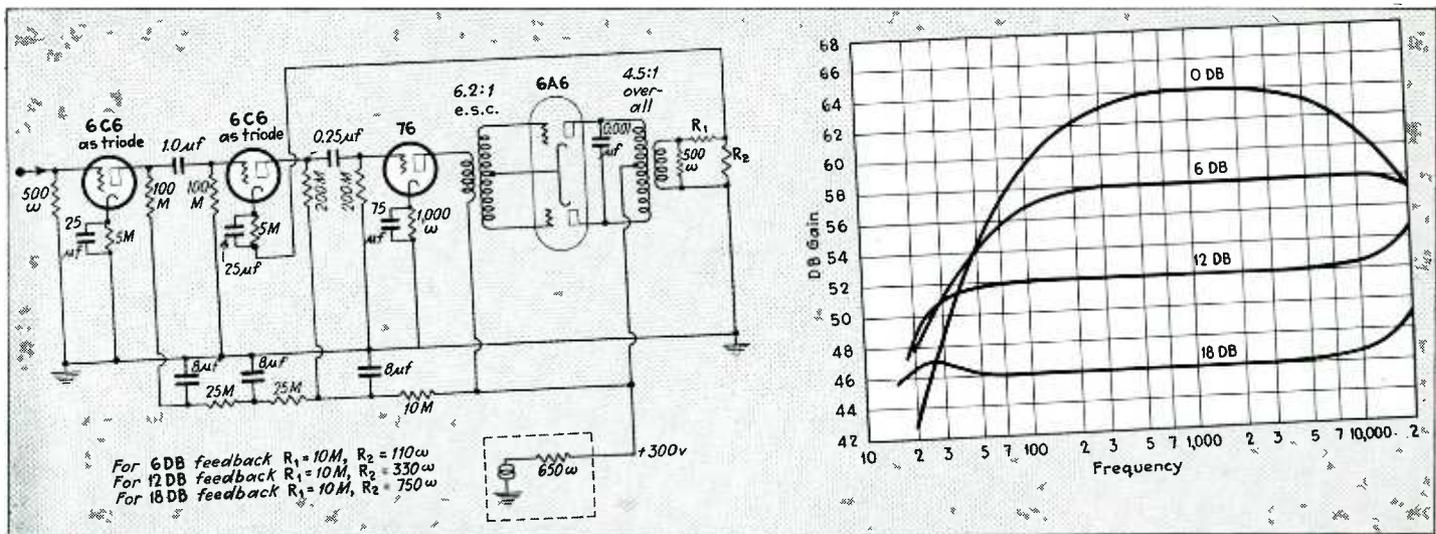
Figs. 10 and 11—A push-pull Class-B unit using a 6A6 double triode, with feedback applied over three stages. The measured frequency response (right) improves greatly as the feedback is increased
