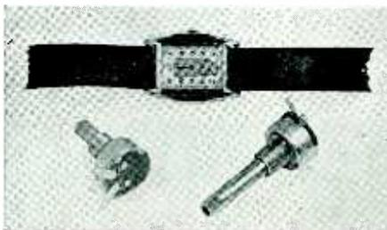
radio manufacturers who require a tone control with hollow shaft for installation in remote control. The volume control shaft passes through the unit and concentric knobs are used for volume and tone control. The sub-midget is used where resistance curve is not critical; tone and sensitivity controls are its chief application.
