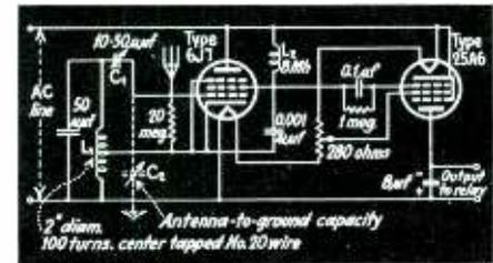
Fig. 2—Relay circuit using metal tubes
