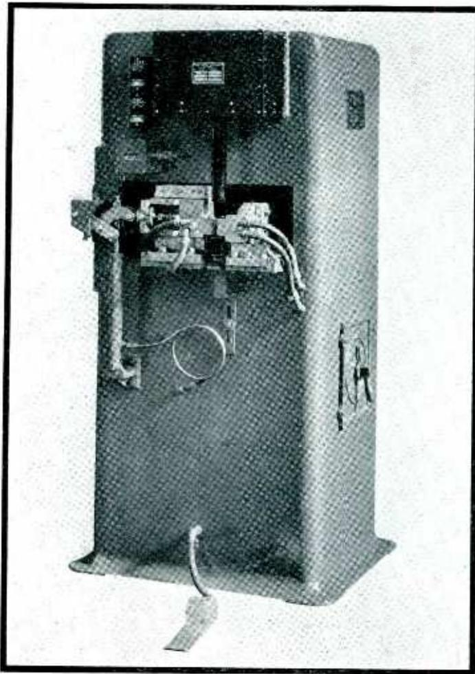
*Early phototube temperature control unit for automatic heat treating valve stem tips; combines economy and speed*
