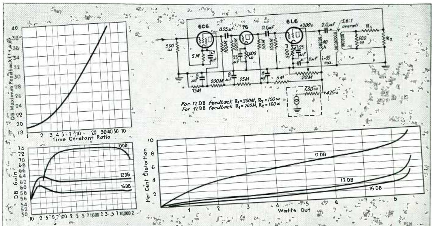
Fig. 1—(upper left) Maximum usable feedback in 3-stage amplifier with resistive feedback and usual coupling circuits. Figs. 2, 3, 4—Single-sided 6L6 unit, its measured frequency response, and single-frequency amplitude distortion vs. output power
