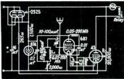
Fig. 1—Voltage-regulated relay circuit
