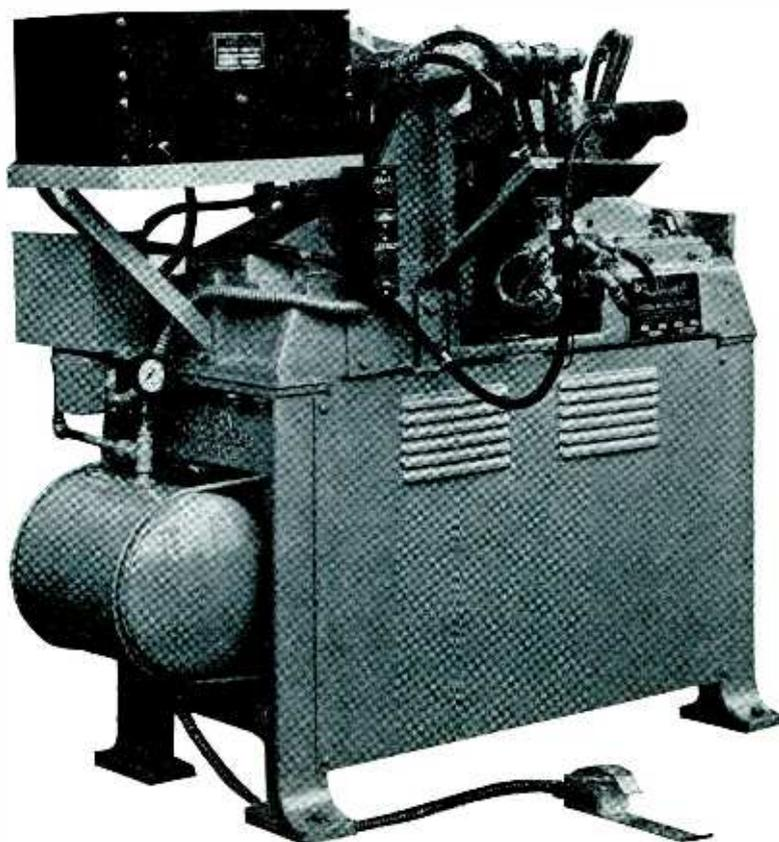
*Heater for annealing central portion of the front axle king pin of automobiles; phototube control connected with amplifier by low capacity cable*
