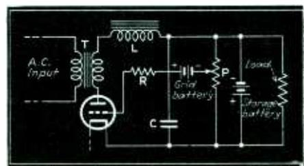
Fig. 1—Wiring circuit of half-wave regulated rectifier
