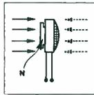
**2.** Discovery of the amazing new "Uni-Phase" principle by Shure Engineers made possible the simplified "Uniplex" uni-directional microphone. It employs only *one* microphone element—achieves *true uni-directivity* through action of acoustic network N. *No other microphone employs this system!\**
