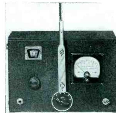
from a single dry cell mounted in the case. A wavechange switch for six bands and a phone jack for monitoring are provided. A damped meter indicates the relative radio frequency field strength.
