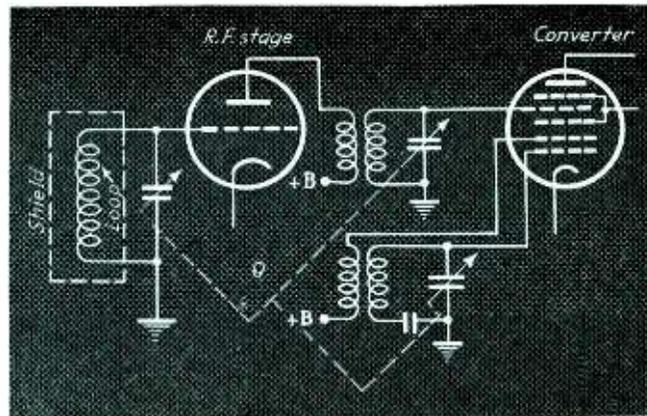
Fig. 5—Schematic wiring diagram of the input circuit for receiver having shielded loop for reducing electrical noise. Condenser tuning the loop is ganged with other tuning condensers.
