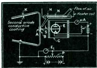
Fig. 1—Circuit showing method of measuring screen potentials of cathode ray tubes
