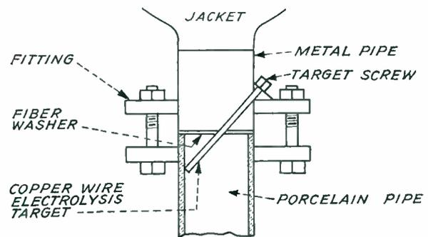
Fig. 5—Drawing showing how targets work
