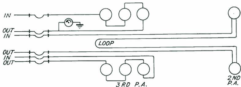
Fig. 6—Diagram of water lines to the different water jackets
