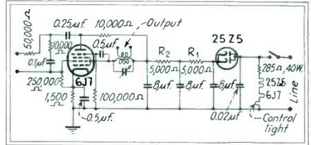
Fig. 2—A-c d-c version of circuit
