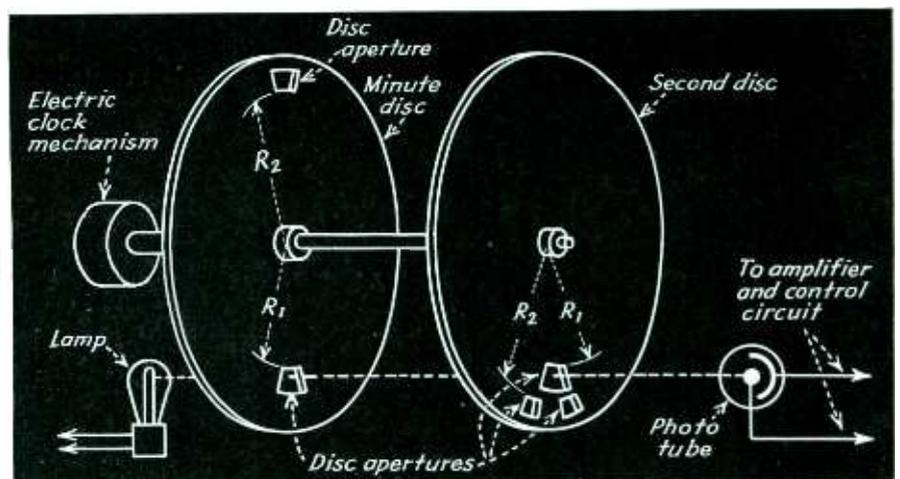
Fig. 1, left — Diagram showing the fundamental mode of operation of clock driven, phototube operated electric timing device
