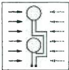
**1.** Previously all uni-directional microphones employed the "Two-Unit Bucking" system requiring two precision-matched elements for true uni-directivity over a wide frequency range. Precision matching is difficult and expensive to attain in practice—involves higher costs.
