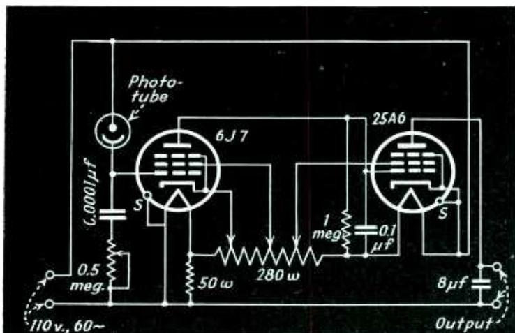
Fig. 3—A simple two stage a-c operated phototube control circuit and amplifier functioning in a negative direction on the received light
