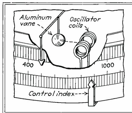
Arrangement of pick-up coils and aluminum vane
