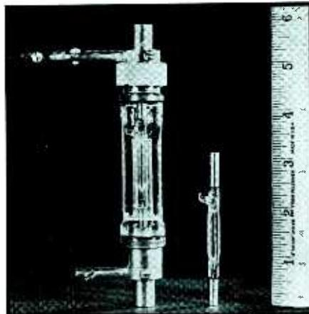
Announced coincidentally by General Electric and Westinghouse, a new 1,000-watt high pressure mercury lamp, shown at right above, is cooled by running water through a jacket surrounding the lamp. The water filters out much of the infrared but allows the ultraviolet and visible radiation to escape. The brilliance attained is about one-fifth that of the sun's surface
