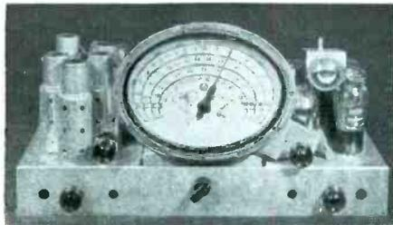
reproduction. A series of amateur tuners covering 10, 20, 40, 80 and 160 meter bands are also available. The tuners are all band switching assemblies with electrical band spread. Full sized wiring diagrams are furnished with the kit.
