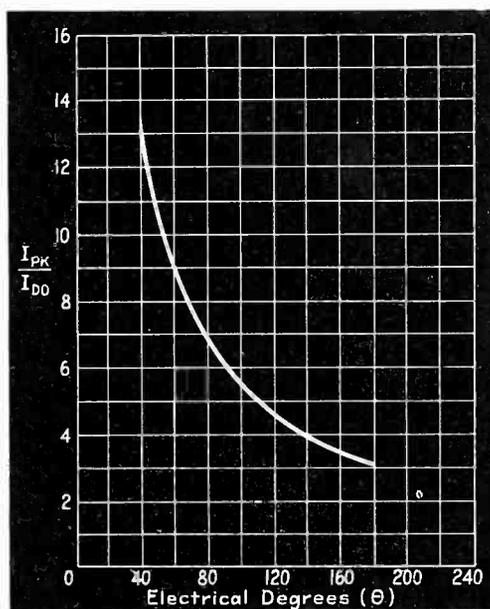
Fig. 4—Relation between peak and averaged d-c components of plate current for Class B or Class C operation
