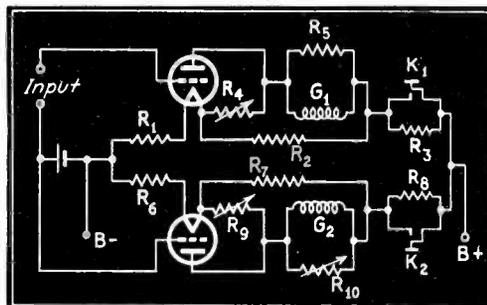
Fig. 1—Schematic wiring diagram of push-pull voltmeter
