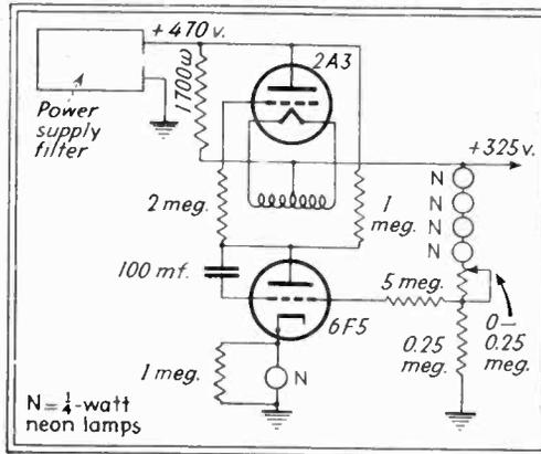
Diagram of voltage regulator based on Bousquet's design
