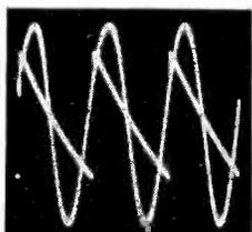
This photograph illustrates the ability of the unit to handle a sawtooth and a sinusoid at the same time and to make them appear as one on the screen of the cathode ray oscillograph.
