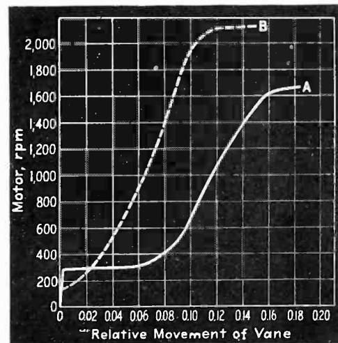
Fig. 5—Relation between motor speed and position of vane interrupting light beam
