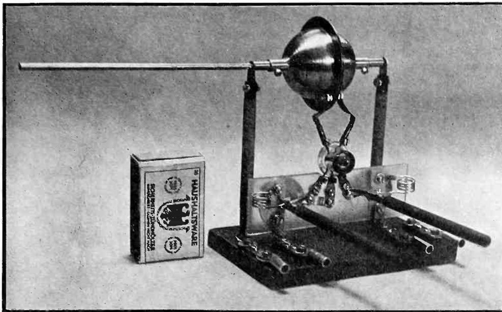
Fig. 3b—Single tube transmitter using an RCA 935 Acorn tube
