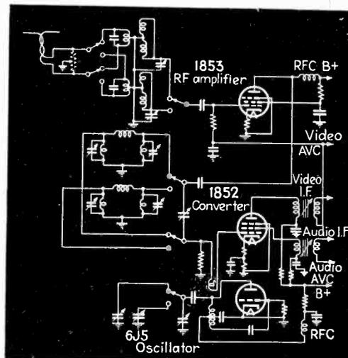
Two channels of the 7-channel television r-f switching system (Lyman)
