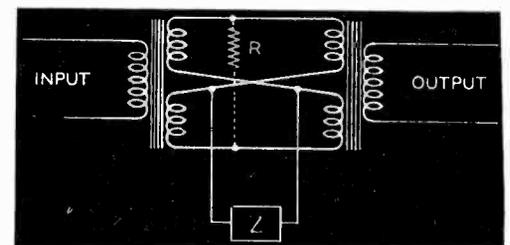
Fig. 3—Adaptation of circuit for distortion measurement
