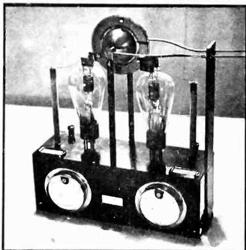
Fig. 8—Push-pull oscillator using RCA 834 tubes
