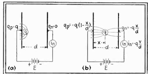
Fig. 1—Diagram illustrating flow of current in tubes operated at high frequencies
