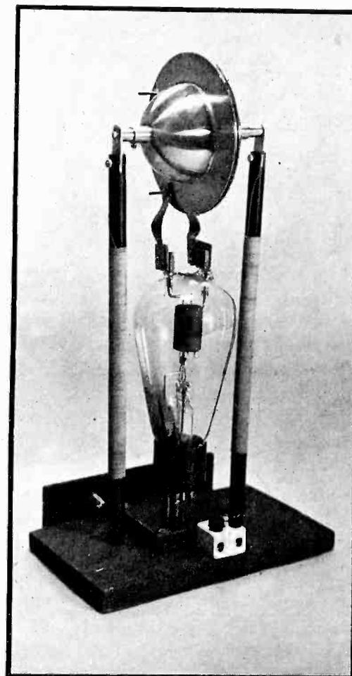
Fig. 3a—Single tube transmitter with RCA 834
