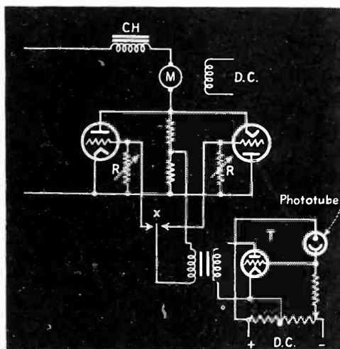
Fig. 4—Use of phototube to control value of inductance for speed control using circuit of Fig. 2
