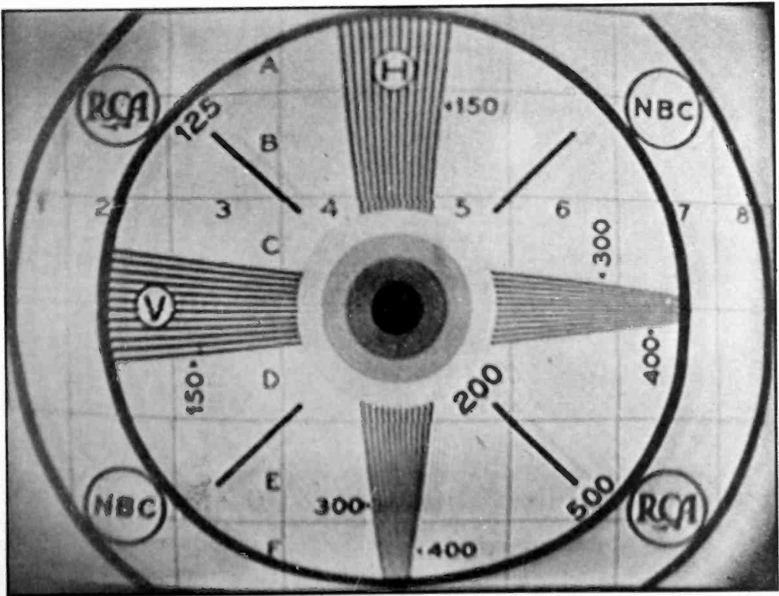
Fig. 2—Image of test pattern, actual size, as received from Empire State transmitter using complete receiver shown in Fig. 1
