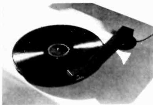
point velocity from 30 to 10,000 cycles without distortion. Low needle point impedance and light weight (6 to 30 grams) on a record permit 500 playings without damage to the record.
