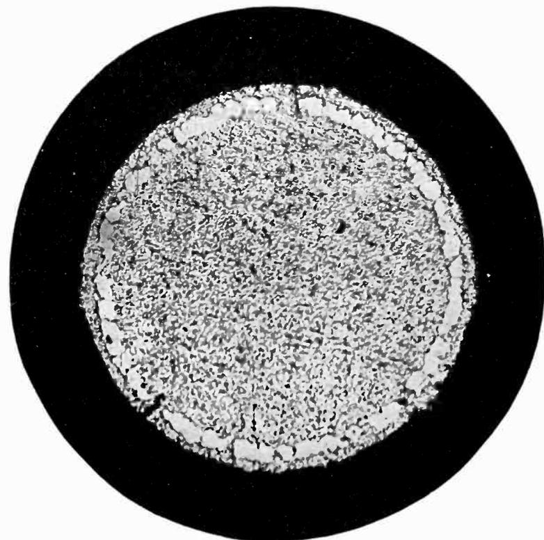
Fig. 2—Cross sectional diagram of carburized thoriated tungsten filament which has been partly decarburized. Magnification, approximately 300X
