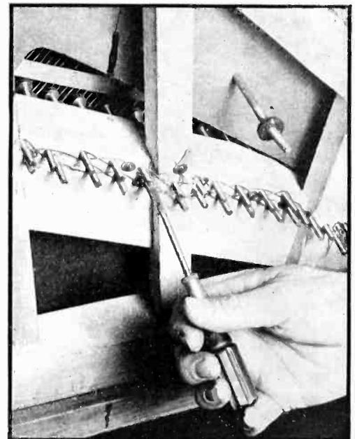
This piano is built without a sounding-board, but contains electrostatic pickup electrodes (above) near each string. The amplified output is applied to a speaker behind the louvers under the keyboard. The instrument contains also, at either side, an all-wave radio and a phonograph
