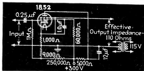
Impedance transformer circuit employing high  $g_m$  tube
