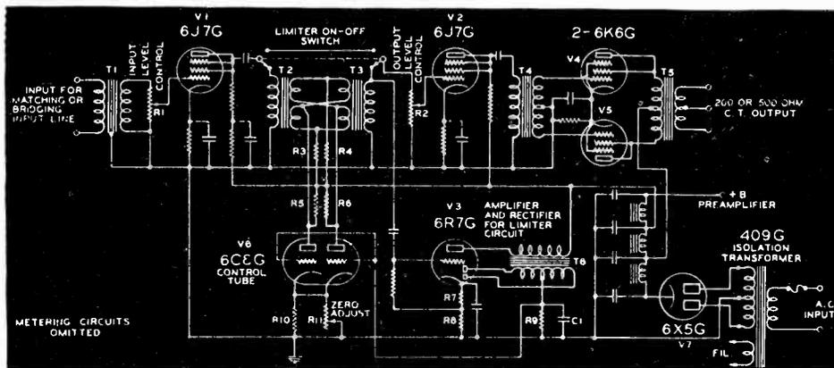
Fig. 1—Circuit diagram of program amplifier with automatic gain control
