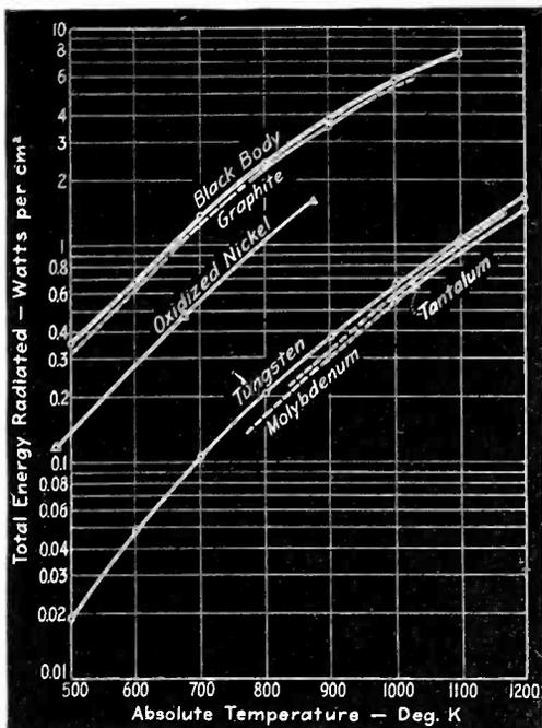
Fig. 3—Characteristics of suitable anode materials for electron power tubes
