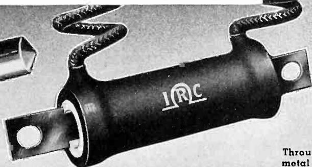
This standard 20-watt wire wound has insulated leads applied during processing, also special brackets, thus eliminating soldering and mounting on the production line.
