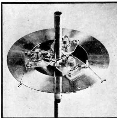
Fig. 5—Transmitter with three internal Acorn tubes. Above, (a) the internal arrangement. Right, (b) the external view
