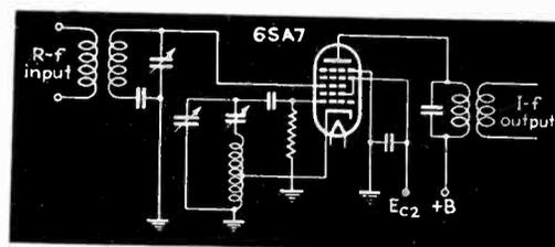
Oscillator circuit for use with the 6SA7; no oscillator anode terminal is required
