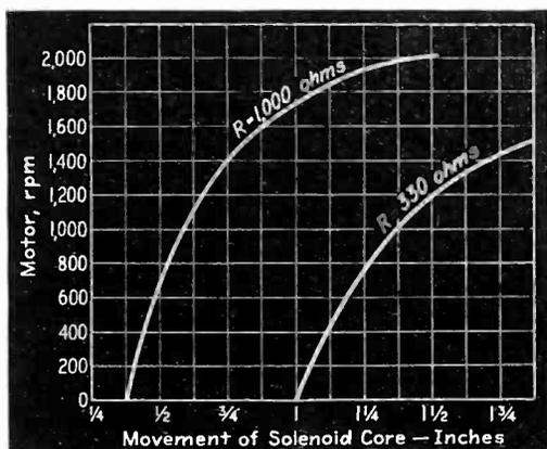
Fig. 3—Speed curves obtained with movable core solenoid and grid resistances shown in Fig. 2
