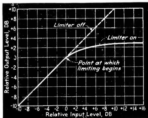
Fig. 2—Input-output characteristics of limiter circuit
