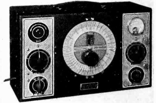
Verni Vider dial. With its accurately calibrated output of 1/2 to 100,000 microvolts at frequencies from 100 kc to 30 Mc, it provides an accurate yardstick of receiver over-all performance.
