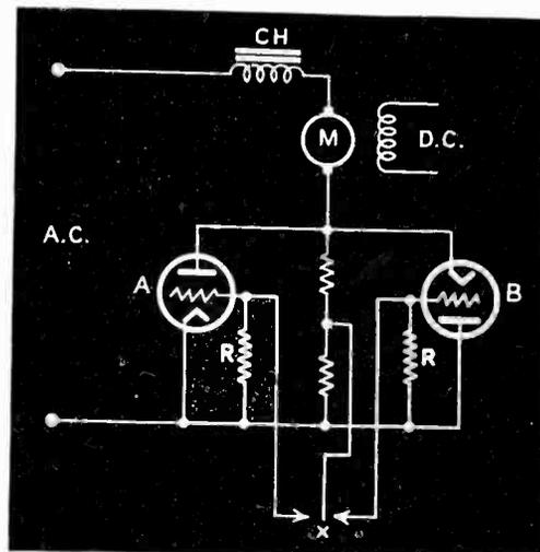
Fig. 1—Circuit for obtaining reversal and speed control of motors from thyratron tubes
