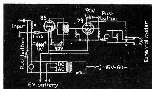
Overvoltage timer circuit useful in noise measurements
