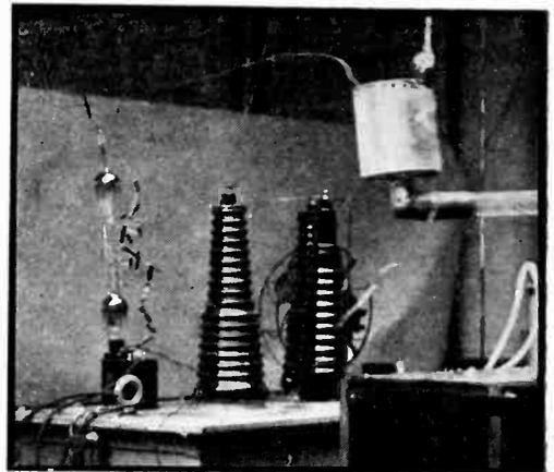
Rectifier (left) in 100 kilovolt set-up
