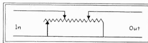
Single-resistor attenuator element
