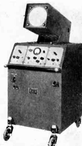
special cathode-ray oscillograph, Model 136-B, makes it possible to examine the wave form of minute impulses and to produce a large image on the tube for photographic purposes.
