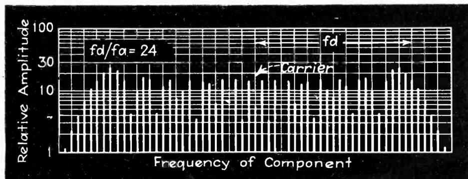
Frequency spectrum of a frequency modulated wave whose deviation frequency is 24 times the audio modulating frequency. Note the low amplitude of the carrier
