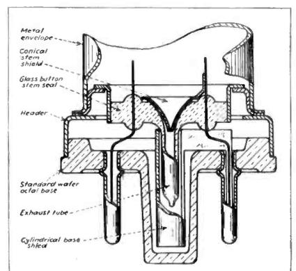
Base construction of the new RCA single-ended Twin Triode Amplifier is shown in this cross-section diagram. It also shows shield cone and cylinders for reducing inter-electrode capacitance.
