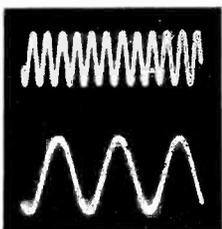
This photograph illustrates a comparison of two harmonically related signals on one oscillograph obtained by using
