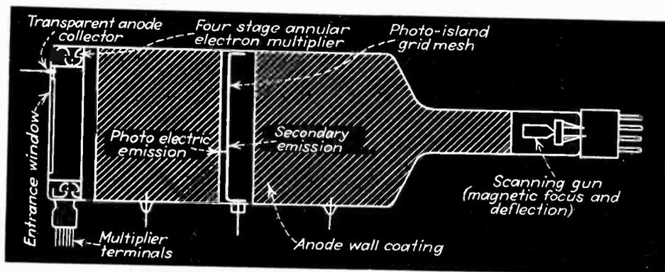
The Farnsworth storage-type image-dissector tube, which displays no shading signal and has ten times the sensitivity of the ordinary iconoscope
