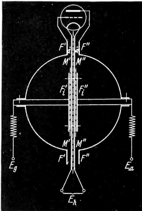
Fig. 6—Schematic circuit of oscillator with external tube
