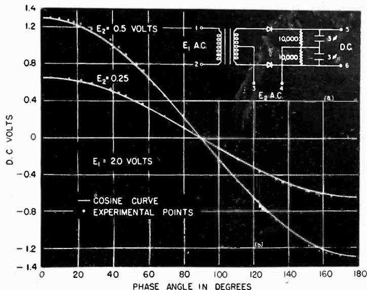
that if the generator  $E_2$  is replaced by a resistance and if a direct potential is applied at the terminals 5 and 6, then a voltage of the frequency of  $E_1$  and having a magnitude directly proportional to the d-c bias will appear across this resistance. Two applications have been published<sup>3</sup> and are shown in Fig. 8. In (a) a direct current amplifier is shown whose stability is essentially that of
