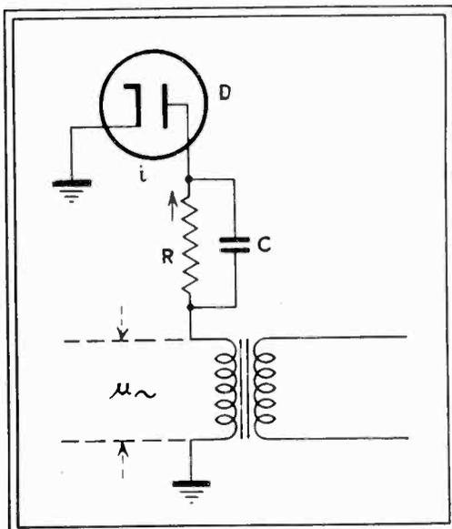
Fig. 1—Schematic wiring diagram of impulse detector
