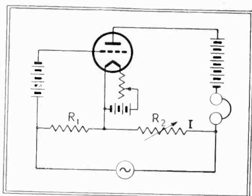
Fig. 1—The conventional measuring circuit
