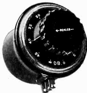
Silver contacts; ball-bearing rotor shaft; clock spring pigtail. Single sliding contact in input circuit results in contact noise being attenuated within the unit in direct proportion to loss introduced in the circuit providing constant noise-to-signal ratio. Impedance practically constant over entire range of pad. Long life; trouble-free service . . . famous Remler quality.
