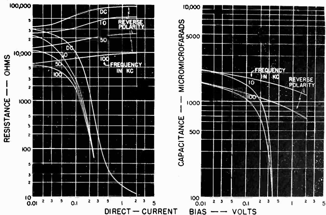
Fig. 2—Small-signal resistance and capacitance vs bias voltage of "Varistor" unit
