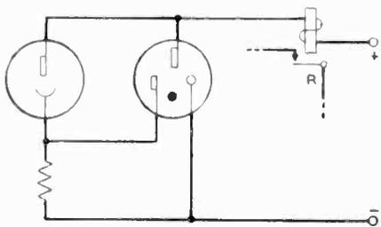
Photoelectric relay circuit using 313C cold cathode tube.
