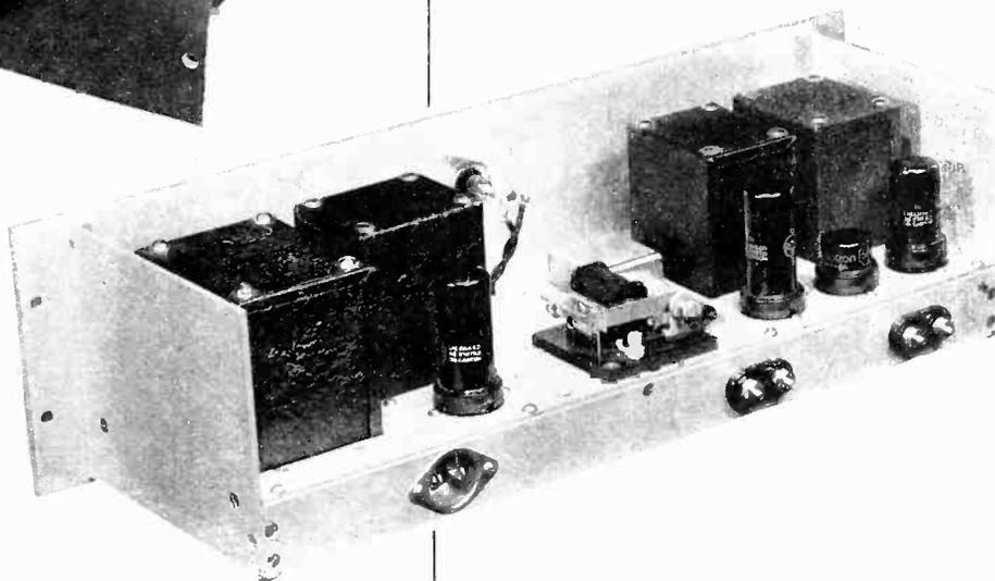
The unit is designed to operate on lines which carry a level of eight vu or higher. It is self-monitoring and a failure within itself will cause an alarm
