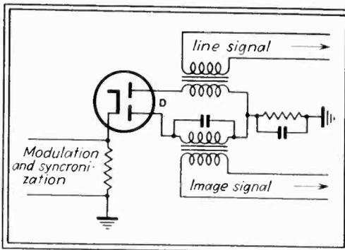
Fig 2—Double diode impulse detector circuit
