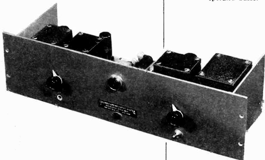
The alarm is given by the large red pilot light in the center of the panel and by a sparkless, a-c operated buzzer
