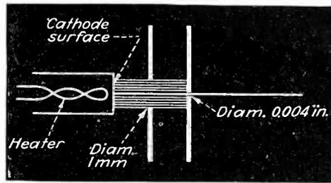
Fig. 7—In the present form of the Orthicon, this very simple electron gun is used
