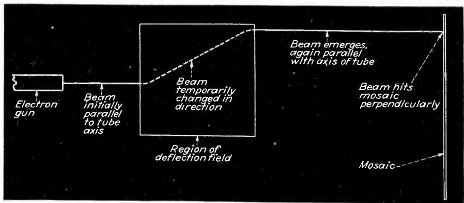
Fig. 4—To preserve the perpendicularity of scanning, the field deflects the beam temporarily. A combination of electric and magnetic forces is employed in the deflection system
