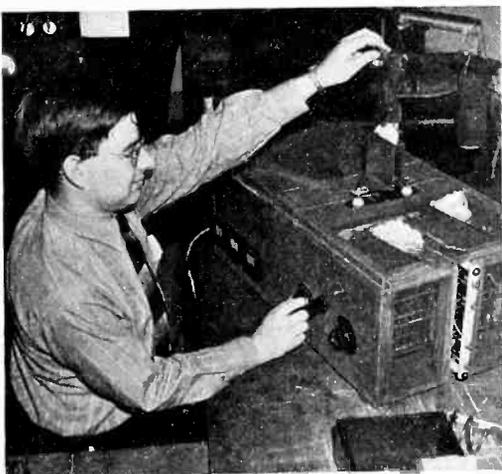
Charles Millikan, graduate engineer at the California Institute of Technology, pops corn in a cellulose bag by using short radio waves. The device operates on the same principle as that employed in diathermy machines, but is rather uneconomical when used solely for corn popping
