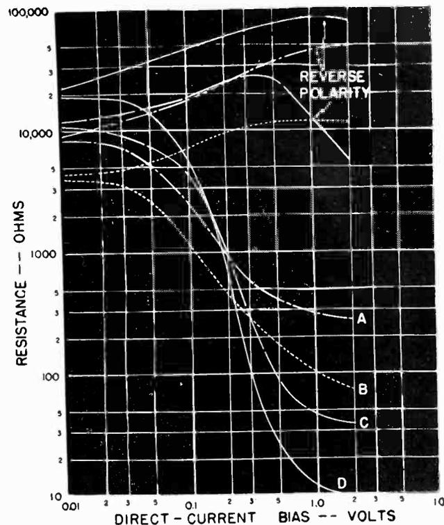
Fig. 1—Static characteristics of CuO rectifiers of four manufacturers
