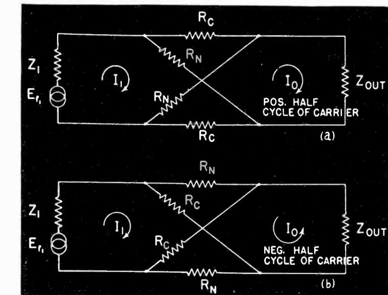
Fig. 12—Equivalent circuits for the ring modulator
