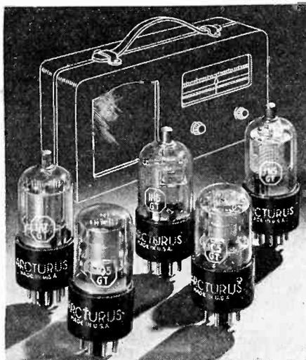
GT, power output pentode; 1A7G and GT, pentagrid converter; 1C5G and GT, power output pentode; 1H5G and GT, diode-triode; 1N5G and GT, r-f pentode; and 1Q5G and GT, beam power output tube. Also announced by Arcturus is a line of eight new dial lights.
