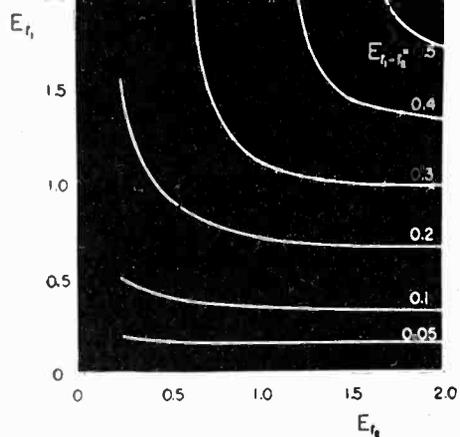
Fig. 11—Voltage levels for two carriers and difference frequency
