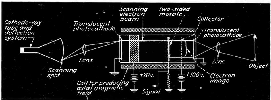
Fig. 6—Another developmental form of the tube used a two-sided mosaic, with image on one side and scanning electrons in the other. The flying spot of light was retained
