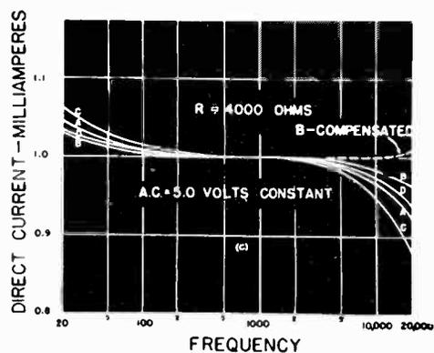
largely dependent on the constants of the transformer and on the time constant of the parallel resistor and condenser. The low frequency droop can be raised by increasing the  $RC$  product, while the high frequency droop can be compensated as before by inserting a parallel resistor and condenser between the points 1 and 2. It is essential that rectifier units having high resistance in the non-conducting direction be chosen in order to keep the  $RC$  constant high.
