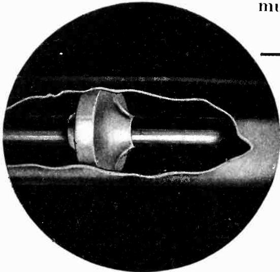
Fig. 1—Section of Isolantite coaxial cable. The shape of the insulator serves to distribute the lines of force uniformly over its surface
