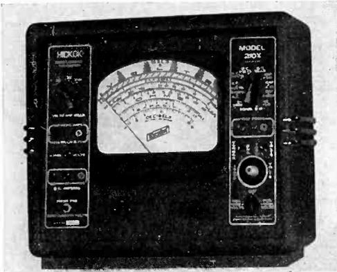
has ranges for measuring up to 10,000 volts. It will also measure currents up to 25 amperes, resistances up to 50 megohms, capacitances to 200 microfarads. A decibel range is included.
