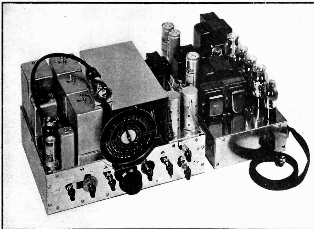
The receiver is contained in two chassis; the r-f and i-f units and first audio stage are in the left chassis and the audio power amplifier and power supply are in the right chassis. All controls and a heater transformer for the tuner tubes are mounted on the tuner chassis
