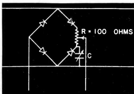
rollers placed on either side of a sheet of moving paper in a paper mill and since a d-c recording galvanometer is connected across the terminals 1-2, variations in paper thickness are recorded continuously as a function of time.
