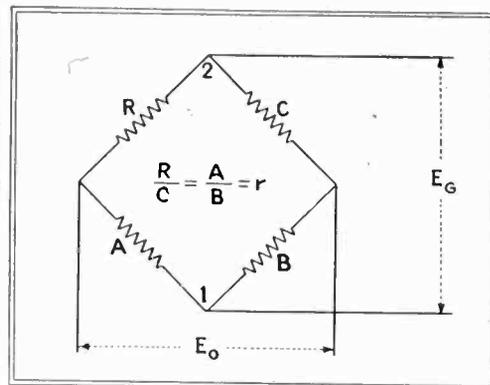
Fig. 1—Basic bridge circuit
