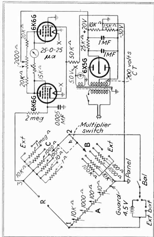
Fig. 2—Complete circuit diagram of bridge
