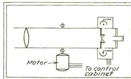
Basic phototube and prism arrangement
