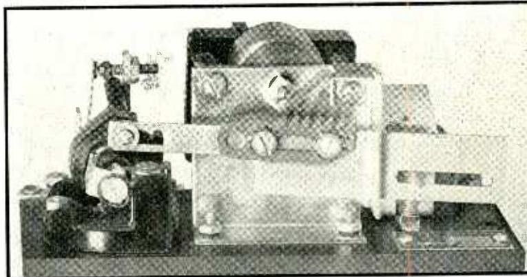
A typical clock-type delay relay, used for cathode protection in large gas-filled tube circuits. The relay introduces a fixed delay of six minutes, then automatically recycles itself ready for the next operation
