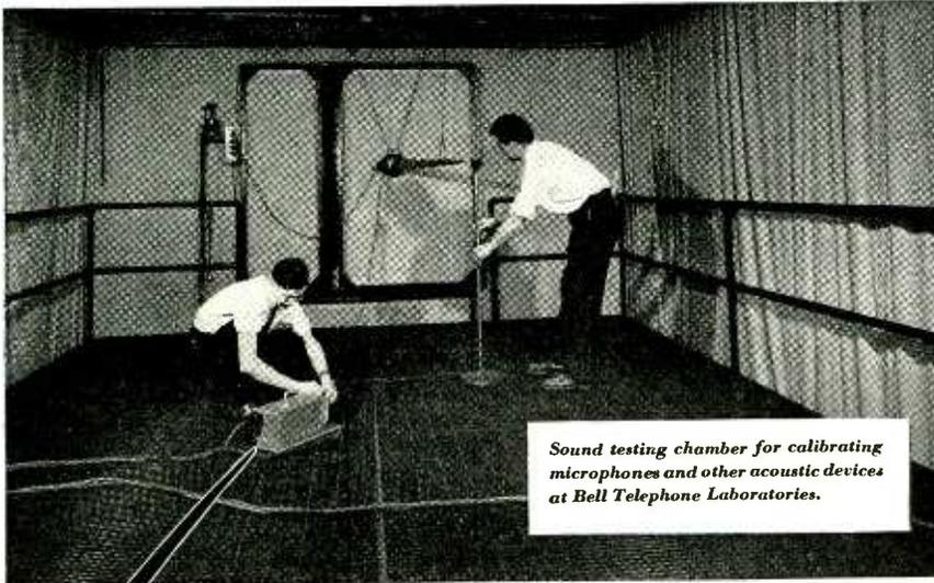
Sound testing chamber for calibrating microphones and other acoustic devices at Bell Telephone Laboratories.
