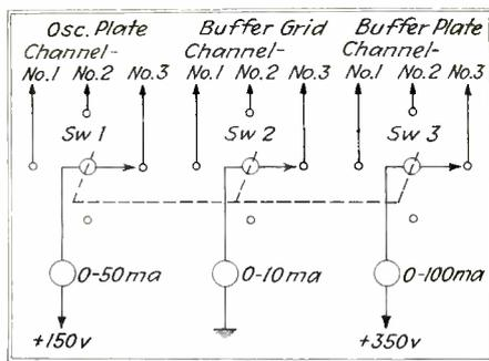
Above, meter switching for the exciter stages. All the switches are ganged
