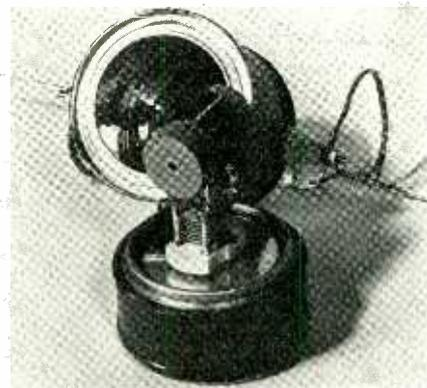
Internal arrangement of suspended circuit
