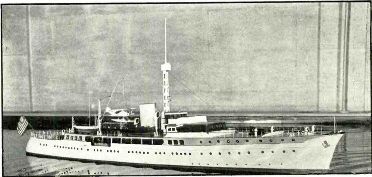
The North Star is a five-foot model of a 240-foot pleasure yacht. It is remotely controlled by means of a radio system and interlocking relays which operate propelling and steering motors
