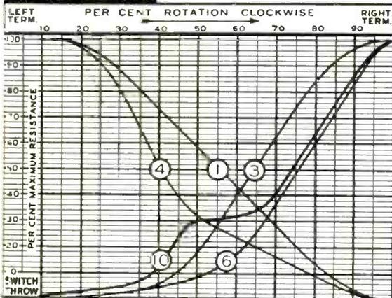
The resistor curve of a volume control is more important than its overall resistance... that is why Centralab controls are furnished with the variety of curves shown here. Curve six is most widely used for high resistance radio grid and diode controls. Curve 1, or 4, are best for C bias, and Curve 3 for antenna C bias. Curve 10 is used on tapped controls.
