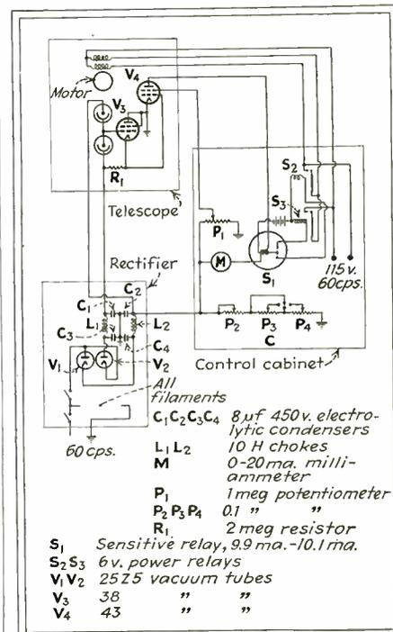
Complete circuit diagram of the telescope control
