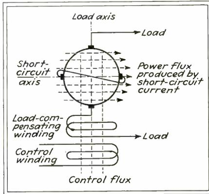
Diagram showing principle of operation of the Amplidyne Generator
