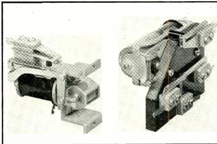
Two unusual constructions in the sensitive relay class: a high speed counting relay, and a relay, designed to have minimum capacitance, for switching the video circuits in a television studio
