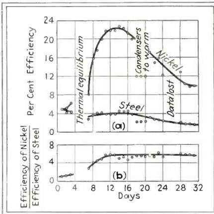
Comparison of nickel and steel condensers over a testing period of 32 days
