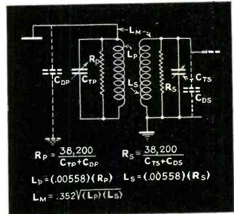
Fig. 6—Design relationships for a wide-band i-f transformer, based on a mid-band frequency of 11.25 Mc, and a bandwidth of 4.2 Mc
