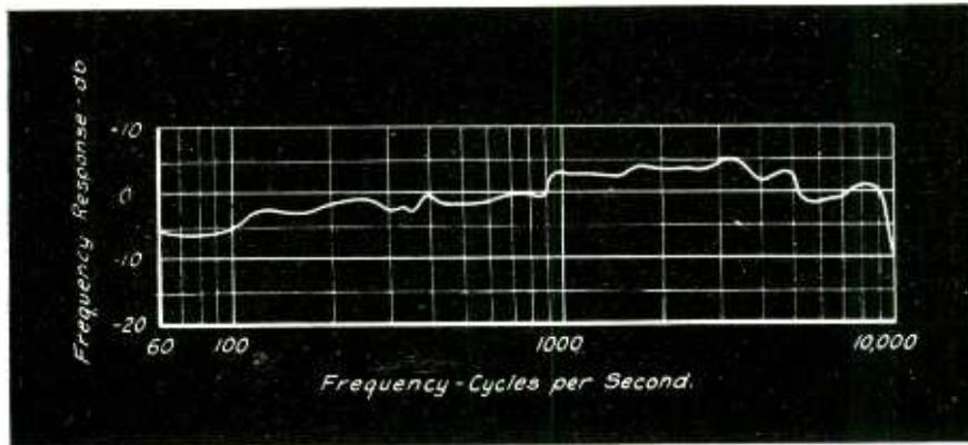
Fig. 8—Frequency response curve of the super-cardioid microphone for an incidence angle of zero degrees and with the microphone one foot from the sound source
