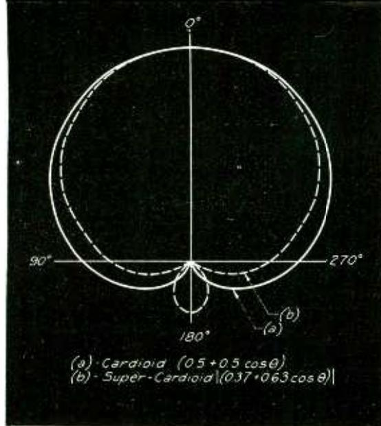
Fig. 1—(Above) Cardioid and super-cardioid directional patterns. Probability calculations indicate that few sounds originate directly in front of the microphone
