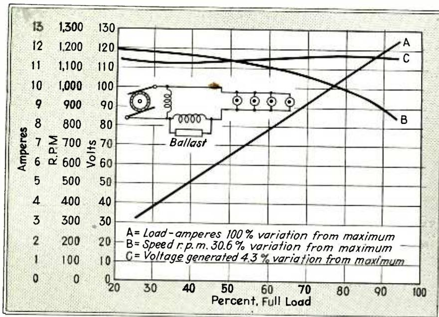
Fig. 7—Load characteristics of compound wound d-c generator driven by water wheel with constant head. Ballast placed in parallel with the series field
