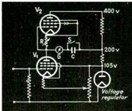
Fig. 2—The basic circuit of the voltage integrator using two pentodes and a voltage regulator tube
