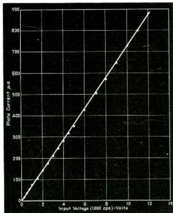
Fig. 4—Input-output characteristics of the combined circuits of Fig. 2 and Fig. 3, illustrating that a linear relationship is accurately attained
