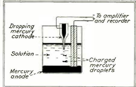
Diagram showing the principle of operation of the dropping mercury cathode
