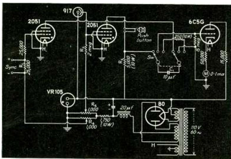
Fig. 2—Wiring diagram of instrument, including voltage-regulated power supply
