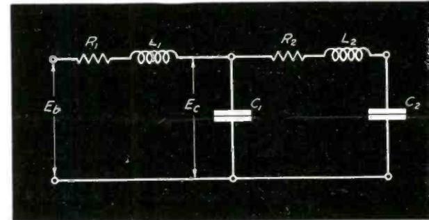
Fig. 6—(Above) Equivalent electrical circuit of the acoustical network
