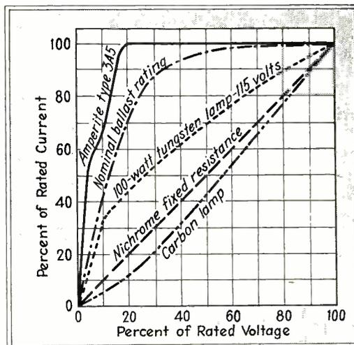
Fig. 2—Voltage-current characteristics of carbon and tungsten lamps compared with those of resistance regulators. Neither type of lamp offers much advantage over a straight dropping resistance whereas the regulator tubes provide regulation over a wide voltage range
