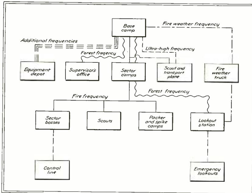
Fig. 1—Block diagram of the radio net used by the U. S. Forest Service in fighting a forest fire of the "conflagration" class—one whose area is 50,000 or 75,000 acres and whose perimeter is about 100 to 150 miles
