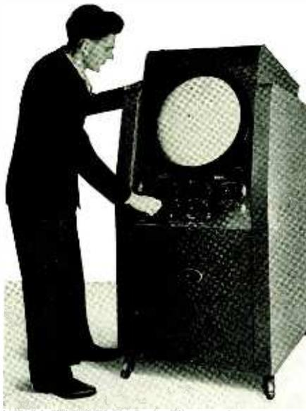
★ Designed particularly for lecture-room and demonstration purposes, this new DuMont Type 233 Cathode-Ray Oscilloscope provides huge oscillograms on its 20-inch high-intensity screen. Also invaluable for critical laboratory investigations.
