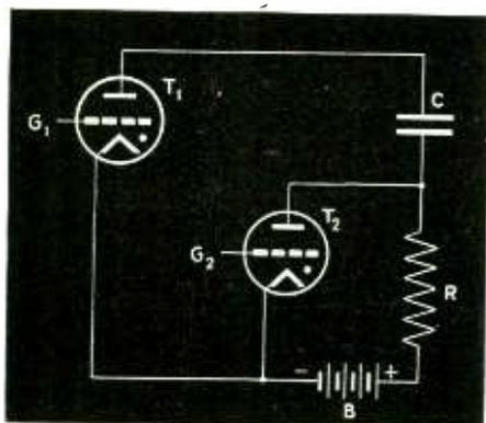
Fig. 1—Basic circuit of interval timer using two gas tubes and a condenser
