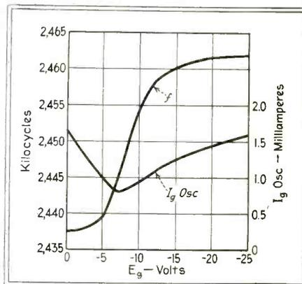
Fig. 2—Variation of oscillator frequency and oscillator grid current of the circuit shown in Fig. 1 as the modulating grid voltage is varied
