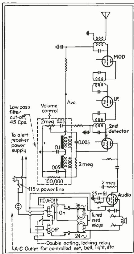
Fig. 2—Simplified circuit diagram of the alert receiver
