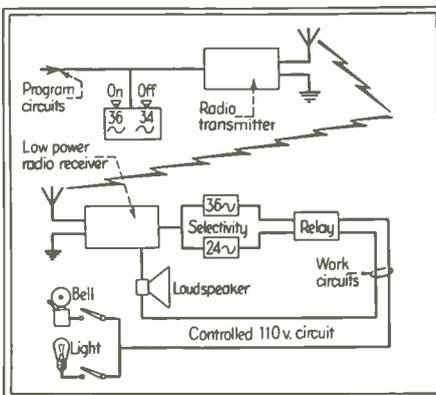
Fig. 1—Block diagram of the transmitter-controlled receiving system
