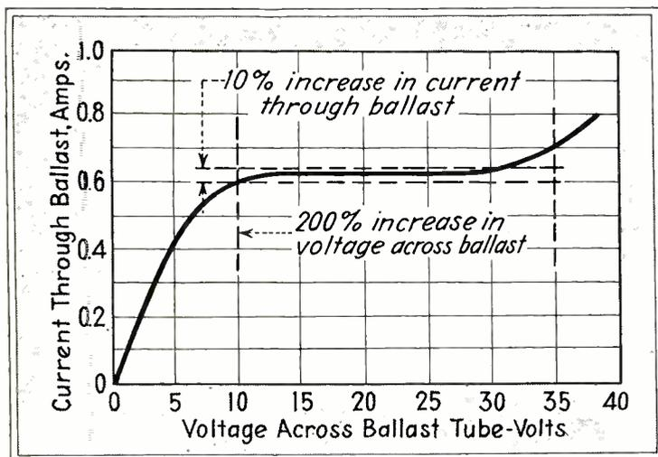
Fig. 1—Nominal characteristics of ballast tube. For a 10 percent change in current through the ballast, a voltage change of 200 percent occurs
