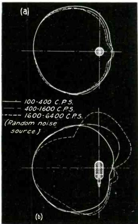
Fig. 3—(Left) Horizontal (a) and vertical (b) plane polar response patterns of a two unit cardioid microphone
