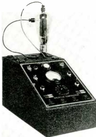
grid control; mercury rectifiers—current wave form and plate current; high vacuum rectifiers—current wave form, and plate current; high vacuum control tubes—wave form, plate current, and grid control; full-wave rectifiers (2 plate)—wave form and plate current on each half, individually.
