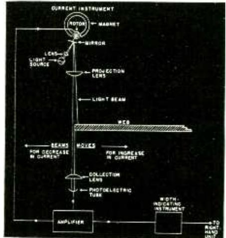
Fig. 2—Diagram illustrating principle of operation of the photoelectric width gage
