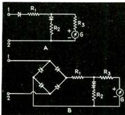
Fig. 1—Fundamental half-wave circuit (A) and full wave bridge rectifier circuit (B) for straightening out the characteristic of the rectifier
