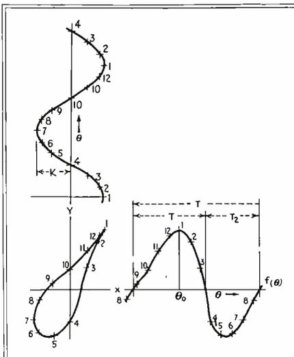
Plotting the Lissajous figure for the fundamental sine component of  $f(\theta)$  with  $\theta_0$  at the positive peak
