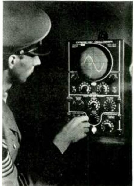
can be used under adverse lighting conditions or in total darkness when necessary. The specially processed steel panel is treated with a non-radioactive luminous paint that retains its maximum luminosity for several minutes after exposure to ordinary light, and can be observed for an hour or more after that. The glow is of the same color and intensity as the standard medium persistence screen of the cathode-ray tube used. The black-out panel is an optional feature in Type 208 oscillograph.
