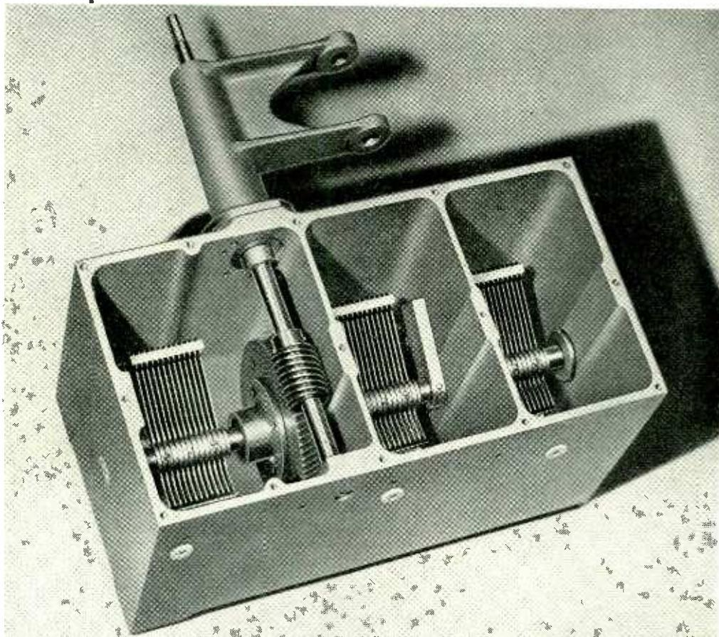
Marine condenser built to withstand severe vibration.
