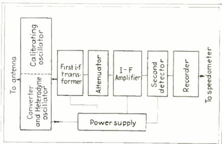
Fig. 2—Block diagram of the portable field intensity recorder
