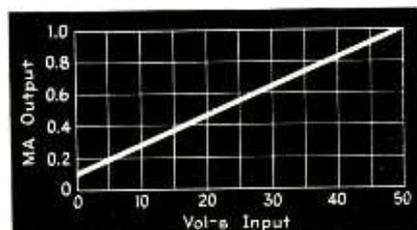
Fig. 5—VTVM calibration curves. Above—current output versus input volts. Below—calibration of current output in terms of time
