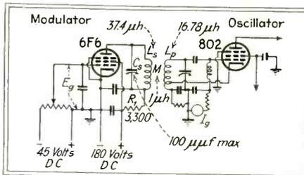
Fig. 1—Circuit diagram of the frequency modulator inductively coupled to a self-excited oscillator operating at 2.5 Mc
