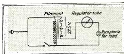
Fig. 6—Circuit of the set-up shown in Fig. 5 in which a filament transformer supplies the additional voltage required by the drop in the ballast resistance
