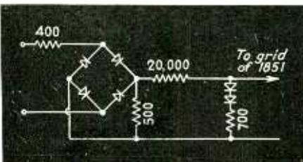
Fig. 3—Practical network for obtaining linear output from a commercial bridge type copper oxide rectifier. Resistance values are given in ohms
