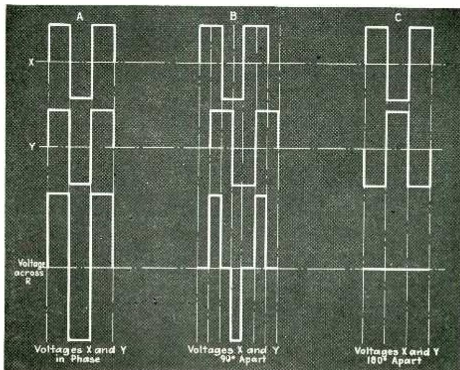
Fig. 2—Algebraic addition of two square waves produces a wave whose average amplitude is a direct indication of the phase angle between the original waves
