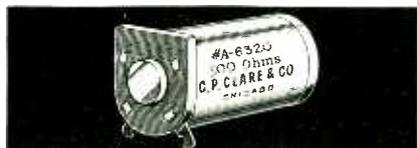
The small coil is equipped with a front spool head having a flat side. This locks the entire coil in place against the heelpiece, preventing it from turning or becoming loose. The screw holding the coil in the heelpiece is equipped with a split type lockwasher. The coil is carefully wound to exact turns on precision machines. Coils can be supplied impregnated
