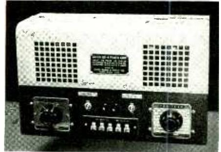
ma direct current. The unit illustrated is the SC-4 which produces 7.5 volts at 5 amps alternating current, and 500 volts at 200 ma, direct current.
