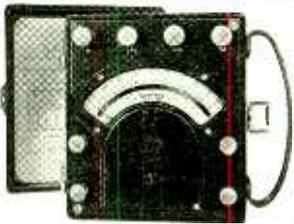
PY-5 portable, 1/2% accuracy, for a-c measurements, has mirrored dial for accurate reading.
