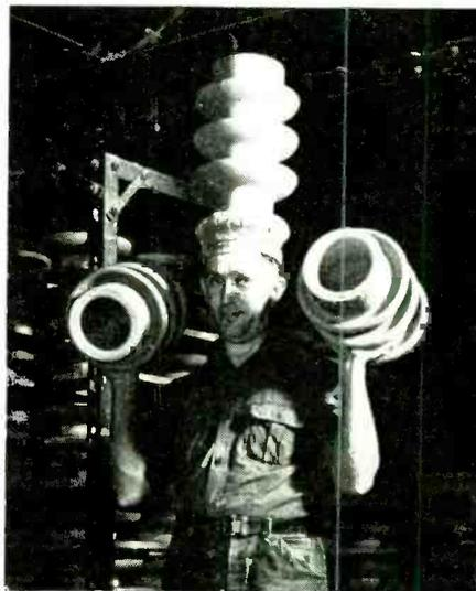
The insulators shown here are for condenser bushings to insulate high voltage wires attached to transformers and circuit breakers. Stephen Kelly at the Westinghouse plant at Derry, Pa., balances a 20-lb. high-voltage insulator on his head and one in each hand. He walks a few steps to a conveyor which carries them to the kilns, thus speeds up production
