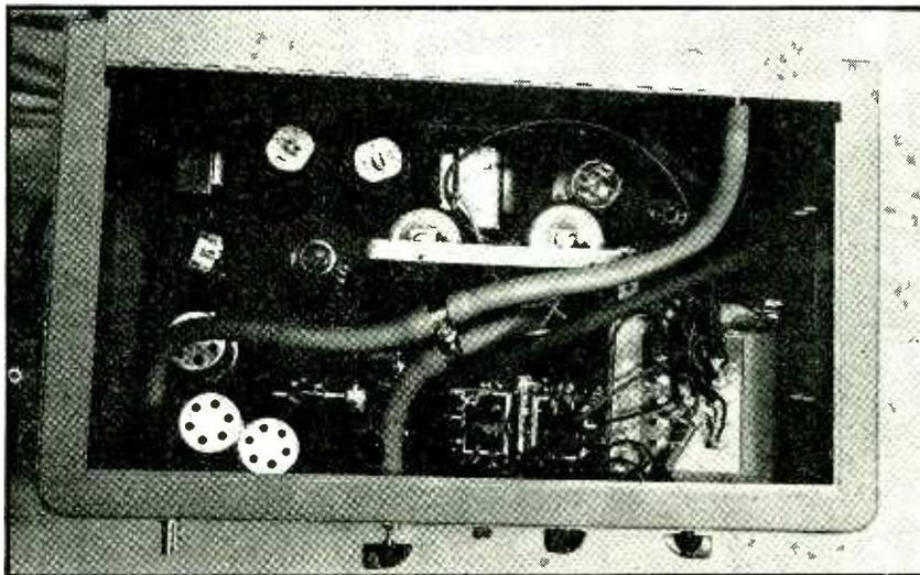
Inside view of the unit housing the amplifier, power supply, thyatron and relays
