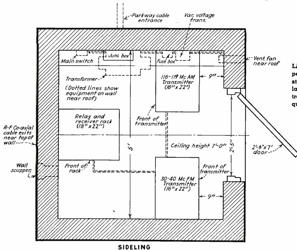
**LAYOUT**—Plan view of typical hilltop repeater equipment house. All six repeater stations have 116-119 Mc amplitude modulated transmitters and combination control receiver and relay racks. The frequency modulated transmitter is omitted at Tuscarora and Ray's
