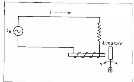
Fig. 1—An electromechanical device where the input voltage produces a motion of velocity  $V$  in the armature
