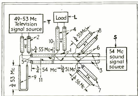
odd number of quarter wavelengths at the same frequency and the third having an effective electrical length equal to an odd number of quarter wavelengths at a different frequency. T. M. Gluyas, Philco Radio & Television Corp. Mar. 15, 1939. No. 2,275,587.
