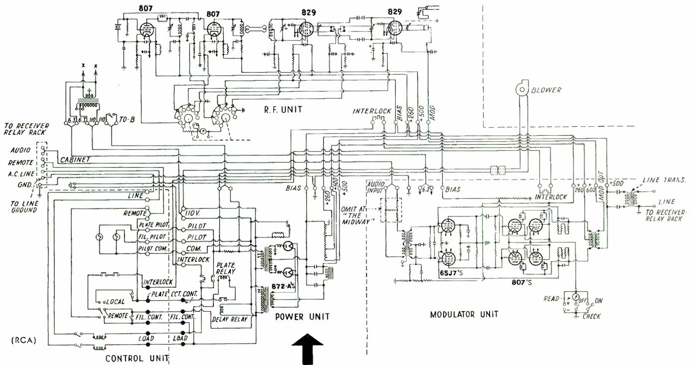
**REPEATER**—50-watt, 116-119 Mc amplitude modulated transmitter of special design. There is one of these at each of the six hilltop relay stations and one at The Midway patrol headquarters
