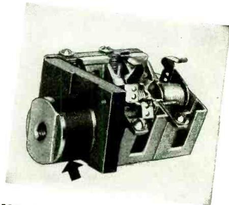
**FOR MOTORS**—The highly arc-resistant quality of G-E mycalex, the fact that it won't oxidize or carbonize, and its resistance to deterioration make it the ideal material for compression-molded brush-holder studs.
