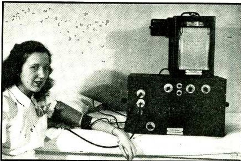
The instrument in use, cuff on patient's upper arm and stethophone strapped to forearm. Amplifier, power supply, control thyatron and relays are contained in the lower unit, while the modified dynamic speaker structure driving the sound actuated pen may be seen projecting to the left of the upper unit housing the pressure recorder
