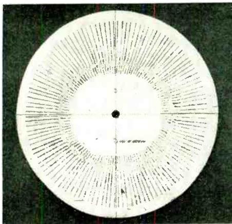
FIG. 1—Plot of typical test coil when using pencil lead as a Fluxgraph recording stylus
