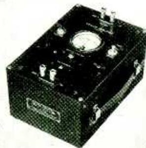
A highly stable amplifier giving gains of exactly 10 and 100 times. Operated by self-contained batteries. Through the use of special circuits the gain is independent of battery voltage, circuit constants and tubes within 2% from 10 to 100,000 cycles. Particularly useful with our Model 300 Electronic Voltmeter to increase its sensitivity, permitting voltage measurements down to 30 microvolts. Send for Bulletin 7.
