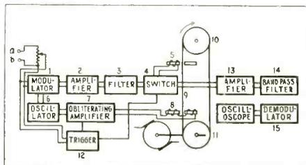
Fig. 3—Block diagram of the complete magnetic recording and reproducing system
