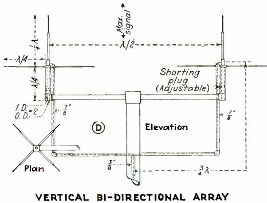
**DETAILS**—The five antenna types used by fixed stations are here illustrated, with electrical as well as mechanical data shown. All of them employ 70 ohm coaxial transmission lines
