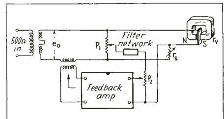
Fig. 2—Feedback applied to a light-valve circuit
