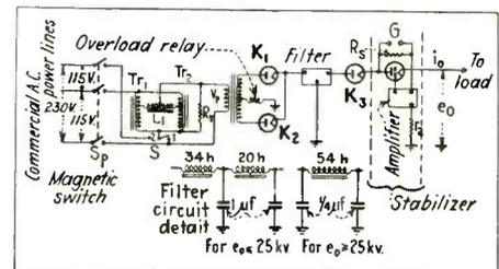
Fig. 1—High-voltage electronically stabilized power supply, including the filter circuit details
