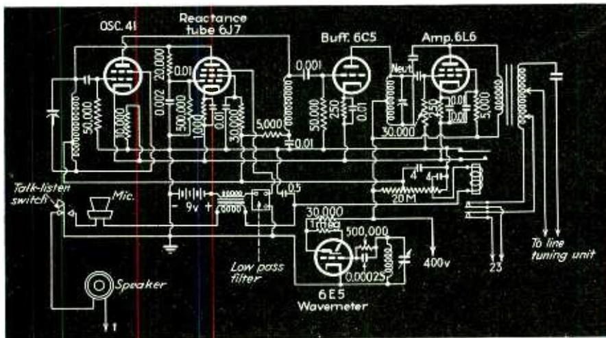
Fig. 1—Circuit diagram of transmitter working "straight through" without frequency multiplication. The reactance tube modulator provides a maximum frequency deviation of 12 kc
