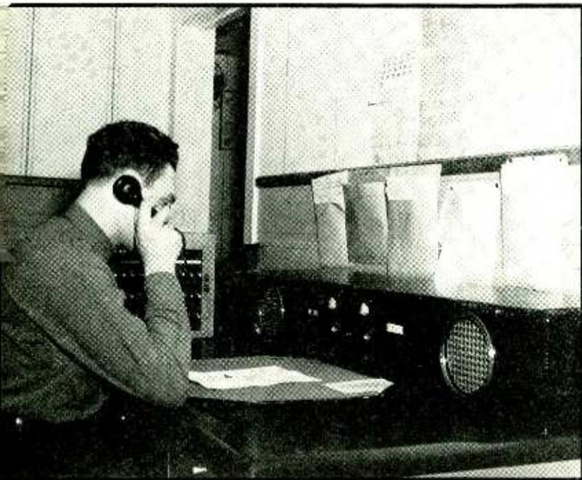
**MIDWAY PATROL HEADQUARTERS**—Many of the messages transmitted over the turnpike communication system originate at this "shuttle" relay point. One meter on the panel of the control unit illustrated indicates r-f when the local 116.95 Mc transmitter (in an adjacent room) is in use. The other is a modulation level indicator. Receivers at The Midway are tuned to 37.5 and 33.94 Mc
