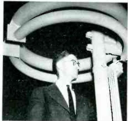
The circular antenna, described by M. W. Scheldorf, has unusual applications for use on vehicles, because of its ruggedness and small size
