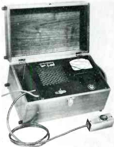
many applications in photography, and can be used to measure the density of spectrographs, brightness of paints, measurement of low turbidities and haze, etc.
