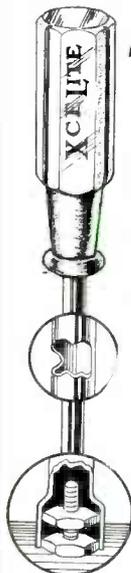
• One of the handiest tools ever designed for electrical and radio work—especially panel assembly jobs. The nut is readily tightened or loosened without damage to the panel. On telephone or power switchboard, the hollow shaft readily slips over the long protruding bolts or studs and the socket firmly engages the nut. Shock-proof handle; precision machined shafts and sockets. Five sizes, from 5/16" to 5/8" (nut sizes). Full details on request.
