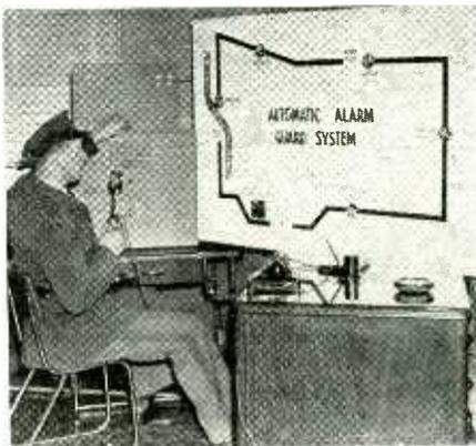
Shown here is the master control board of the "acoustic fence" which helps protect a war production plant of the E. I. duPont de Nemours Co. somewhere in the United States. A light glows on the "map" outlined on the control board which notifies the guard that someone is tampering with some part of the miles of high wire fence surrounding the plant
