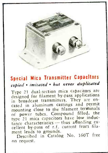
**Special Mica Transmitter Capacitors**
