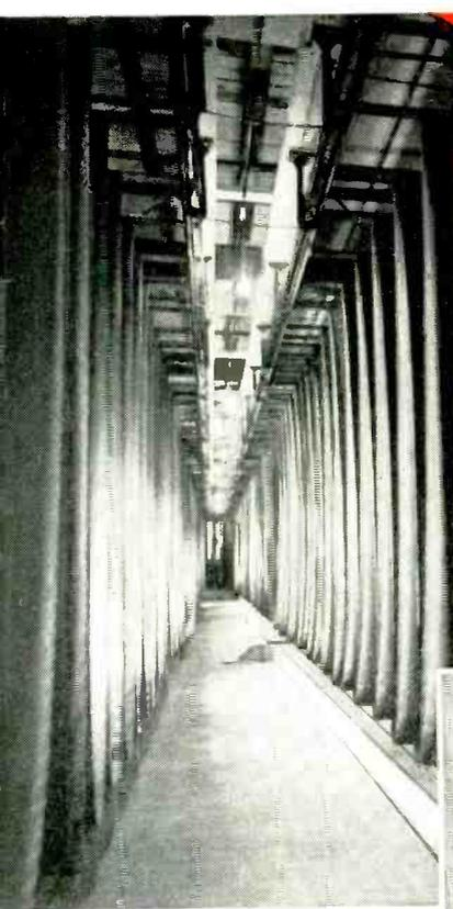
**MEASURING X-RADIATION.** The 1,400,000-volt constant potential X-ray equipment installed at the National Bureau of Standards utilizes kenotrons to develop the high potential. The c-c generator (double stack at left) consists of a high-voltage resistance potentiometer (narrower column), and 10 individual voltage-doubling rectifiers, cascaded one above the other (wider stack), using two kenotrons in each 140-kv stage. The stacks at right are 10-section X-ray tubes, one being a spare.
