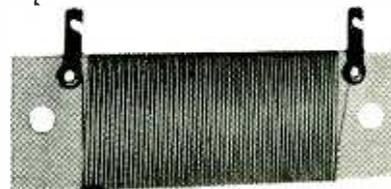
TYPE JN—mica card, standard tolerance 1%, maximum resistance—100,000 ohms, size 1" wide x 3/4" long x 1/16" thick. Mounting by insulated holes to clear 6/32 screw. Terminals: hot tinned copper lug.
