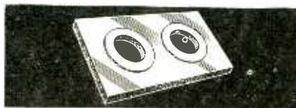
Spring insulators are made from special heat treated Bakelite that permits punching without cracks or checks and possesses minimum cold flow and low moisture absorption properties. Each Type K Relay is given a 1000 volt a. c. insulation breakdown test.
