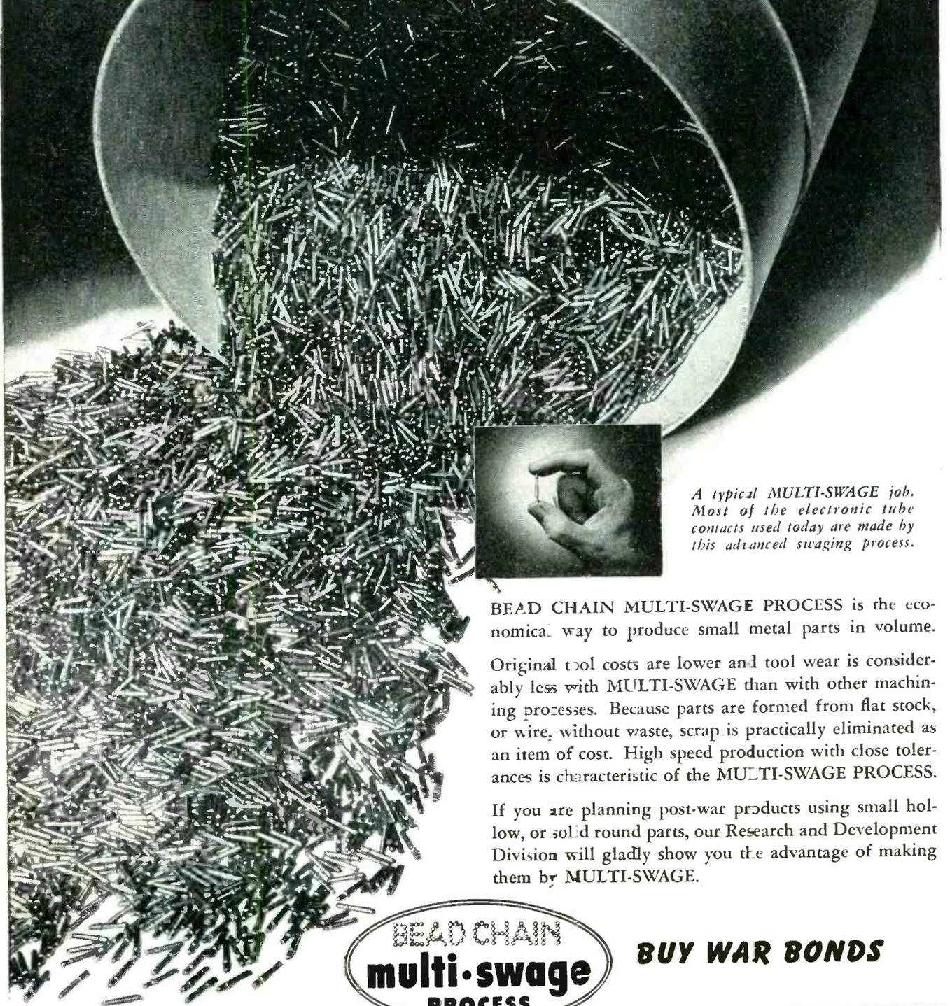
*A typical MULTI-SWAGE job. Most of the electronic tube contacts used today are made by this advanced swaging process.*
