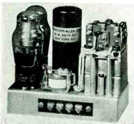
energized by power supplies turning out between 100 and 135 volts at frequencies between 350 and 450 cps, at temperatures ranging between 40 and 65 deg C with up to 95 percent relative humidity. Maximum temperature rise on continuous duty from a 25 deg C ambient is 25 deg C. The unit withstands 10-g shock-impact or vibration-acceleration tests
