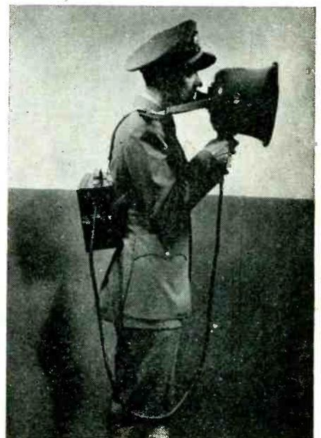
A portable amplifier and self-contained batteries permit this electronic megaphone to be used anywhere for sound reinforcement. A product of Operadio Mfg. Co., the unit has the same specifications outlined on page 125 of November ELECTRONICS
