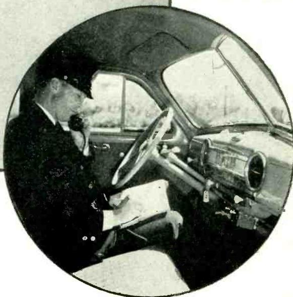
Forty-four mobile units with two-way phase-modulated radio equipment and seven supervisory cars with receivers keep streetcars and buses operating smoothly under all emergencies, proving the effectiveness of low-power p-m in covering 190 square miles of territory
