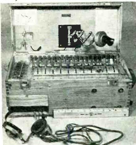
View of a ten-line Italian telephone switchboard for field use. Switches rather than cords are used for making connection. Except for broken transmitter horn, this captured equipment appears to be in operating condition. It would seem that the microphone and its support might easily be damaged by accidental closing of the cover of this unit
