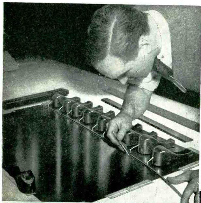
To speed the making of templets for complex aircraft parts, one of America's leading fighter plane manufacturers uses an ingenious method of photographing tracings directly on steel plates. The original drawing is carefully traced on a sheet of VINYLITE Rigid Plastic. The result is an extremely clear, plastic negative.
