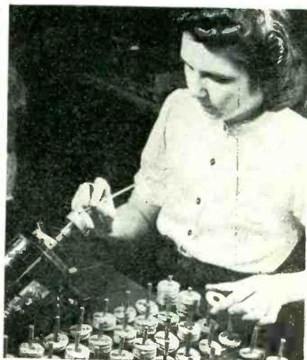
Applying colloidal graphite solution (Aquadag) to discs for copper-oxide rectifiers with a brush while the discs are rotated by an electric motor at a Westinghouse plant. The solution reduces contact resistance
