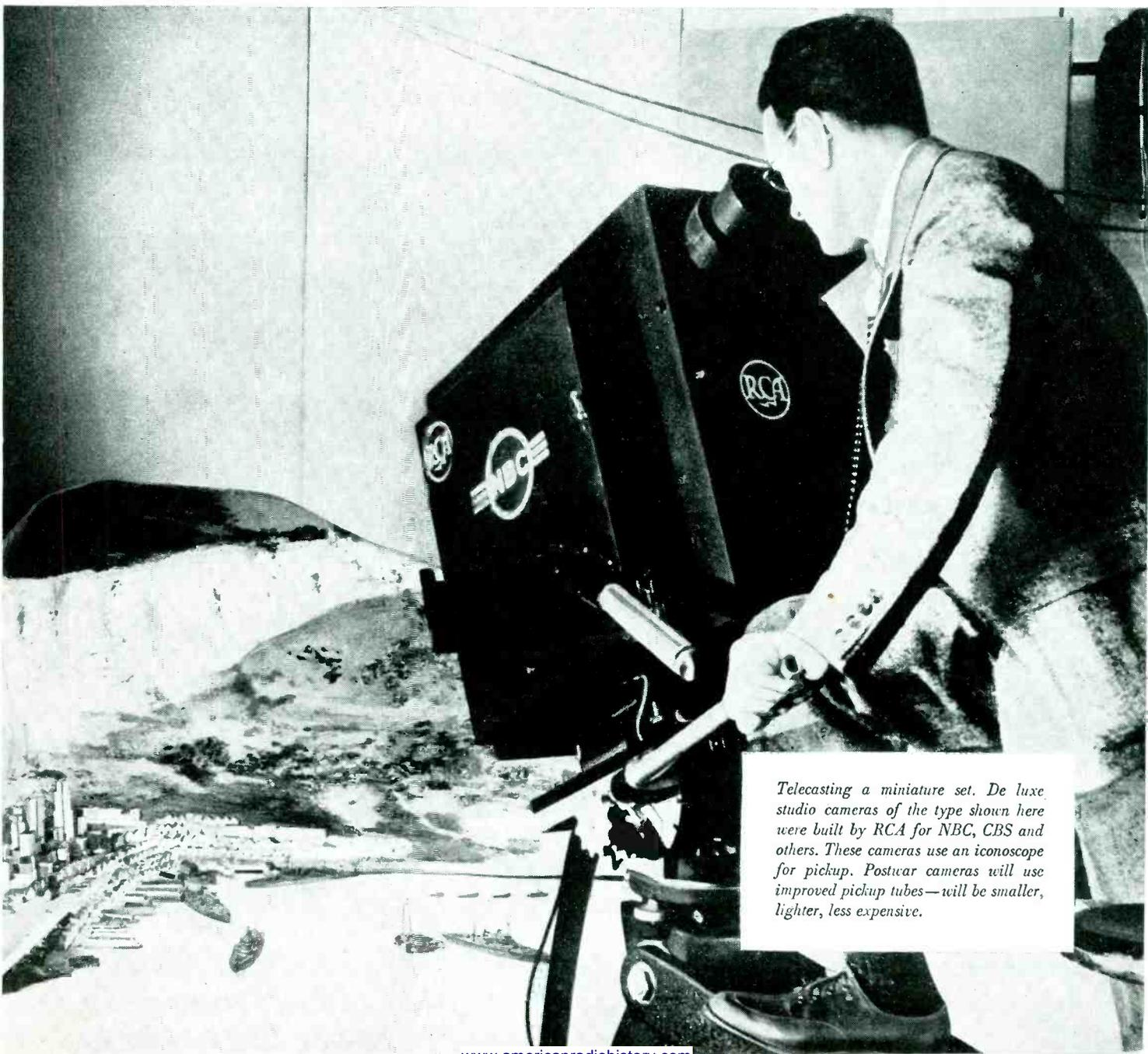
*Telecasting a miniature set. De luxe studio cameras of the type shown here were built by RCA for NBC, CBS and others. These cameras use an iconoscope for pickup. Postwar cameras will use improved pickup tubes—will be smaller, lighter, less expensive.*
