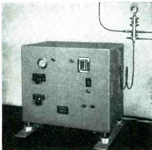
**AUTO-DRYAIRE**, a completely automatic device for maintaining pre-set pressures of moisture-free air in coaxial transmission lines. It is independent of critical gases and heavy cylinders and will function for indefinite periods, providing 1,000 cubic inches of conditioned air per minute.
