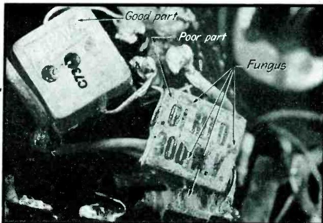
Close-up of two capacitors in Signal Corps SCR-610 equipment, showing how moisture-proofing material provided a home and food for molds in one case while the other component part was unaffected
