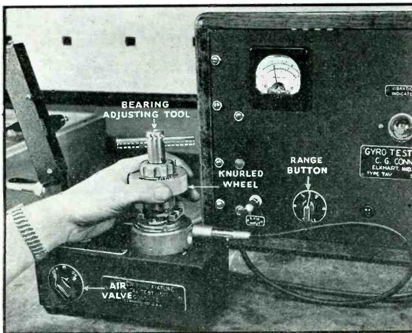
Bearing adjustments can be made to permit a gyro to coast from full speed to rest in a specified time, indicated on the meter. Such adjustments can be made in a few seconds, whereas previous practice was to measure coast time (in the neighborhood of ten minutes) and then make successive adjustments after the gyro had come to rest
