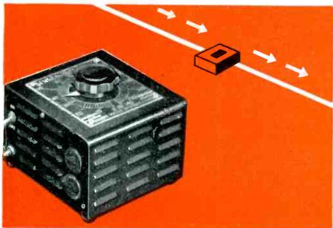
**VARIABLE-VOLTAGE AUTOTRANSFORMER** used for smooth control of uninterrupted voltage and small amounts of power. Mechanically strong, compact, and light in weight, designed for panel or bench mounting. Operates on low input power and low exciting current, with high efficiency and excellent regulation throughout entire range from zero to full load. Made in three capacities. Bulletin GEA-3635A.
