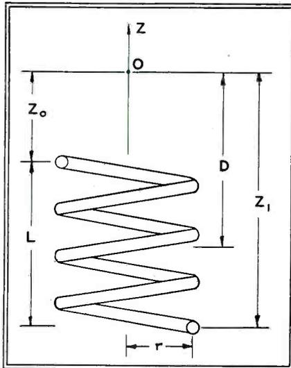
Fig. 1—Helical heating coil
