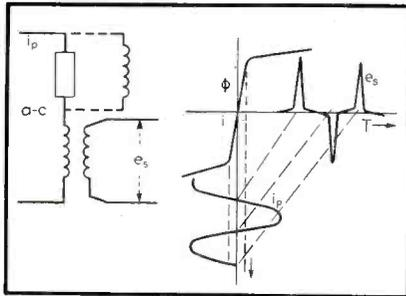
Fig. 10—(left) Use of peaking transformer. The series impedance may be resistive or reactive (shown as dotted)
