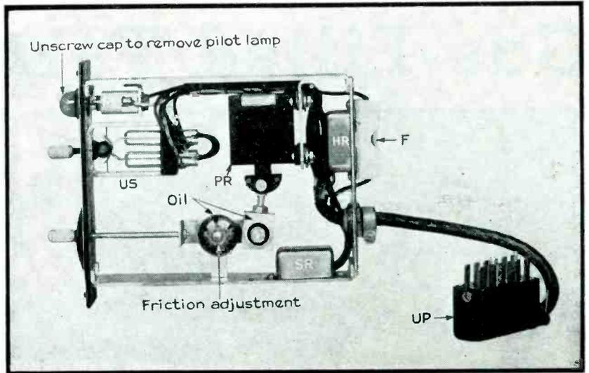
Small solenoid with adjustable core, PR, in a unit control panel
