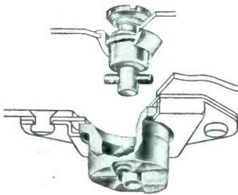
Camloc Fasteners are comprised of three units, Stud Assembly, Grommet and Cam Collar. They are four to ten times faster in installation than similar devices.
