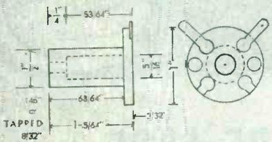
The molded Bakelite bobbins, upon which the chokes illustrated are wound, are carried in stock to these dimensions.
