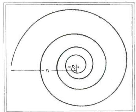
Fig. 8—An Equiangular Spiral for the special case  $r_o/r_1$  equal to 0.1 and  $N$  equal to 4
