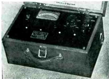
mental samples of insulating material. The instrument consists of an electronic rectifier, a Thyrite bridge circuit, and an electronic-tube voltmeter. It is available in two types. One type has a scale calibrated from 1 to 50 megohms and measures resistance at 500
