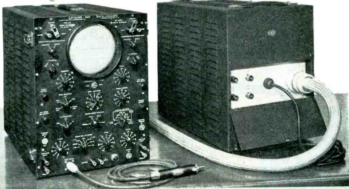
Wide band vertical axis amplifier usable to 10 MC.
