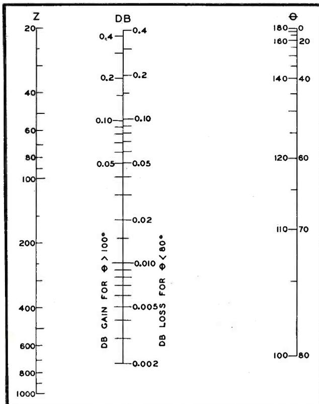
FIG. 4—Chart for large values of impedance  $Z$  and small db losses and gains
