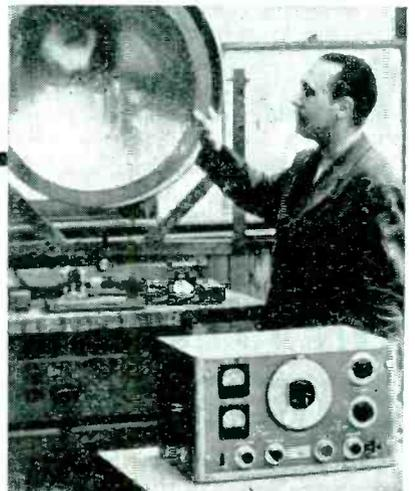
*Audio signal generators providing standardized voltage throughout the audio frequency range. Model 250AG Audio Signal Generator illustrated.*
