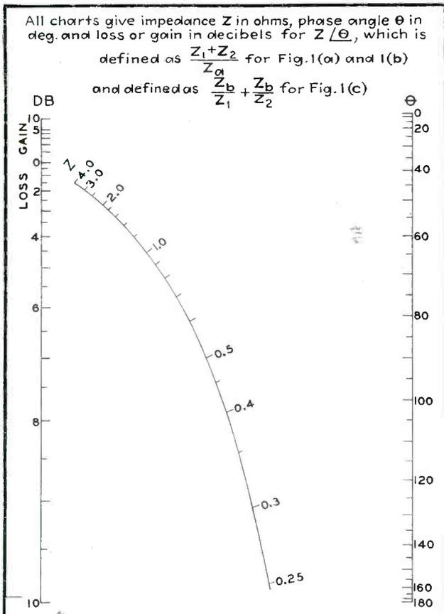
FIG. 2—Chart for small values of impedance  $Z$  and large db losses and gains
