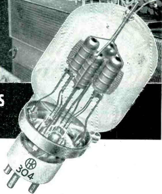
THE HK-304H Gammatron is a high-voltage, low-impedance tube capable of passing large amounts of current. This unusual combination of features is made possible by the use of four separate sets of tube elements operating in parallel within one glass envelope. Max. plate dissipation, 300 watts.
