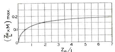
Fig. 5—Maximum field factor when spacing to work is fixed
