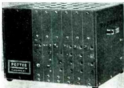
Plug-in construction of various connected units is used throughout. The timer measures 15 x 10 x 10 inches, and weighs approximately 30 lb.
