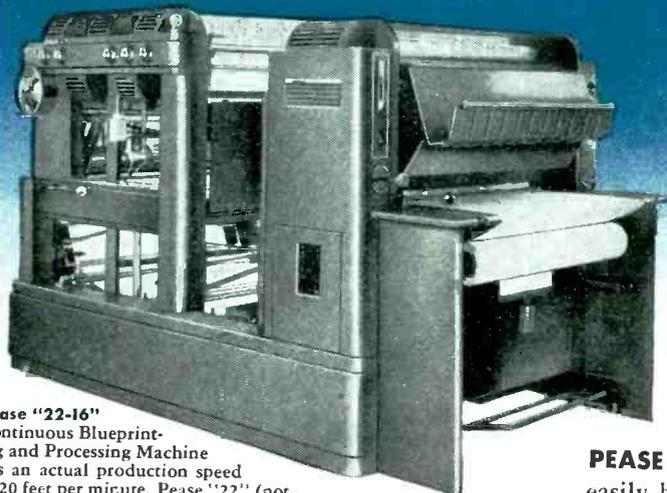
Pease "22-16" Continuous Blueprinting and Processing Machine has an actual production speed of 20 feet per minute. Pease "22" (not illustrated) has a speed of 30 feet per minute.
