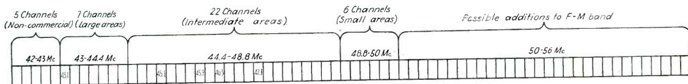
FIG. 2—Allocations in present f-m band and possible extension of the band
