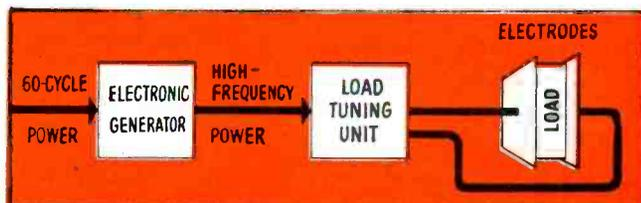
Fig. 1. Elements of an electronic heating installation. Standard 60-cycle power is converted by electron tubes to high-frequency (radio-frequency) power for heating.
