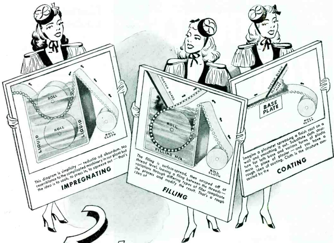
This diagram is simplicity — reductio ad absurdum. No resemblance to the complicated machinery in our plant but the idea is to soak, to press in, to squeeze out — that's
