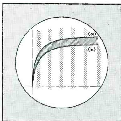
FIG. 1—Cathode-ray oscilloscope screen, showing mask between upper (a) and lower (b) tolerance curves. The additional vertical stripes avoid continuous light output when items under test are defective
