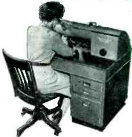
**NEW, COMPACT, G.E. ELECTRON MICROSCOPE** distinguishes objects as small as 1,000,000th of an inch... magnifies them directly to 5,000 or 10,000 times actual size. If photographic enlargements are wanted, blow-ups can be made to show objects at 100,000 times their true size. Can be plugged into a regular 110-volt A.C. line.
