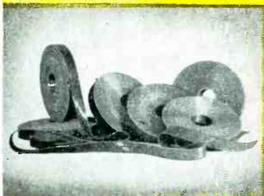
**EMPIRE BIAS-CUT TAPES** have elongation properties not possessed by standard straight-cut tape. They are ideal for application to conductors and coils, conforming more readily to irregular surface. Extra stretch avoids the coning effect produced when wrapped helically. Available in yellow (suitable for continuous oil immersion,) or black (for higher dielectric strength).
