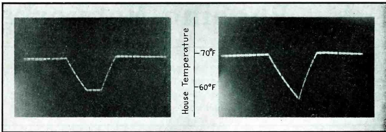
FIG. 3—Representative oscilloscope patterns of house temperature plotted against time of day. Each pattern represents a 24-hour day during which outside temperature was 0°F. Left: Heat supplied during low period. Right: No low-period heat
