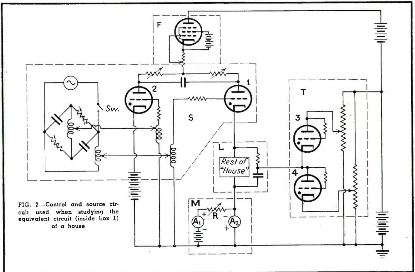
FIG. 2—Control and source circuit used when studying the equivalent circuit (inside box L) of a house
