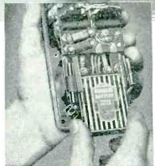
Battery slides into place, Easily inserted or removed.
