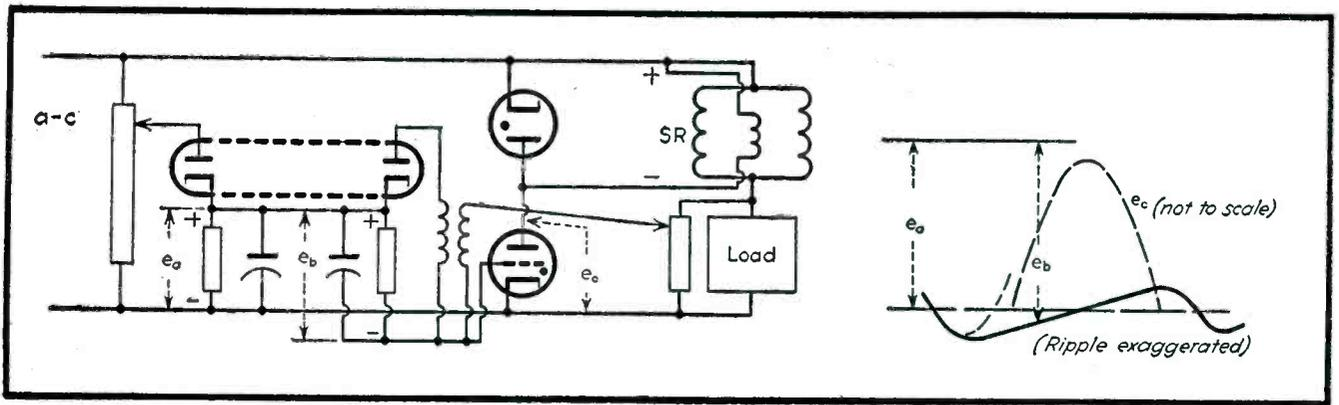
Fig. 9—Grid control for saturable reactor excitation, with curves of wave form
