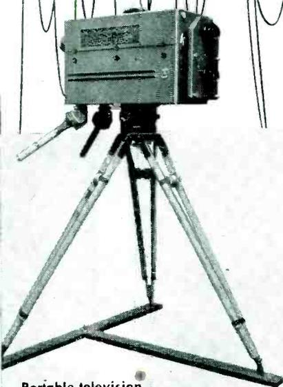
Portable television camera developed by RCA engineers. An improved version of earlier models, this camera uses an orthicon-type pickup tube; has a built-in view finder and focusing device.
