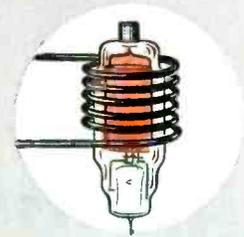
Electronic heat reaches through glass walls to degas metal elements in radio and fluorescent tubes without affecting the envelopes. Action is instantaneous.
