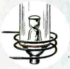
Electronic heat can bond glass to metal faster with finer control of heated area. Often increases production units from hundreds to thousands per hour.
