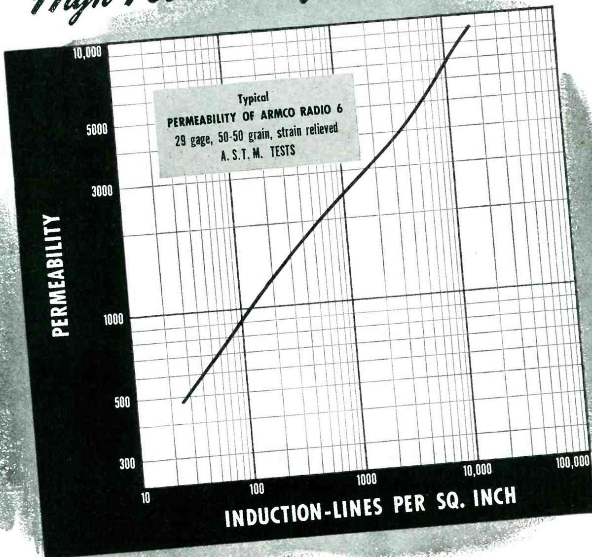
Typical high permeability of ARMCO "Radio 6" at various inductions is shown on the curve reproduced here. This grade of electrical steel was created for use in audio transformers, but it is also excellent for the cores of other electromagnetic apparatus. Its primary purpose is to provide superior magnetic qualities at the lower inductions.
