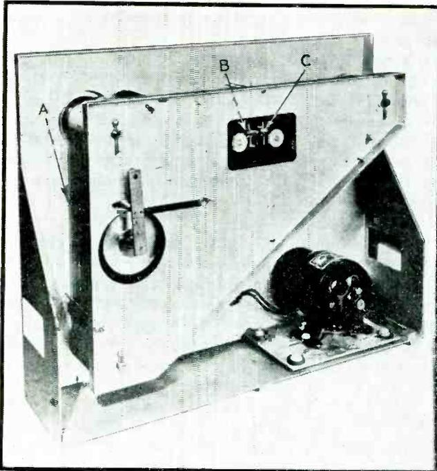
A 100-foot endless tape of special magnetic steel called "Vicalloy" (at A) provides a full minute of voice recording. At B—wiping-out coil; C—recording and playback coil
