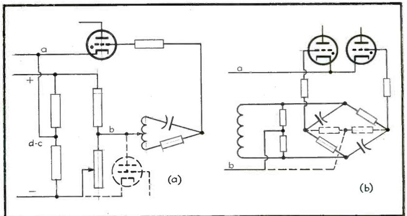
Fig. 8—Control by varying d-c voltages. At (a), a tube (shown as dotted) is employed as the variable resistor; at (b), circuit variation to control two thyatrons and to obtain mid-tap
