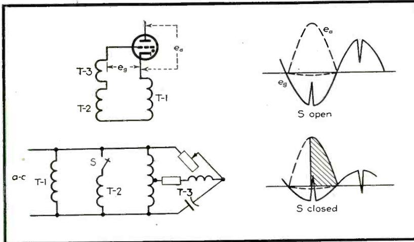
Fig. 13—Three-transformer grid circuit for thyatron used to fire an ignitron as in Fig. 12. T-1 supplies hold-off voltage; T-2 supplies turn-on voltage; T-3 supplies peaking voltage, adjustable phase; S is a control switch
