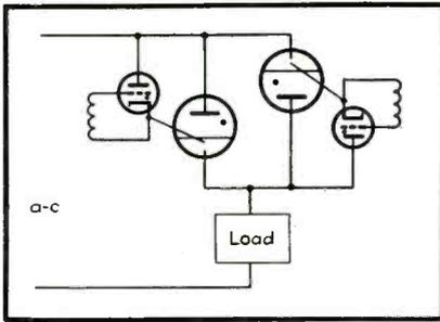
Fig. 12—Anode firing of ignitrons by thyratrons acting as single-phase a-c switches
