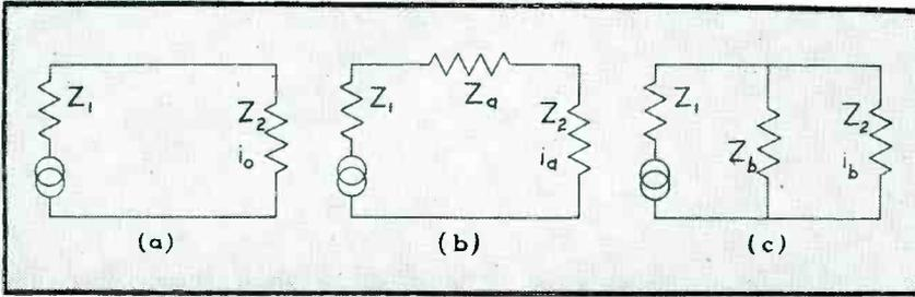
FIG. 1—Equivalent circuit of transmission line (a), same circuit with inserted series impedance (b), and same circuit with inserted shunt impedance (c). Accompanying charts give insertion loss or gain in these circuits
