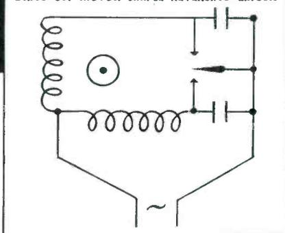
Design Engineers requiring a low-inertia, quick-reversing unit will be interested in the many new types of Kollsman Drag Cup Motors—particularly the new 115 volt 60 cycle units which can be run directly from a regular single-phase outlet with the addition of a capacitor as shown in the main illustration.
