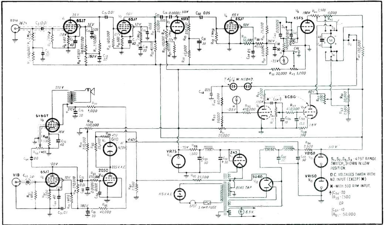
FIG. 3—Schematic wiring diagram of Conn electronic gyro test unit. The tube complement corresponds to the tube designations given in Fig. 1
