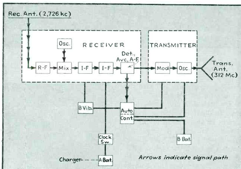
FIG. 1—Block diagram of W6XFE gear, comprising a medium-frequency super-heterodyne automatically controlling and modulating an ultrahigh-frequency oscillator. Details are given in the schematic of Fig. 2
