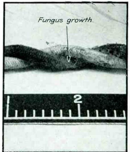
Interphone amplifier section of Signal Corps SCR-528 radio set, showing fungus growth on cabling, and close-up of twisted-pair
