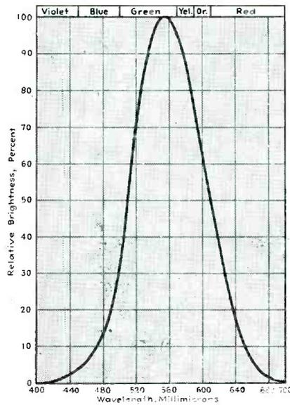
FIG. 3—Standard visibility curve for the average human eye, with wavelength ranges corresponding to common colors
