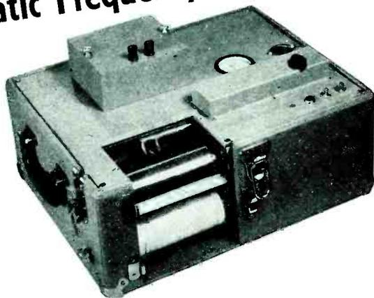
**Provides, automatically, frequency response characteristics of all kinds of communication apparatus on standard charts.**
