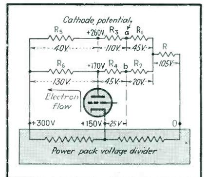
FIG. 2—Diagram illustrating how current drawn through  $R_6$  by the conducting triode section upsets potentials in one branch of the resistance network
