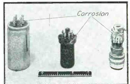
A vibrator, tube and cable-connector, illustrating how corrosion attacks in the tropics when such parts are untreated
