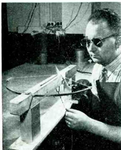
This cross-bow shoots an arrow that stretches hot quartz into thin filaments for calibrating electron microscopes
