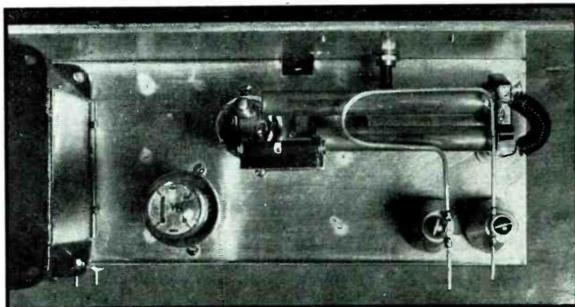
Simple super-regenerative receiver used at KFCD in Los Angeles to pick up signals from W6XFE, nine miles away on Flint Peak
