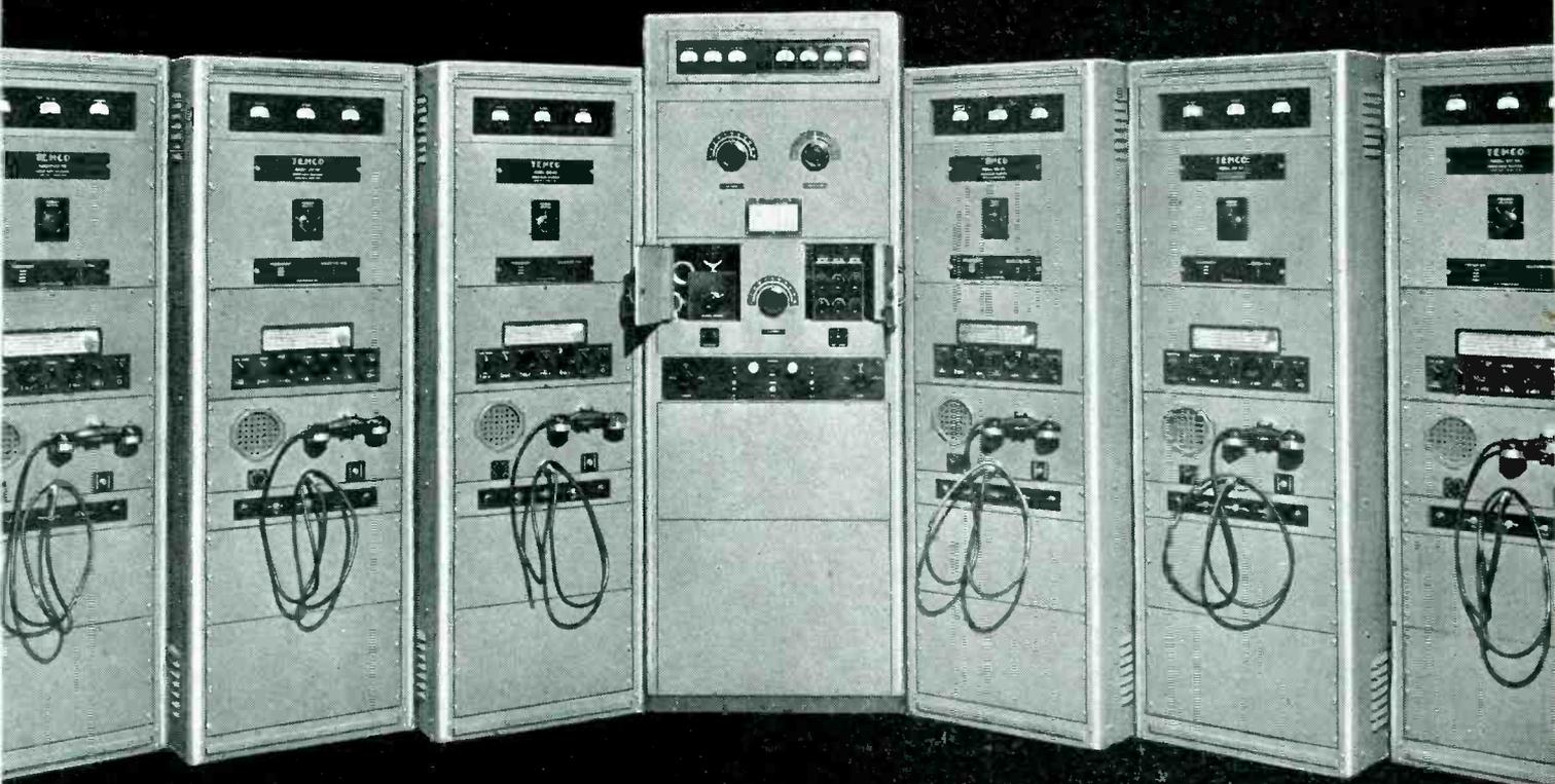
A 2-way radio telephone system, comprising 6 TEMCO Model 100 MS 100-watt output transmitters and Model 600 SG 600-watt transmitter, both for telephone and telegraph operation.
