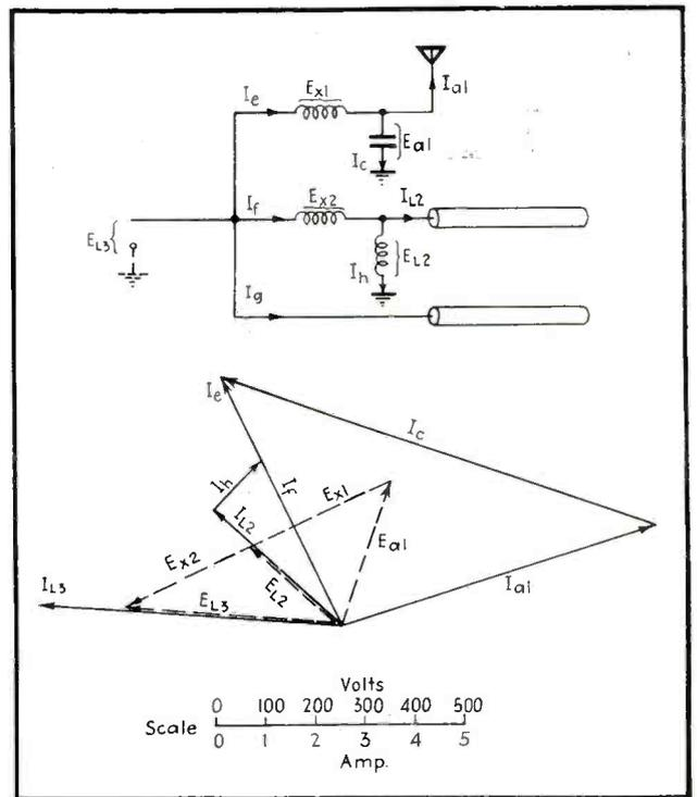
nitudes of the voltages across these transmission lines. With this data, the impedance-matching networks between the transmission lines and the antennas can now be designed.
