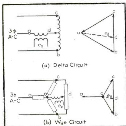
Fig. 2—Auto-transformer or potentiometer to add a fixed voltage to a variable out-of-phase voltage for limited degrees of phase shift
