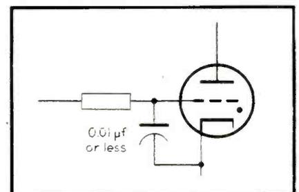
Fig. 15—Grid-cathode capacitor for protection against surge or transient voltages
