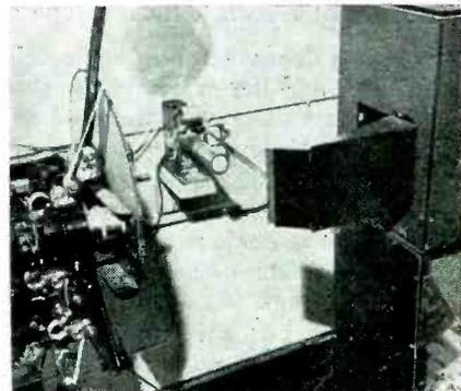
The two-reel movie "Patrolling the Ether," produced by MGM and sponsored by FCC, was broadcast with this equipment. At the left is the projector for the 16-mm film whose image was projected onto an iconoscope in the transmitter at the right. Slides can be projected into the transmitter. By the machine in the center, while printed titles can be combined with projected slide backgrounds in the mechanical device at the lower right.
