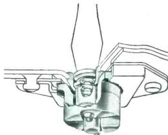
Camloc High Speed Fasteners operate with a quarter turn of the screw driver. They secure doors and access panels in metal, plastic and plywood.
