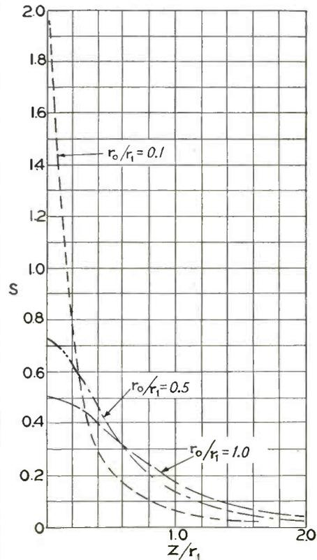
Fig. 9—Variation of the factor  $S$  of an Equiangular Spiral as a function of  $Z/r_1$  for a number of values of  $r_0/r_1$ .
