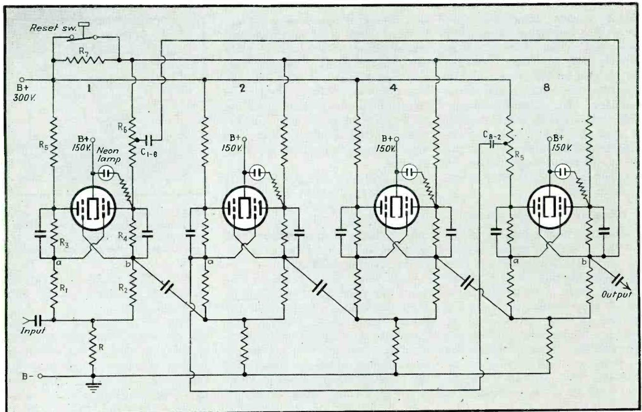
FIG. 3—Complete circuit of the four-tube counter decade
