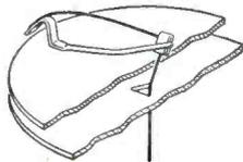
The TUNG-SOL Damper Bar construction is positioned to hold the filament tension spring to one side, thus taking the whip out of the filament above the mica disc. This whip would allow the filament to vibrate, the cause of low frequency pitch known as "howl".
