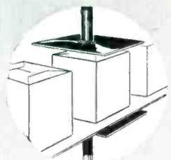
Electronic heat seals packages rapidly and completely in matters of seconds on continuous production lines. Packaged goods containing foods are sterilized.
