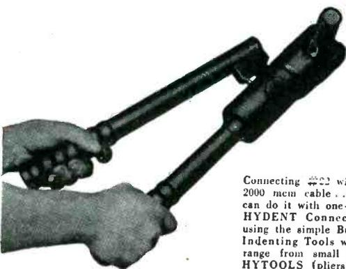
Connecting #22 wire or 2000 mcm cable . . . you can do it with one-piece HYDENT Connectors, using the simple Burndy Indenting Tools which range from small hand HYTOOLS (pliers), to hydraulic HYPRESSES.
