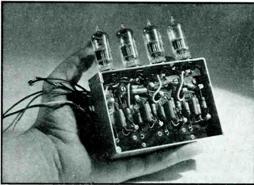
Complete counter decade using four miniature 6J6 tubes. Additional resistors and capacitors are on the other side of the vertical insulating strip. Neon indicating lamps are remotely mounted on another panel
