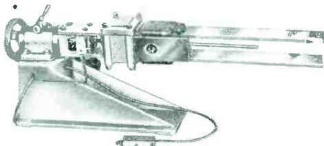
**Features:** Simple harmonic motion with variable amplitude. • Variable frequency from 20 to 70 C.P.S. • Vibration testing can be made in any direction through 360°. • Capacity up to 5 lbs. • Vibration acceleration is provided to 30 G. plus. • Only 75 watts are required for maximum test conditions. • Can be mounted on any bench without transmitting extraneous vibration. • Variable frequency direction provided. • No moving cranks, gears, or bearings in the vibration system.
