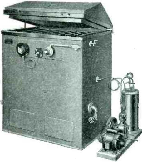
Specifically designed to meet all requirements of latest "SALT FOG TESTING PROCEDURE SPECIFICATION" in accordance with recommendations of the Committee On Standardization Of Salt Spray Test.
