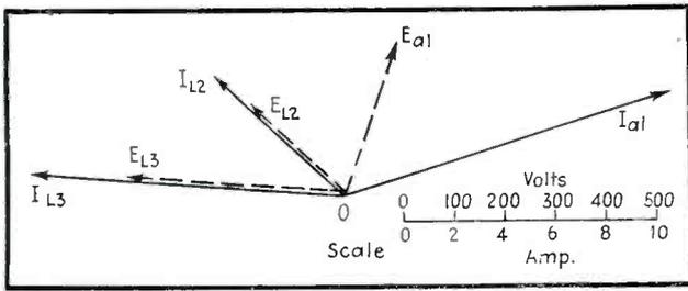
FIG. 7—Vector diagram of voltages and currents which must be produced by phase-shifting and power-dividing networks
