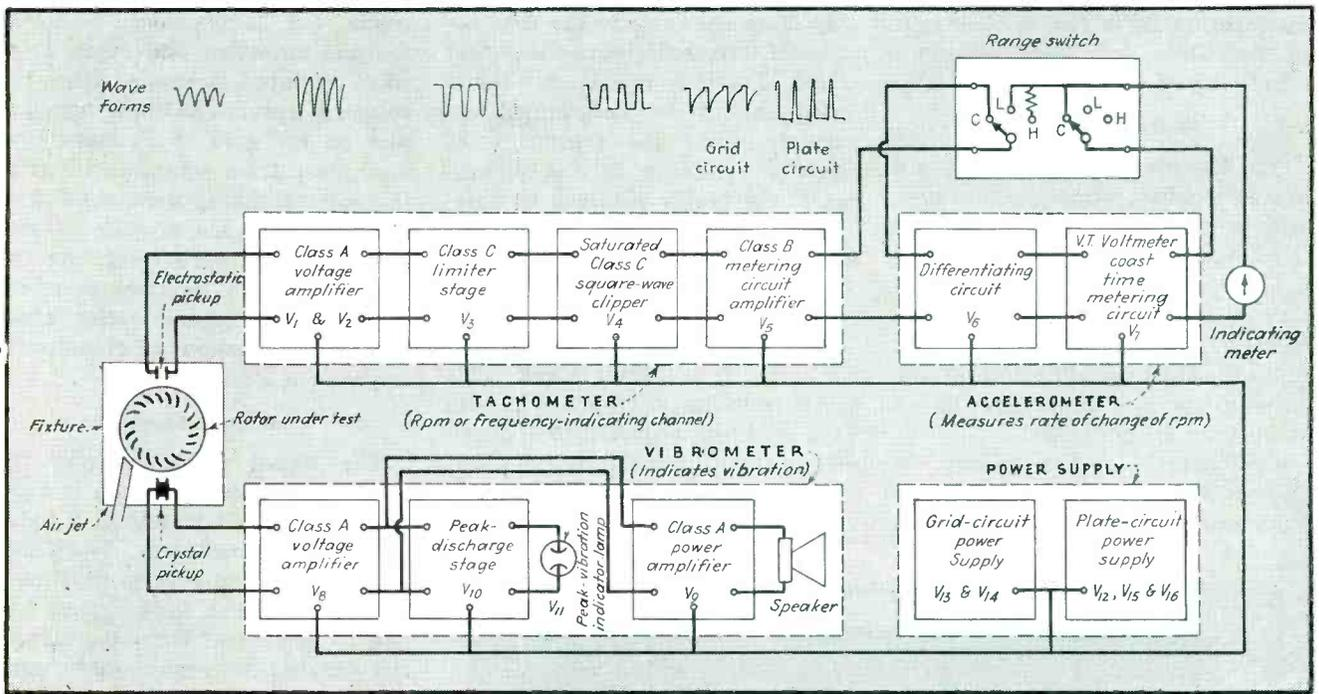
FIG. 1—Block diagram illustrating functional elements of tachometer, accelerometer, and vibrometer. The curves at upper left illustrate oscillographic wave forms observed in portions of the circuit above which they appear
