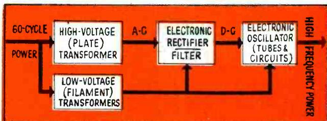
Fig. 2. Simplified block diagram of an electronic generator. In large units, the transformer is located outside the generator enclosure.
