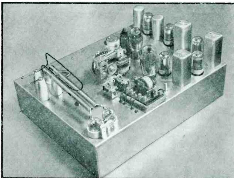
Top view of repeater unit. The receiver is at the right, relays in the center and transmitter at the left
