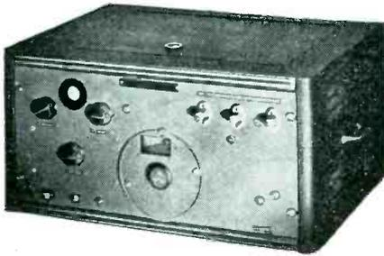
**DESIGNED** for precision measurements of small capacitance and inductance, the G-E radio frequency capacitometer has found acceptance in colleges and industrial laboratories due to its simplicity and compactness.
