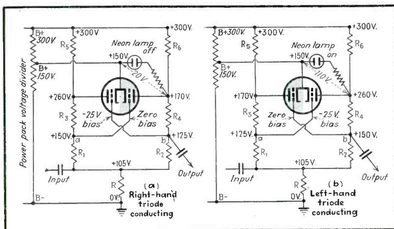
FIG. 1—Simplified version of one stage of the counter decade, giving potentials with respect to ground for the two possible operating conditions
