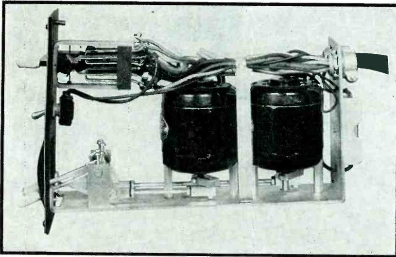
Two rotary control inductors with switches in a control unit used as in Fig. 6
