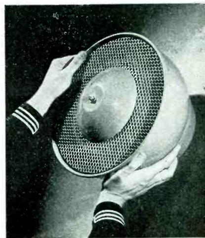
sound pressure of 50 dynes per sq cm when operated at the rated electrical input and measured at 10 feet from the speaker on the sound axis in open air.
