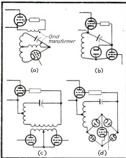
Fig 7—Vacuum tubes replacing resistor of Fig. 5
