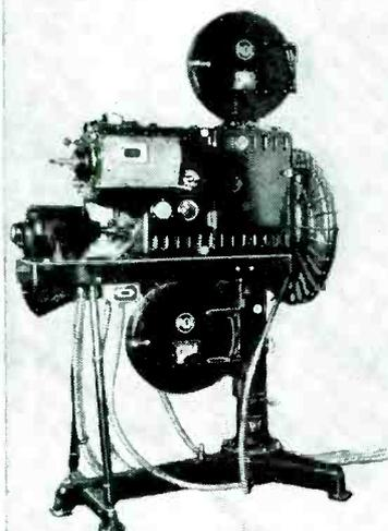
Film projector developed by RCA television engineers. Special construction allows regular movie film (24 frames per second) to be used with 30-frame-interlaced system of television broadcasting now in use.
