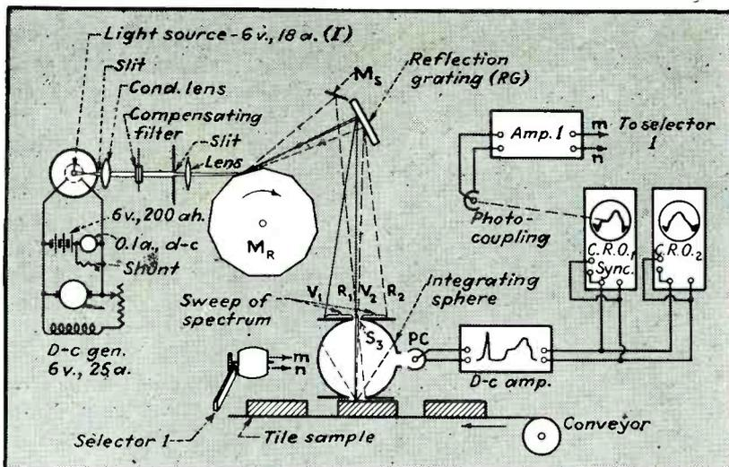
FIG. 5—Arrangement for sorting colored objects, showing one selection channel
