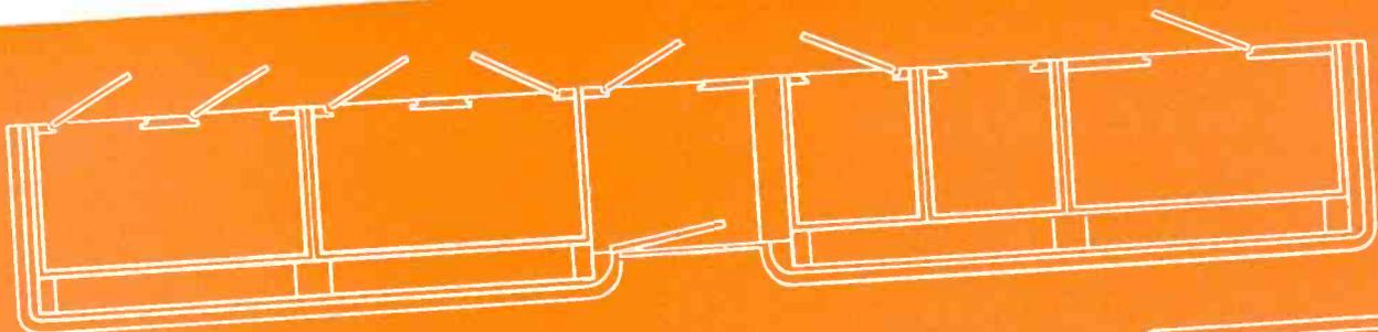
**FLOOR PLAN AND END ELEVATION.** The total length of the transmitter is 39' 6"; height 7' 6"; depth 6' 6". The transmitter proper consists of four cubicles, each 8' wide and 5 1/2' deep. A wide passageway is provided in the center of the transmitter; and electric interlocks prevent transmitter from being placed in operation until all entrance doors are closed.
