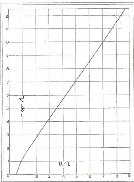
Fig. 3—This diagram shows the optimum value of the radius of a helical coil as a function of the dimension  $D$ , with the coil length fixed
