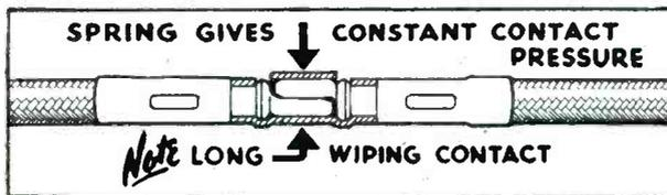
The entire T&B Disconnect system centers around two identical Sta-Kon (solderless) Tips which, when connected, are held firmly together by a strong Beryllium copper spring coupler. Under the constant pressure of the coupler, the tips are maintained in direct, long-wiping contact with each other.
