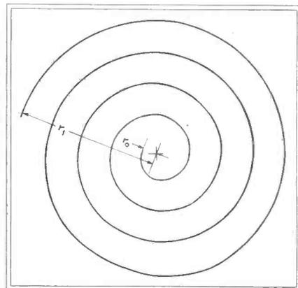
Fig. 6—An Equidistant Spiral, sometimes called the Spiral of Archimedes, for the special case  $r_0/r_1$  equal to 0.1 and  $N$  equal to 4
