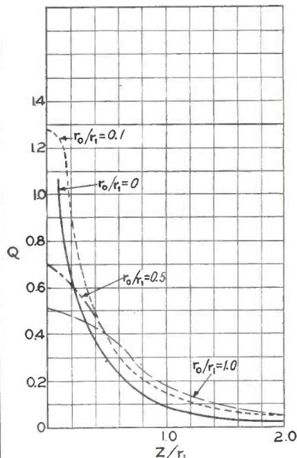
Fig. 7—Variation of the factor  $Q$  of an Archimedes Spiral as a function of  $Z/r_1$  for a number of values of  $r_0/r_1$
