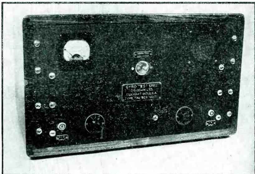
Front-panel view of gyro test unit
