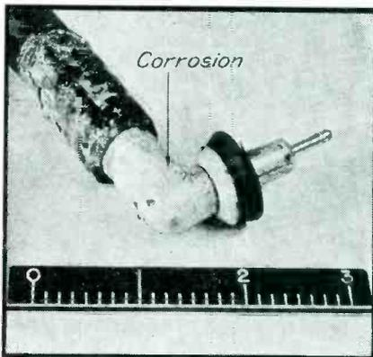
Another example of corrosion of a metal part, coupled with fungus growth on insulation
