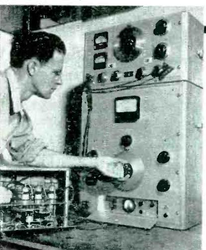
*Harmonic wave analysers with many new features including variable band width. Model 300A Wave Analyser illustrated.*
