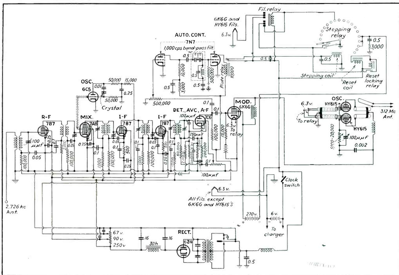
FIG. 2—Schematic of mountain-top radio repeater unit shown on a preceding page in block-diagram form
