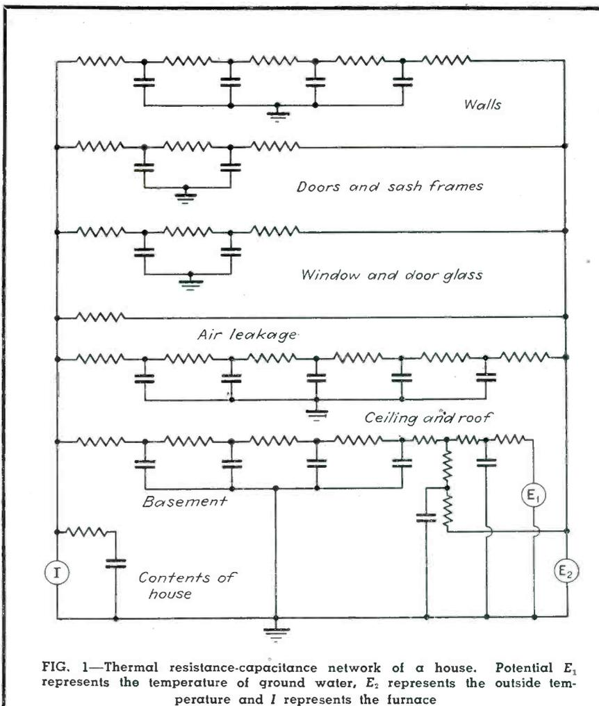
FIG. 1—Thermal resistance-capacitance network of a house. Potential  $E_1$  represents the temperature of ground water,  $E_2$  represents the outside temperature and  $I$  represents the furnace
