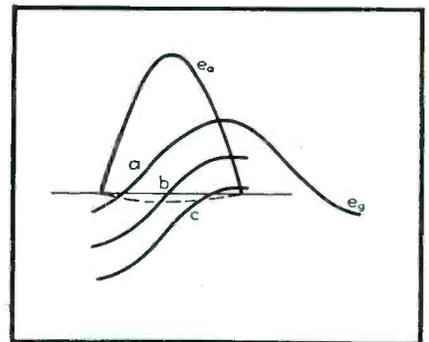
Fig. 4—Grid control by fixed alternating and variable direct voltages. Compare this with Fig. 3
