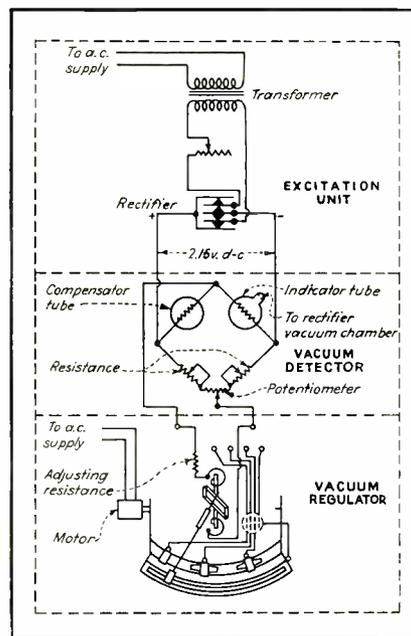
FIG. 6—Hot-filament gage connected in a bridge circuit of a vacuum regulator
