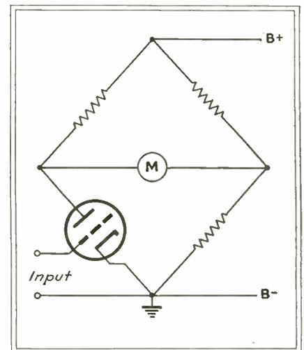
Fig. 2—Stripped to essentials, the electronic voltmeter consists of a bridge circuit in which the current flow in the milliammeter is proportional to the unbalance of the bridge
