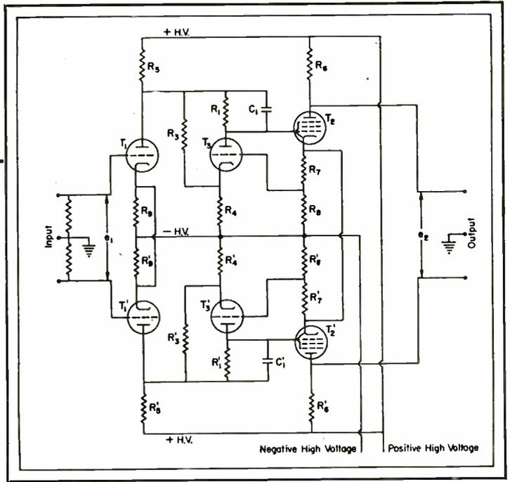
An aperiodic coupling element permits response to zero frequency and to high frequencies limited only by conventional limitations in RC coupling. Useful in CR-tube deflection; has a voltage gain of 5000
