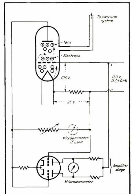
FIG. 7—Circuit for an ionization gage, using a triode tube
