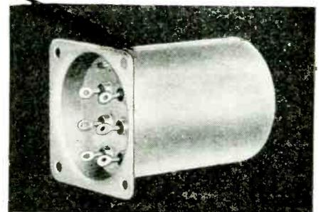
5. Completed assembly after operating atmosphere has been introduced and tubulation sealed off.
