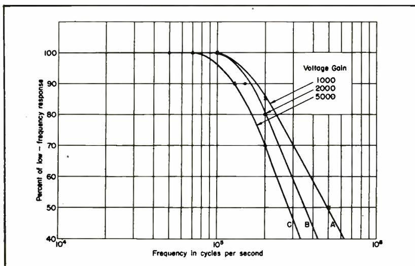
Fig. 6—High-frequency response characteristic of the amplifier
