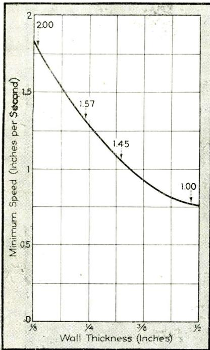
FIG. 4—Scanning speed required for hardening various wall thicknesses by self-quenching, down to 1/8-in. Numbers on curve refer to power requirement relative to lowest
