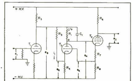
FIG. 2—Basic circuit in which a tube,  $T_3$ , stabilizes the amplifier
