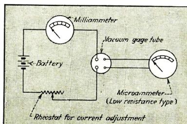
FIG. 4—Circuit for thermocouple vacuum gage
