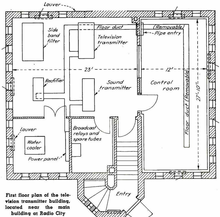
First floor plan of the television transmitter building, located near the main building at Radio City
