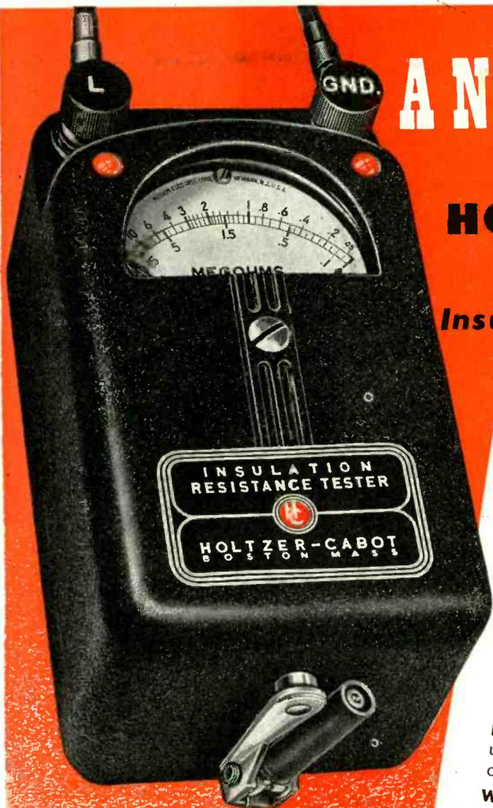
**Hand Generator** — eliminates batteries and external power supply. Delivers 500 Volts D.C. testing voltage regardless of the direction in which crank is turned.
