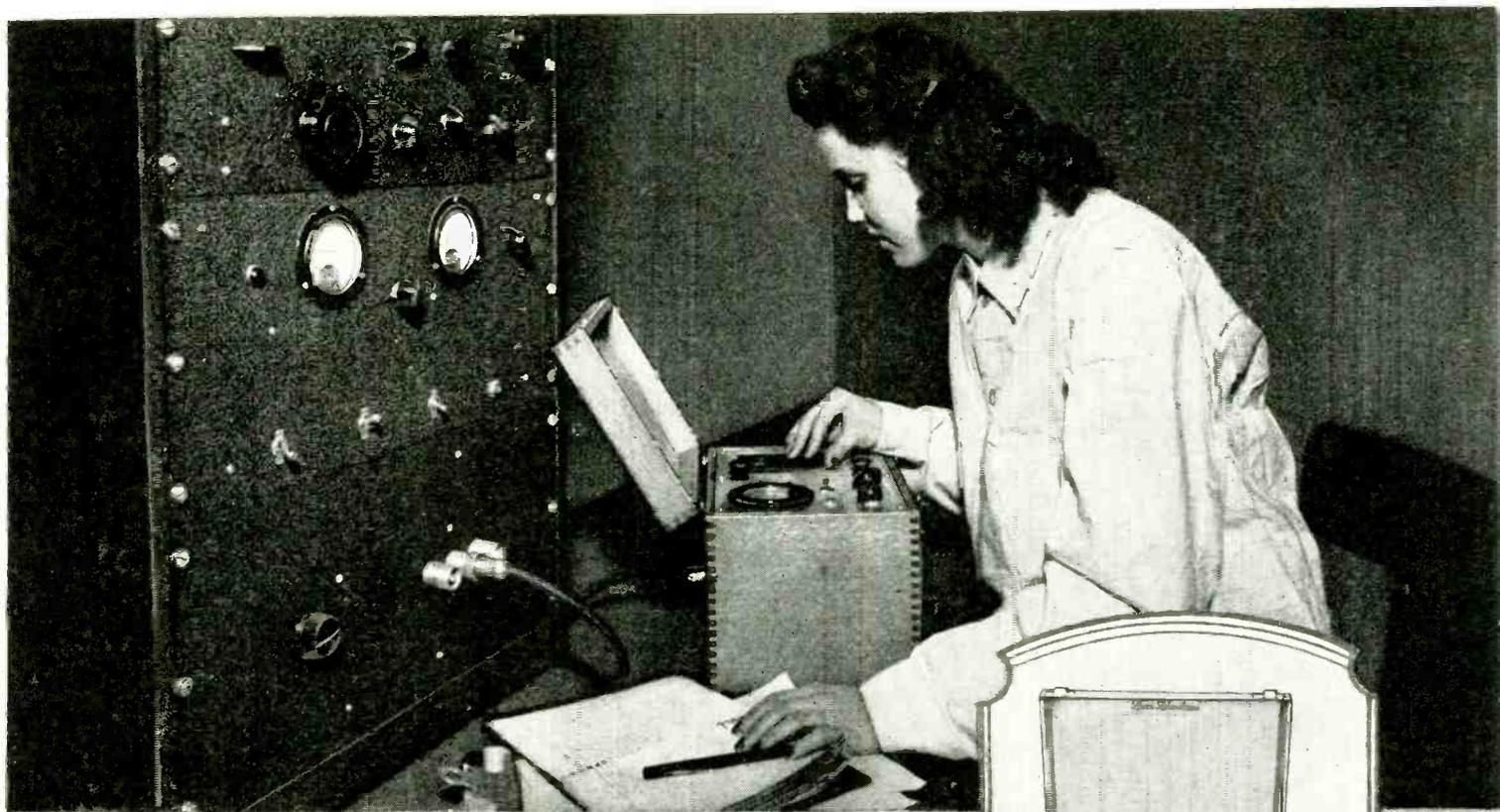
*Calibration of a Lavoie Precision Frequency Meter, using a Crystal Calibrator developed in our laboratories*
