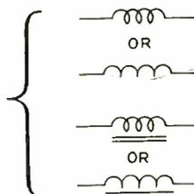
NOTE: When it is desired especially to distinguish magnetic core inductors, a line or lines parallel to the axis of the loops should be used.
