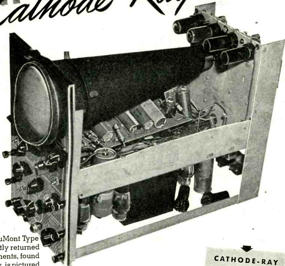
Several badly damaged DuMont Type 208 oscillographs were recently returned for repairs. One of the instruments, found to be definitely beyond repair, is pictured herewith. The main chassis was bent in two directions. The main bank was torn from its fittings, every lead wrenched free from its soldered connection. The panel was badly dented and twisted. Several tubes were jolted from their sockets. The instrument was only good for salvaged components. Yet . . .
