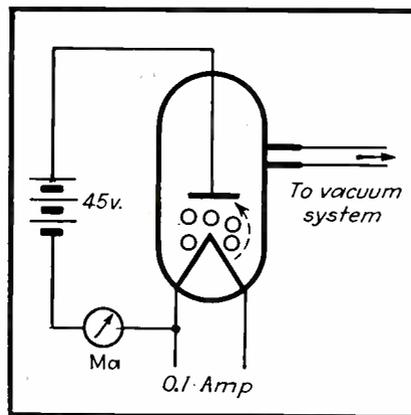
FIG. 8—An emission gage using a diode tube
