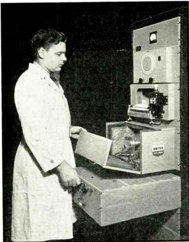
Air-operated vibration generator designed especially for testing aircraft radio equipment
