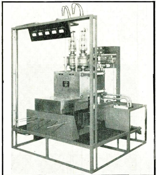
Final f-m amplifier of WMFM in Richfield. Plates are water-cooled, and jets of cool air are forced around grid and filament leads. Shafts in foreground are for tuning and neutralizing
