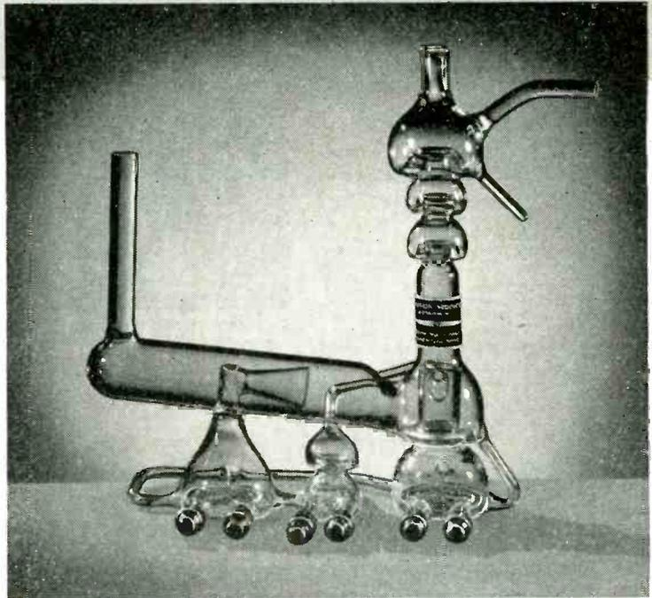
*Glass Fractionating Diffusion Pump, Type GF-5A*
