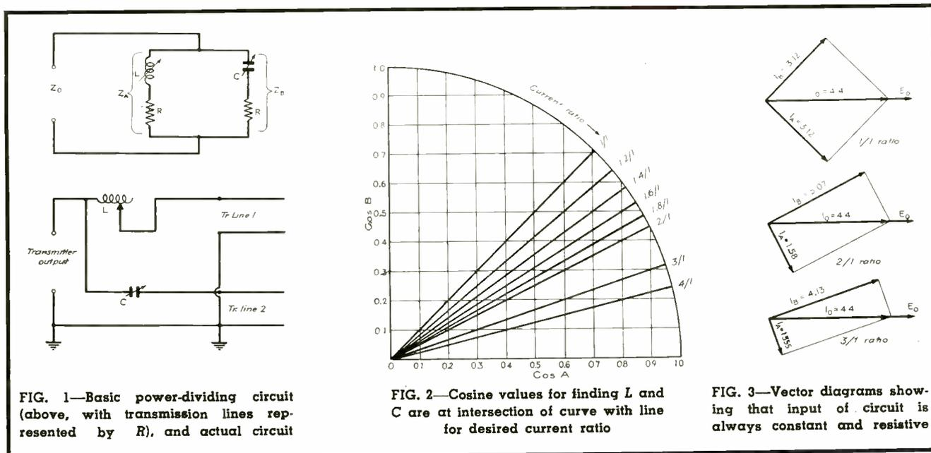
FIG. 1—Basic power-dividing circuit (above, with transmission lines represented by  $R$ ), and actual circuit
