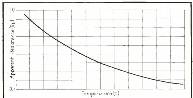
FIG. 2—Same data as in Fig. 1, plotted on semi-log paper to show linear relationship
