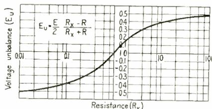
Voltage unbalance of a Wheatstone bridge plotted against the value of the variable thermometric resistance in one arm of the bridge, for a constant impressed voltage  $E$  and equal resistance values  $R$  in the other three arms of the bridge
