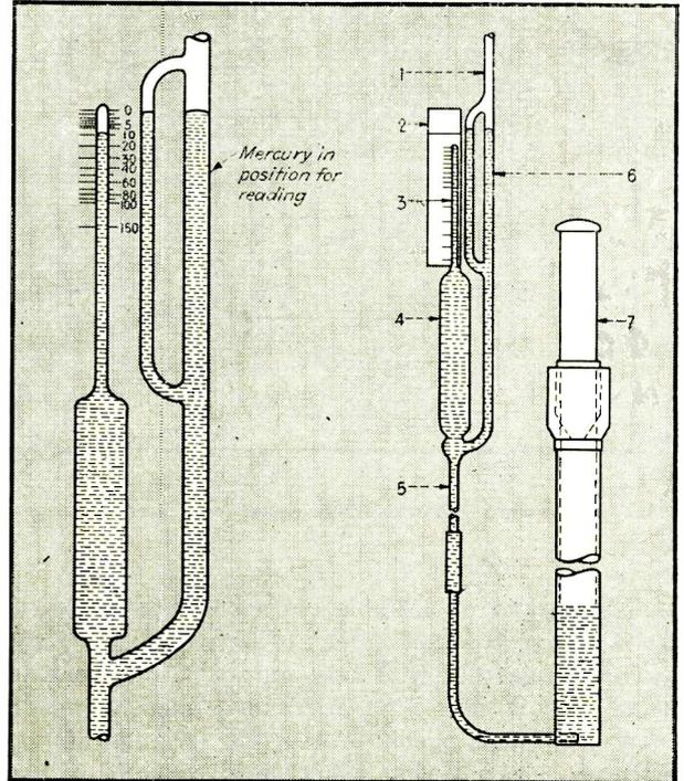
FIG. 2—The barometer vacuum or McLeod gage
