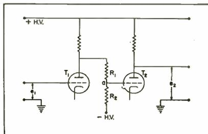
FIG. 1—Hypothetical circuit for direct coupling between two tubes
