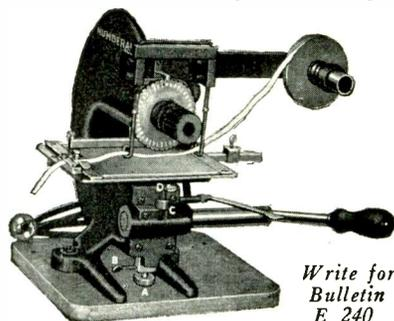
An ideal machine for hot stamping letters and figures on plastic nameplates, and other small parts, with the use of colored roll leaf. Furnished with an electric heating element, and rheostat for regulating heat. All figures and entire alphabet are on one dial.
