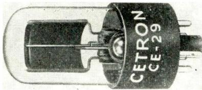
octal 5-pin base, interchangeable with similar tubes produced by other manufacturers. This tube is similar to the manufacturer's type CE-30. These two tubes together may be used to convert equipment from being red sensitive to blue sensitive and vice versa. CE-29 is particularly sensitive to blue and violet light near the short wavelength limit of visibility. Bulletin No. PC-15.
