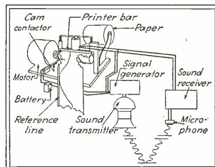
Fig. 3—A continuous recording of depth may be made by permitting the impulses of the reflected waves to actuate a printer mechanism
