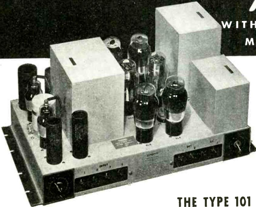
Input impedance 600 ohms and bridging. Gain 600 ohm input 61 db., bridging input 46 db. Frequency response 30 to 16,000 c.p.s. either input—600 ohm output  $\pm 0.5$  db., 30 ohm output  $\pm 1$  db. Power output—production run average: +47 V.U. with less than 3% RMS harmonic content.
