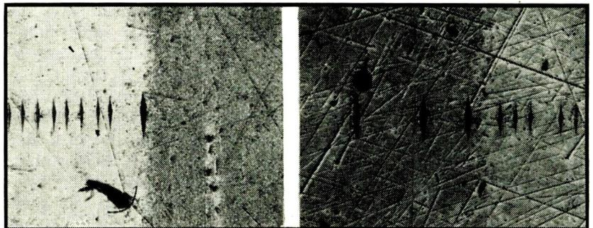
FIG. 5—Appearance of hardness-testing indents at 100 times magnification. These micrographs show a 20-mil layer with several impressions in a line from the core to the edge. The micrograph at the left is SAE 1095 steel, while the one at the right is SAE 4340 alloy steel. (Courtesy Wilson Mechanical Instrument Co.)
