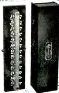
Left—Type 53 Interior Junction Box showing Type 53 Terminal Strip. Terminals providing solder clips on cable side and screw connections on drop side are mounted in specially selected kiln dried maple terminal strip. Furnished in 13 and 26 pair capacity.
