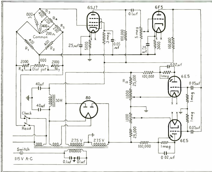
Bridge circuit and electronic amplifier used to feed the grids of the 6E5 indicator tubes. The plates of these tubes are supplied with a.c. by the high-voltage winding of the power transformer
