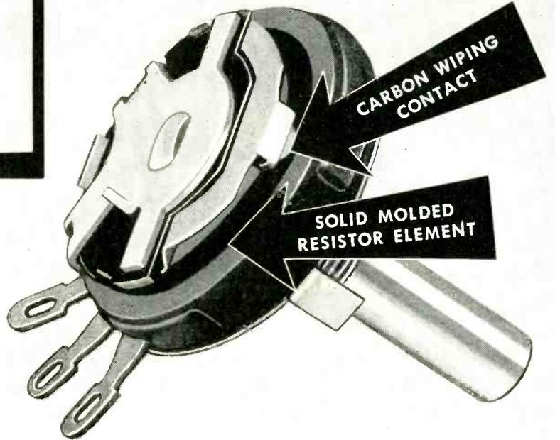
Type J Bradleyometer showing how low-resistance carbon brush makes a smooth contact with the resistor element.
