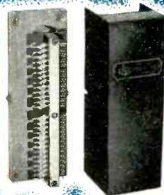
Left—Type 52 Interior Junction Box showing Type 52 Terminal Strip. Furnished in 10, 20 and 26 pair sizes. Special sizes up to 52 pairs to order. Solder connections for permanently low resistance. Terminal block of heavily tinned, formed metal clips set into hard rubber insulation.
