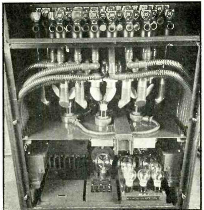
Smoke-detecting cabinet with front panel removed to show pipes going to various parts of a ship. The lamps under the pipes make faint smoke visible in windows under the numbers in the pipe outlets, and the large lamp at bottom center provides light for the photoelectric cell
