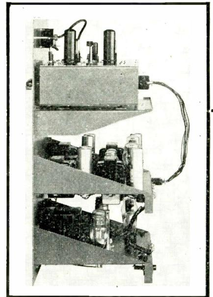
Right profile showing the arrangement of component parts and tubes in rack-and-panel instrument
