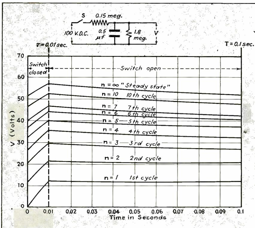
FIG. 3—Output voltage plotted against time for the first seven cycles, the tenth cycle and the final steady-state condition in the circuit shown, for the numerical values and waveform assumed in the example
