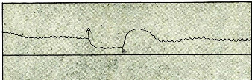
FIG. 4—Inkwriter record obtained by a Valsalva experiment with the photoelectric plethysmograph. The dip between points A and B indicates increased congestion and corresponding higher ear density
