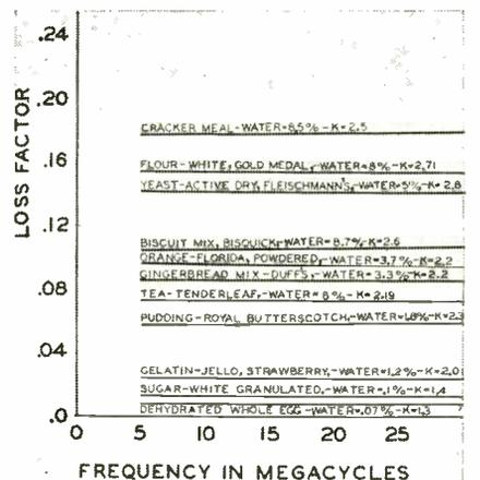
The relation between electrical loss factor and frequency is shown by the curves above for a representative selection of foods
