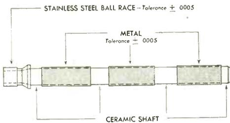
**I**LLUSTRATED is a "precision condenser" equipped with Stupakoff insulators and metallized ceramic sub-assembly.
