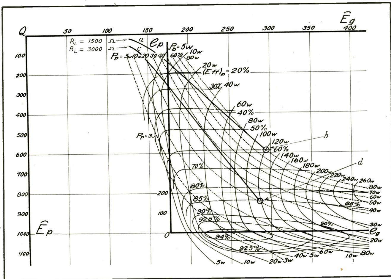
FIG. 2—Chaffee contour diagram for accurate determination of the operating characteristics of a UV211 tube when  $\bar{E}_b$  is 1000v and  $\bar{E}_c$  is —175v
