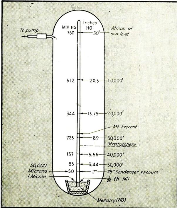
FIG. 1—Columns of mercury (Hg) at various pressures
