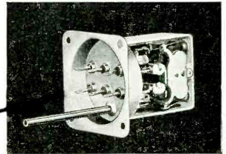
3. Relay is mounted on the base assembly and wired to the sealed terminals.
