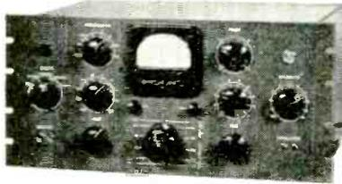
they are ideally suited for measurements on separate amplifiers, complete audio channels and transmitters of all types, including AM, FM and Television Audio. These or the preceding models of the same series are in use in nearly every medium or large station, in network studios and in the laboratories and test set-ups of most manufacturers.
