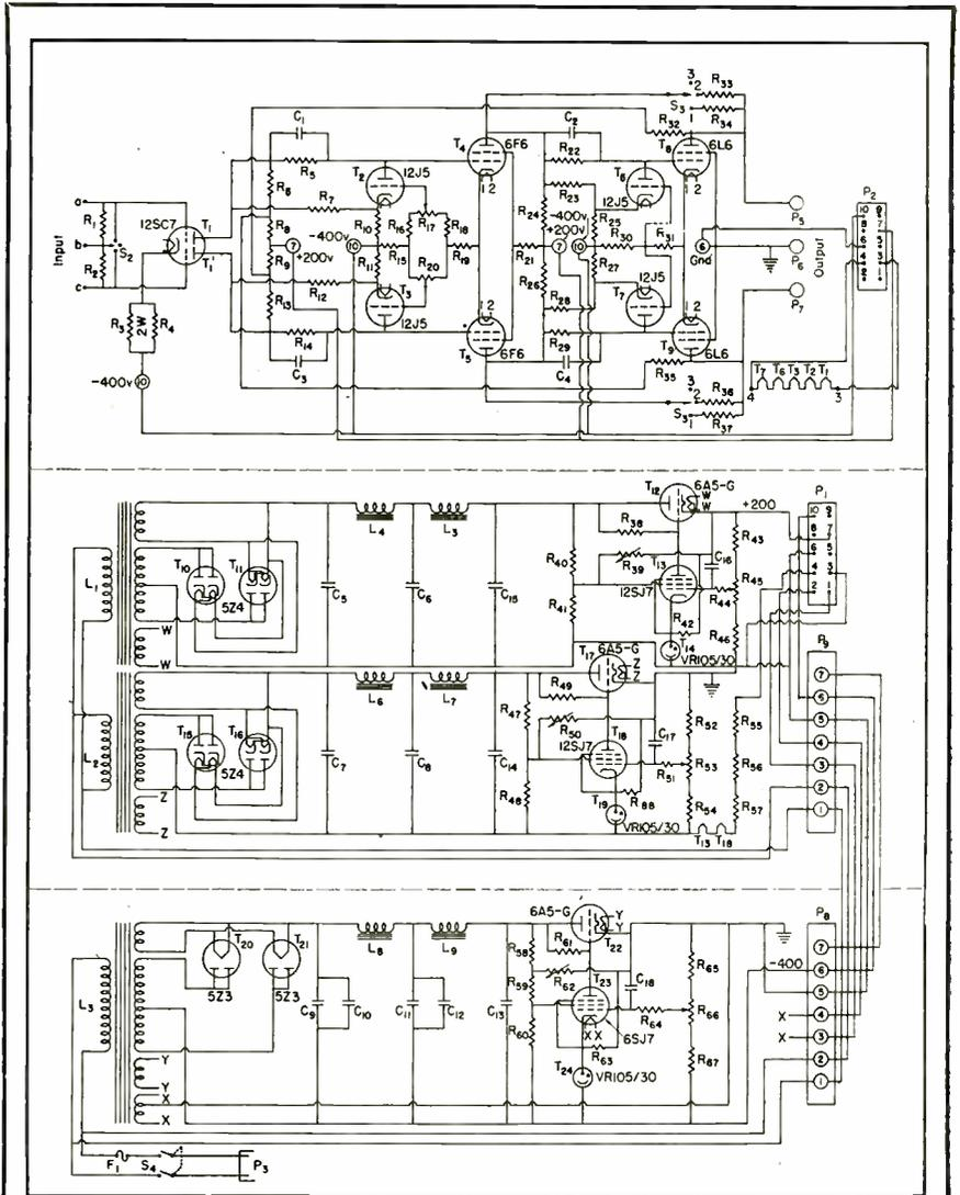
FIG. 5—Schematic of complete stabilized direct-coupled amplifier. Parts list is given in the accompanying text
