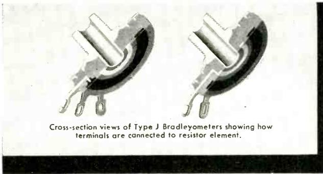
Cross-section views of Type J Bradleyometers showing how terminals are connected to resistor element.
