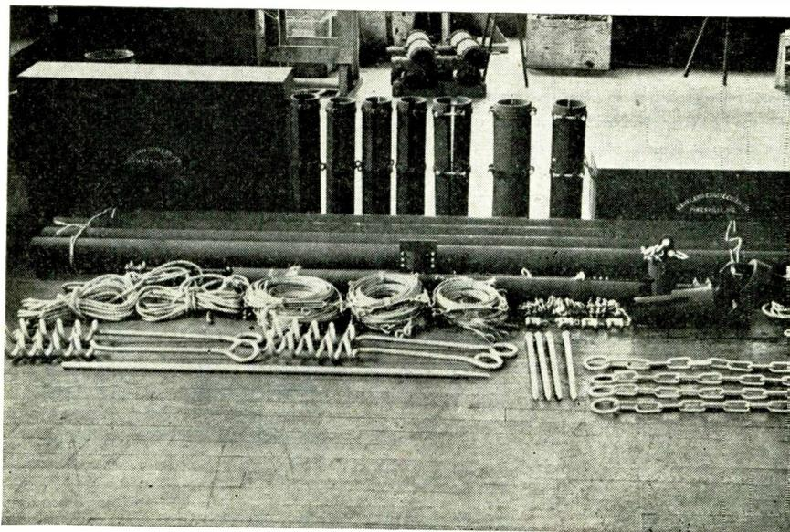
Complete kit of units forming the plywood antenna mast that is flown to captured airfields for ground-to-plane communication by the Army Air Force. Three men can erect it in 30 minutes
