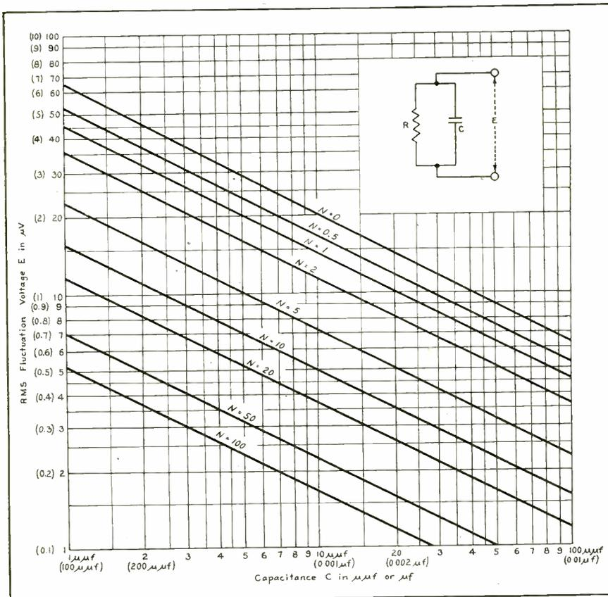
Chart giving rms value of fluctuation voltage across  $R$  and  $C$  in parallel, between a given frequency limit and infinity. The frequency limit is converted into a value  $N$  as explained in the accompanying article. When values in parentheses are used on one scale, the parenthesis values on the other scale must be used
