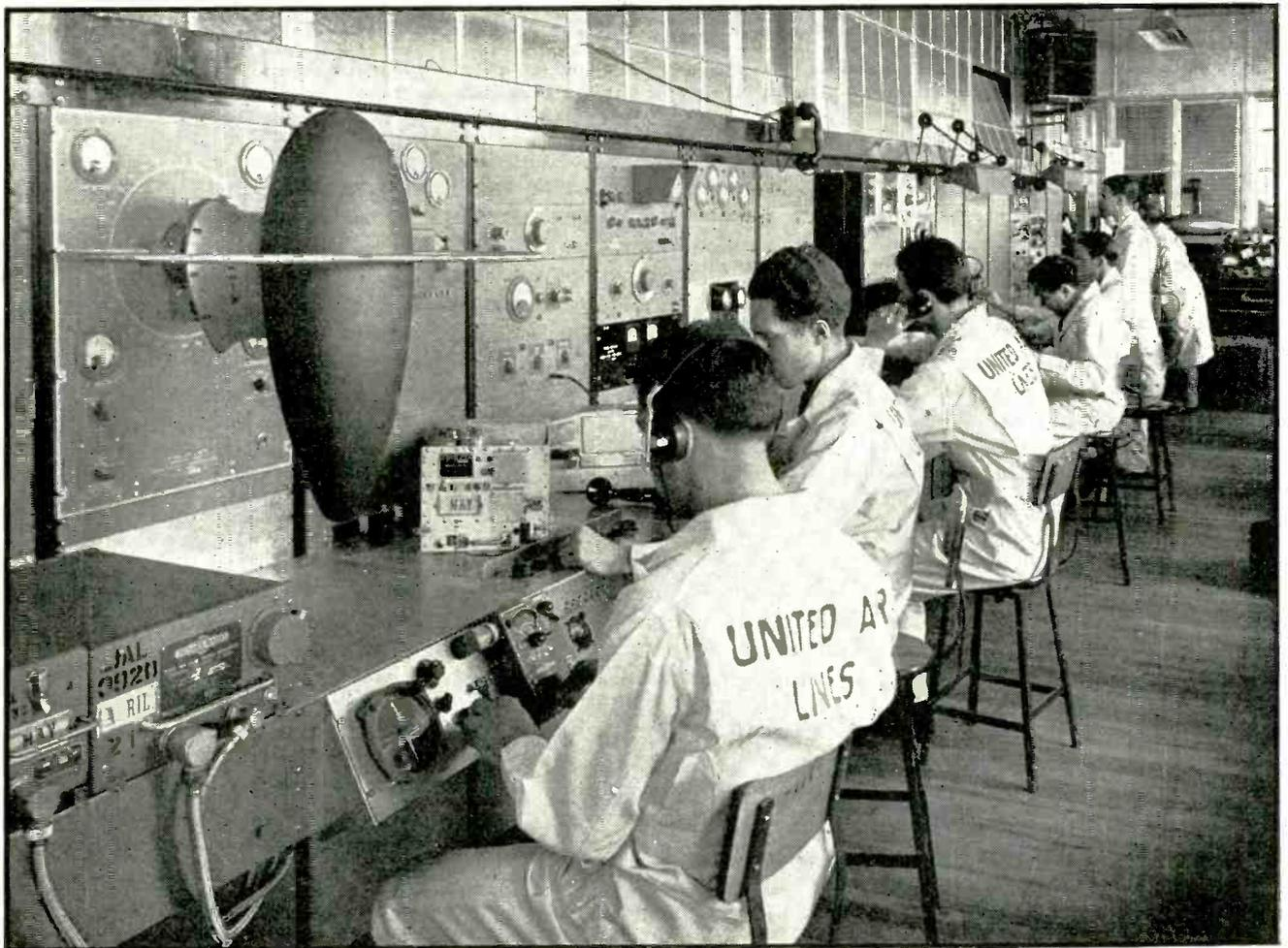
Test panels in the radio-electric department of United's base in Cheyenne. Left to right: Automatic direction-finder test panel; receiver test panel; interphone and loop test panel; oscilloscope for visual checking; a-f signal generator and vacuum-
