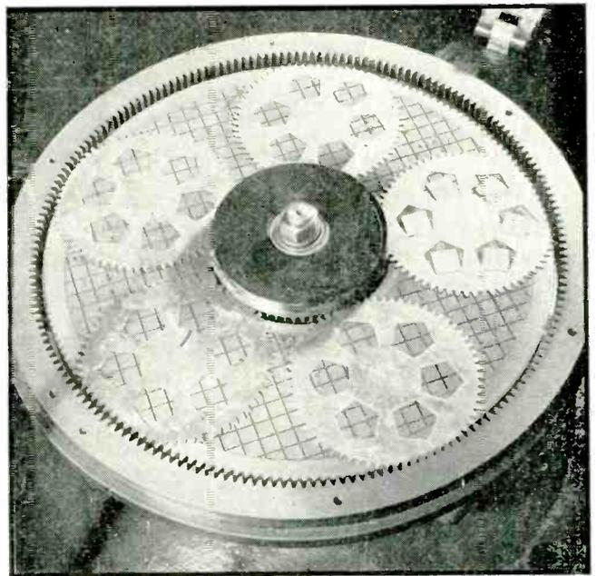
ABOVE: In one step of the grinding process, the quartz wafers are placed in pentagonal holes in planetary gears that revolve and rotate with abrasive between two cross-grooved plates
