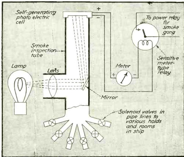
Air samples drawn from each protected space in a ship are examined by a smoke-detecting unit containing a self-generating photoelectric cell and a light source
