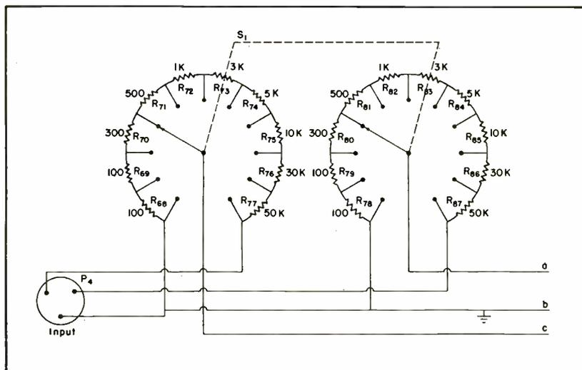
FIG. 7—Input attenuator detail. Each resistor is a  $\frac{1}{2}$ -watt unit
