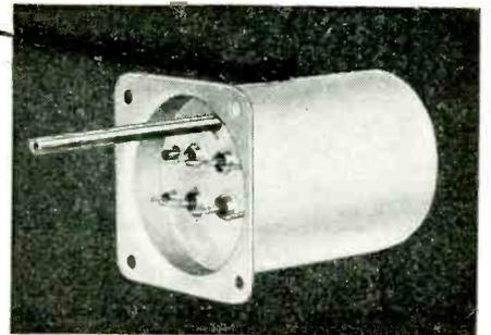
4. Steel enclosure is placed over the relay base assembly and hermetically sealed to the base. Filling gas is inserted through metal tube.
