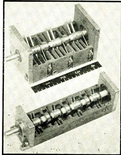
German variable capacitors used in current production. Steatite shafts insulate the molded alloy rotor section, permitting grounding of the one-piece molded alloy stator. Grooves in rotor plates permit spreading apart or squeezing together rotor surfaces for precision tracking
