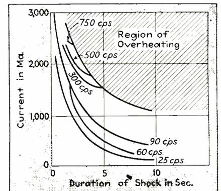
FIG. 7—Minimum currents necessary to cause death from shocks of different duration at several frequencies
