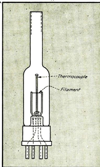
FIG. 3—Thermocouple vacuum gage tube
