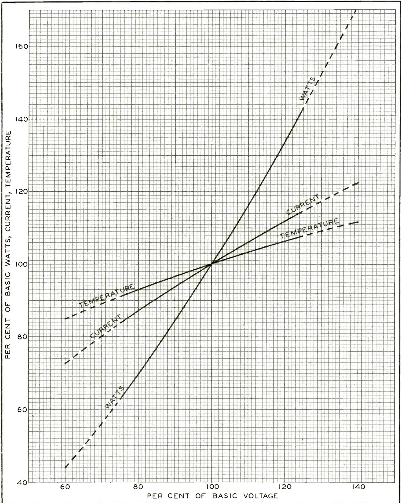
FIG. 1—Chart giving wattage, current and temperature of a filament or heater at operating voltages up to 25 percent above or below basic voltage, with sufficient accuracy for most engineering purposes. Accuracy drops in dotted regions
