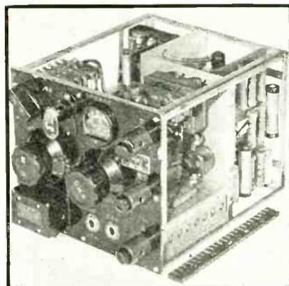
Modern Japanese aircraft radio transmitter, a part of the Model 99 Type 3 set. Values of resistors and capacitors are marked in English, and American chassis construction is employed
