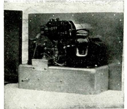
Internal view of the components and their mountings in the strain gage test set. The gain of the amplifier is adjusted by the shaft at the rear of the chassis
