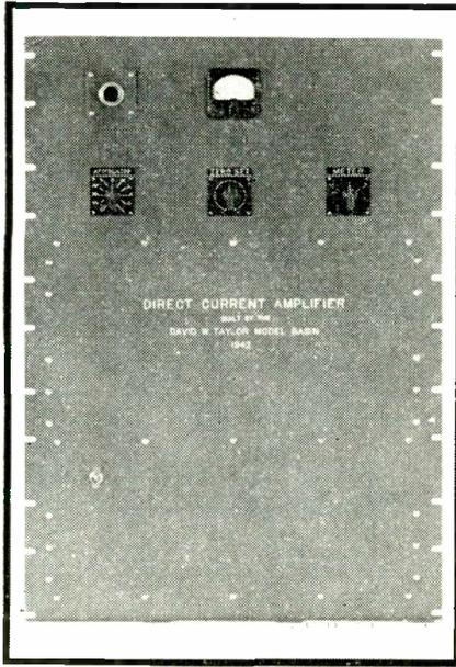
Front elevation of the oscilloscope-deflection amplifier having a voltage amplification of 5000
