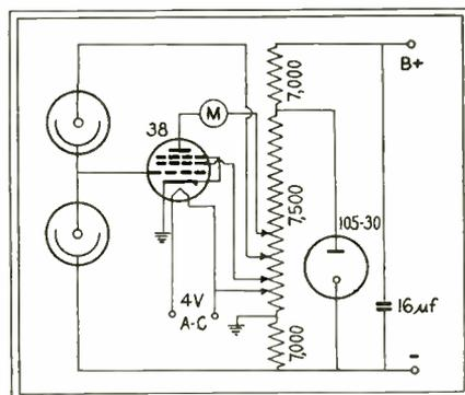
The circuit of the microdensitometer contains a 0-200 microammeter to register the unbalance of the bridge circuit formed by the phototubes. Not shown in the diagram, a 150,000-ohm resistor is in series with the meter to limit the current to slightly less than full-scale deflection of the pointer
