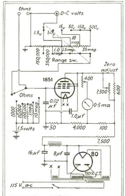
Fig. 1—Complete circuit of the electronic voltmeter using a 0.5 ma milliammeter. Voltages ranges from 1.5 to 500 volts are covered with an input resistance of one megohm per volt
