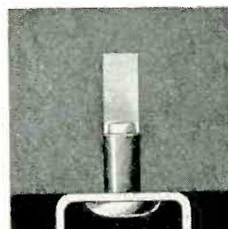
Here's a close-up of how the Cherry Rivet is fastened tight in a solid base. Note it holds by shank expansion alone—no head.
