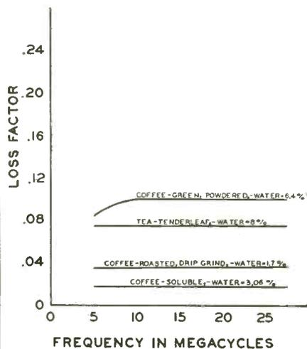
Loss factor curves for tea and three forms of coffee, ground, drip and pulverized, show that the loss factor is substantially independent of frequency
