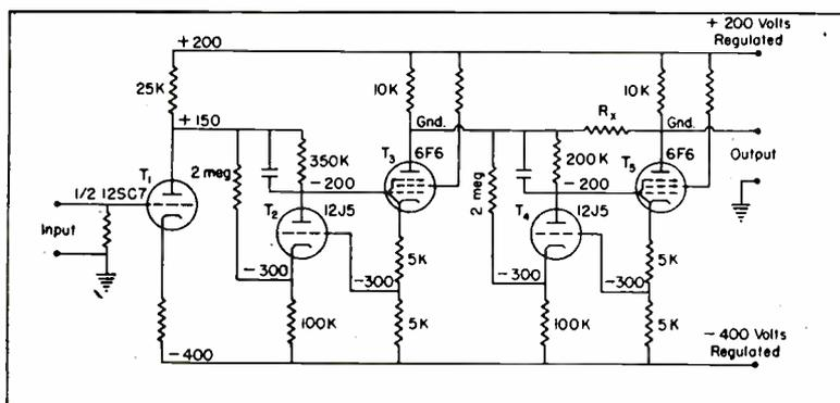
FIG. 4—Cascaded direct-coupled amplifier, showing voltages with respect to ground. For reasons stated in text, this circuit proved impractical
