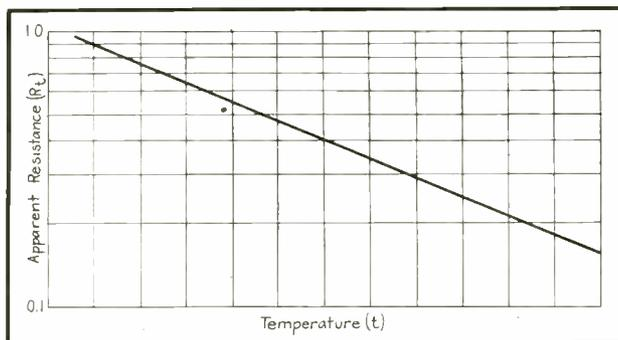
FIG. 1—Typical thermometer bulb characteristic plotted on rectangular coordinates
