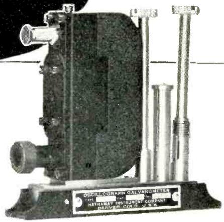
The HATHAWAY Type OA-2 OSCILLOGRAPH GALVANOMETER employs a magnetic circuit of unique design, combining for the first time, high sensitivity with small size. Universal mounting is  $\frac{3}{8}$ " wide, allowing Type OA-2's to be mounted side by side on  $\frac{3}{4}$ " centers. Therefore, oscillographs using this galvanometer may use more elements in a given space.
