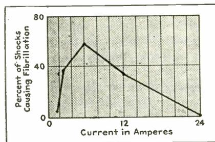
FIG. 3—Effect of electric current on susceptibility of sheep hearts to ventricular fibrillation. Each shock was applied for 0.03 sec at 60 cps, in the most sensitive part of the cycle
