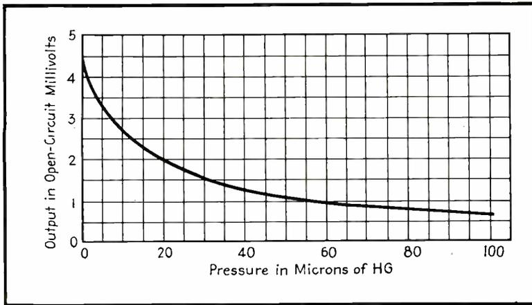
FIG. 5—Characteristic curve for a thermocouple vacuum gage
