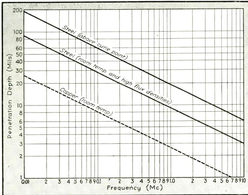
FIG. 1—Penetration depth vs. frequency for steel in the process of being hardened. A curve for copper is shown for reference
