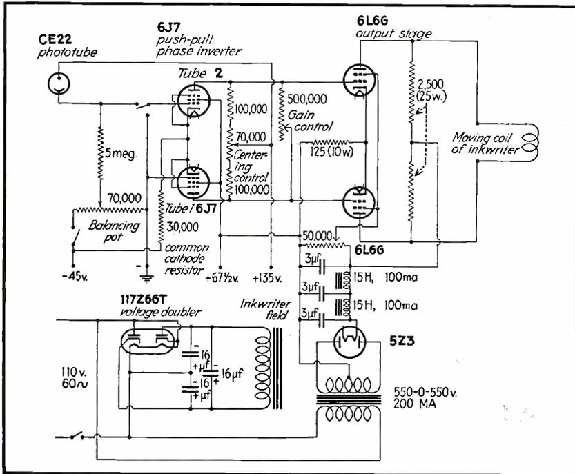
FIG. 3—Push-pull amplifier circuit used with the plethysmograph to actuate one pen of a six-channel Grass electroencephalograph
