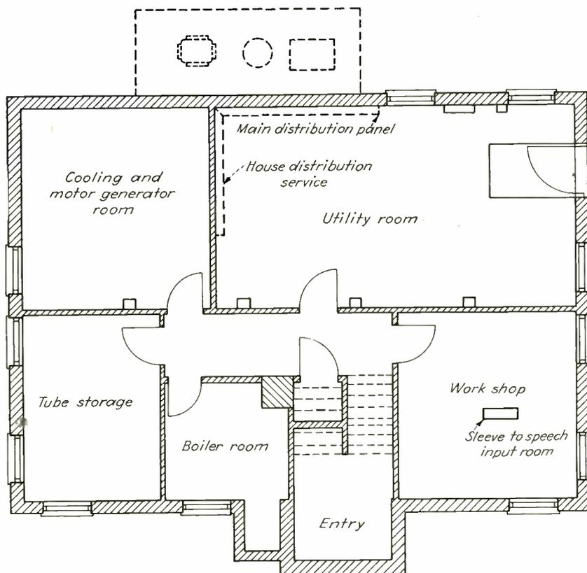
Basement floor plan of the f-m transmitter at Richfield. A work shop, boiler room, and tube storage racks are provided. Cooling equipment for the water-cooled tubes and motor generators are also housed in the basement
