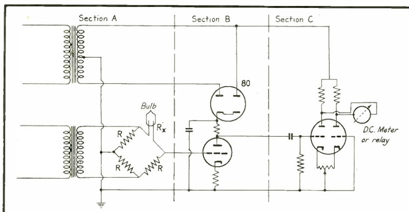
inator element which receives the a-c signal and produces a pulsating direct current flow between the plates of the two triodes to actuate either an indicating meter or a sensitive relay. This section is essentially an a-c Wheatstone bridge with one triode section serving as the variable resistance element.
