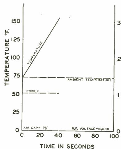
Change of temperature and power with heating time for Bisquick mix in dry form. Here the power input remained practically constant during sterilization
