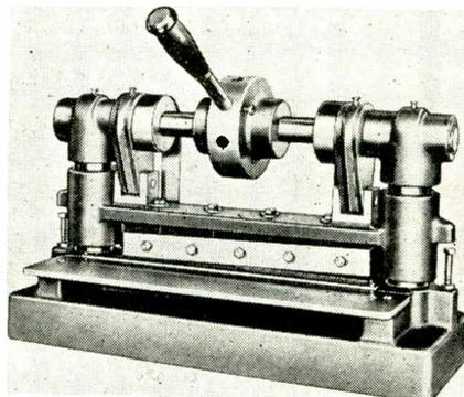
slitting and notching operations to close tolerances. Tolerance accuracy is 0.001 inches in all duplicated work. The maximum shearing width is 12 inches, and the maximum shearing capacity, for instance, on 18 gauge steel plate is
