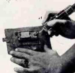
2 In die and tool departments, for grinding, finishing and touching up dies, molds, jigs, etc.
