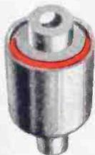
**SILENTBLOC MOUNTING** to control vibration from motor, cushion shock loads, isolate vibration between parts of equipment or isolate delicate instruments and controls from foreign vibration. Engineered design determines rate of deflection in any plane.
