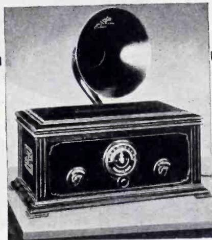
Another important step forward was achieved with this first single-dial radio produced by Magnavox in 1923. Its importance at the time is appreciated when we remember that all previous radio sets required the use of three dials for tuning in a station.
