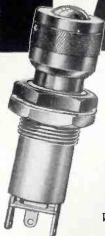
Designed especially for Aircraft, this Approved Pilot Light is compact, light, and mounts in 5/8" panel hole. Finger pressure on head of unit closes bulb-testing circuit. Turning the knurled head regulates the intensity of light. Send for details.
