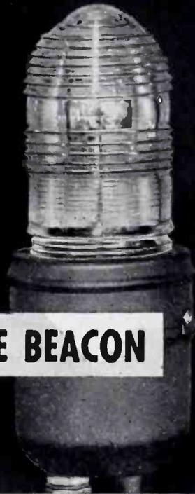
**G-E MYCALEX** was chosen for the socket of the G-E Novalux Portable Flashing Beacon for three reasons: First—the performance of this amazing material under high humidity conditions; second, because of guaranteed high mechanical strength of at least 14,000 lbs. per square inch; third, it eliminates expensive molds. G-E mycalex can be fabricated from sheets with common machining operations.
