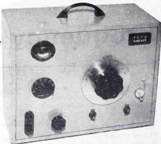
The circuit-constant checker. At the left are the tuning indicator, band selector, connections for external vtvm, and bucking-voltage potentiometer. Below the large oscillator-tuning control are the on-off and the Q switch. External tuning-capacitor receptacle is at the right
