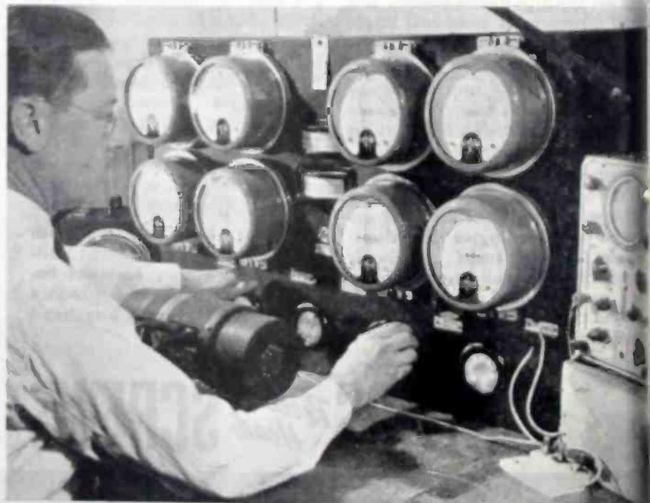
Test panel for Westinghouse dynamotors having four separate output voltages from 14 to 300 volts. Output voltages are held constant for normal input-voltage variations by a regulator field which weakens when the input voltage rises and strengthens when the voltage drops
