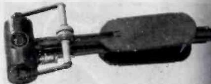
bearings to eliminate all end thrust and play occasioned by train motion and vibration.
