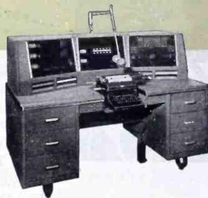
The MS-97 Remote Control Unit, built to individual requirements, provides a method of installing control equipment in a manner which will place all the equipment in locations readily accessible to the operator. The compact low structure of this unit permits it to be installed in such a way that the operator may have a full unobstructed view in all directions.
