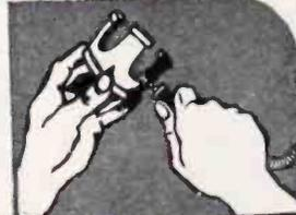
3 For de-burring, grinding, finishing, polishing and other light production jobs—particularly valuable on irregularly-shaped parts
